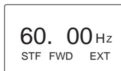
3) When the operation panel switch "正転 (Forward)" is turned ON, the motor starts to rotate in the forward direction.
