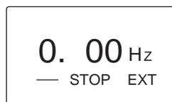
2) Set the frequency setting potentiometer to the predetermined frequency (60Hz) on the operation panel of a demonstration machine.
