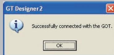
When the personal computer is correctly connected with GOT, the above dialog box will appear.
