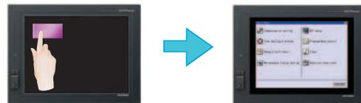
Touch the special function switch to switch the screen to applicable menu and so on.
