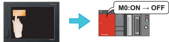
Touch the bit switch to turn ON/OFF the bit device.
