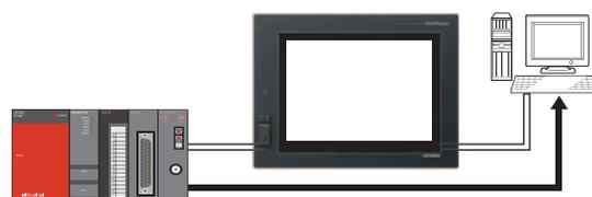
Synchronization of the GOT controller data and the information system's data library (execution system) can be done without using the communication gateway.
