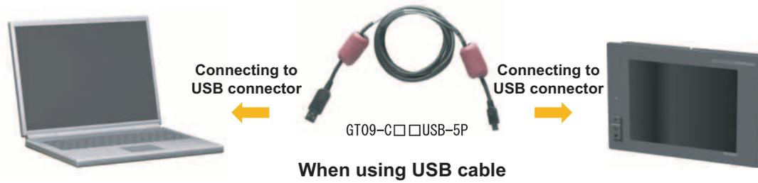
\* To make USB communication with GOT, the USB driver must be installed.
