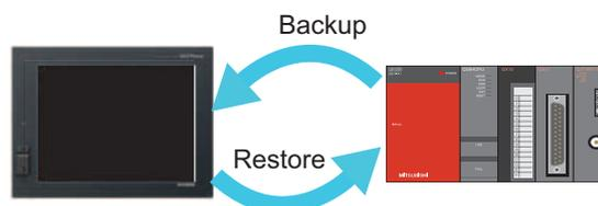
Back up setting contents for the controller, and restore through GOT.
