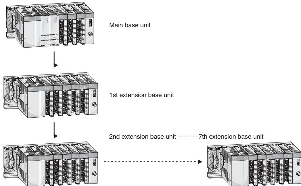
The base unit and extension units are simply connected to one another by extension cables. These connecting cables also supply the extension units with the operating voltage of 5 V DC.
