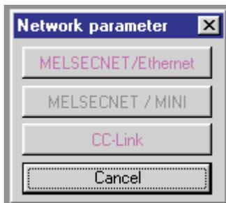
This opens up the dialogue box to allow the Ethernet module to be configured which can be seen below.
