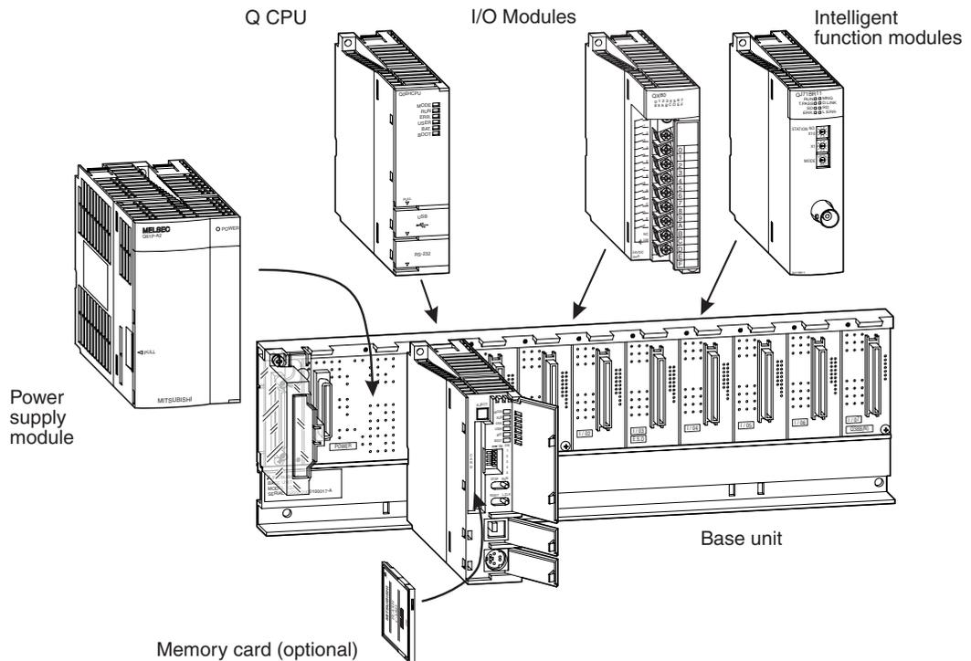
The CPU and modules are held in a base unit which has an internal bus connection for communication between the individual modules and the CPUs. The power supply module which supplies the voltage for the entire system is also installed on this base unit.
