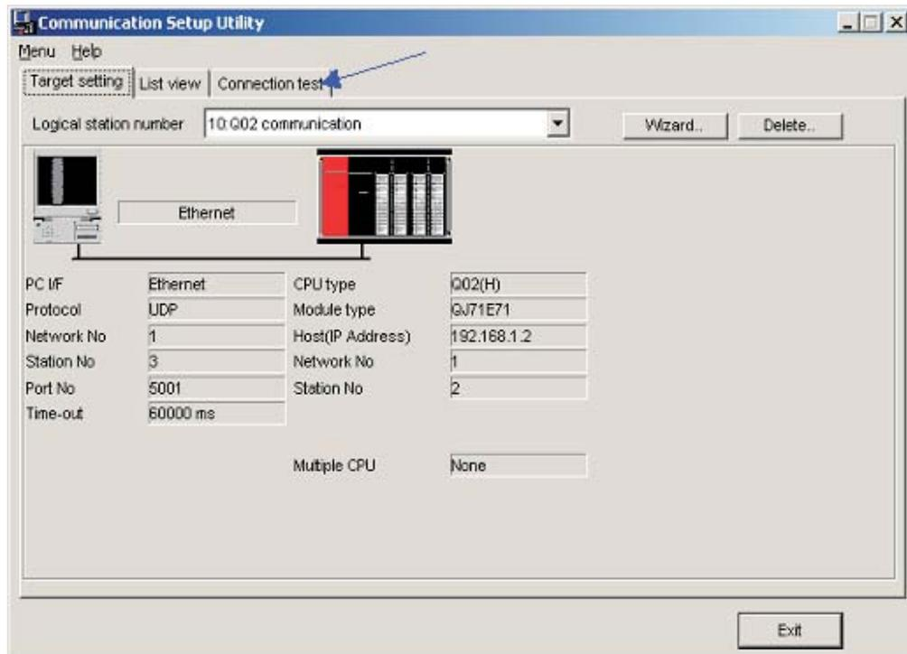
Select the **Logical station number** for which you want to accomplish the test. The **Diagnosis count** shows how many successful connection came. **Result** shows the test results. In case of an error an error number is indicated.
