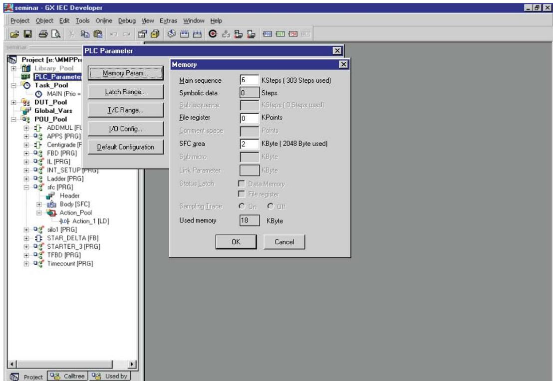
This is not the case for Q series, as Q supports SFC's in the program area. Also for FX range, SFC's actually compile to STL code in the program area.
