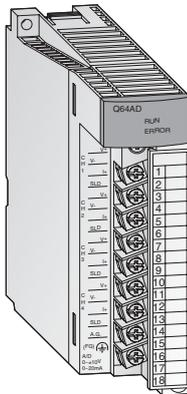
The analog input modules convert analog process signals into digital values which are further processed by the Q CPU. The A/D converter modules combine a high resolution (0.333 mV / 1.33  $\mu$ A) with a high conversion speed (80  $\mu$ s per channel).
