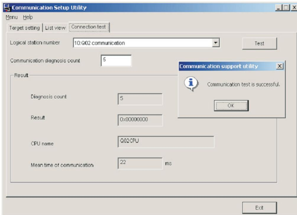
After configuring the communication paths you can access all controller devices (read/write) with Microsoft programming languages like MS Visual Basic, MS C++ etc.
