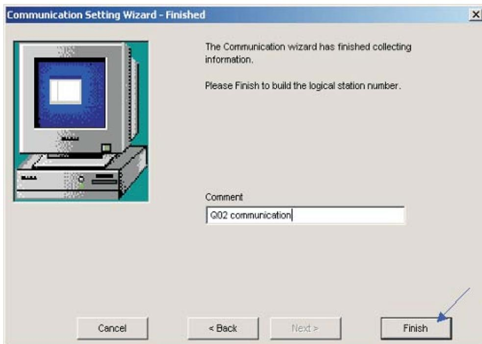
Now the definition of communication is finished. Under the folder **Connection test** the connection can be examined.
