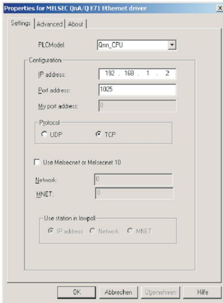
As with the MQE settings earlier, note that E71 port number 1025, decimal 1025 is equal to hex 401 (set in the PLC Local station port number – refer back to part 10 of section 18.1.1).
