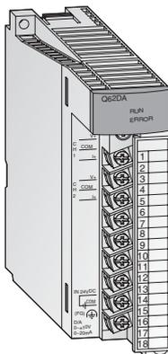
The analog output modules convert digital values into analog current or voltage signals. The resolution of 0.333 mV respectively 0.83  $\mu$ A and the extremely short conversion time of 80  $\mu$ s per output channel are only two of the many features of this modules. Isolation between process and control by means of optocouplers is also a standard feature.
