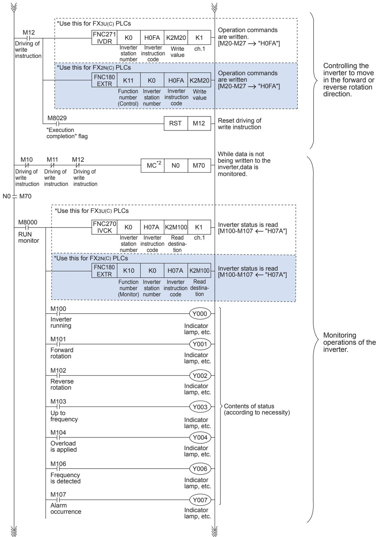
\*2. MC denotes the start of a master control block. In this example, the master control block "N0" is only executed when data is not being written to the inverter.
