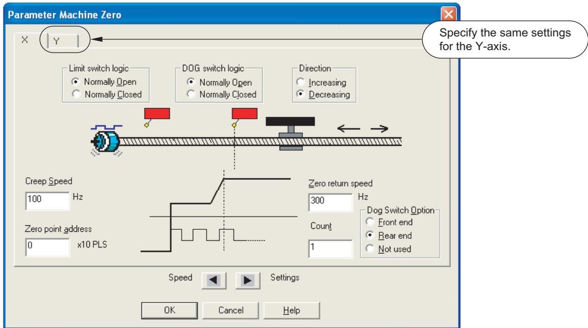
Since mechanical hardware will not be connected to the FX2N-20GM for this example, it is not necessary to configure the limit switch and DOG switch settings in the parameters. It is, however, necessary to reduce the [Creep speed] and the [Zero return speed].
