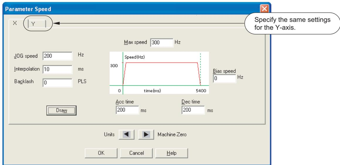
The [Max speed] is set very low in order for the VPS software to trace the path during operation through the “Monitoring Window.” In turn, both the JOG speed and interpolation value must be reduced. (In practice, it is impossible to have the JOG speed set to a value higher than the Max speed setting.)
