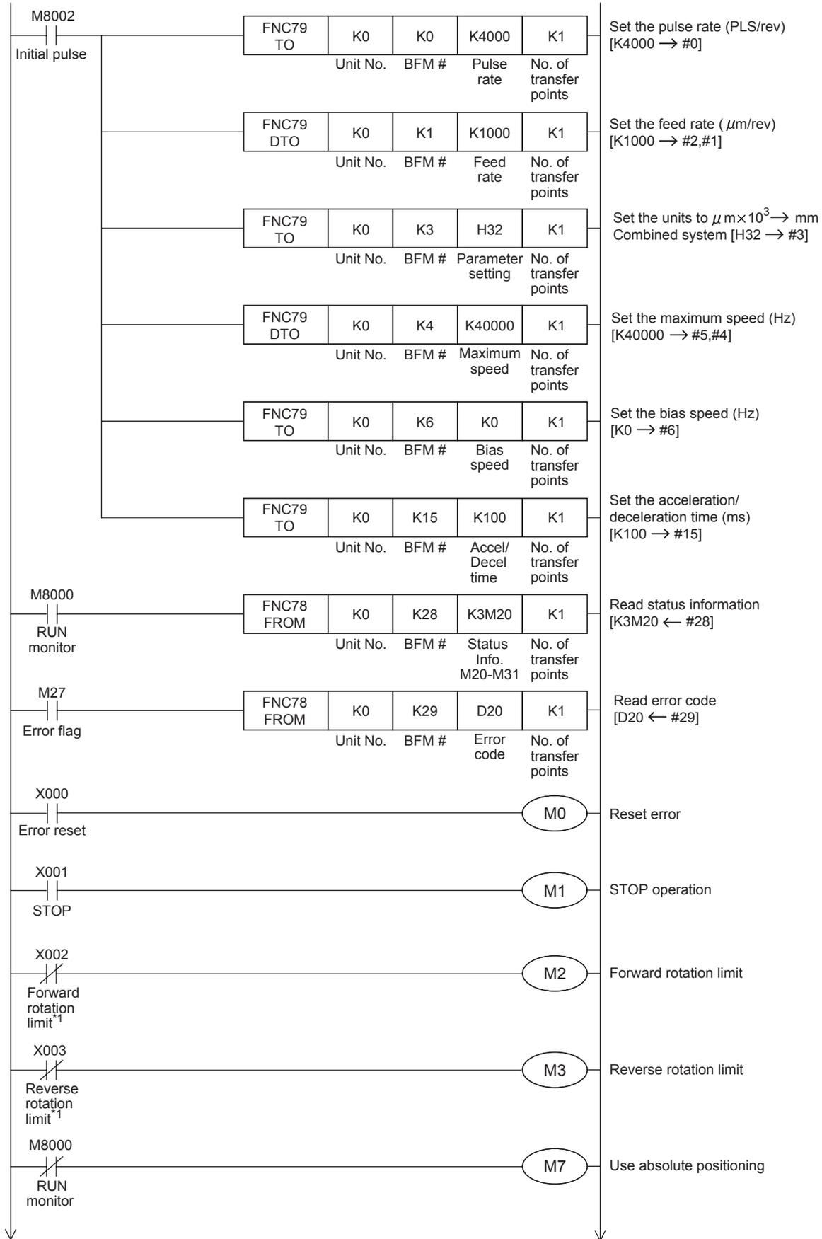
\*1. The forward and reverse rotation limit switches must be wired so that they are turned ON by default. When these limit switches turn OFF (due to the workpiece going out-of-bounds), M2 or M3 will turn ON and cause the pulse operation to stop.
