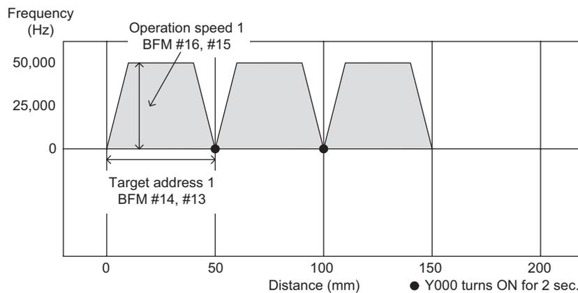
In order for the program to function correctly for the specified number of repetition cycles, the START command input (X007) must not be turned ON again during the positioning operation. If the START command is turned ON again, the counter C100 is reset, which clears the number of repetitions.
