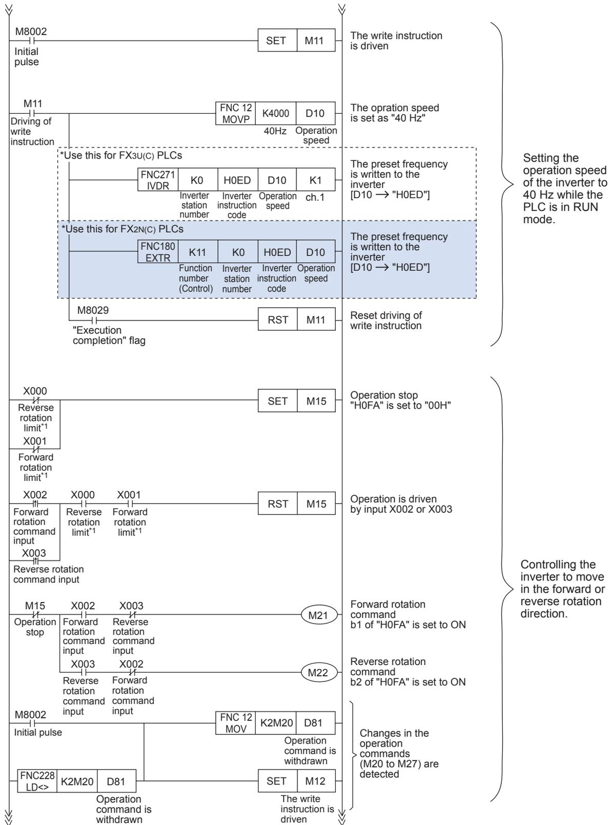
\*1. The forward and reverse rotation limit switches must be wired so that they are turned ON by default. When either of these limit switches turns OFF (due to the workpiece going out-of-bounds), the inverter operation will be stopped.
