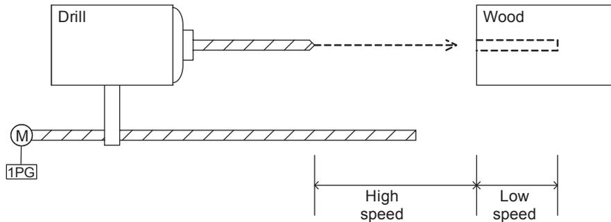
The two speed positioning operation is illustrated in the following graph. Neither the zero point return nor the JOG instructions are used in the ladder program.
