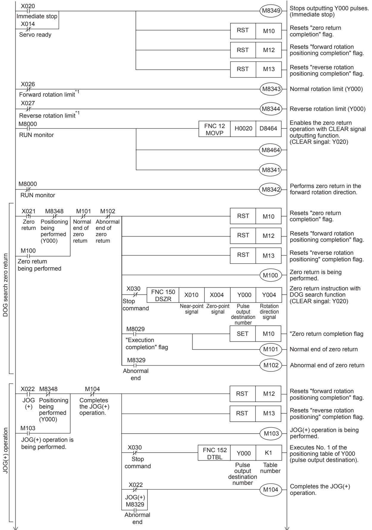
\*1. The forward and reverse rotation limit switches must be wired so that they are turned ON by default. When these limit switches turn OFF (due to the workpiece going out-of-bounds), M8343 or M8344 will turn ON and cause the pulse operation to stop.
