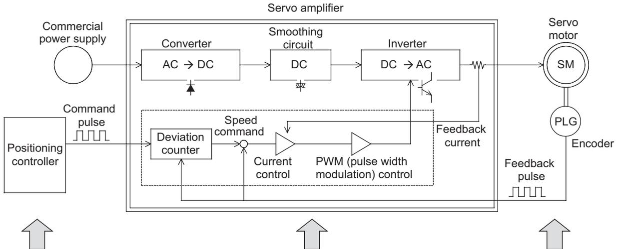
The positioning controller generates a specified quantity of forward rotation (or reverse rotation) pulses at a specified frequency.
