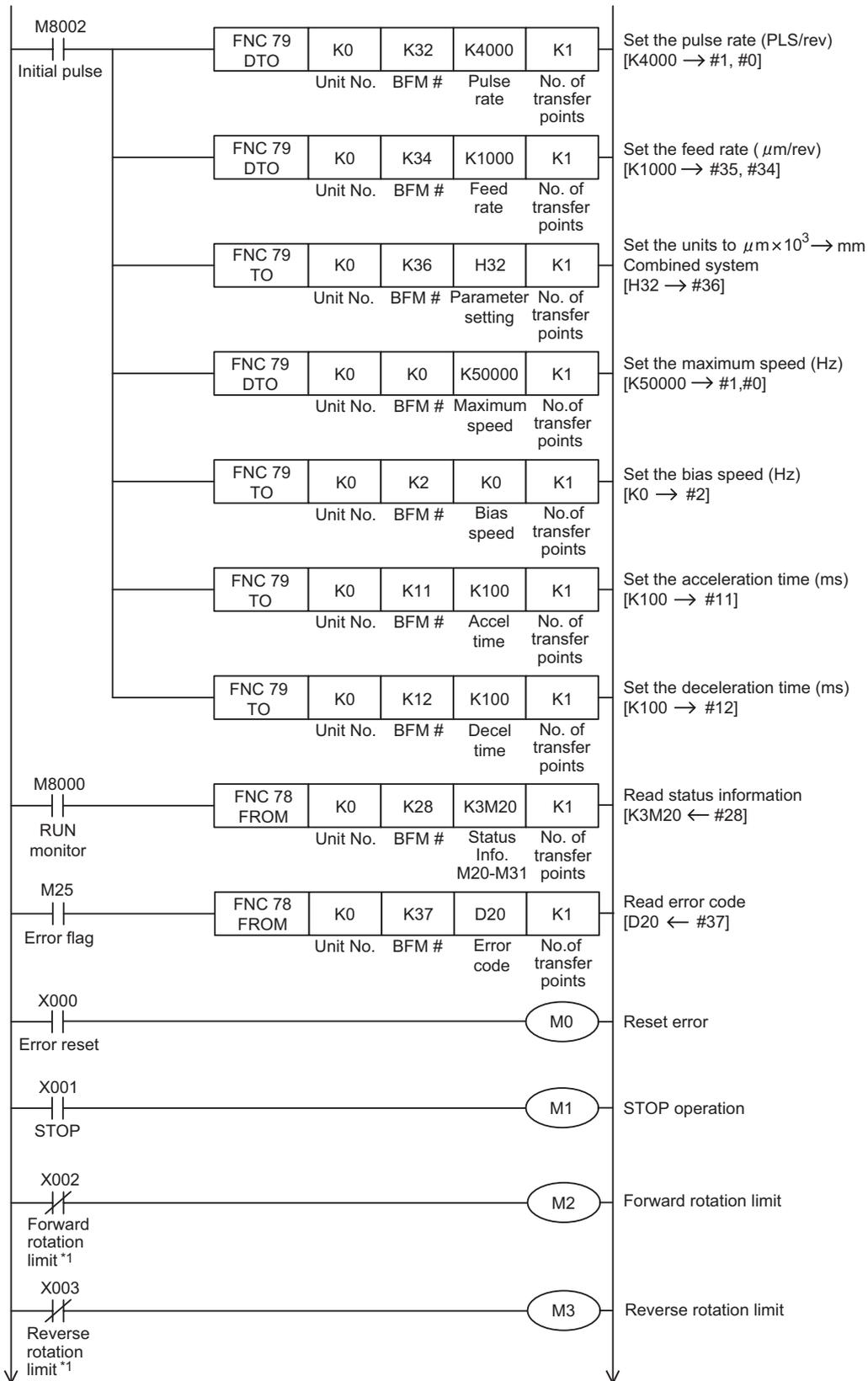
\*1. The forward and reverse rotation limit switches must be wired so that they are turned ON by default. When these limit switches turn OFF (due to the workpiece going out-of-bounds), M2 or M3 will turn ON and cause the pulse operation to stop.
