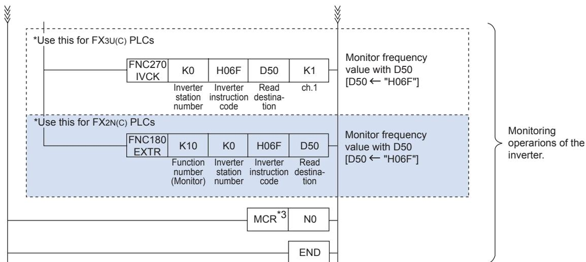
\*3. MCR denotes the end of a master control block. In this example, the master control block "N0" is only executed when data is not being written to the inverter.
