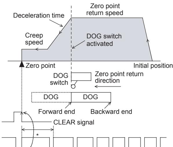
\* The location of the DOG switch should be adjusted so that the backward end of the DOG is released between two consecutive zero point signals (1 pulse per rotation of the motor).
