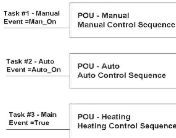
Consider our original control program. Conditional Jump (CJ) instructions could be used to isolate, either routines #1 or #2, when not in use. The Heating control routine is always required to run.
