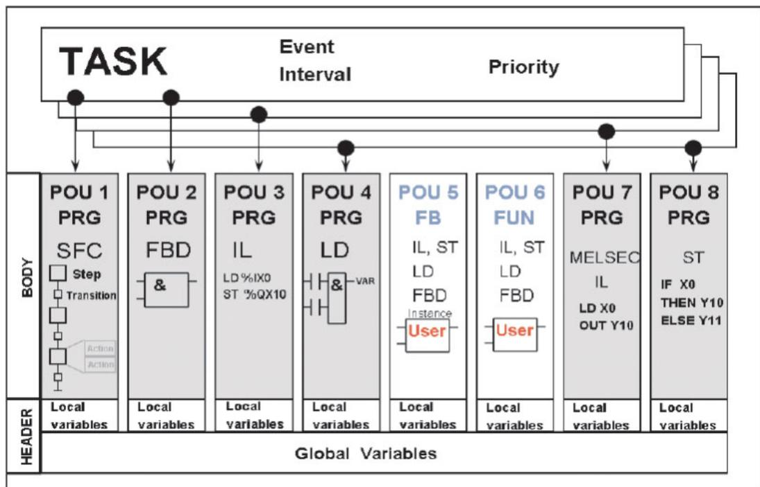
Overall Project Configuration illustrating POU integration using SFC, FBD, IL, LD and MELSEC IL and ST format programs.
