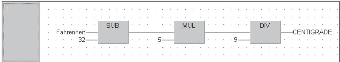
**Hint:** When entering the CENTIGRADE variable, it is not necessary to type it, simply right click on the variable box (or press F2).
