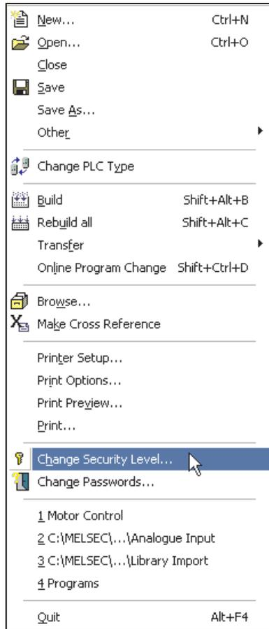
② Enter the password for 'Level 7' and if accepted, the user will be logged on at this level.
