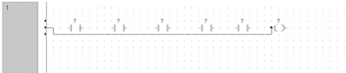
The pen can then strike through all contacts, from the bus bar, to the coil. In the Ladder Editor the suggestion is to invoke the **Auto Connect** feature when dropping elements onto the POU body or connecting parallel elements. It should however be disabled when connecting a row of contacts as shown in the following screen, or inserting a contact into an existing network.
