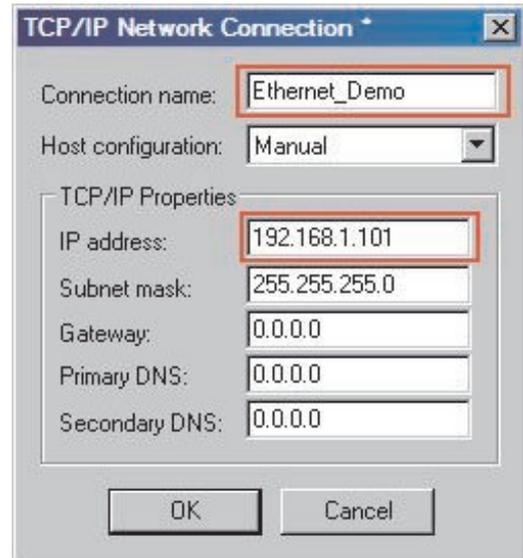
When a HMI of the E1000 series is connected to the network, the following setting is required for the FX3U-ENET (refer to section 18.2, step ④):
