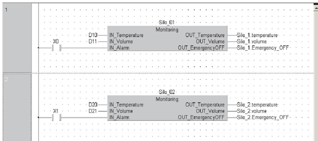
The GVL has been extended to define addresses for all elements of data unit types. Not defined addresses are handled by the system.
