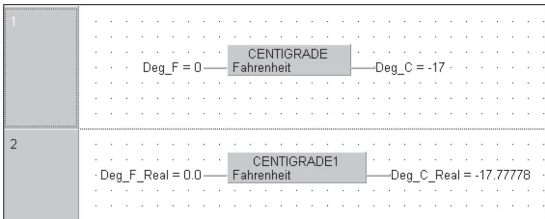
Modify the value of the input variable “Deg\_F\_Real” and observe the output result on the display. Note the 7 Digit floating point accuracy.
