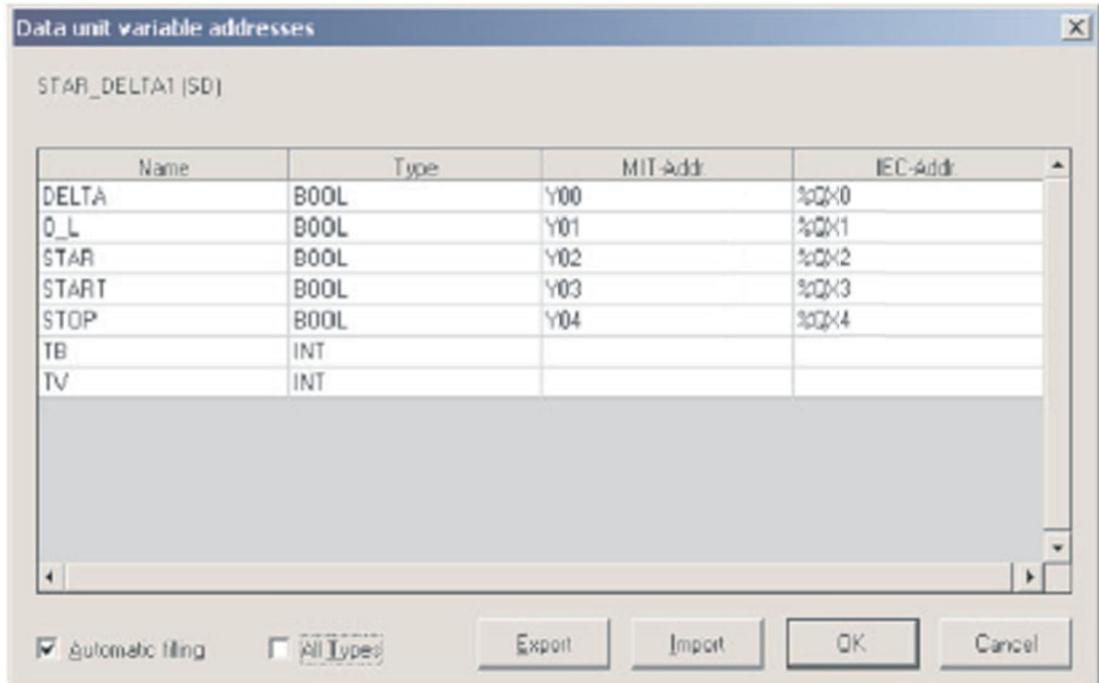
The system will try to sequentially 'Auto Fill' the variables of type BOOL. Although in many situations this is recommended, in this case it is only partially successful.
