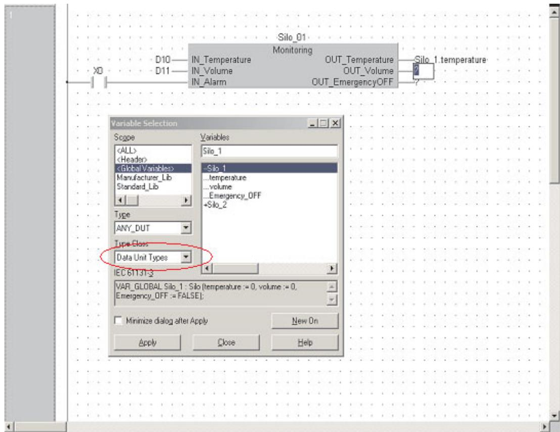
In this example a function block of the type “Monitoring” has been programmed for assigning the register value and the Boolean input to the elements of the DUTs. Two separate instances (Silo\_01 and Silo\_02 ) of this function blocks were then created for two silos.
