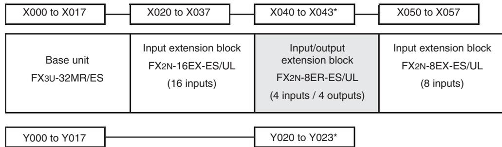
\* The inputs from X044 to X047 and the outputs from Y024 to Y027 are occupied by the FX2N-8ER-ES/UL, but they can not be used.
