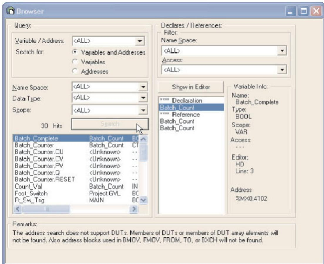
Specific variables etc. can be searched by using the query selection boxes. Individual details of the highlighted entry are then shown on the right hand side of the window.
