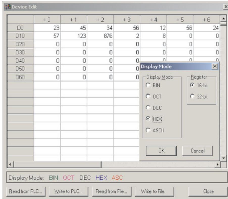
It should be noticed that the selected row now displays values in hexadecimal, the other values remain unchanged. In fact, individual cells can have different display formats, making this feature extremely flexible.
