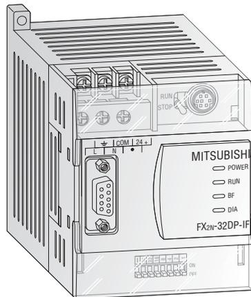
It is not necessary to install an FX base unit to a remote I/O station. The FX2N-32DP-IF connects the connected I/O modules or special function modules to the master station of a PROFIBUS/DP network.
