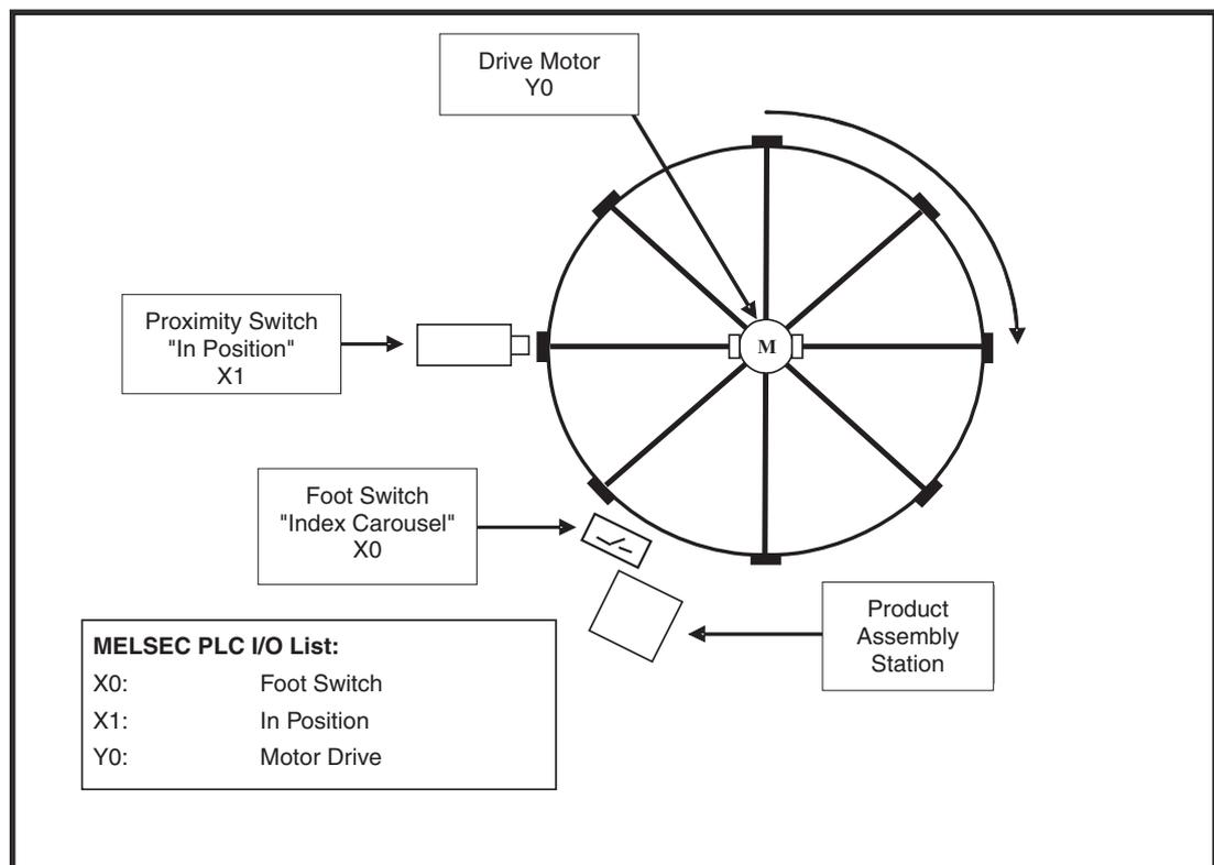
There are a number of issues that must be addressed when designing a PLC program for the above application. Using a standard Start / Stop circuit is not possible without modification due to the following difficulties:
