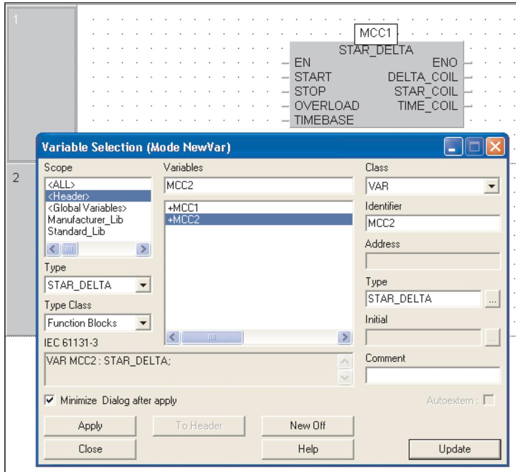
An Instance is the copy of the function block for this POU. For this example simply type MCC1 and MCC2. Notice that once entered, the instances are listed in the variable selection window as +MCC1 and +MCC2 as Type: STAR\_DELTA.
