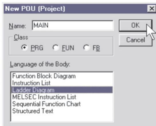
The name of the POU will be ‘MAIN’ and it should be specified as a **Ladder Diagram** of type **PRG** (Program).
