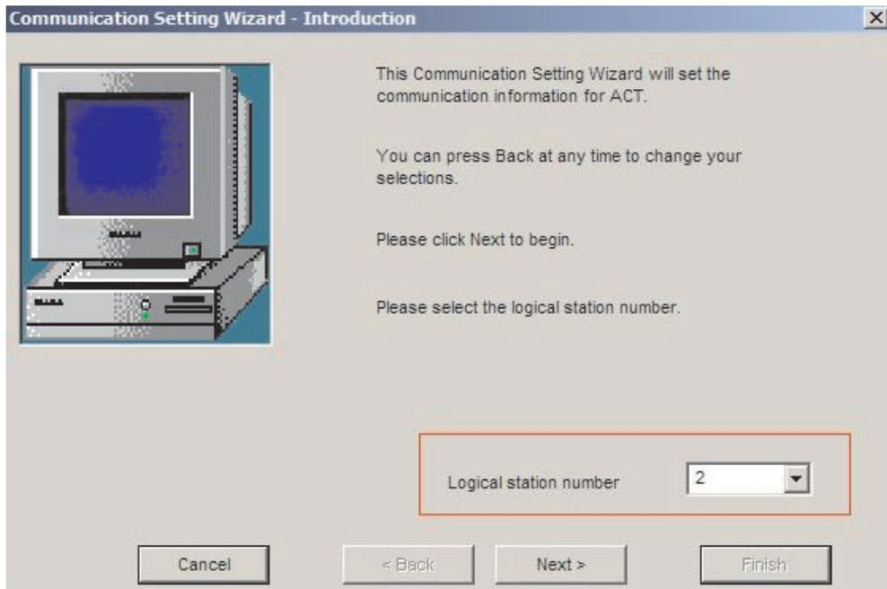
③ Next, configure the **Communication Settings** on the PC side. (Select the **Ethernet board**.)
