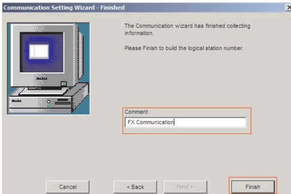
Now the definition of communication is finished. Under the folder **Connection test** the connection can be examined.
