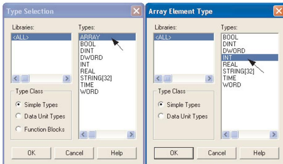
Note that when the array entry first appears, it will be dimensioned to the default value of ARRAY [0..3] OF INT. It is necessary to re dimension it to [0..9] of INT for this example, as shown below:
