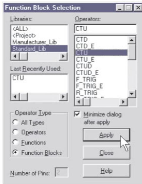
Drop the IEC Function Block onto the empty Ladder network:
