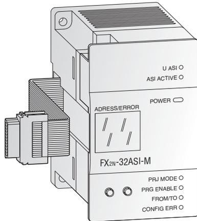
The FX2N-32ASI-M serves as master module for the connection of the FX1N/FX2N and FX3U/FX3UC PLC to the AS-Interface system. Up to 31 slave units with up to 4 inputs and 4 outputs can be controlled.
