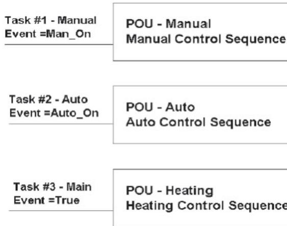
When GX IEC Developer compiles the project, it automatically inserts, program branching instructions, into the program, in line with event driven tasks.
