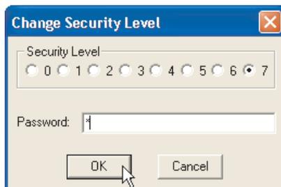
Once logged on, the security attributes for many items may be altered. For example one of the most common security options is to change access to POU's, i.e. User Functions and Function Blocks.
