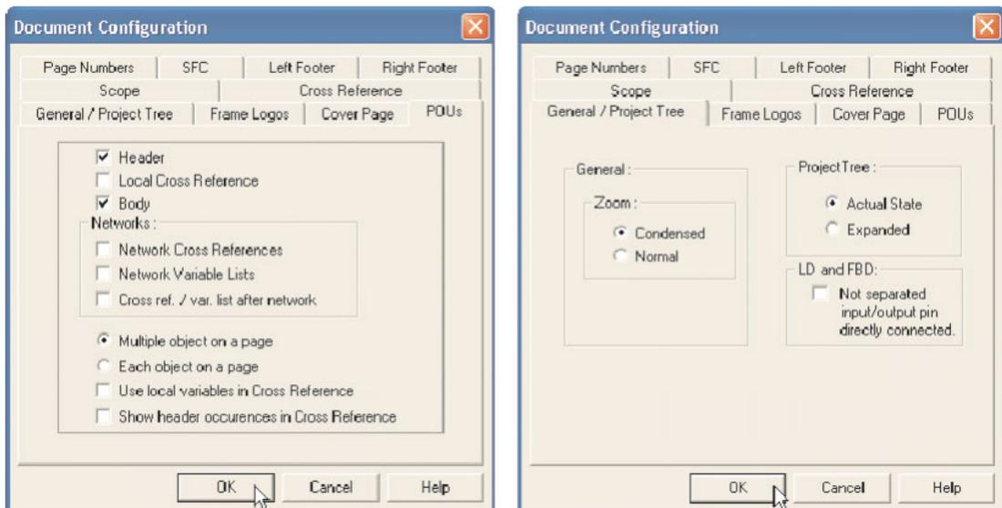
Specification for SFC appearance and cross reference specifications, are available from the **SFC** and **Cross Reference** tabs:
