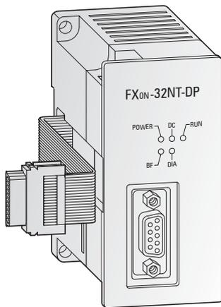
The FX0N-32NT-DP PROFIBUS DP slave module enables the attached FX base unit to be a slave station on a PROFIBUS DP network. Transfer of up to 40 bytes of data per cycle is supported at up to 12 Mbps.
