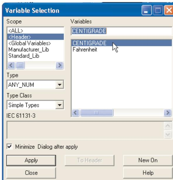
CENTIGRADE is automatically placed in the header variable list as it is the name of the function, it must therefore also be specified as the output argument.
