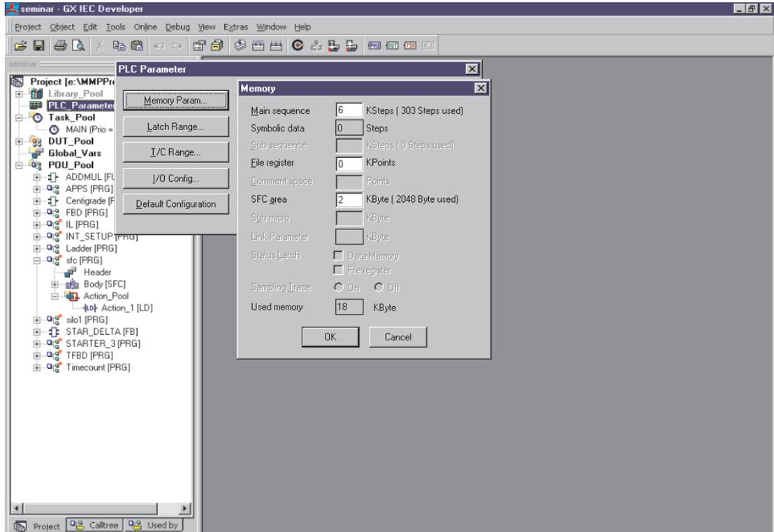
This is not the case for Q series, as the MELSEC System Q supports SFC's in the program area. Also for FX range, SFC's actually compile to STL code in the program area.
