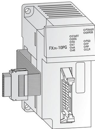
They are very suitable for achieving accurate positioning in combination with the MELSEC FX series. The configuration and allocation of the position data are carried out directly via the PLC program.
