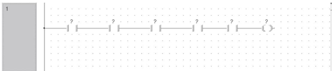
When using multi-legged or 'pinned' functions such as MUL, the number of input parameter legs, can be incremented/decremented by using the special toolbar, icons shown. This can also be achieved by placing the cursor at the bottom edge of the function, holding down the left hand mouse button and then dragging away as shown below:
