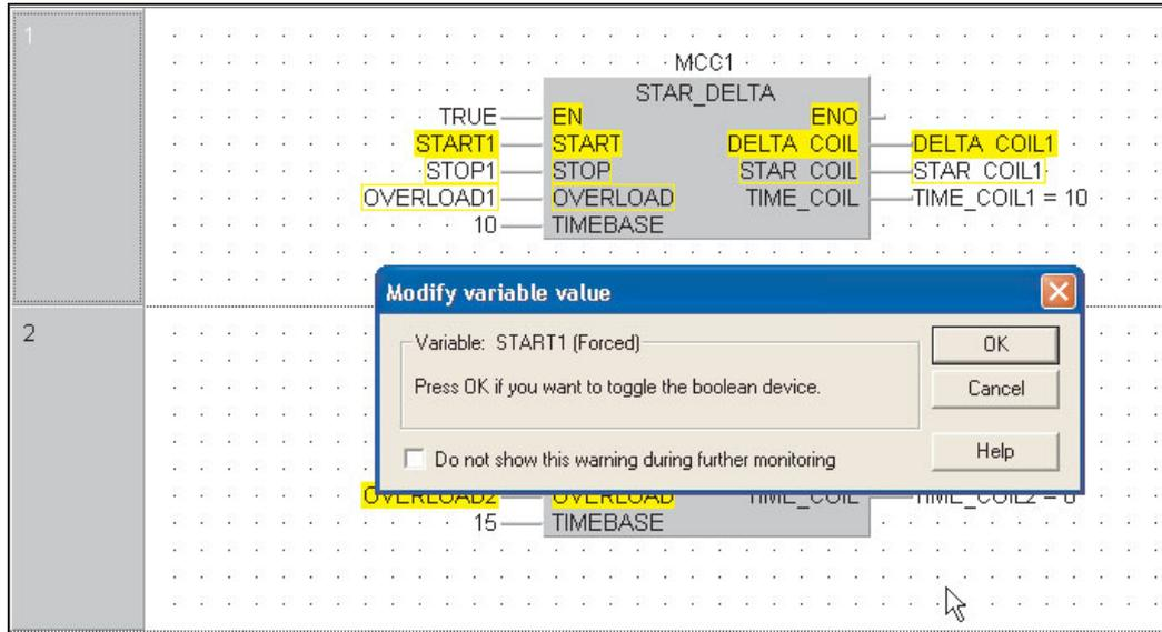
For Integer/Real variables, use the same procedure, i.e. double click on the variable name, whilst in monitor mode. The new value can be entered either as decimal or as a hexadecimal value.
