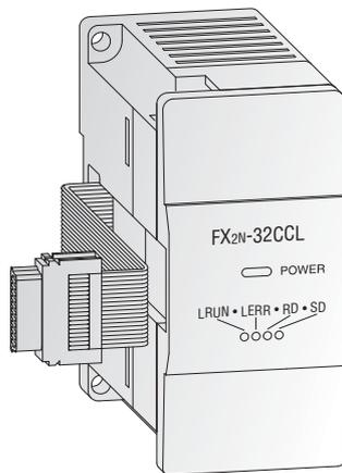
Thus the network is expandable via the digital inputs/outputs of the FX modules to a maximum of 256 I/Os.
