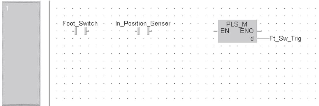
Finally, the ladder network must be finalised by connecting up the elements as follows.
