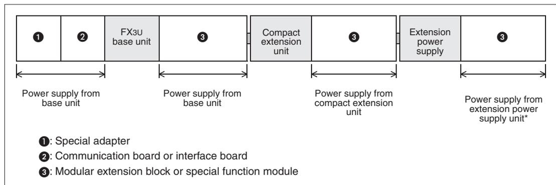
\* When connecting an **input** extension block on the downstream side of an extension power supply unit, this input extension block is supplied from the base unit or from an input/output powered extension unit which is mounted between base unit and extension power supply unit.
