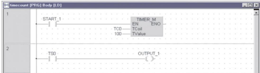
In the following example, the counter has been programmed using identifiers which would have to be declared in the Global and Local Variable tables:
