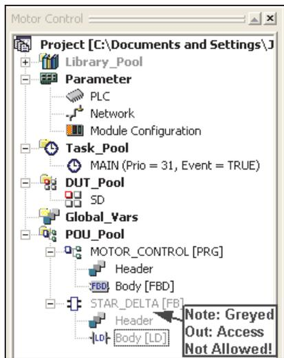
Access attributes for any individual object or complete folder in the 'Project Navigation Window' above can be individually set, allowing higher degrees of flexibility in the program security settings.
