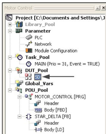
The new DUT will now be displayed under the **DUT Pool** in the project.
