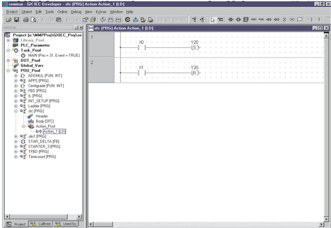
Each Transition can be a simple device i.e. Mitsubishi address X0, or an identifier name, or more complex, as a single network program written in either IEC, IL, LD, Structured Text or FBD:
