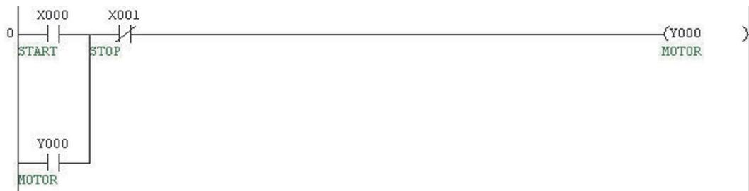
Note that all occurrences of the devices X0, X1 and Y0 will be displayed automatically within the program with the attached comment.
