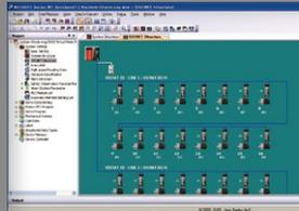
The motion control design and maintenance software includes intuitive graphic based programming together with a digital oscilloscope simulator, further helping to reduce a motion systems TCO.
