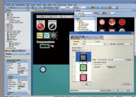
The GOT (Graphic Operation Terminal) screen creation software has been designed with 3 main features; Simplicity, Graphic Design, and Easy Usability, further helping to create graphic screens in fewer steps.
