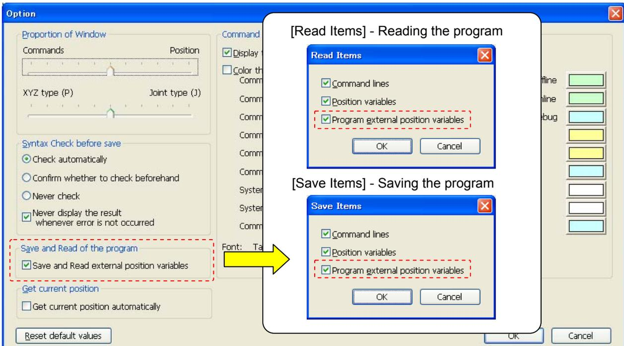
Figure 8-15 Initial setting of "Program external position variables" in the [Read Items] and the [Save Items].
