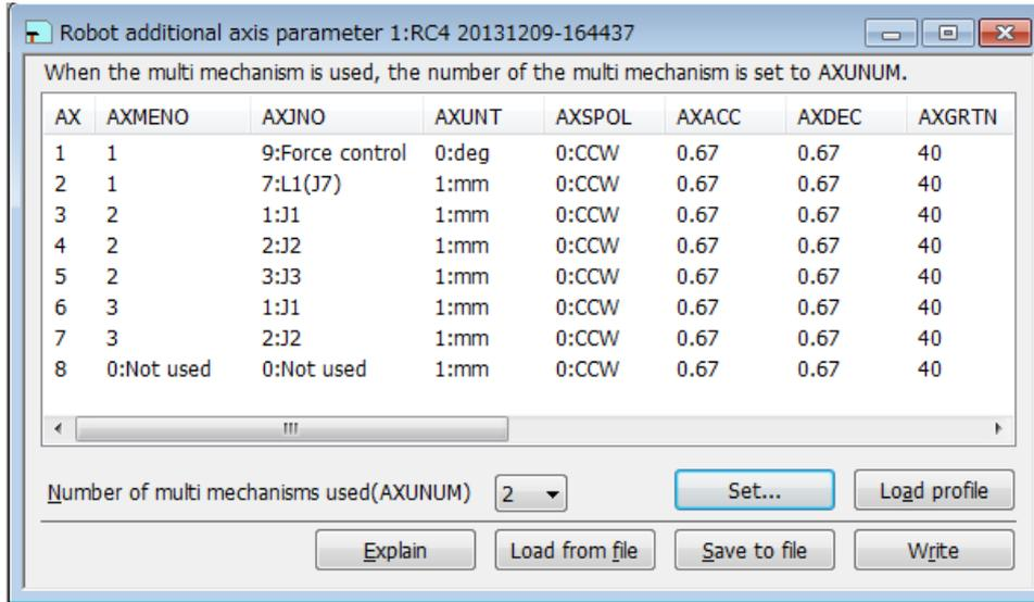
Figure 10-18 Robot additional axis parameter (Version 3.01B or later)
