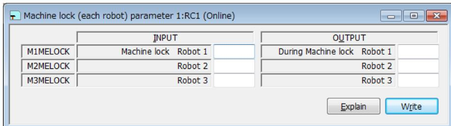
Figure 10-47 Dedicated input/output signals assignment - Machine lock (each robot) parameter
