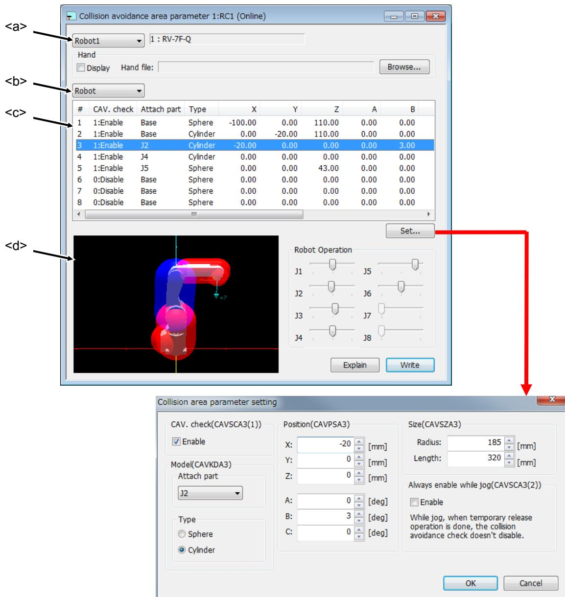
**Figure 10-29 Collision avoidance area parameter**
