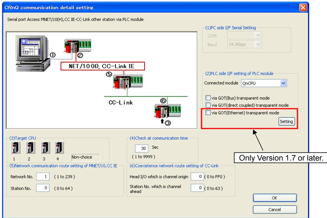
**Figure 6-6 RS-232 (Serial Communication NET/10(H), CC IE through CPU Unit – CCLink Other Station Access) Detailed Settings**
