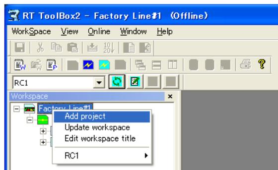
Figure 5-11 Adding a Project from a Project Tree
