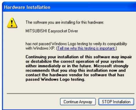
4) As the screen on the left appears, click the [Continue Anyway] button to continue the installation of the USB driver. (No problem will occur after installation of the USB driver.)
