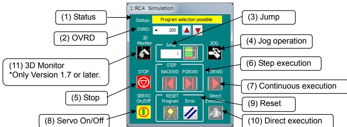
Figure 16-5 Simulation Operation Screen
