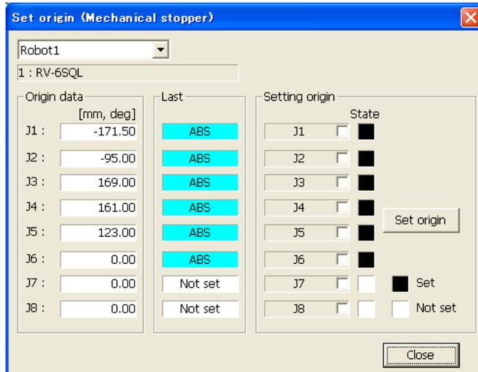
Figure 12-4 Origin Setting (Mechanical Stopper) Screen
