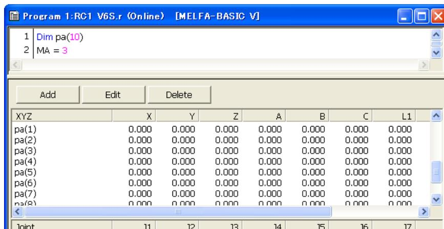
Figure 8-24 Array Variable Display
