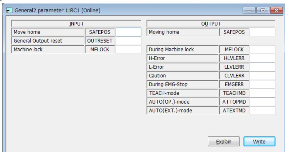
Figure 10-39 Dedicated input/output signals assignment - General2 parameter
