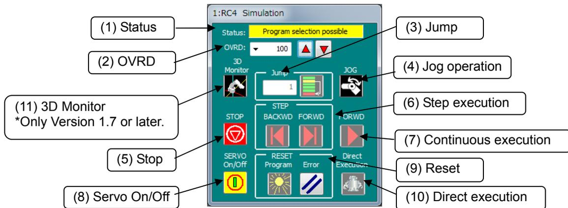
Figure 16-5 Simulation Operation Screen
