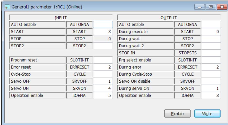
Figure 10-38 Dedicated input/output signals assignment - General1 parameter
