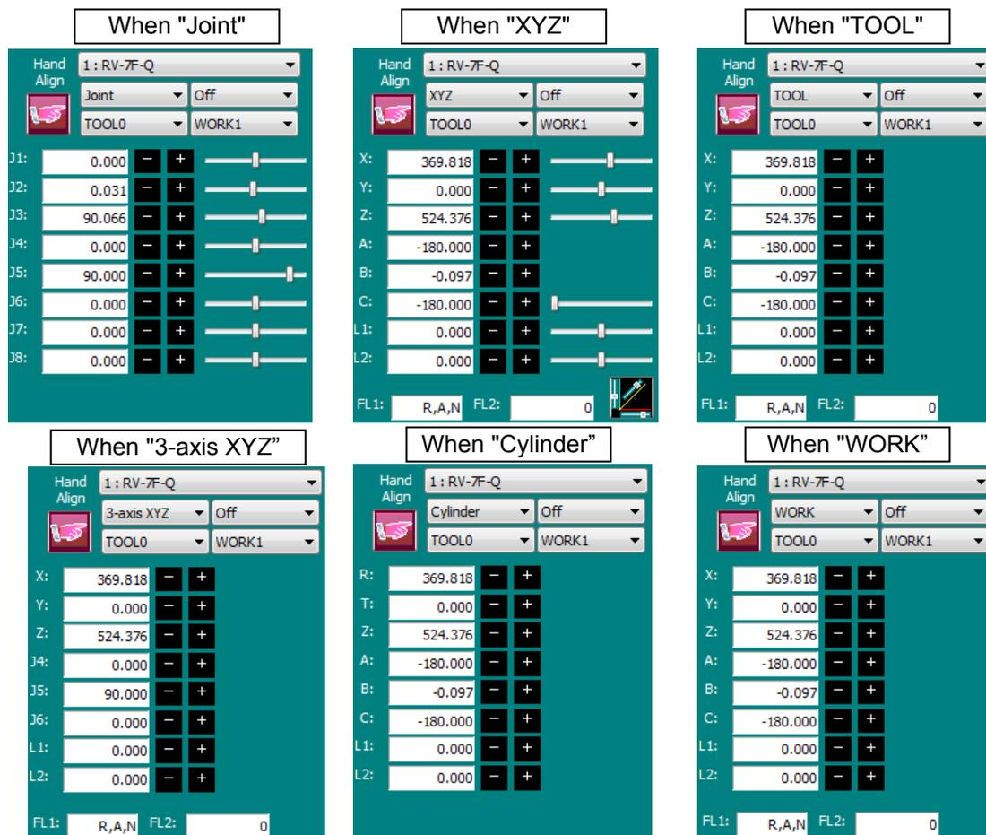
Figure 16-39 Screens for Jog Operation with Different Move Methods Selected
