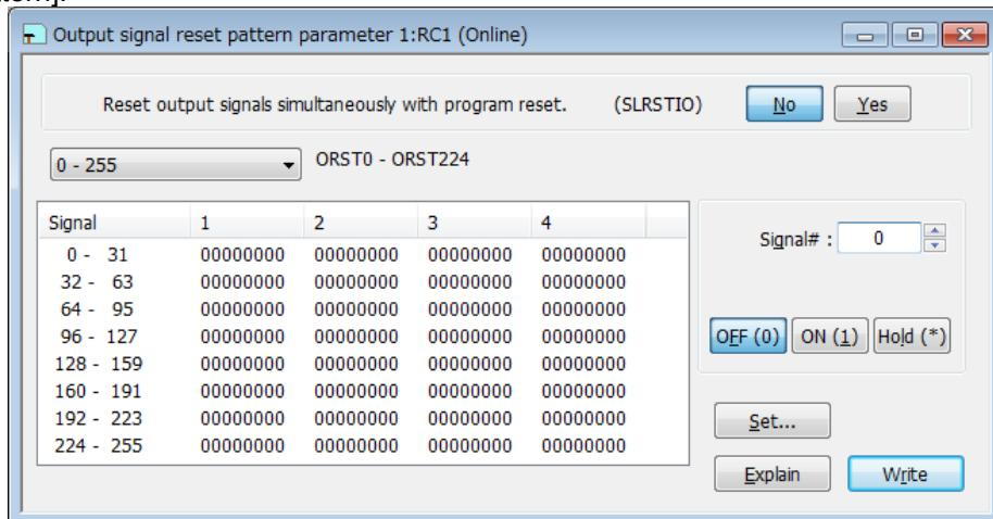
Figure 10-36 Output signal reset pattern parameter
