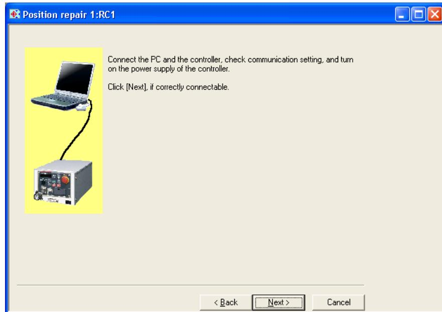
Check the communication settings and connected to the robot controller, click the [Next] button. For the setting method, see "**6 Connecting with the Robot**".
