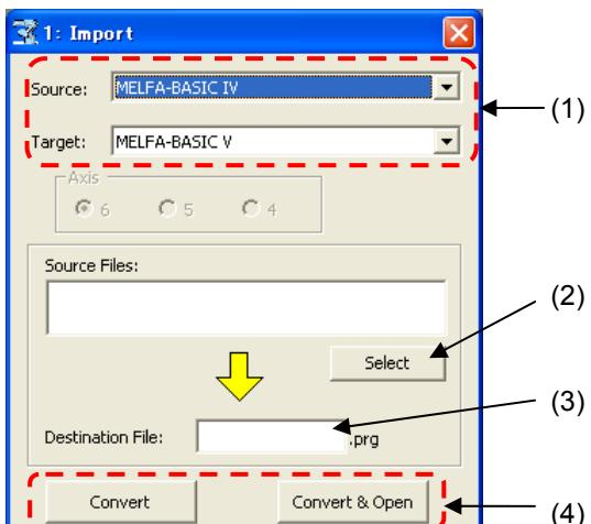
Figure 8-71 Conversion from MELFA-BASIC IV to MELFA-BASIC V
