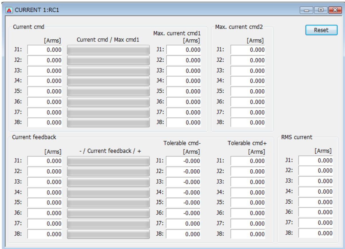
Figure 12-42 Servo monitor - Current
