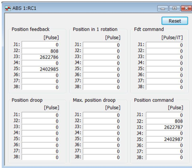
Figure 12-40 Servo monitor - ABS
