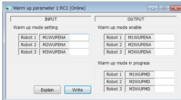
Figure 10-43 Dedicated input/output signals assignment – Warm up parameter
