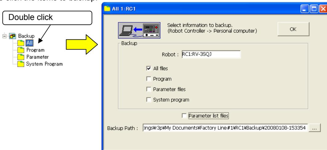
Figure 14-3 Backup (When Batch Is Selected)
