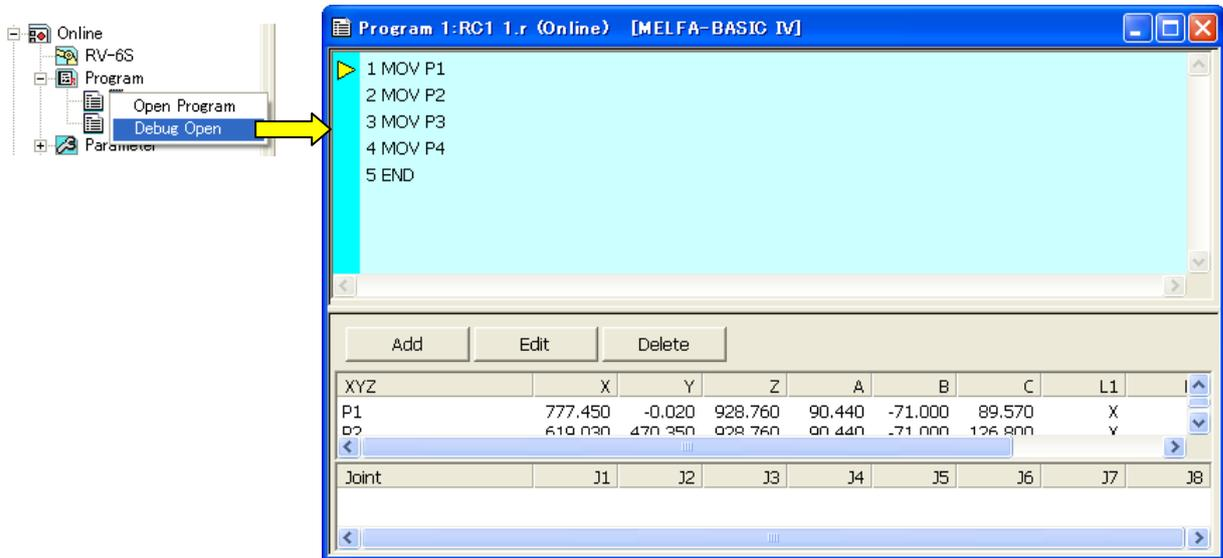
Figure 16-32 Program Selection for Simulation
