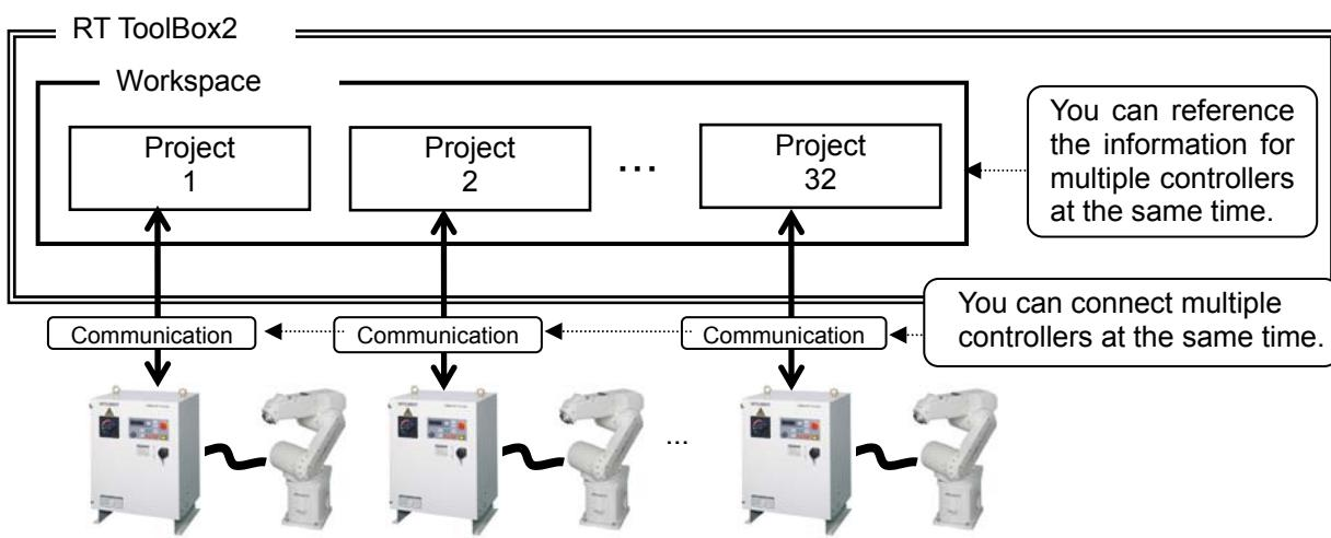
Figure 5-1 Using Multiple Robot Controllers
