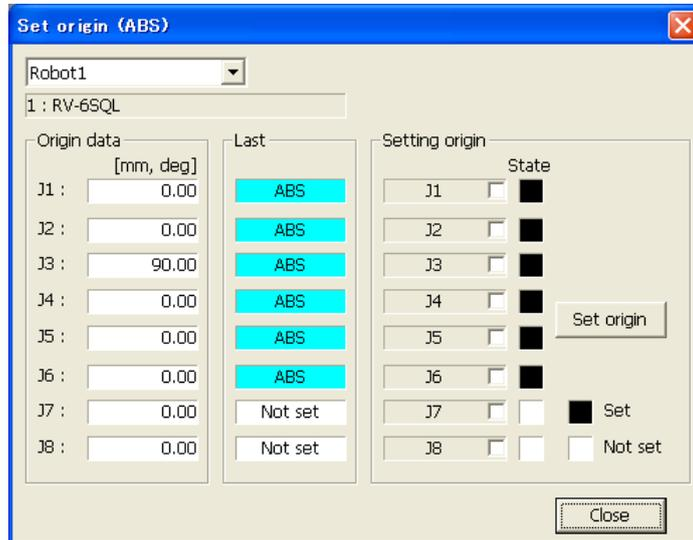
Figure 12-6 Origin Setting (ABS Origin Technique) Screen
