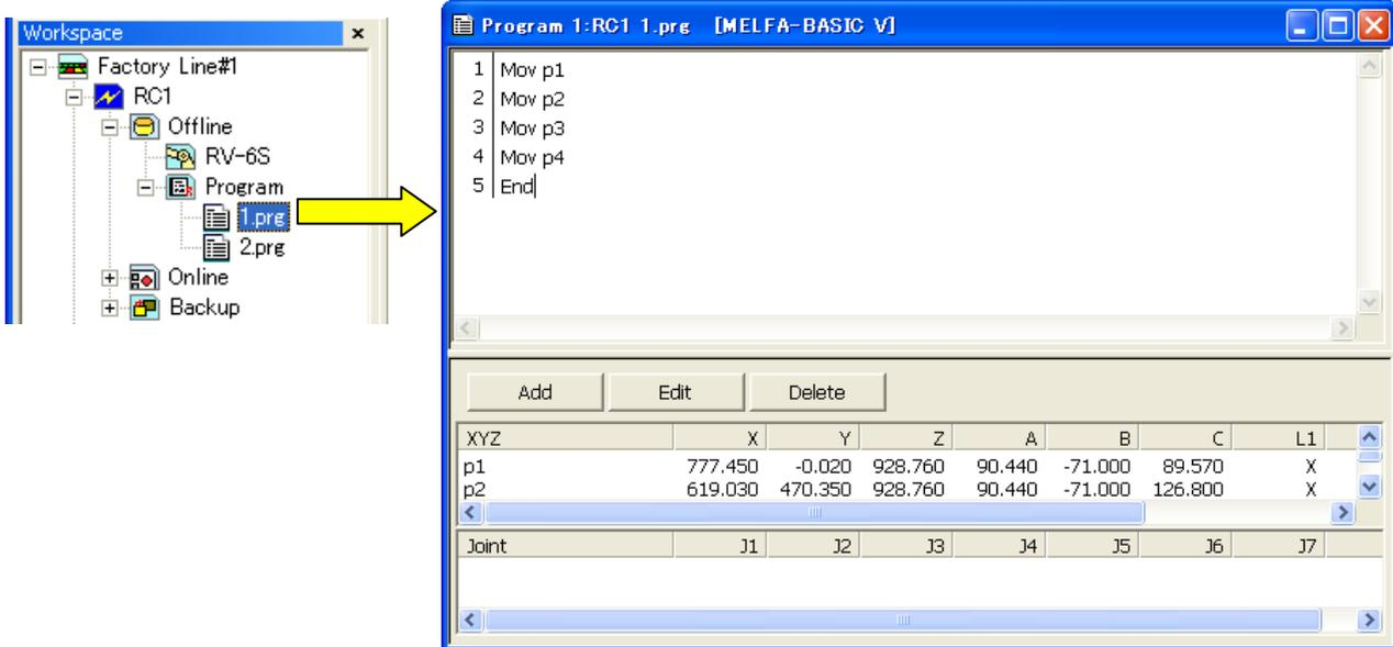
Figure 8-4 Opening a Program on the Computer
