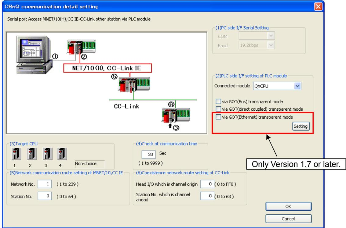
**Figure 6-7 USB (Serial Communication NET/10(H), CC IE through CPU Unit – Serial Communication Other Station Access) Detailed Settings**
