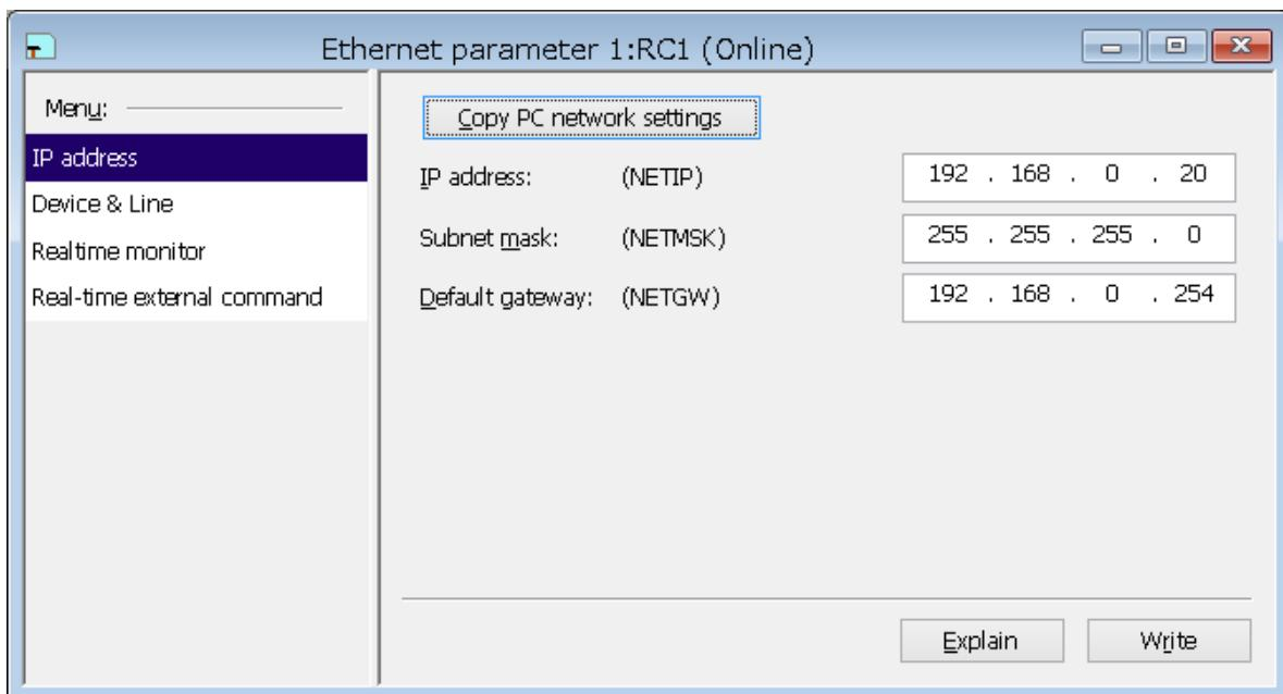
Figure 10-49 Ethernet parameter – IP address (Version 3.00A or later)
