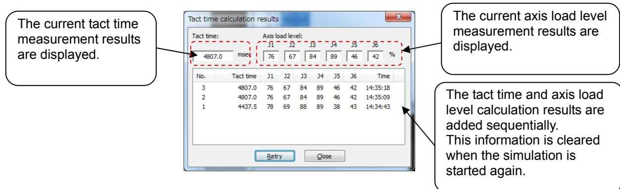
Figure 16-46 Tact time Measurement Results (The axis load level calculation is possible.)
