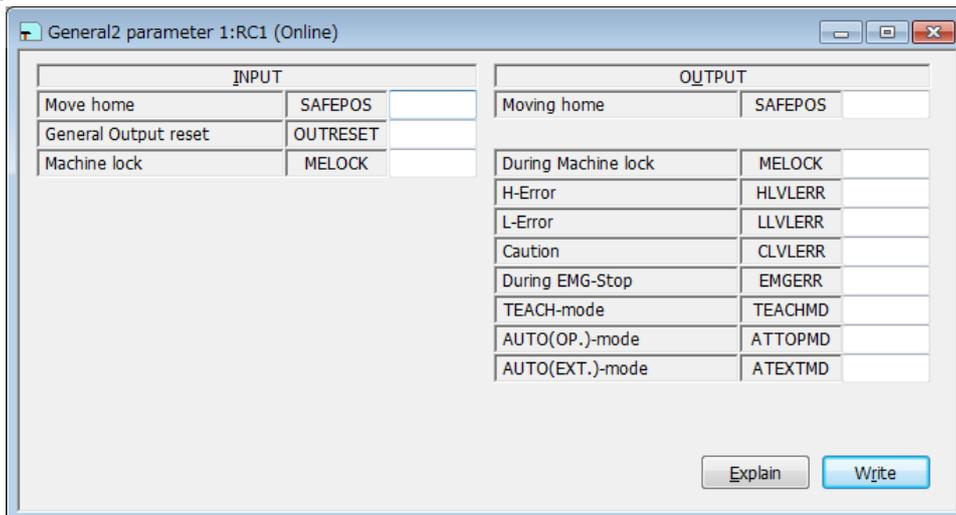
Figure 10-39 Dedicated input/output signals assignment - General2 parameter
