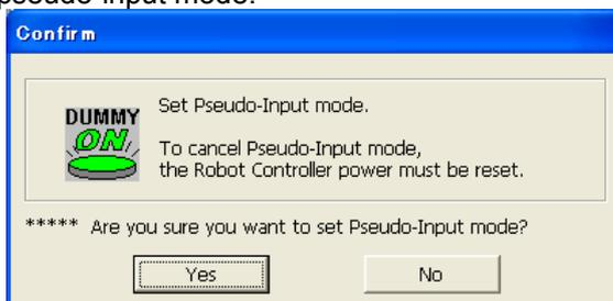
**To release a robot controller from pseudo-input mode, switch the power for the robot controller Off, then On again.**
