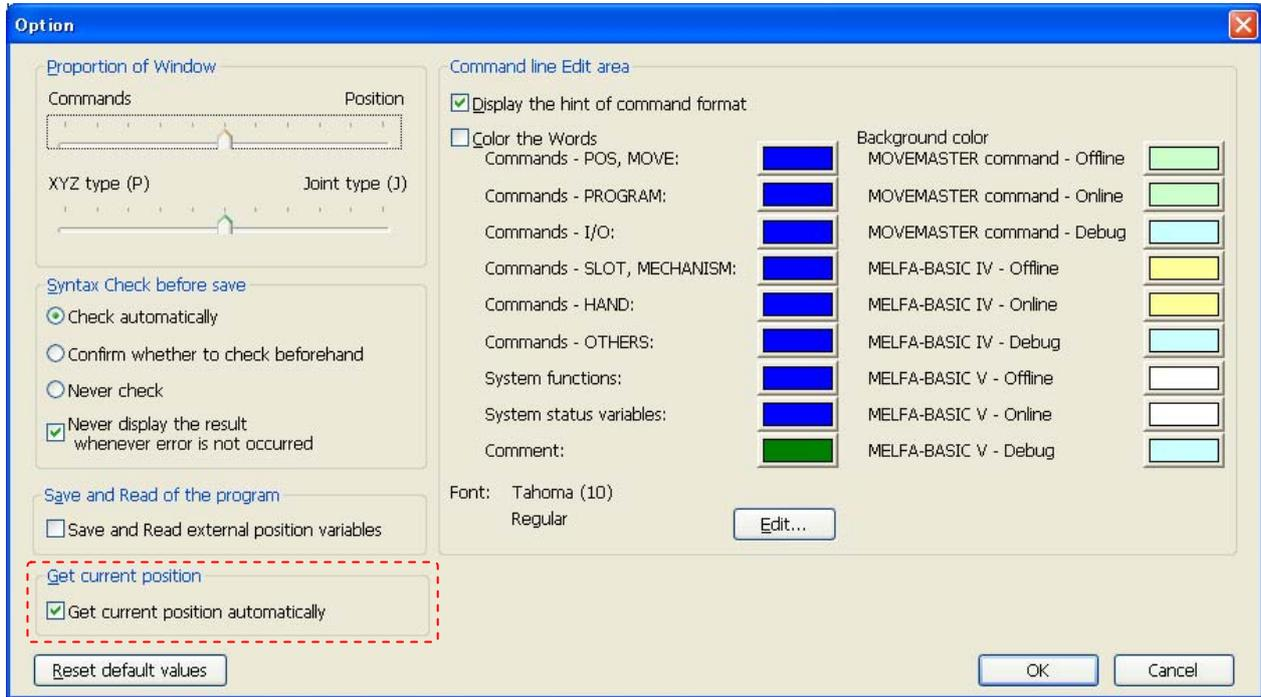
Figure 8-16 Setting the get current position.
