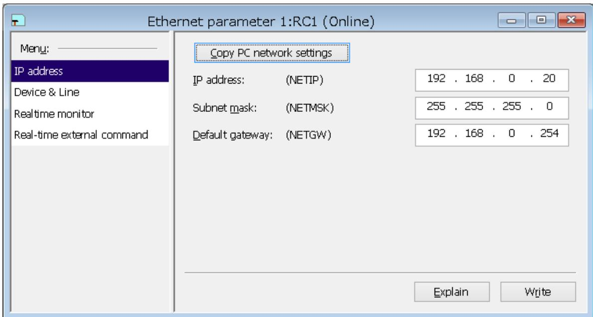
Figure 10-49 Ethernet parameter – IP address (Version 3.00A or later)
