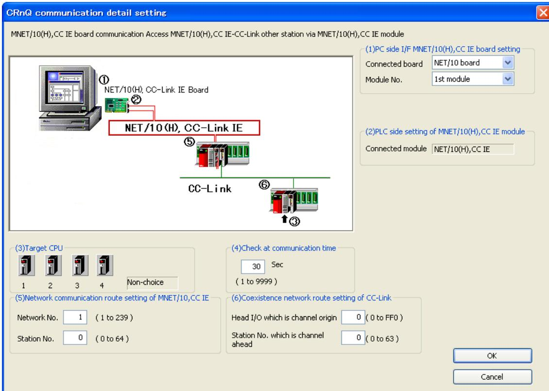
**Figure 6-8 NET/10(H), CC IE (NET/10(H), CC IE Board Communication NET/10(H), CC IE through NET/10(H), CC IE Unit – CC-Link Other Station Access) Detailed Settings**
