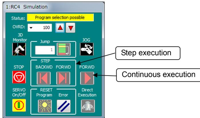
Figure 16-35 Simulation Operation Screen
