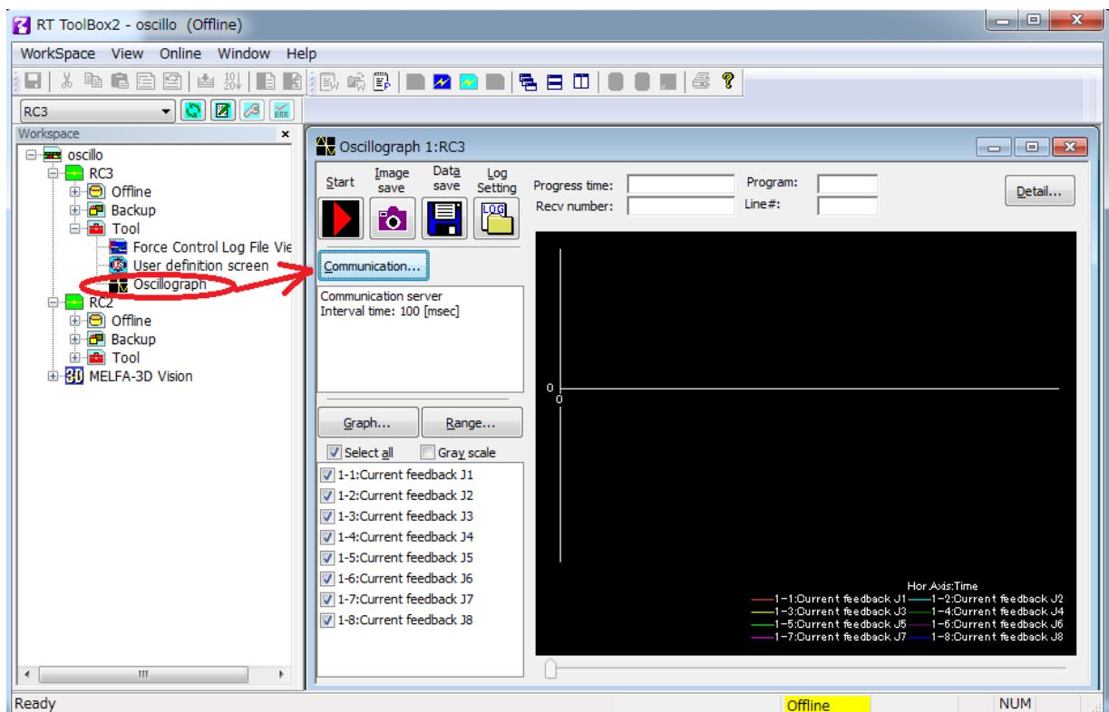
Figure 15-10 Starting the Oscillograph
