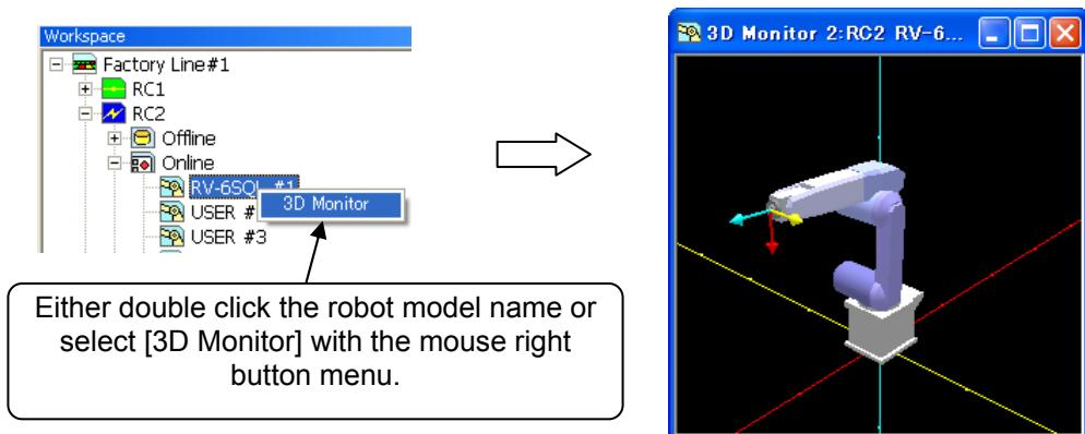
Figure 11-16 Starting Robot View
