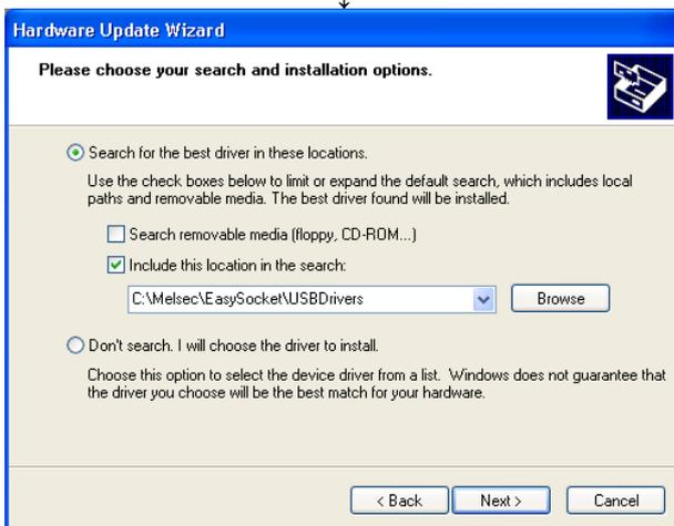
3) As the screen on the left appears, choose "Search for the best driver in these locations". Check "Include this location in the search" and set the "C:\Melsec\EasySocket\USBDrivers". If volume MELSOFT products have been installed, browse the installation destination "EasySocket\USBDrivers" of the first installed product. After setting, click the [Next] button.
