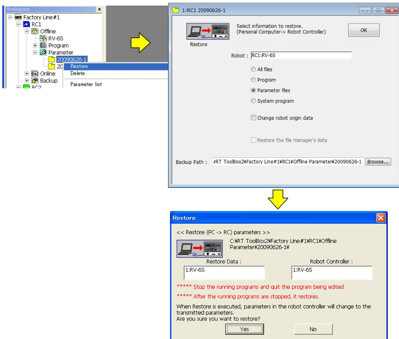
Figure 10-69 Restoring the edited parameter to the robot controller
