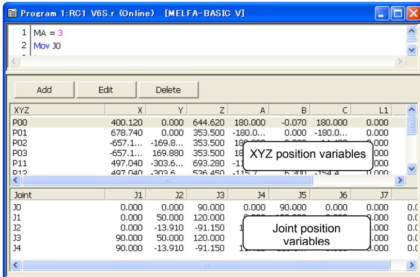
Figure 8-23 Position Variable Edit Screen
