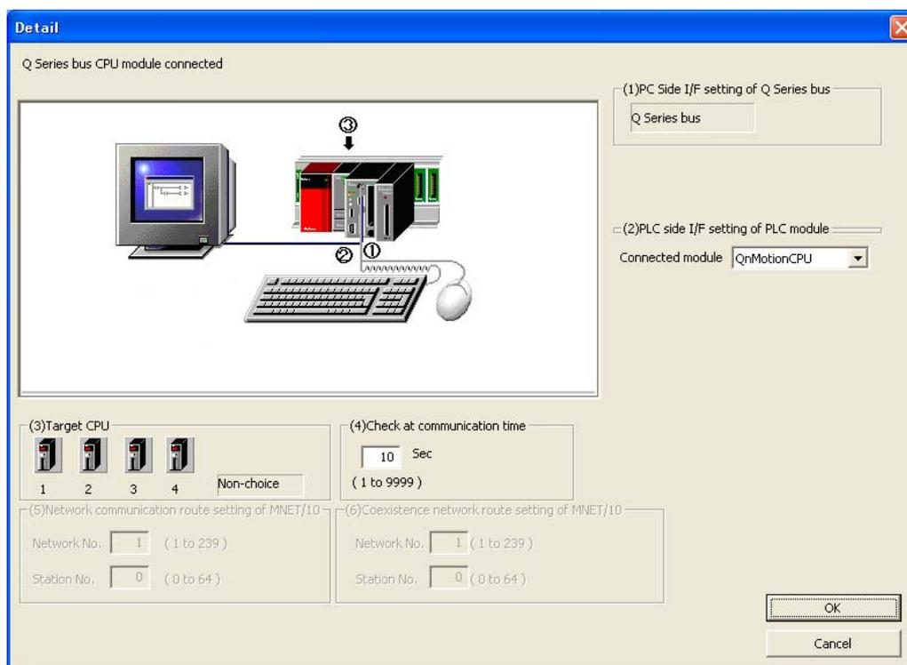
**Figure 6-11 Q Series Bus (Q Bus Communications CPU Unit Connection) Detailed Settings**
