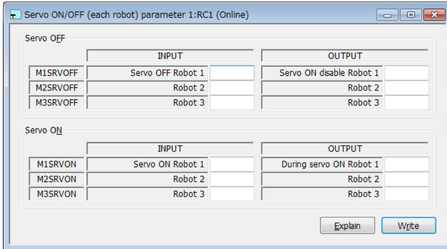
Figure 10-46 Dedicated input/output signals assignment – Servo ON/OFF (each robot) parameter
