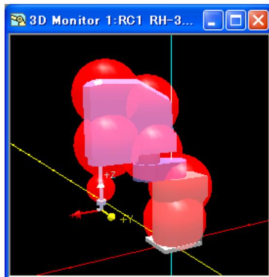
Figure 16-17 Un-display / display of Collision area
