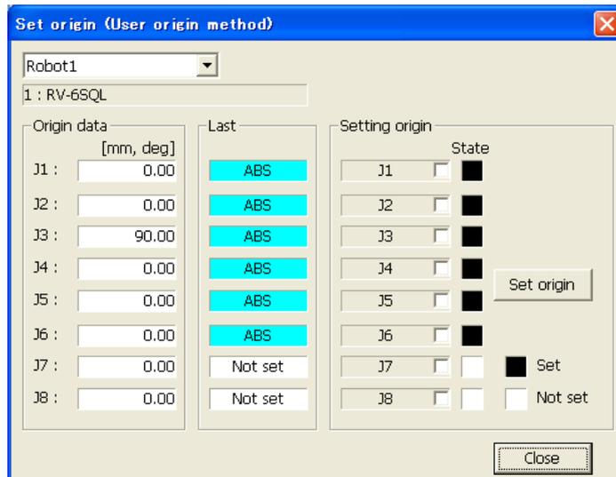
Figure 12-7 Origin Setting (User Origin Technique) Screen
