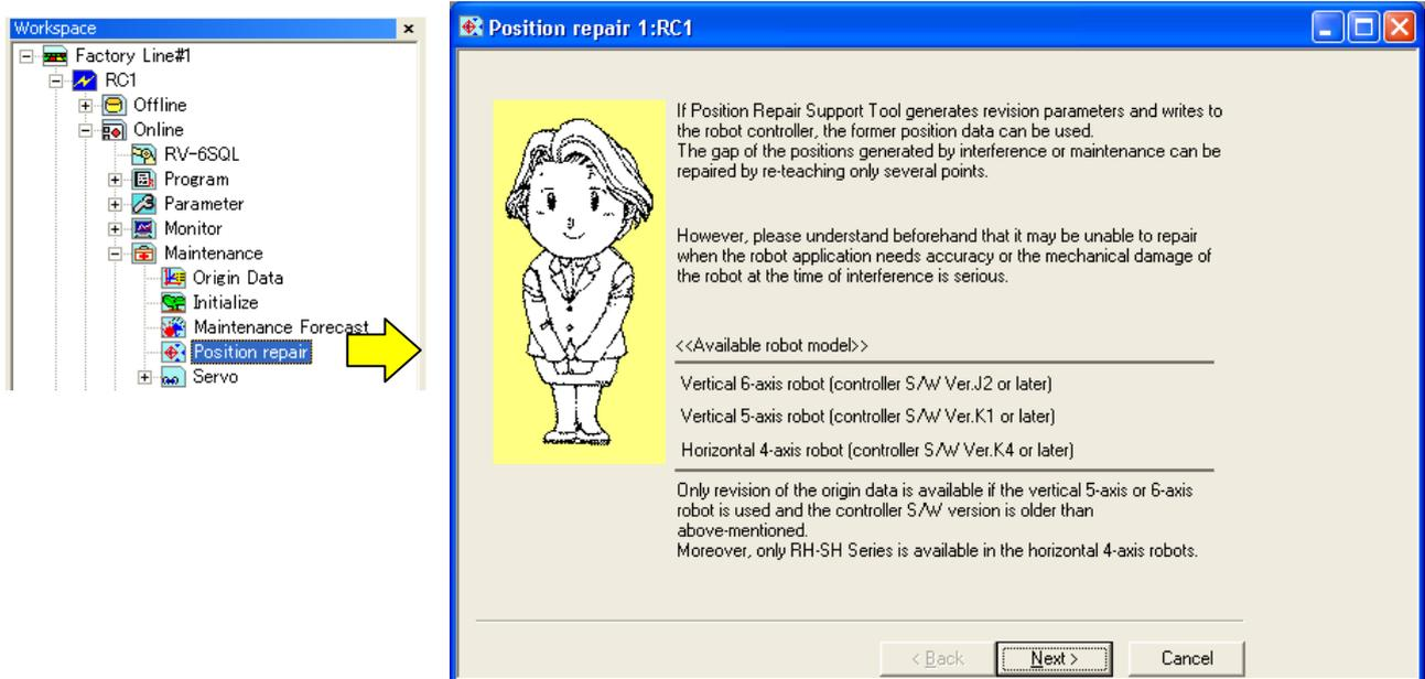
**Figure 12-20 Starting Position Repair**
