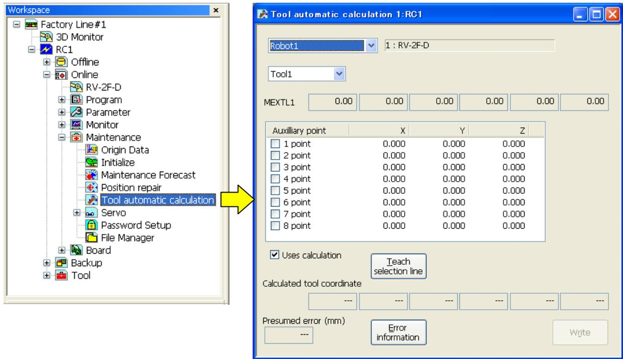
Figure 12-37 Starting the “Tool automatic calculation”
