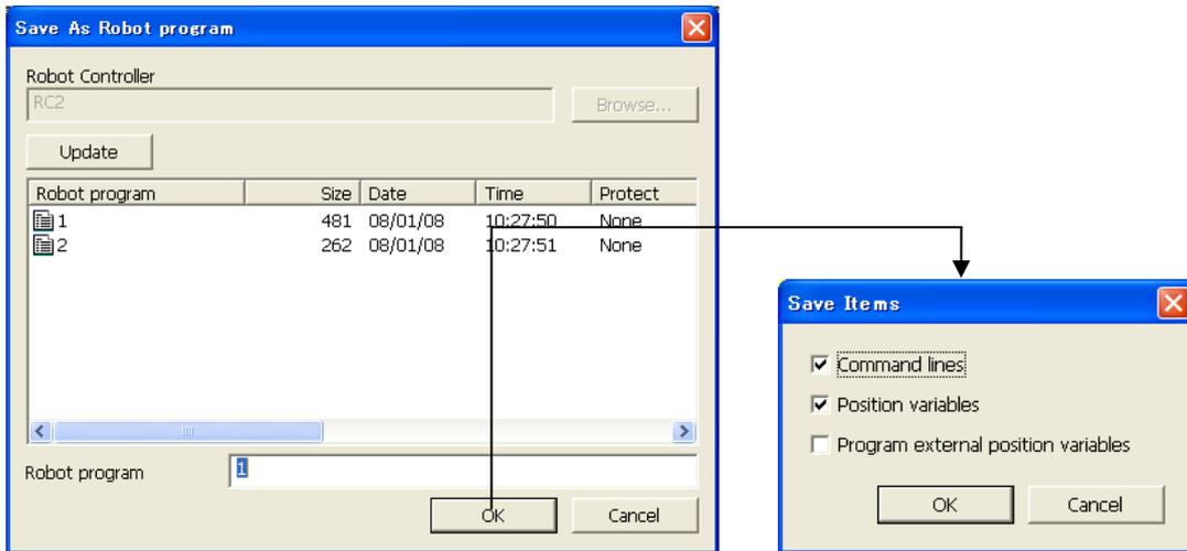
Figure 8-45 Saving on Robot Controller
