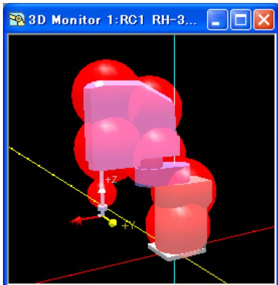
Figure 16-17 Un-display / display of Collision area
