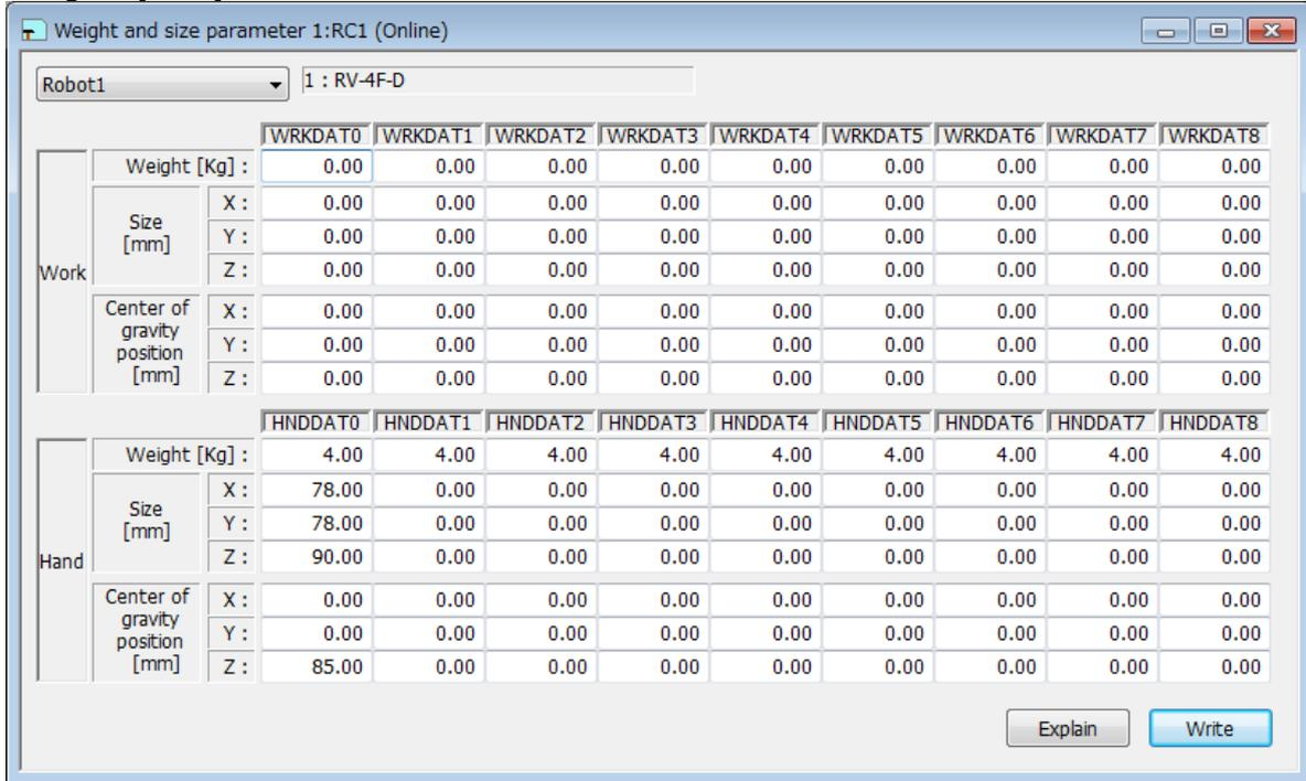
Figure 10-13 Weight and size parameter
