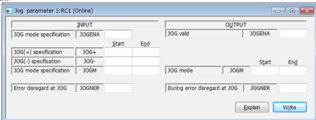
Figure 10-41 Dedicated input/output signals assignment - Jog parameter
