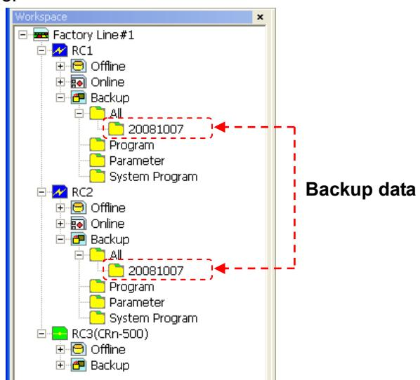
Figure 14-3 The information of saving data from all robot controllers by batch processing.
