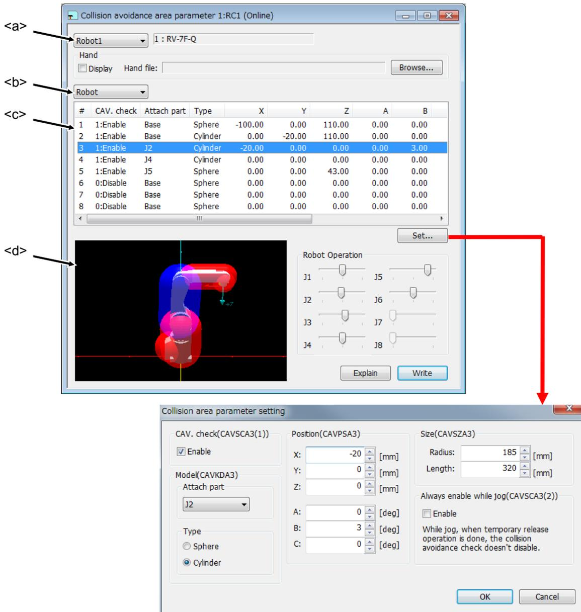
**Figure 10-29 Collision avoidance area parameter**
