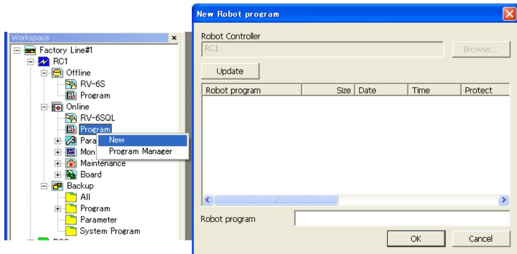
Figure 8-2 Writing a New Program in a Robot Controller
