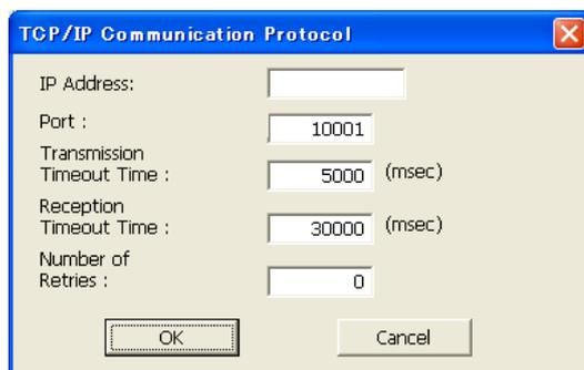
Figure 6-3 TCP/IP Communication Settings
