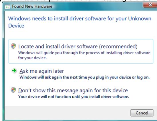
1) The screen shown on the left appears when you connect the personal computer and Universal model QCPU by the USB cable. Select "Locate and install driver software (recommended)" and wait for the search to end.
