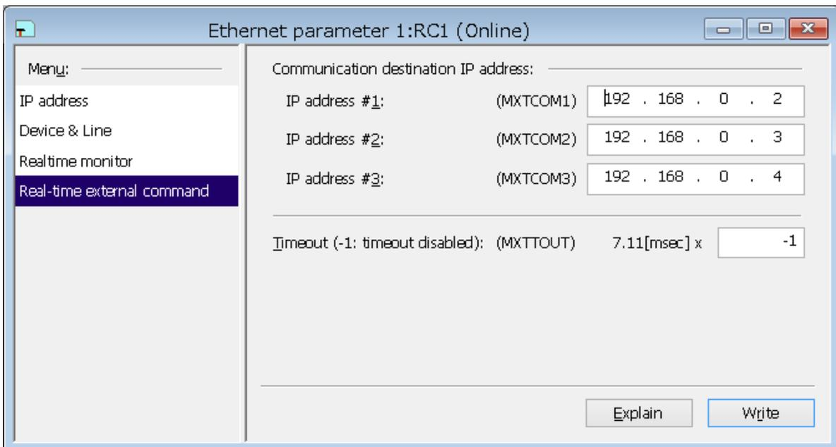
**Figure 10-53 Ethernet parameter – Real-time external command (Version 3.00A or later)**
