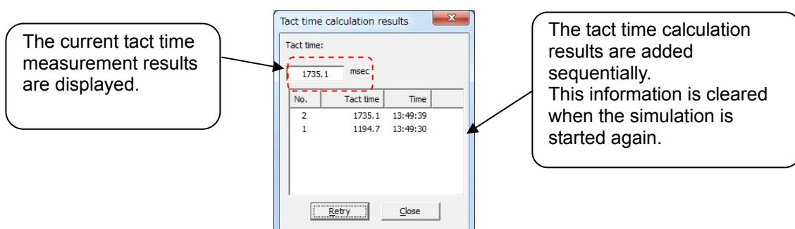
Figure 16-45 Tact time Measurement Results (The axis load level calculation is impossible.)
