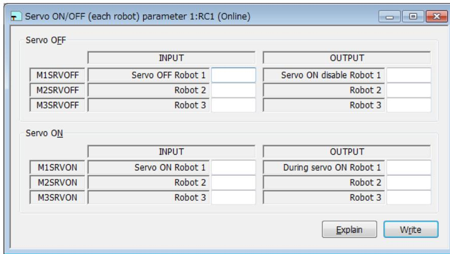
Figure 10-46 Dedicated input/output signals assignment – Servo ON/OFF (each robot) parameter
