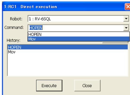
Figure 16-37 Command Dropdown List on Direct Execution Screen
