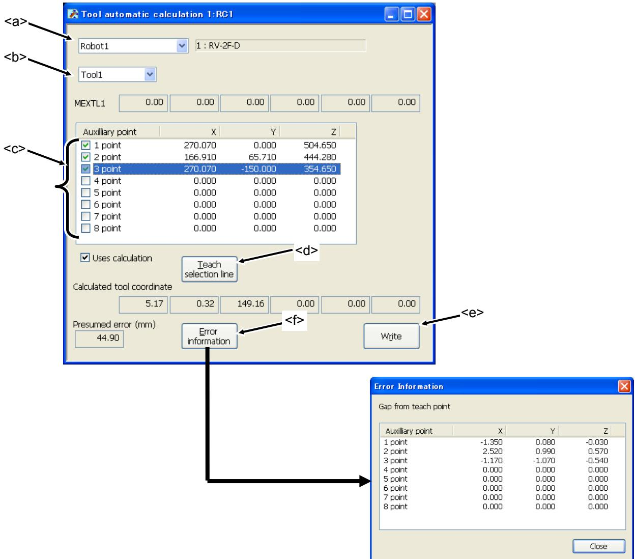
Figure 12-39 The “Tool automatic calculation” screen
