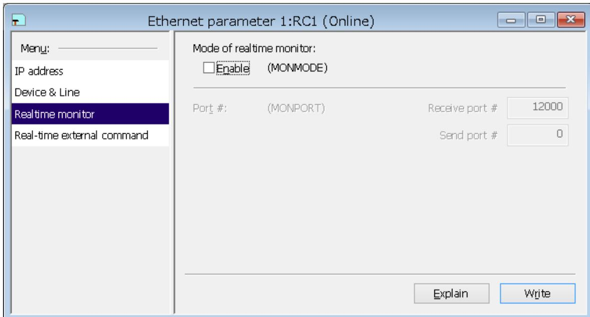
Figure 10-52 Ethernet parameter – Realtime monitor (Version 3.00A or later)
