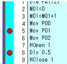
Figure 8-55 Display of Lines with Breakpoints Set
