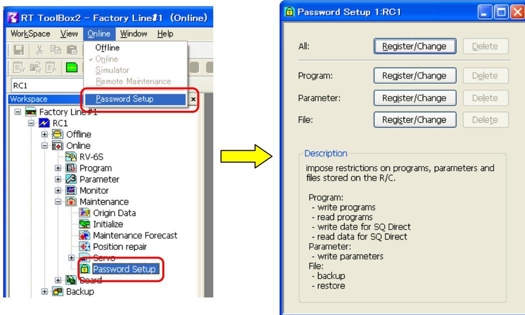
Figure 12-45 Password setup
