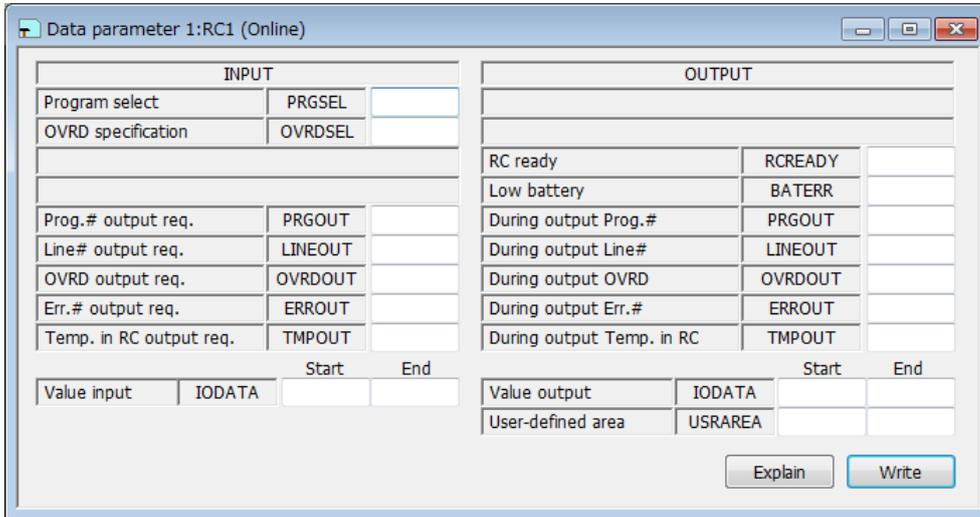
**Figure 10-40 Dedicated input/output signals assignment - Data parameter**
