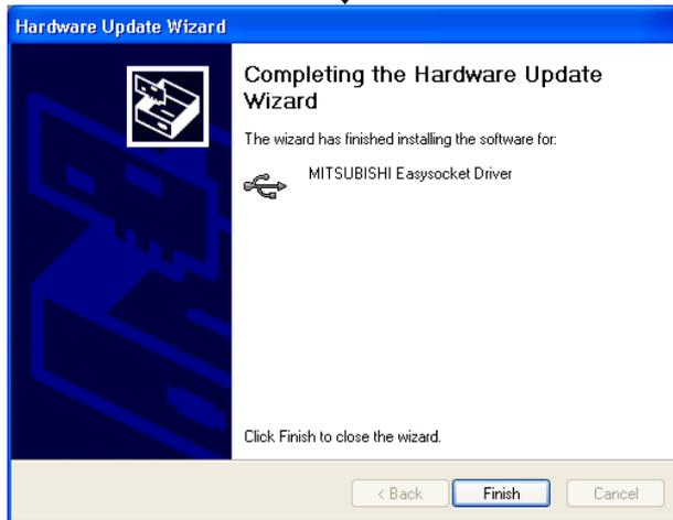
5) The screen on the left appears to indicate completion of installation. Click the [Finish] button.
