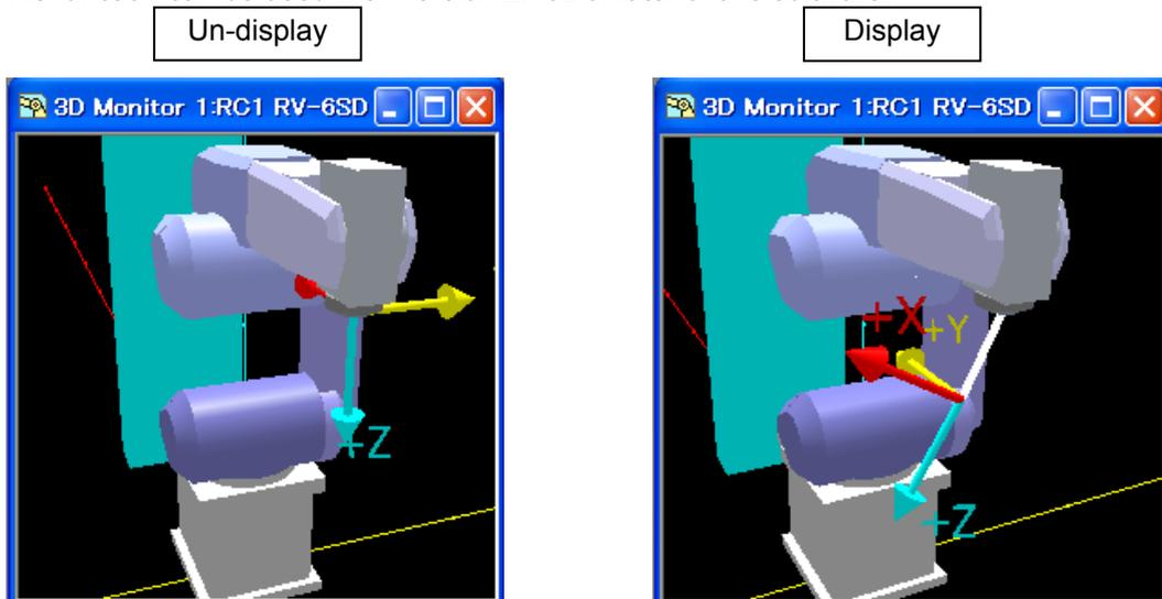
Figure 16-15 Un-display / display of tool
