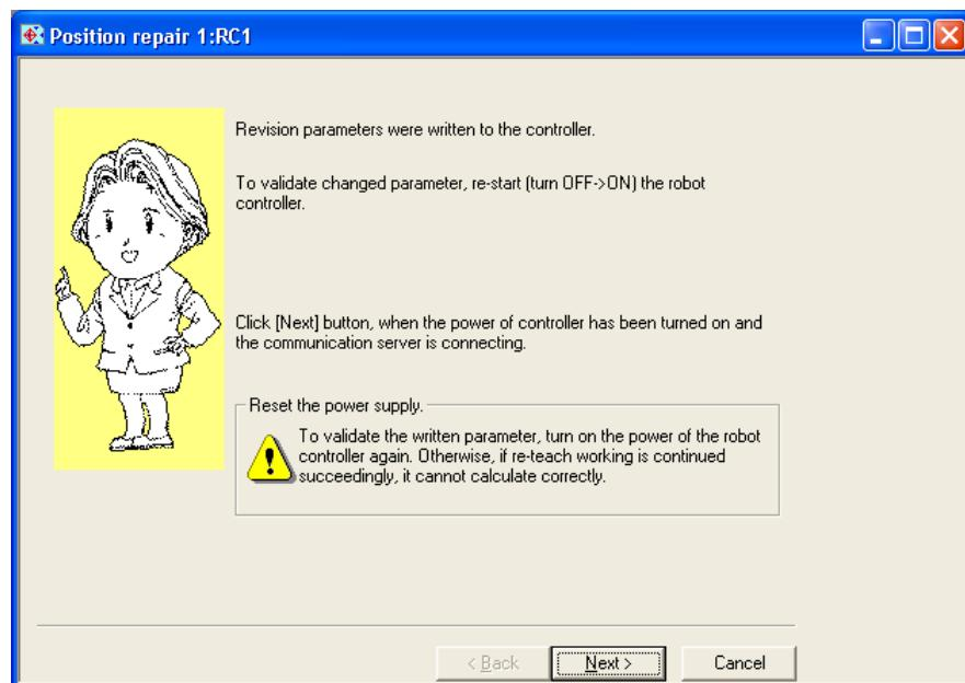
Figure 12-33 Re-start the power supply of the controller Window
