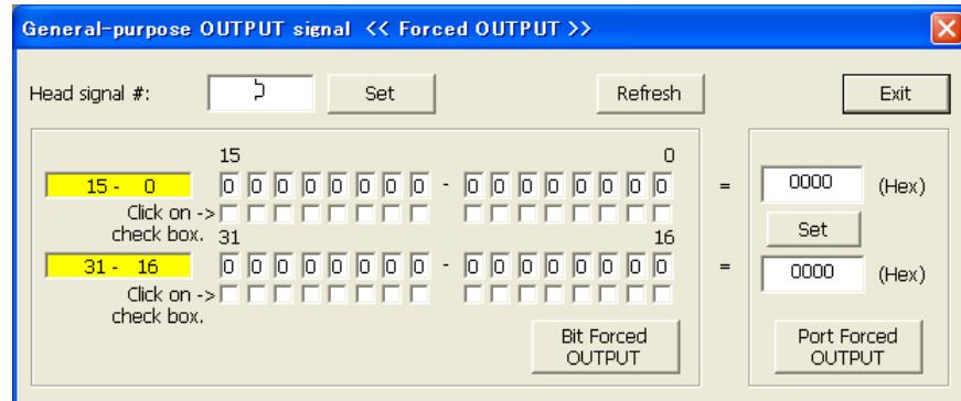
Figure 11-20 Forced Signal Output
