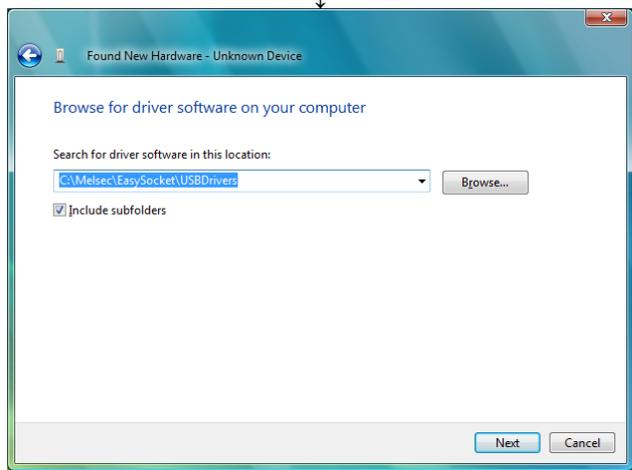
3) The screen on the left is displayed, so select "C:\Melsec\EasySocket\USBDrivers". If volume MELSOFT products have been installed, browse the installation destination "EasySocket\USBDrivers" of the first installed product. After setting, click the [Next] button.
