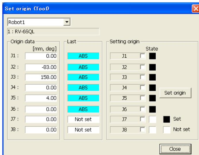
Figure 12-5 Origin Setting (Tool Technique)
