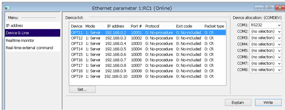
Figure 10-50 Ethernet parameter – Device & line (Version 3.00A or later)
