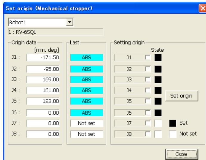
Figure 12-4 Origin Setting (Mechanical Stopper) Screen
