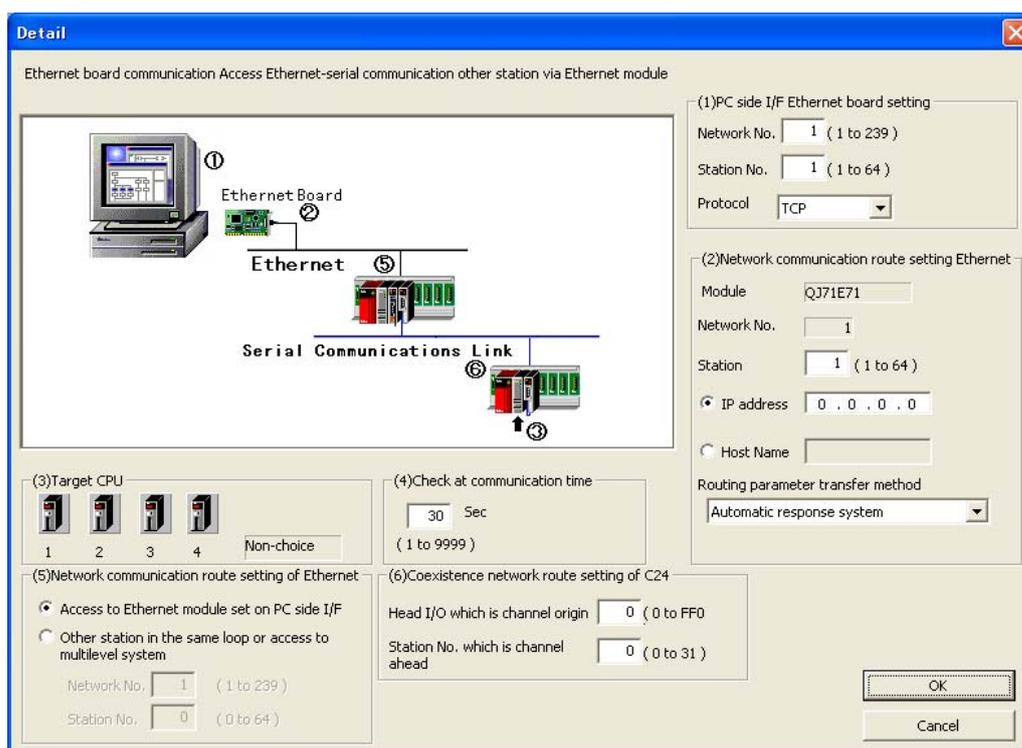
**Figure 6-10 Ethernet (Ethernet board communication Access Ethernet-serial communication other station via Ethernet module) Detailed Settings**
