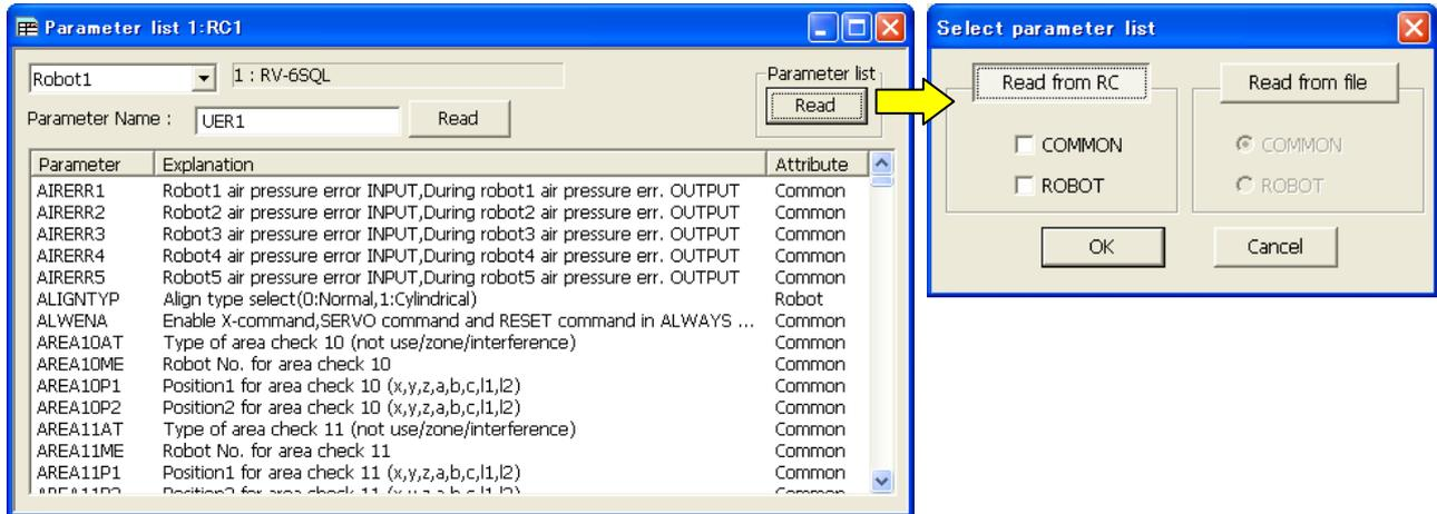
Figure 10-6 Parameter List Reading
