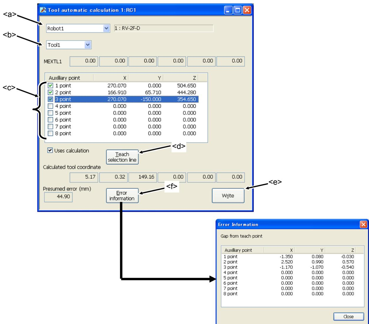
Figure 12-39 The “Tool automatic calculation” screen
