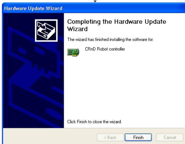
2) When the screen on the left is displayed, the installation is complete. Click the [Finish] button to end the installation.
