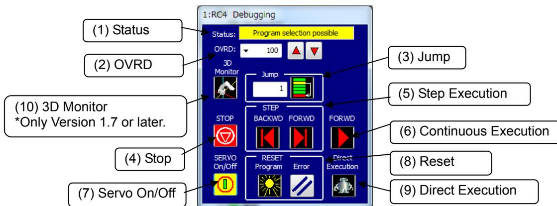
Figure 8-50 Debug Operation Screen
