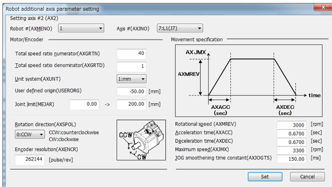
Figure 10-19 Robot additional axis parameter setting (Version 3.01B or later)
