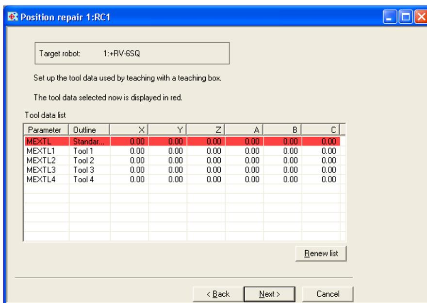
Figure 12-27 Check of Setting Tool Window
