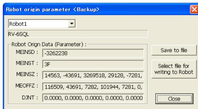
Figure 12-8 Robot Origin Parameter Backup Screen
