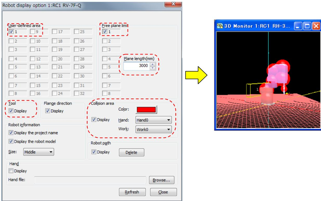
Figure 16-14 Display of Robot display option
