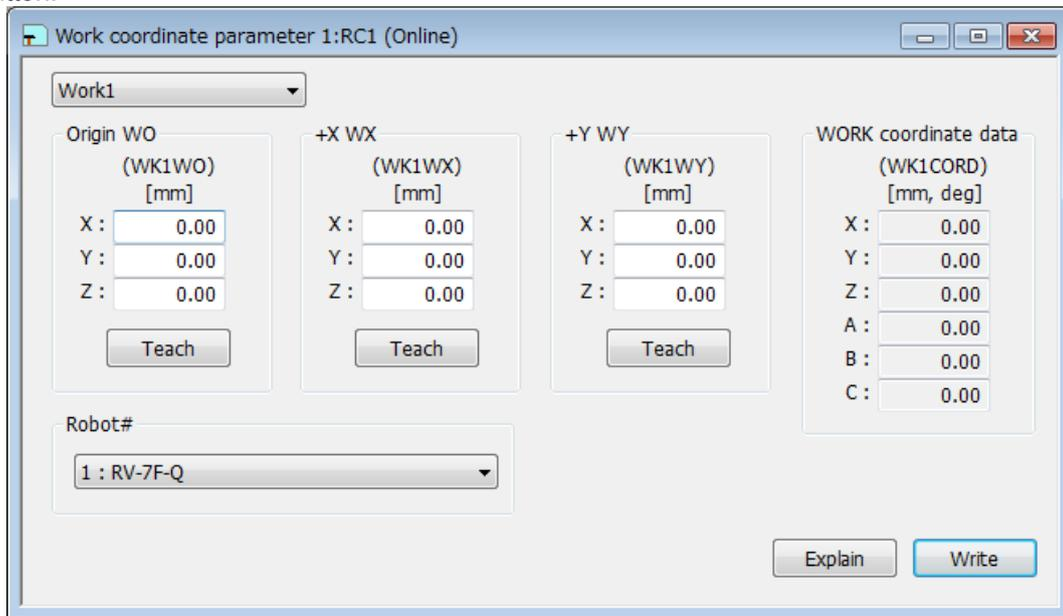
**Figure 10-23 Work coordinate parameter**
