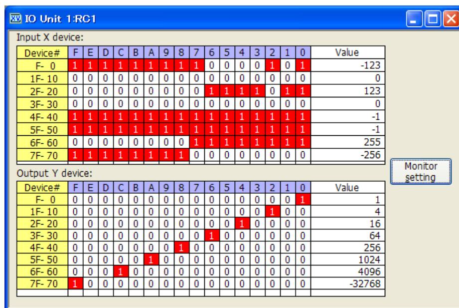
The screenshot shows the 'IO Unit 1:RC1' window with two tables. The top table, 'Input X device:', lists 16-bit binary values for various devices from F-0 to 7F-70, with their decimal equivalents in the 'Value' column. The bottom table, 'Output Y device:', lists 16-bit binary values for various devices from F-0 to 7F-70, with their decimal equivalents in the 'Value' column. A blue box labeled 'Monitor setting' points to the bottom right of the window.
