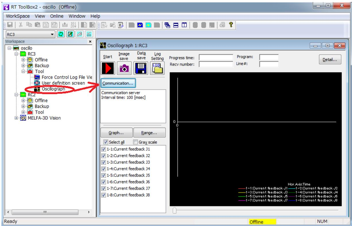
Figure 15-10 Starting the Oscillograph
