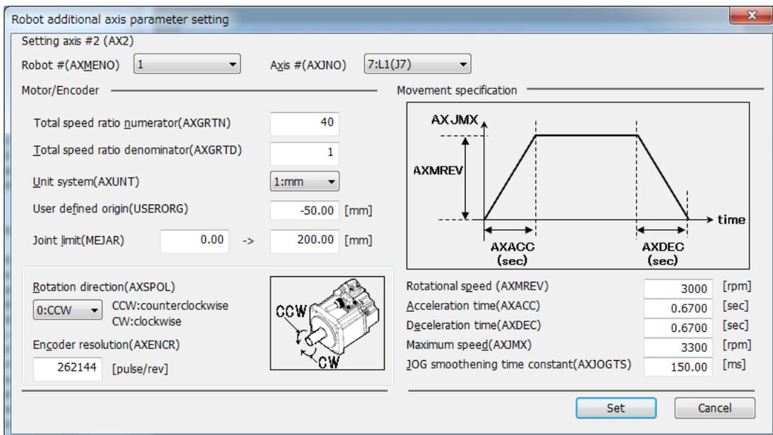
Figure 10-19 Robot additional axis parameter setting (Version 3.01B or later)
