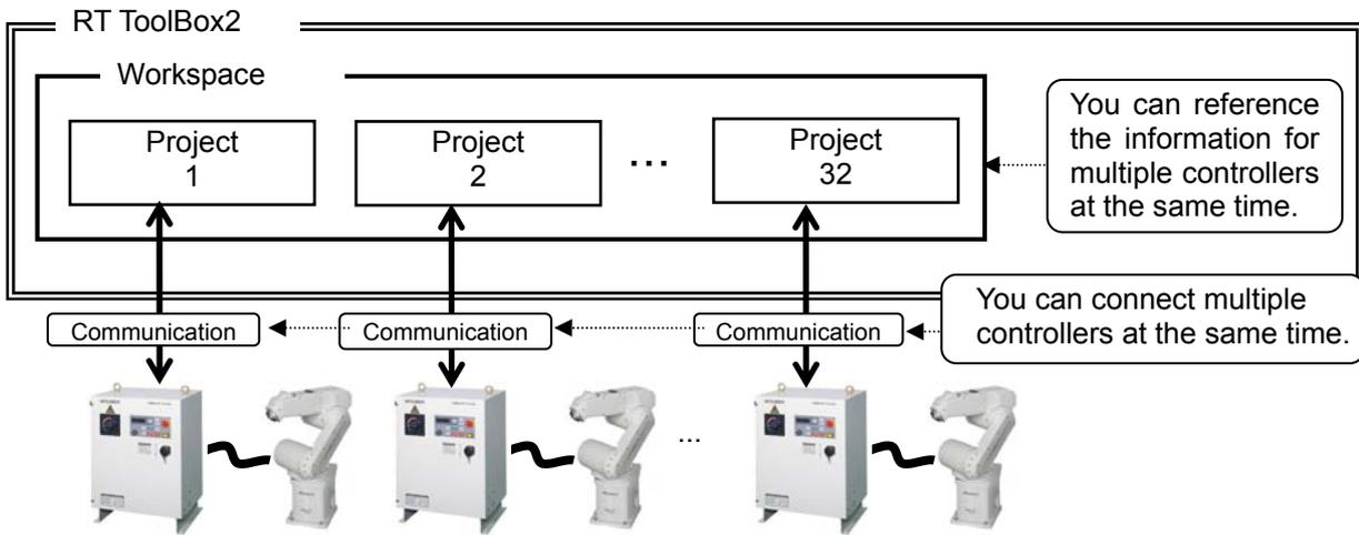
Figure 5-1 Using Multiple Robot Controllers
