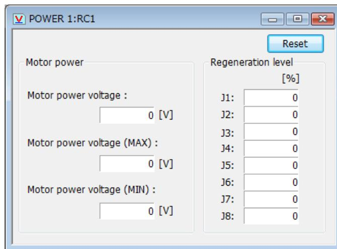
Figure 12-44 Servo monitor - Power
