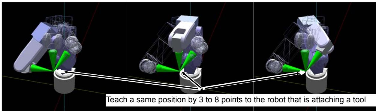
Figure 12-36 Summary the “Tool automatic calculation”
