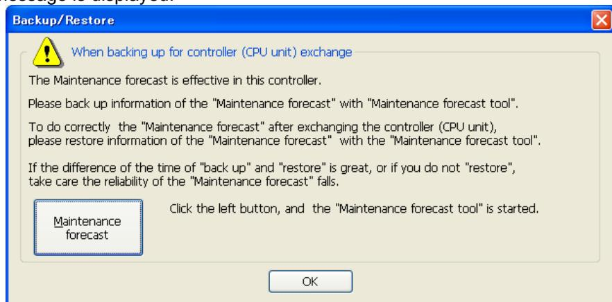
Figure 14-1 Backup When Maintenance Forecasting Information Is Enabled
