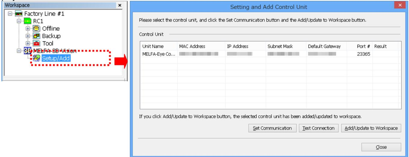
Figure 17-1 “Setting and Add Control Unit” window
