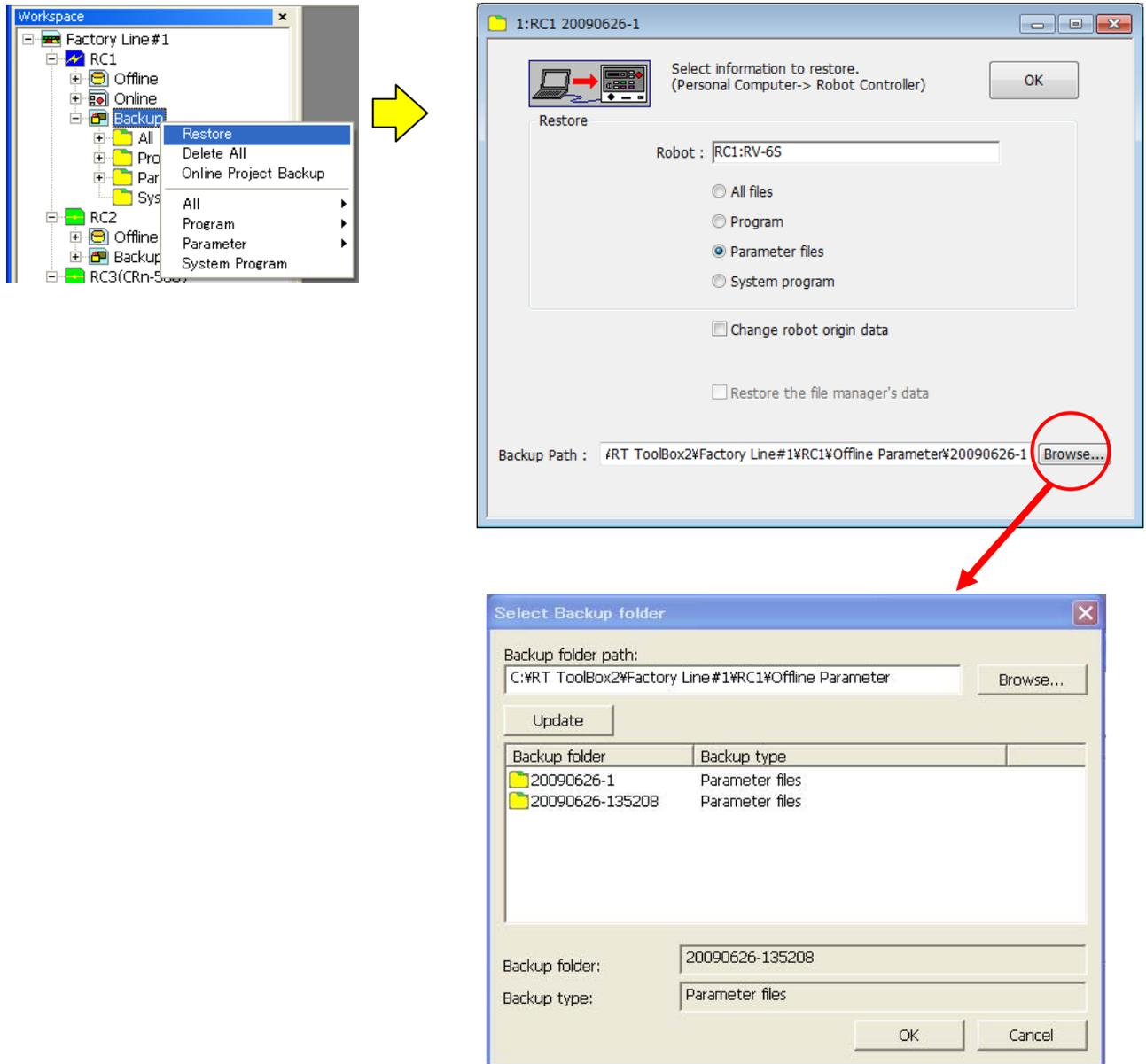
**Figure 10-70 Restoring of parameter file by using backup function**
