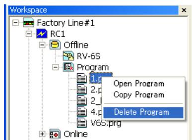
Figure 8-66 Program deletion by using the project tree(Version 1.3 or later).
