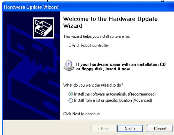
1) When you connect the computer and CR750-D/CRnD-700 series robot controller with a USB cable, the screen on the left is displayed. Select "Install the software automatically (Recommended)", then click the [Next] button. Installation of the USB driver starts.
