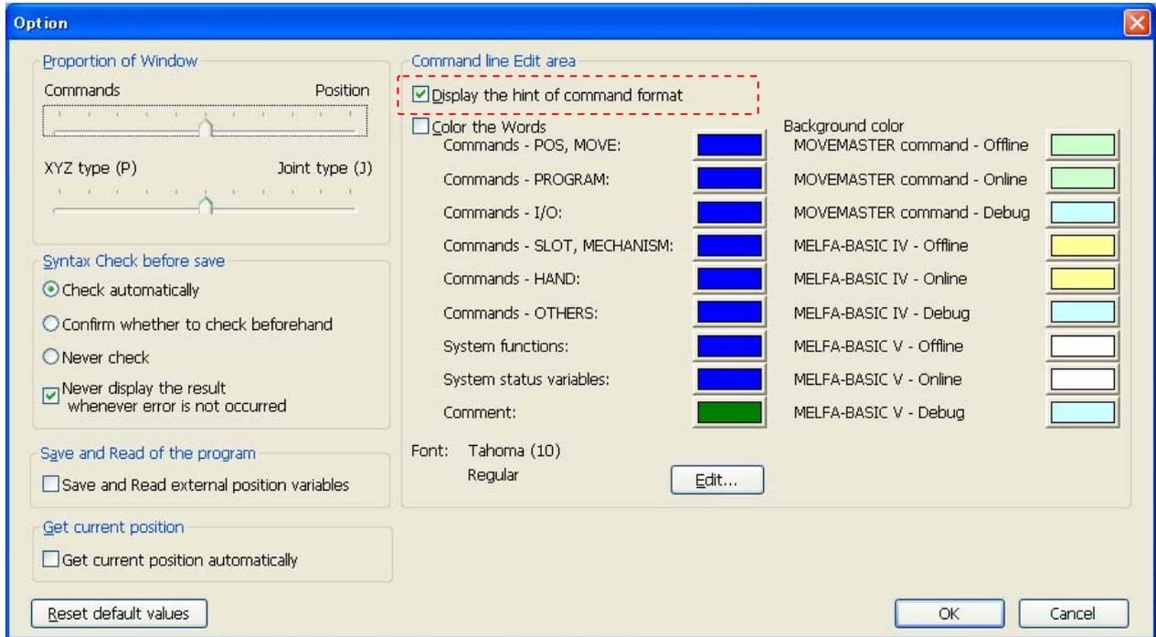
Figure 8-12 Command Edit Area Command Format Hint Display Settings
