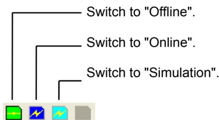
**Figure 5-16 Explanation of Tool Bar**
