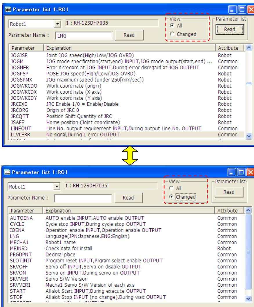
**Figure 10-5 List of parameter changed from initial value**
