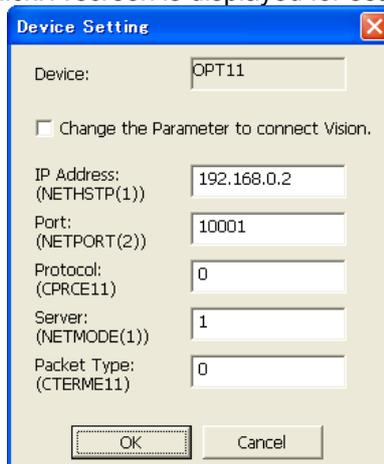
Figure 10-55 Device parameter setting (Version 2.50C or earlier)
