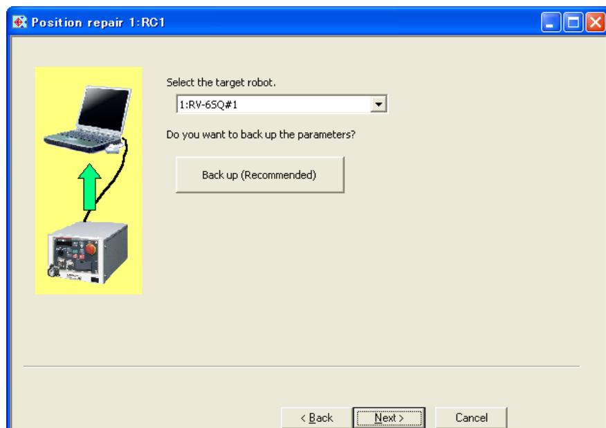
Figure 12-23 Robot and Backup Parameters Selection Window
