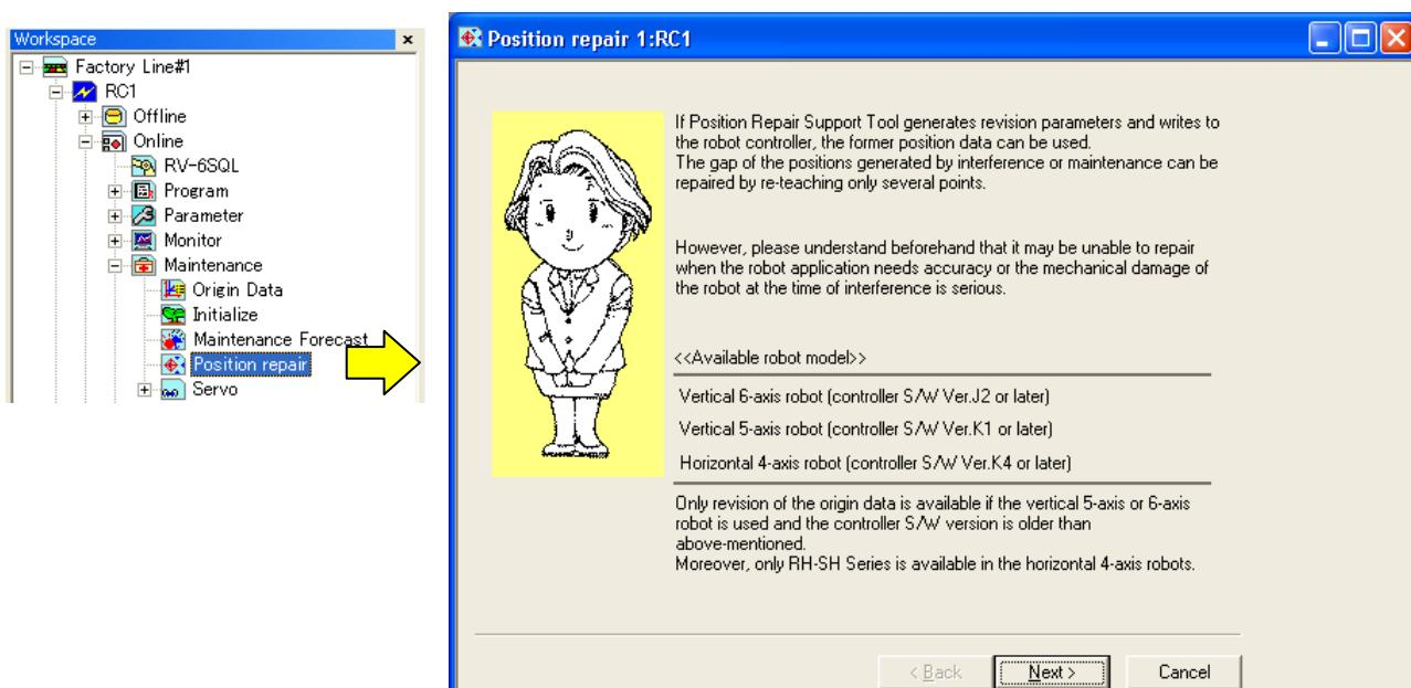
**Figure 12-20 Starting Position Repair**
