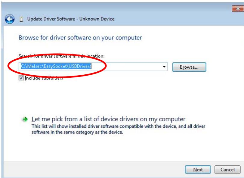
5) The screen on the left is displayed, set "C:\Melsec\Easysocket \USBdrivers". If volume MELSOFT products have been installed, browse the installation destination "EasySocket\USBDrivers" of the first installed product. After setting, click the "Next" button.
