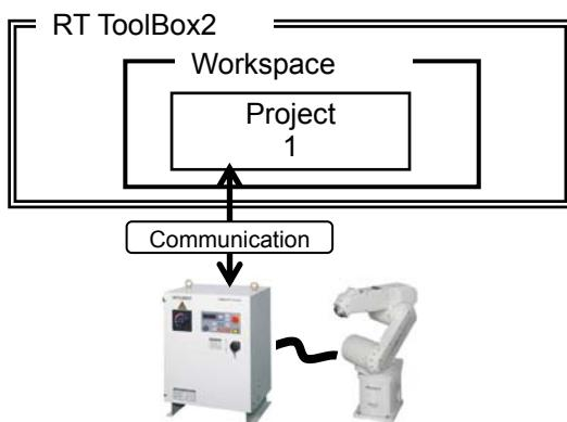
Figure 5-2 Using One Robot Controller
