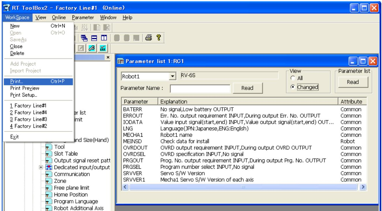
**Figure 10-65 Printing the parameter changed from initial value**
