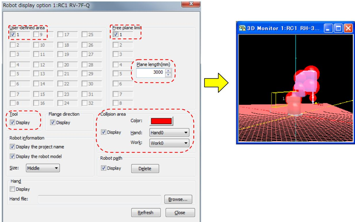
Figure 16-14 Display of Robot display option
