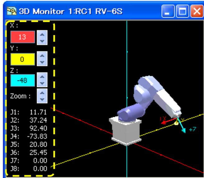
Figure 16-8 the panel to change the perspective of robot view
