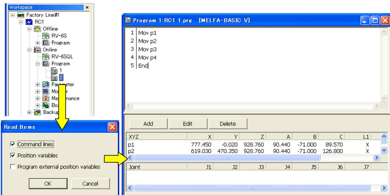
Figure 8-5 Opening a Program in a Robot Controller
