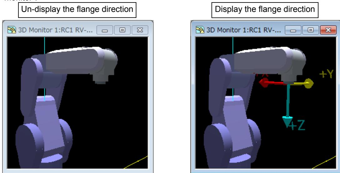
Figure 16-16 Un-display / display of the flange direction
