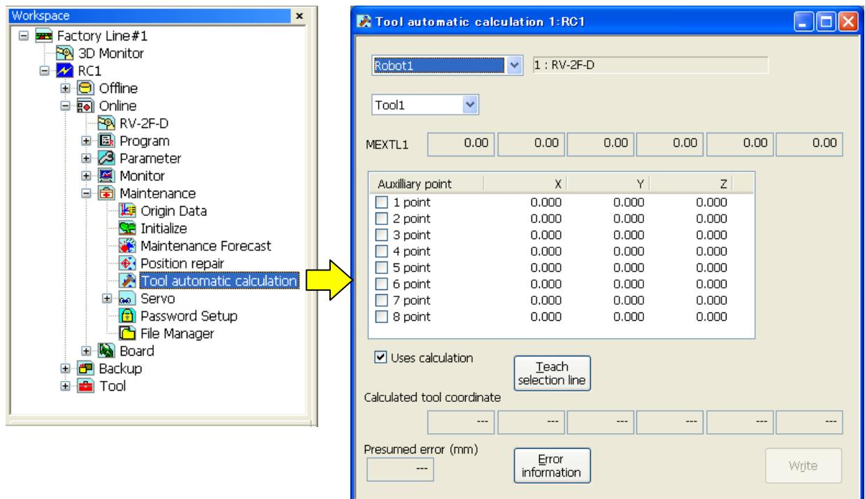
Figure 12-37 Starting the “Tool automatic calculation”
