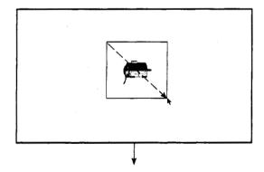
Set the cursor frame to a larger area than the component area. If the enclosed area is smaller than the component, the component cannot be set.
