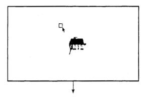
Hold down the left button and move the mouse cursor diagonally down so that the cursor frame encloses the component.
