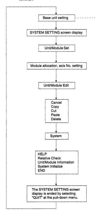
When the base unit is designated at the base unit selection dialog box, the base unit default configuration will be displayed at the SYSTEM SETTING screen.
