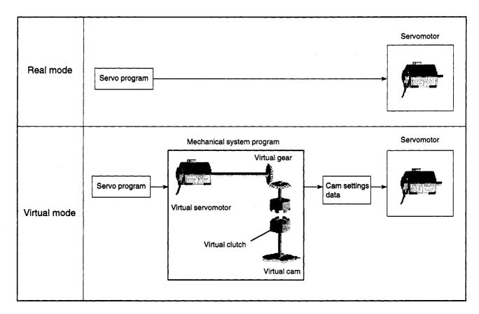
Fig. 1.1 Real Mode and Virtual Mode
