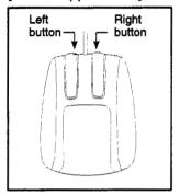
As shown at left, the mouse is equipped with left and right buttons.
