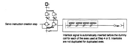
4) In continuous servo instruction creation steps with duplicated axes used at each step and duplicated interlock signals, the duplicated interlock signals are automatically replaced by one interlock signal.
