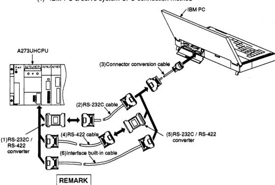
The following converters are recommended in the IBM-PC and servo system CPU connection.
