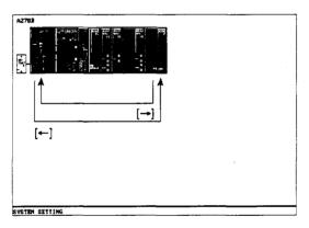
If the  $[\leftarrow]$  key is pressed when the frame is at the left-most module position, the frame will move to the right-most module position.
