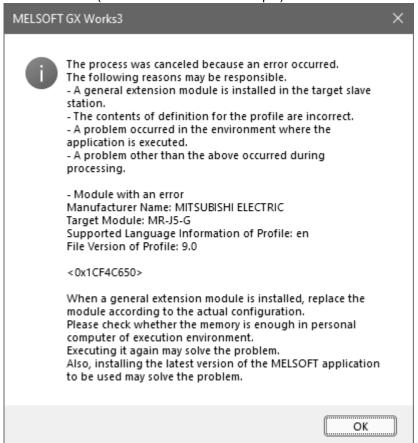
(c) For Simple Motion Module Setting Tool (Version 1.180N as an example)
