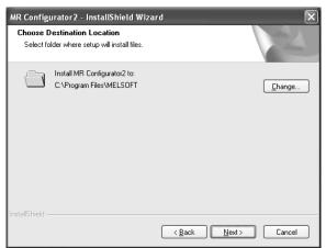
4) The Select installation destination screen appears. Specify the installation destination, and click the "Next" button. This starts installation.
