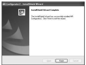
8) When installation is completed, the next screen appears. Click the "Finish" button to end the setup. When restart message appears, starting again to use MR Configurator2.
