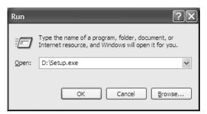
1) Insert the disc into Drive D (disc drive). Then, click the "Start" button on the task bar to open the menu, and click "RUN". When the left window as shown on the left appeared, enter "D:\Setup.exe" and click the "OK" button.
