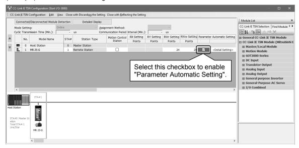
While the servo amplifier is connected, open the Parameter Setting screen from the CC-Link IE TSN Configuration screen and click the Read button to display or edit the parameter setting values of the servo amplifier.
