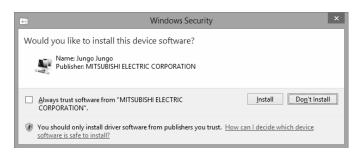
• If the driver is not installed, communication may be partly interrupted. In this case, reinstall MR Configurator2.
