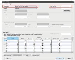
7. Click [Auto recognize]. The inverters connected with the personal computer are automatically detected.
