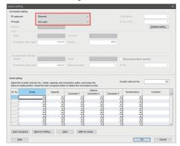
**8.** Select "Model" of the programmable controller connected to the personal computer.
