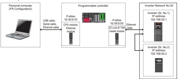
•When using FR-A800 with FR-A8NCG (FR-A800-GN) or FR-F800 with FR-A8NCG and setting the station number using the station number switches
