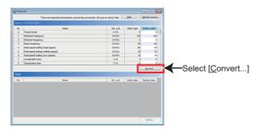
**4.** Specify the model of the [Target inverter] from the lists in the "Convert" sub window. Click [OK] to convert the parameters and close the "Convert" sub window.
