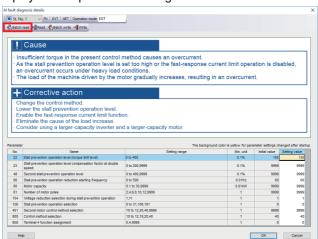
8. Check the corrective actions and change parameter settings as required. After the change, click [Batch write] to write the setting values to the inverters.
