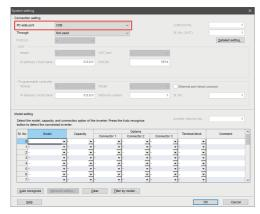
**6.** Click [Auto recognize]. The inverters connected with the personal computer are automatically detected.
