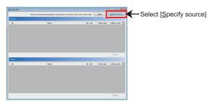
2. Select [Read from connected inverter]. Set the [Connection type], [Target station], and [Connection setting], and click [Detection]. (When multiple inverters are selectable as the source inverter, the "Source inverter" window appears. Specify the model of the [Source inverter].) After detection, confirm the inverter model in the [Model] field, and click [OK]. The parameters are converted and the "Source" window closes.
