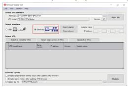
**5.** Click the "Select adapter" button. In the "Select Ethernet Adapter" window, select the network adapter to which the personal computer and inverter are connected. Then click the "OK" button.
