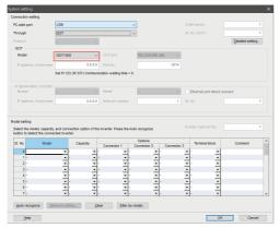
**8.** Click [Auto recognize]. The inverters connected with the personal computer are automatically detected.
