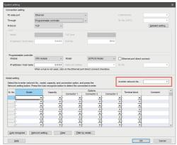
**9.** Click [Auto recognize]. The inverters connected with the personal computer are automatically detected.
