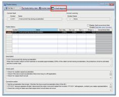
4. The AI fault diagnosis function is activated to find probable causes and display corrective actions for the fault in the fault history using AI technology.
