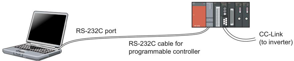
Connect the built-in RS-232C port of the programmable controller to the RS-232C port of the personal computer. Dedicated RS-232C cable QC30R2 is available.
