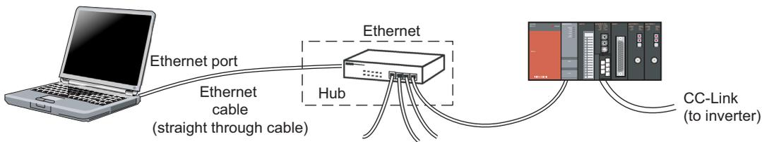
Connect the built-in Ethernet port of the programmable controller to the Ethernet interface module using the Ethernet port of the personal computer. (Straight through cable is available.) Use a hub satisfying IEEE802.3 10BASE-T or IEEE802.3 100BASE-TX standard.
