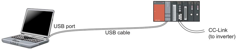
Connect the built-in USB port of the programmable controller to the USB port of the CPU personal computer. One personal computer is connected to one programmable controller. Connection using a USB hub is not supported.
