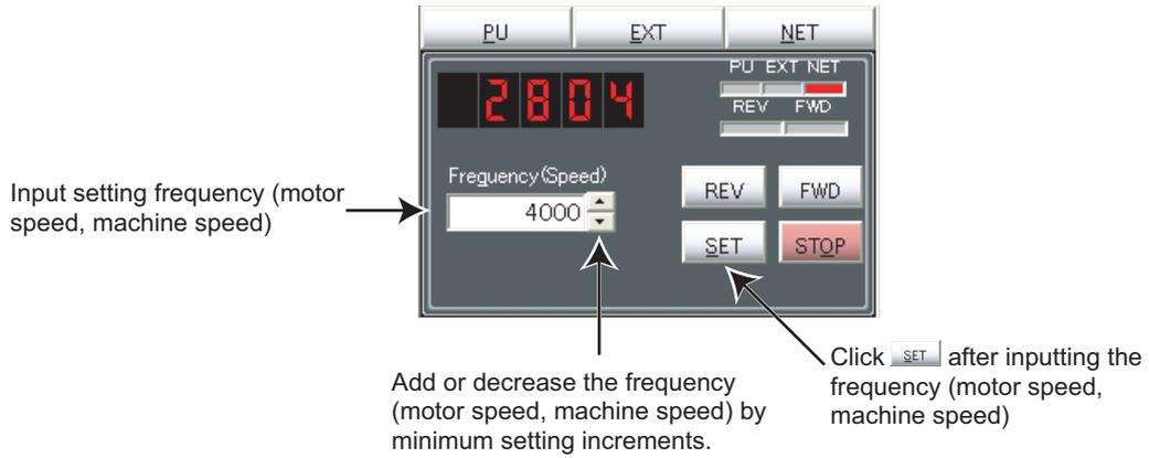
When the set frequency is written, "F" and the "set frequency (speed, machine speed)" is displayed alternately 3 times. After displaying 3 times, the display shows output frequency (speed, machine speed).
