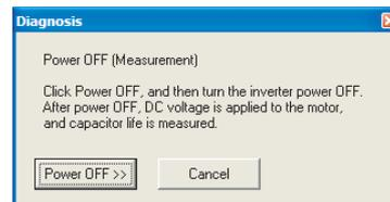
(4) After making sure that the POWER lamp of the inverter is OFF, switch ON the power supply again. Click
