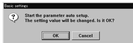
By pressing the [OK] button, the parameters are set automatically and the new values of the parameters that may be set automatically are displayed.
