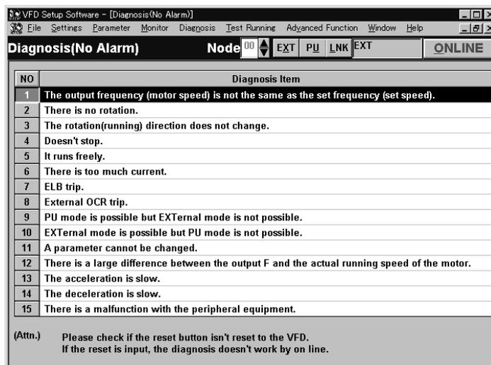
Diagnosis (No Alarm): Shows the diagnosis items. When you choose the corresponding item, the panel appears. Enter data in accordance with the display. As a result, the estimated cause, etc. is shown. For diagnosing the running status, the online mode must be selected.
