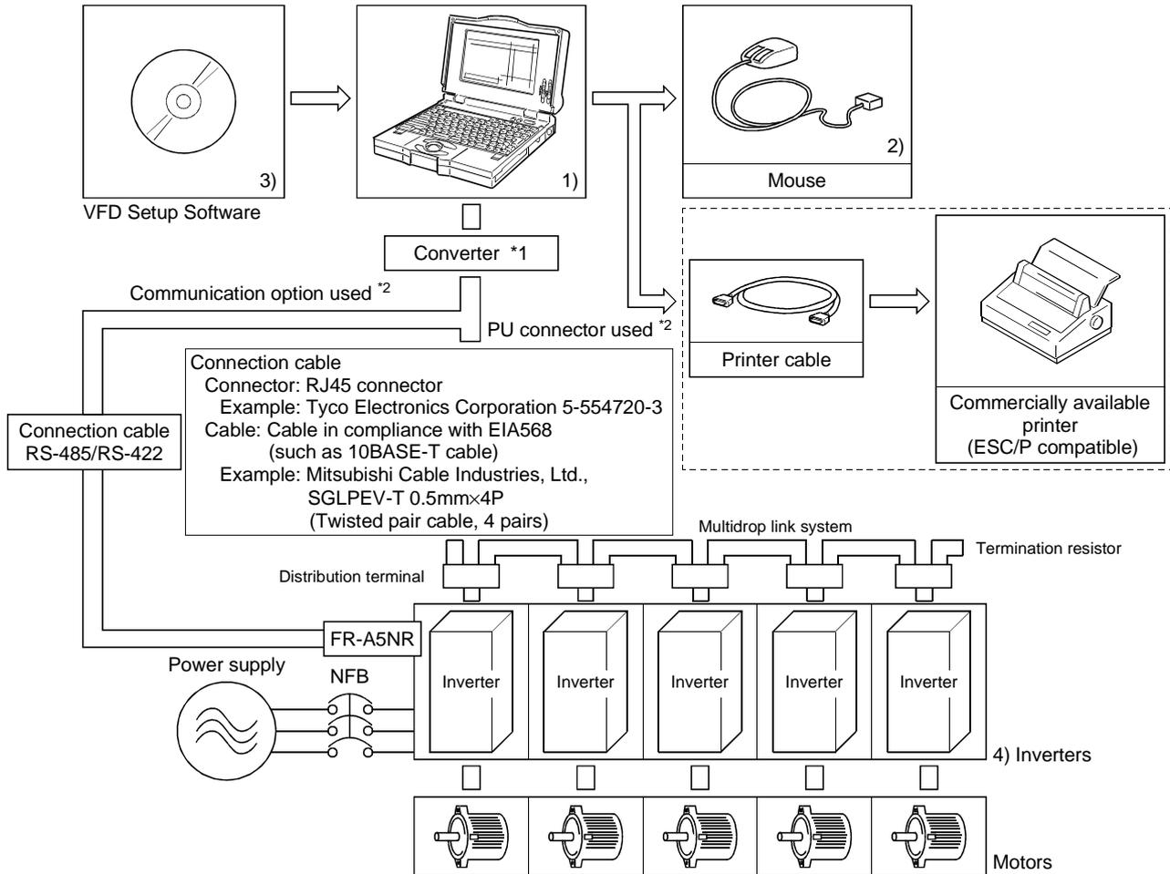
\*1: A converter commercially available is required when the personal computer uses the RS-232C port.
