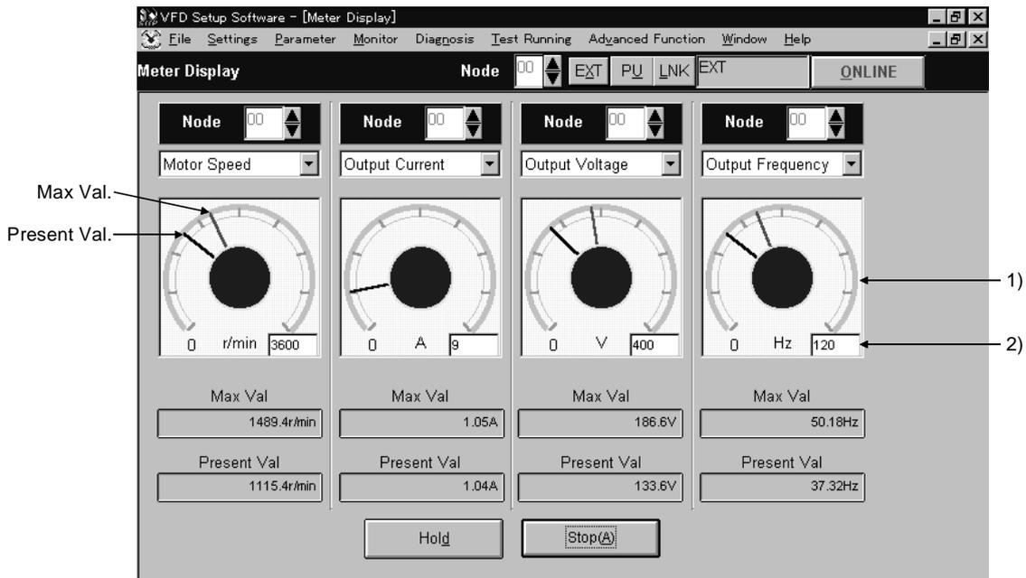
Perform operation as with Data Display. The meter scales are automatically adjusted. After the parameters are batch-read, they are set to the optimum values.
