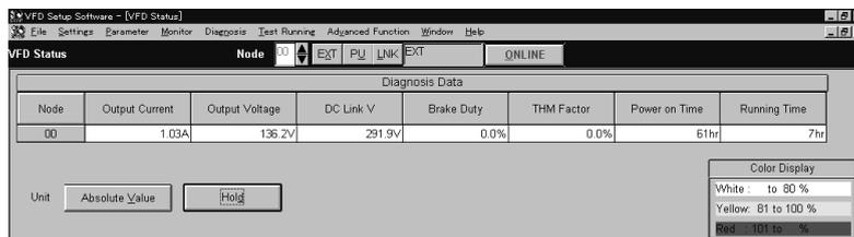
VFD Status: Displays the output current, output voltage, DC link V, Regenerative brake duty, THM factor, Power on Time and Running Time data of all inverter stations specified in the system settings in real time. The data can also be locked by pressing the [Hold] button (Alt+D). The values displayed can be switched between absolute value indication and % indication (Alt+V).
