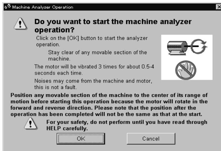
Machine analyzer operation start screen
