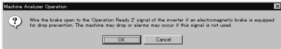
Clicking the [Cancel] button returns to the Machine analyzer setting screen.
