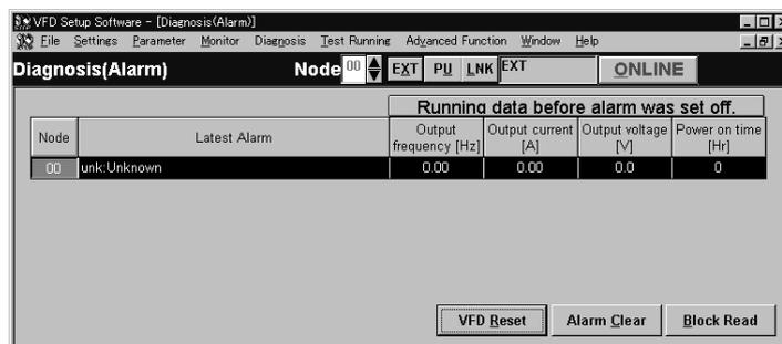
Diagnosis (Alarm): Click the [Block Read] button (Alt+B) to batch-read the information of the inverters where alarms have occurred. By clicking the corresponding item, its comment appears.
