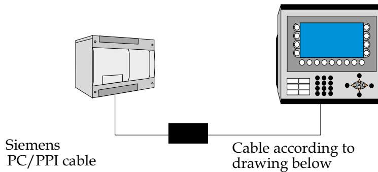
The Siemens PC/PPI cable 6ES7 901-3BF00 from Siemens is connected to PPI port on the PLC system. The cable between the RS-232 port on the terminal is connected according drawing below.
