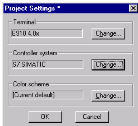
Press **Change...** under Controller system to get the choice list of available drivers. Choose Brand name, Protocol and Model and then press OK. Press OK again to confirm the project settings.
