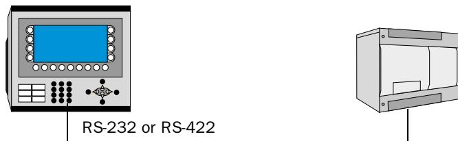
The point-to-point connection can be done via the RS-232C port on the terminal to the RS232 interface on the module USS21A, USS11A, MP/MPB or AIO on the SEW Eurodrive MOVIDYN. For cable configuration see cable drawing below.
