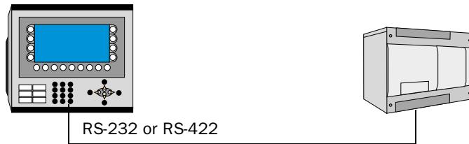
The point-to-point connection can be done via the RS-232C port on the terminal to the RS232 interface on the module USS21A on the SEW Eurodrive MOVIDRIVE. For cable configuration see cable drawing below.
