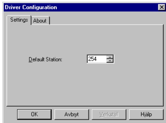
Under Settings you define the default station number. Values 0-99, 254 and 255 can be stated. 0-99 are individual addresses to inverters while 254 is an general address for point-to-point communication. Address 254 can not be used if there are more than one inverter connected to the network because any inverter will reply to this address irrespectively of it's own address. Address 255 is an broadcast address which all inverters are listening to and they will not reply to this message.
