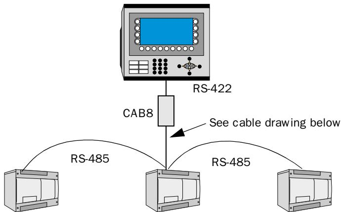
The terminal is connected to an RS-485 network via the adaptor CAB8 which is connected to the RS-422 port on the terminal. CAB8 is a standard adaptor that can be ordered from Beijer Electronics.
