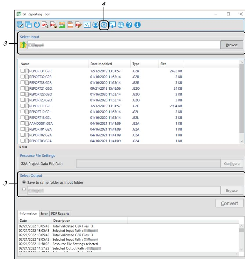
3. Enter the path to the network drive in [Select Input] or [Select Output] in the main window.
