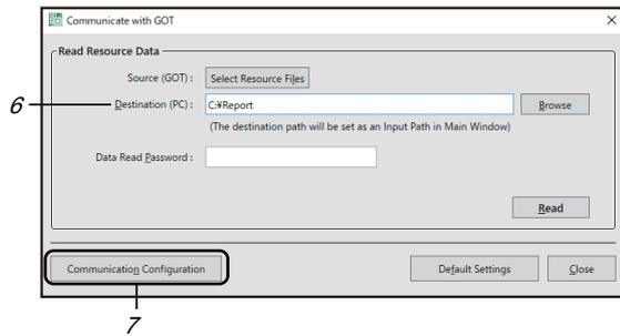
7. Click the [Communication Configuration] button to display the [Communication Configuration] dialog.
