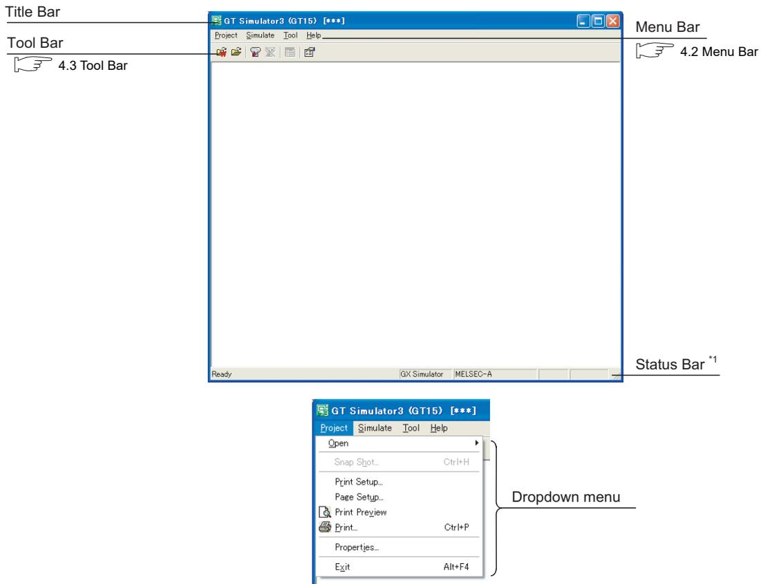
\*1 When using the GOT1000 series (GT11/GT10) simulator, the whole status bar can not be displayed as the screen size is 320 x 240 dots or less.
