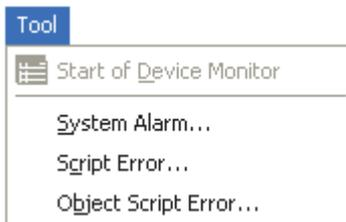
The Tool menu contains options for starting/exiting Device Monitor and displaying each error information.
