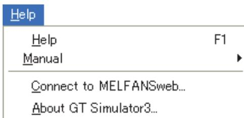
The Help menu contains functions for displaying the GT Designer3 Help and the PDF manual related to the GT Simulator3, as well as for checking the software version.
