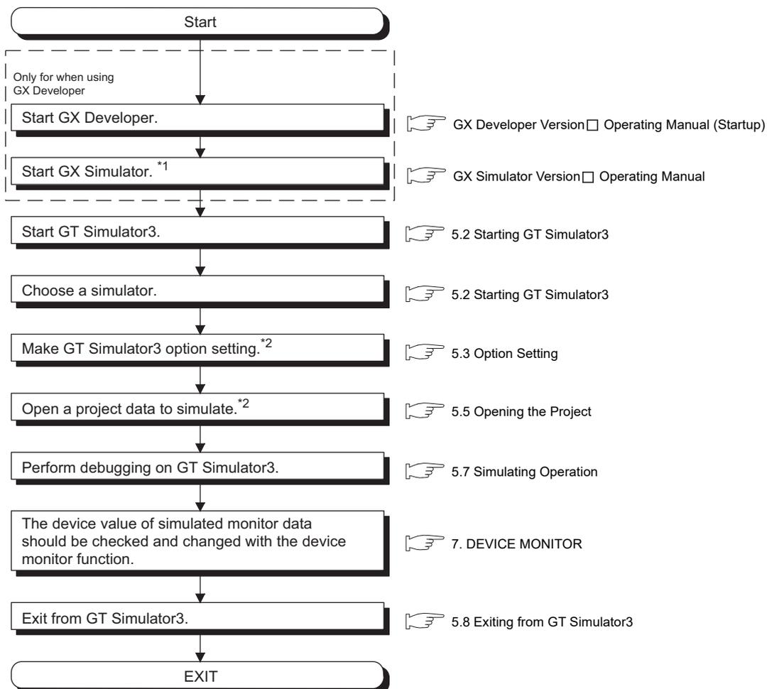
\*1 In the case that GX Developer is not used, GX Simulator is automatically started when the simulation is executed on GT Simulator3.
