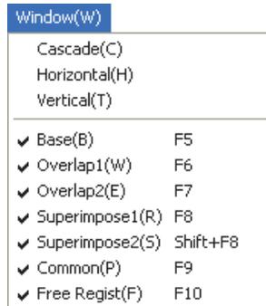
Window menu includes the functions such as aligning the Device Monitor screens and selecting display screens.
