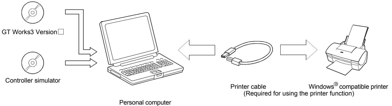
Install a controller simulator to be connected.
