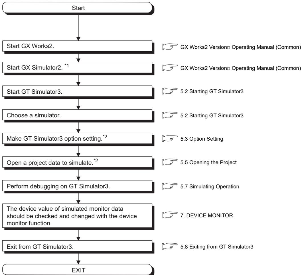
\*1 GX Simulator2 does not start automatically when GT Simulator3 starts a simulation. Start GX Simulator2 from GX Works2 in advance.
