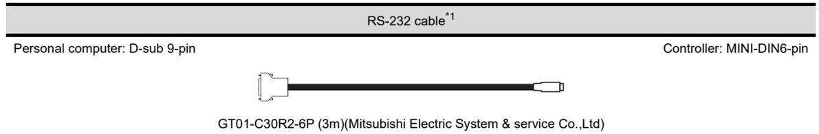
\*1 The adapter L6ADP-R2 is required for the direct CPU connection.
