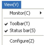
View menu includes the functions such as starting/stopping monitoring and setting the Device Monitor.
