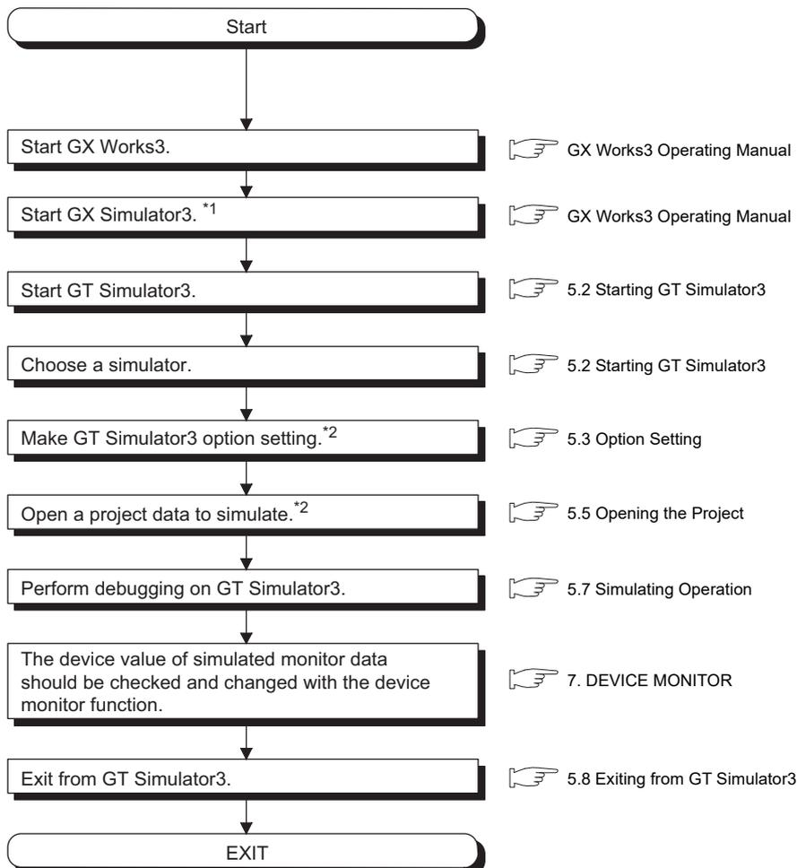
\*1 GX Simulator3 does not start automatically when GT Simulator3 starts a simulation. Start GX Simulator3 from GX Works3 in advance.
