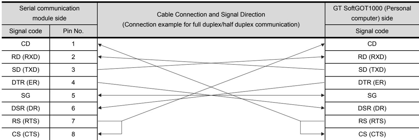
\* DC code control or DTR/DSR control is enabled by connecting the QC24 (N) to an external device as shown above.
