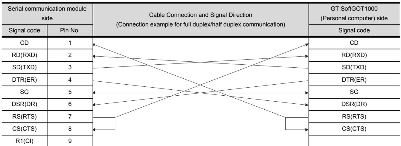
2) Connection example which cannot turn ON/OFF CD signal (No. 1 pin)
