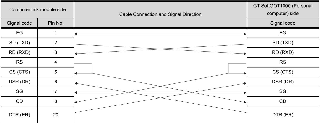
2) Connection example 2 when the C24 (computer link module) has a 25-pin connector
