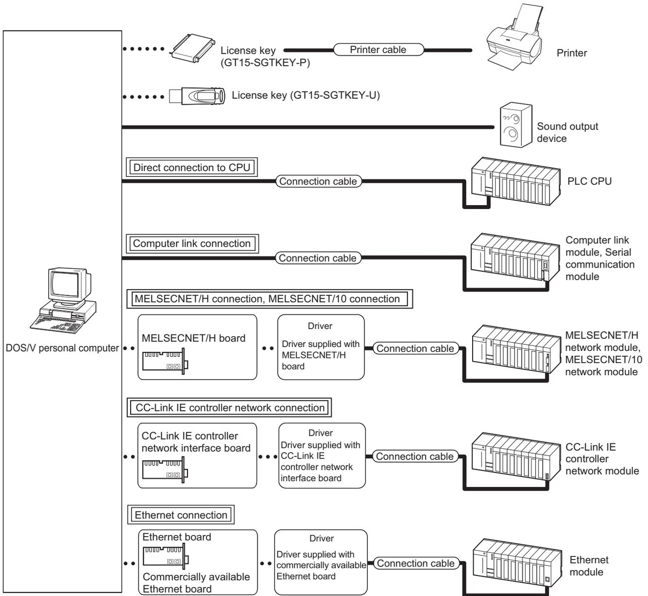
(2) When using GT SoftGOT1000 with PC CPU module
