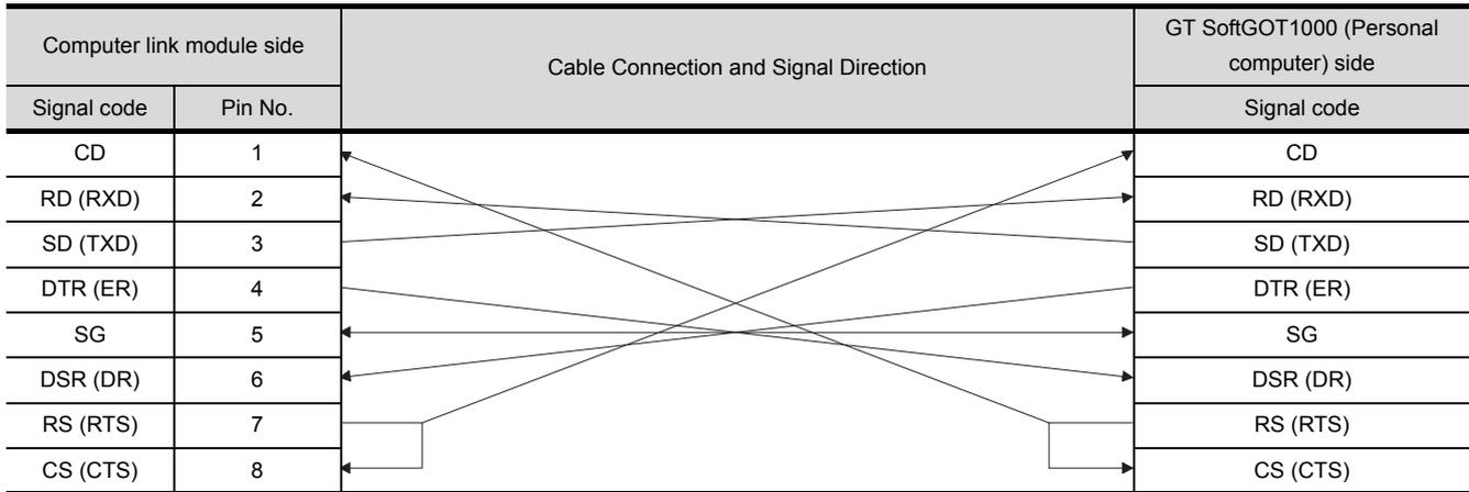
4) Connection example 2 when the C24 (computer link module) has a 9-pin connector
