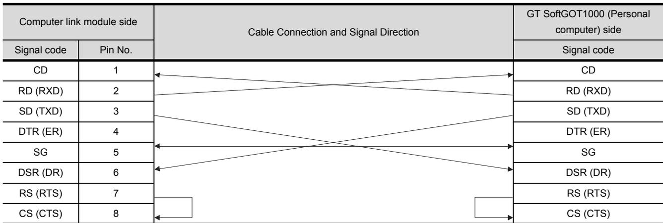
\*1 DC code control or DTR/DSR control is enabled by connecting the DTR and DSR signals of the computer link module to an external device as shown above.
