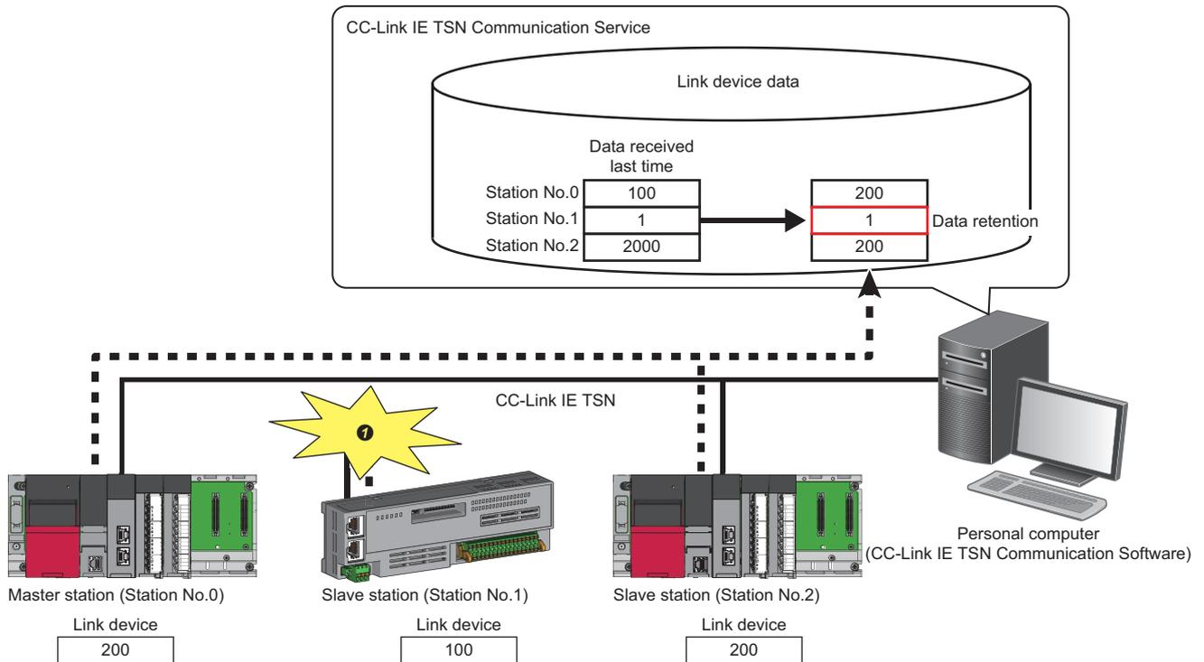
① CC-Link IE TSN Communication Service retains the last received link device data because a disconnection occurs in the slave station (station No.1) on CC-Link IE TSN and CC-Link IE TSN Communication Service fails to receive its link device data.
