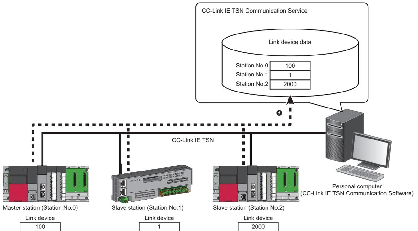
① CC-Link IE TSN Communication Service receives link device data which is sent by CC-Link IE TSN.
