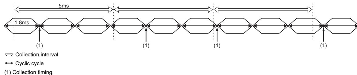
A collection interval can be specified longer than that of a cyclic cycle; therefore, the amount of data stored in the buffering area can be suppressed.
