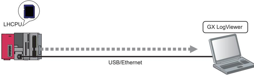
An LHCPU can be connected to a personal computer with the following communication routes.
