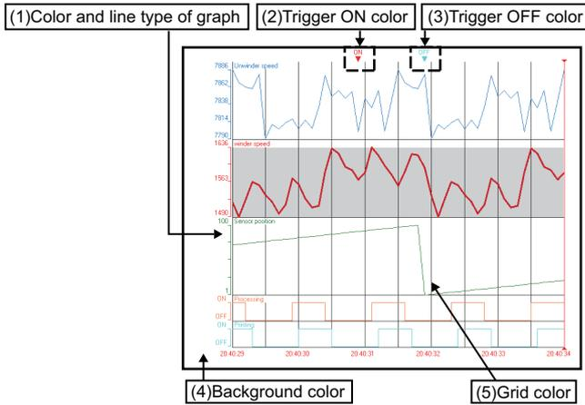
The color settings for the background, grid, and trigger ON and OFF are common to all trend windows, so any changes are applied to all the trend windows being displayed; however, the color settings does not support the 'Set Graph View by the Auto Reflect Function' function.
