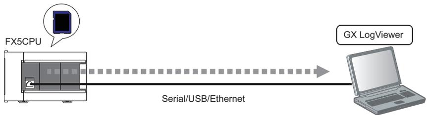
An FX5CPU can be connected to a personal computer with the following communication routes.
