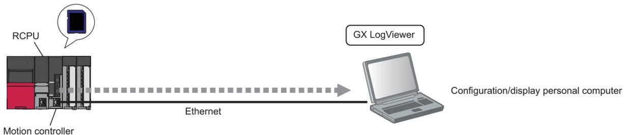
A motion controller can be connected to a personal computer with the following communication route.
