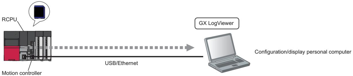
An RCPU can be connected to a personal computer with the following communication routes.
