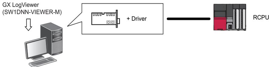
Use an Ethernet board that is built-in to a personal computer or commercially available.
