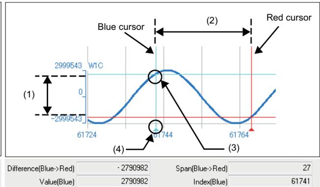
Since an analog module does not have time information in the logging data, only the index display is available.
