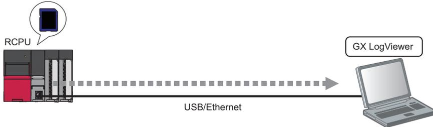
An RCPU can be connected to a personal computer with the following communication routes.
