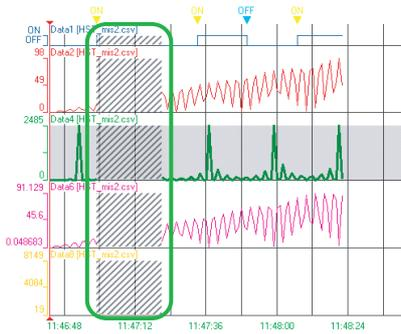
When the data of a CPU module is sampled at less than 1 millisecond interval, '0' is output to all digits of microsecond or less of the sampled time in the file to which the sampled data output.
