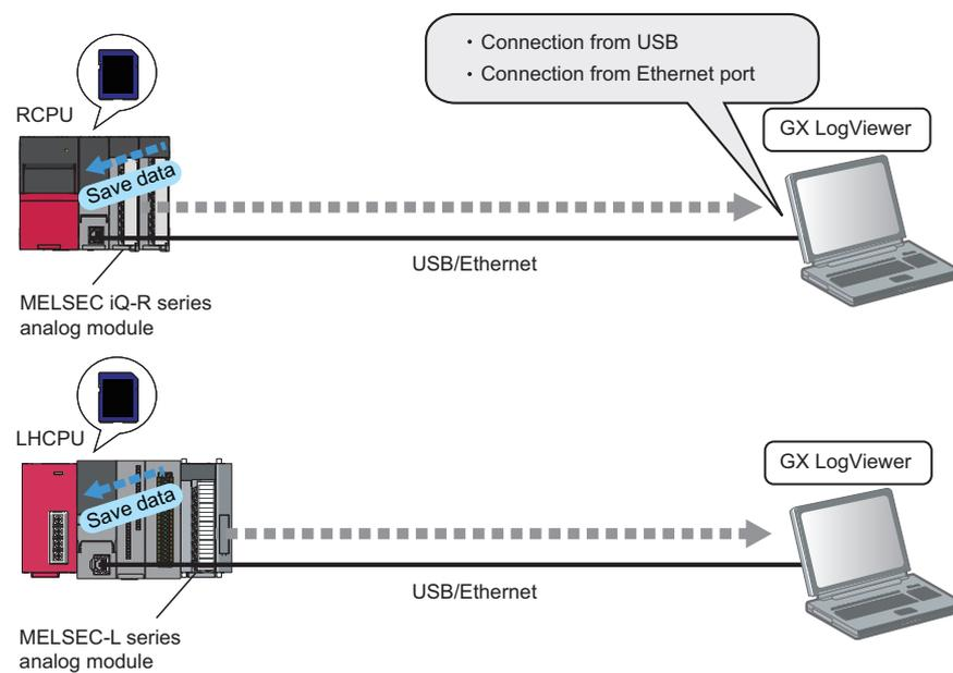
The communication route for a MELSEC iQ-R series analog module is the same as that for an RCP.
