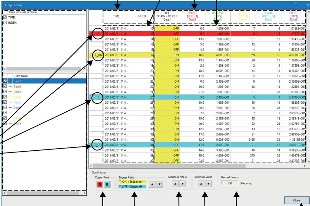
The screenshot shows the 'Dump Display' window with a table of data. The table has columns for TIME, INDEX, BIT (On/Off), and several numerical data columns. Annotations (1) through (12) point to specific UI elements:
