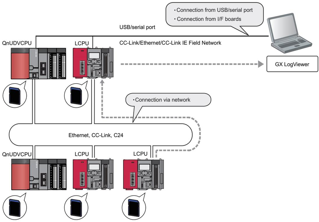
A QnUDVCPU and an LCPU can be connected to a personal computer with the following communication routes.
