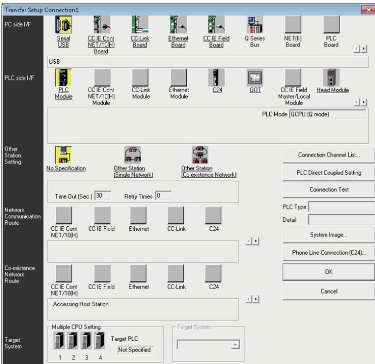
An item underlined in the "Transfer Setup" screen can be set the detail by double-clicking it. In addition, an item that has been set is highlighted in yellow.
