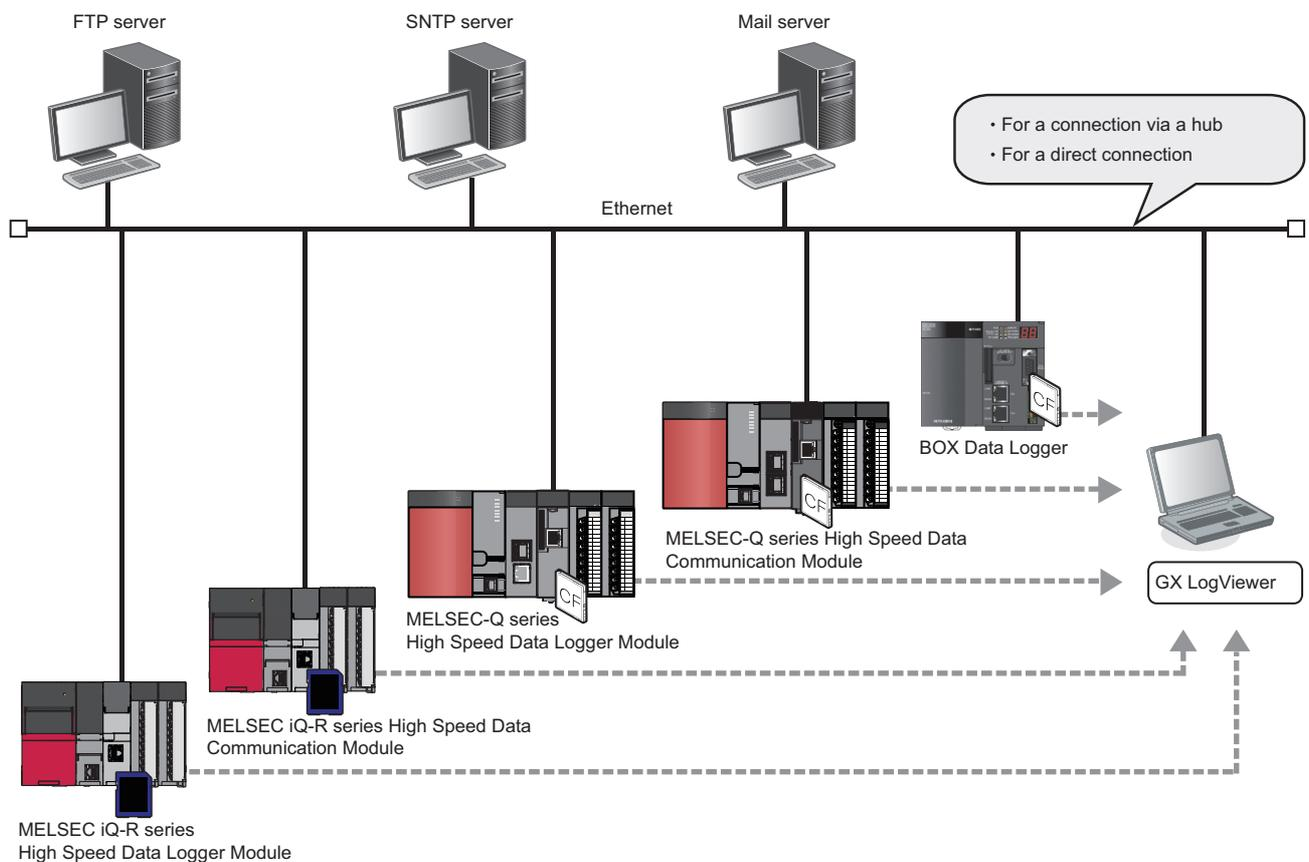
A data logger and data communication can be connected to an Ethernet port of a personal computer with the following communication routes.
