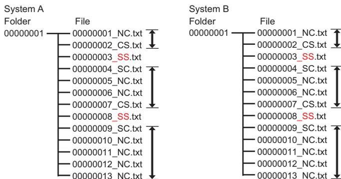
A data logging file of an RnPCPU (redundant mode) can not be consecutively displayed with a data logging file of the different system.
