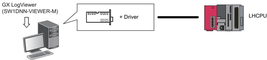
Use an Ethernet board that is built-in to a personal computer or commercially available.
