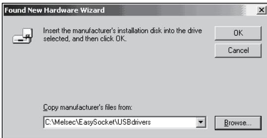
4) As the screen on the left appears, set the GX Configurator-QP installation destination "Easysocket\USBdrivers" and click the **Next>**.
