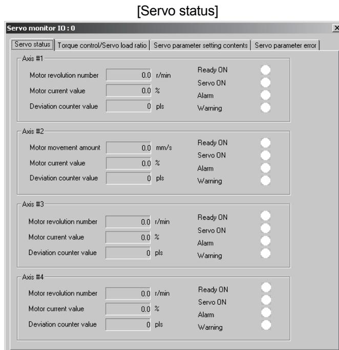
(Screen example: Axis #1 operation monitor screen displayed when the QD75M is chosen in model selection)
