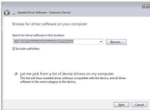
4) The dialog box shown on the left appears. Set the installation location of this product, "EZSocket\EZSocketGOT\Drivers" and click **Next**. The left dialog box shows an example when "C:\MELSEC\EZSocket\EZSocketGOT\Drivers" is set. When multiple MELSOFT products have been installed, set the installation location of the first-installed product.
