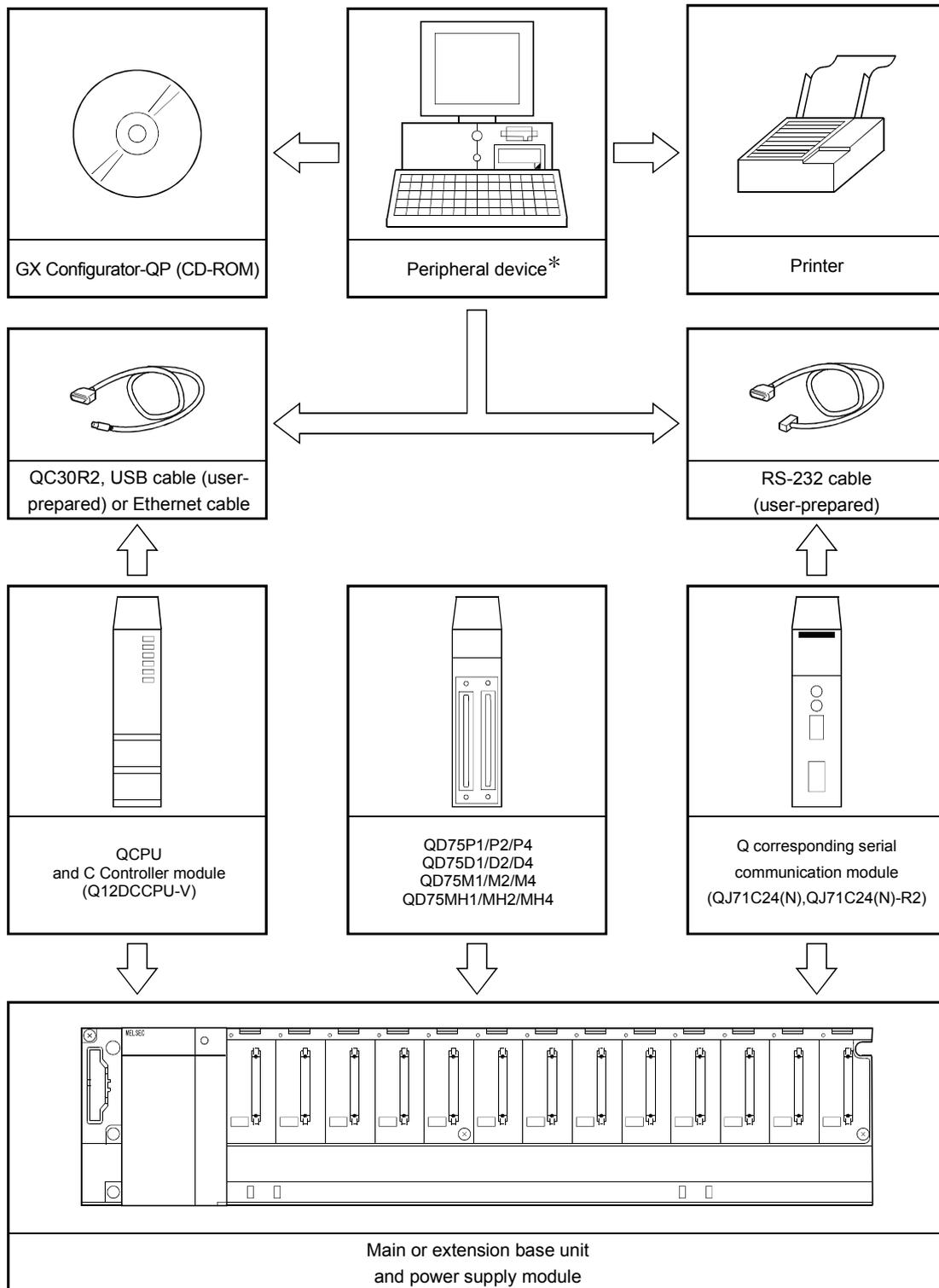
\* : When the PC CPU module is used as a peripheral device, the connection cable is not needed since it is loaded to the base unit module directly. For details of the PC CPU module, refer to Manual for PC CPU module.
