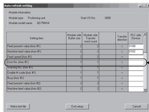
This single line is counted as one parameter that has been set. A blank is counted out. All setting items of this setting screen are added to the numbers of other intelligent function modules to calculate a sum total.
