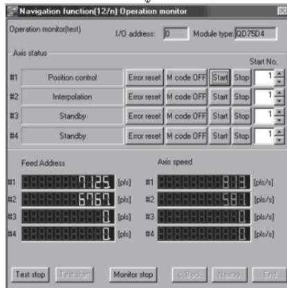
9) Set the positioning data No. in Start and click the "Start" button to start test operation. Use the "Stop", "Error reset" and/or "M code OFF" button as necessary.
