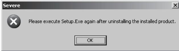
3) If the message shown on the left appears, click the **OK** button, uninstall GX Configurator-QP, and then reinstall it.
