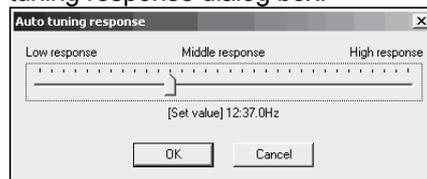
When performing operation from the keyboard, enter the value and press the "Enter" key to determine the value.
