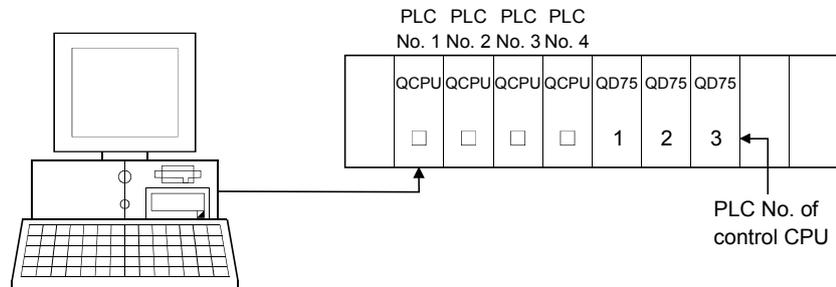
In Connection Setup, specify the control CPU type and PLC No. of the QD75 to communicate with.
