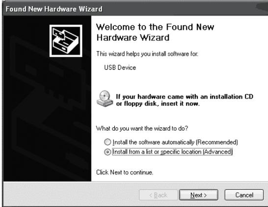
1) The screen shown on the left appears when the personal computer and the CPU module is connected with USB cable. Choose "Install from a list or specific location [Advanced]" and click the **Next>**.
