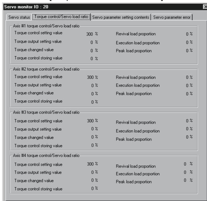
(Screen example: Axis #1 operation monitor screen displayed when the QD75M is chosen in model selection)
