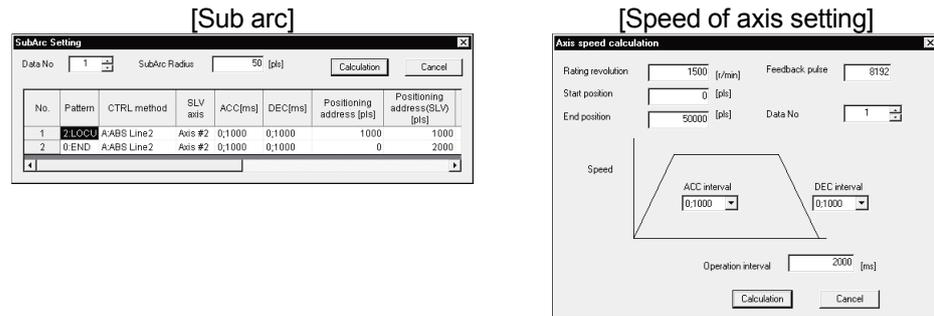
These functions allow the optimum positioning data to be set without complicated calculation and advance measurement.
