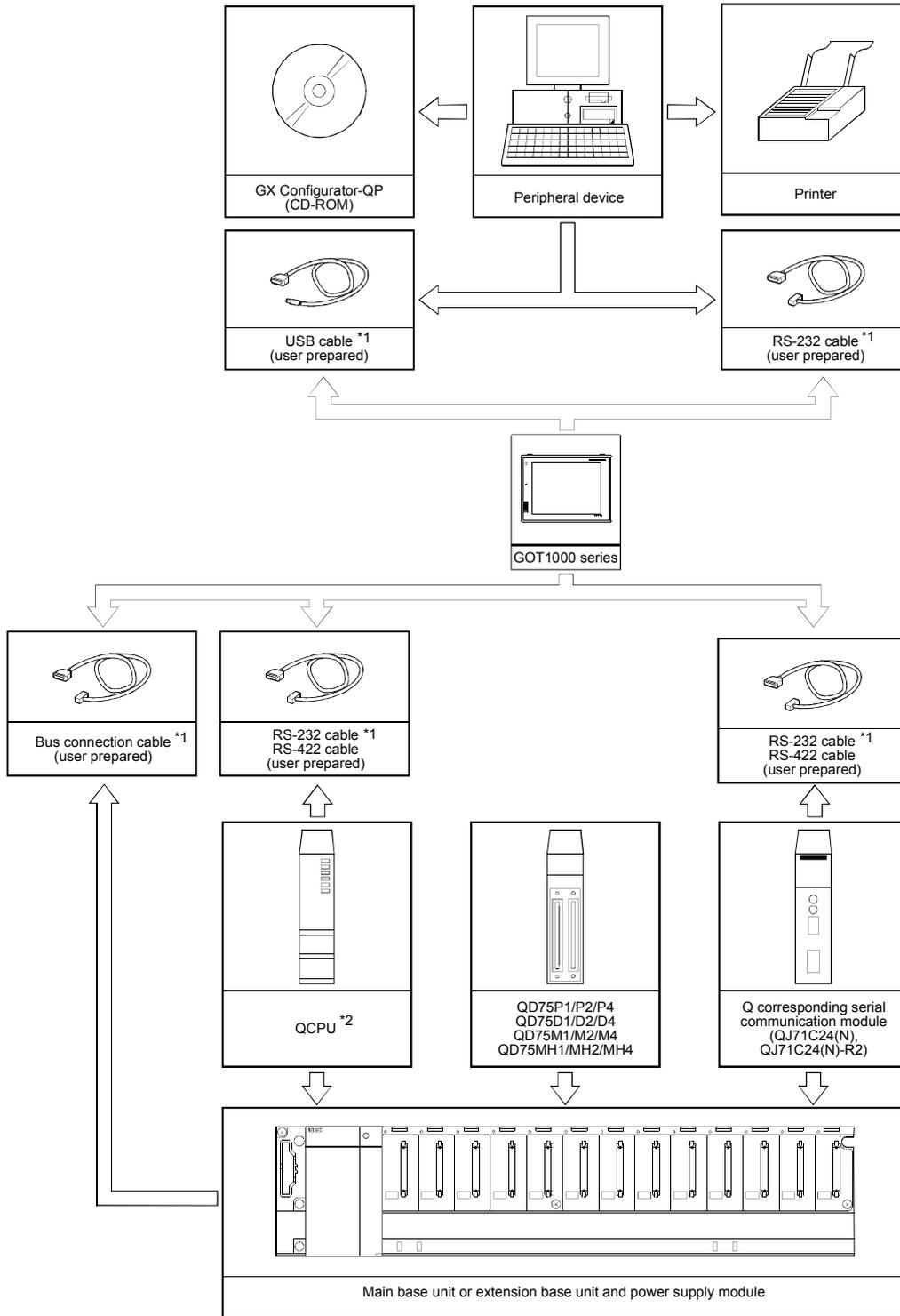
\*1: For cables for connection of a peripheral device to the programmable controller via GOT by the GOT transparent mode, refer to the GOT1000 Series Connection Manual (Mitsubishi Products).
