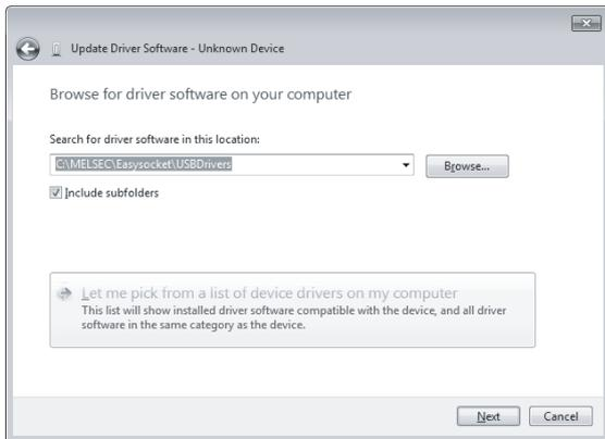
7) The screen shown on the left appears. Set installation location of GX Configurator-QP, "Easysocket\USBdrivers". Then, click the **Next>** button. The left screen is an example when C:\MELSEC\Easysocket\USBdrivers is set. If multiple MELSOFT products have been installed, refer to the installation location of the first installed product.
