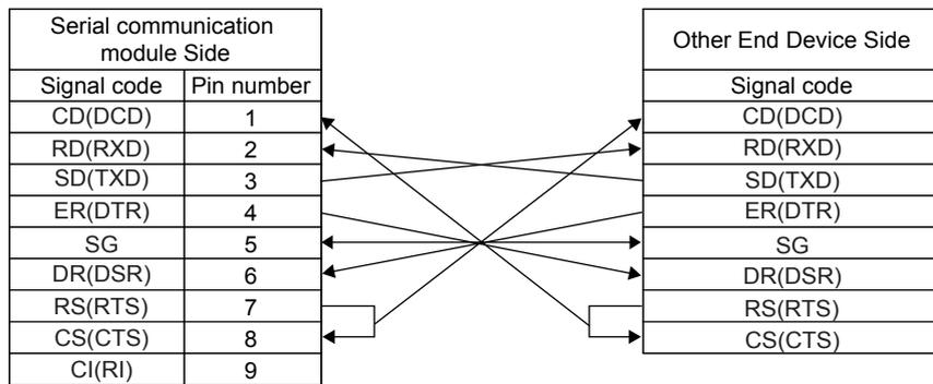
• Connection example which cannot turn ON/OFF CD signal (No. 1 pin)
