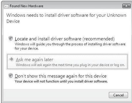
1) The screen shown on the left appears when the personal computer and the CPU module is connected with USB cable. Choose "Locate and install driver software (recommended)" and wait until searching ends.
