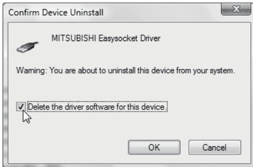
3) The warning dialog box shown on the left appears. Select "Delete the driver software for this device." and click the **OK** button.
