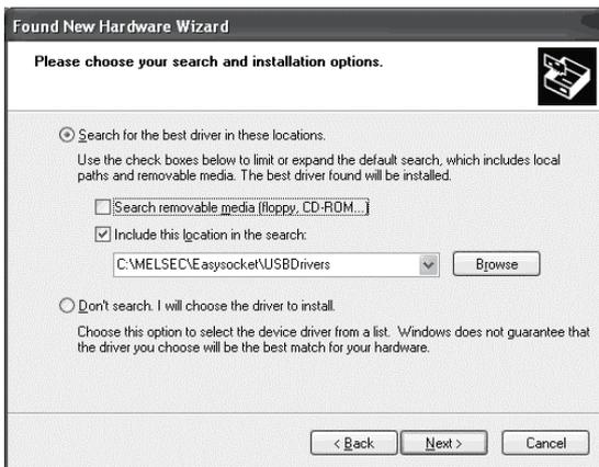
2) As the screen on the left appears, choose "Include this location in the search". Check "Include this location in the search" and set "Easysocket\USBDrivers" of the folder where GX Configurator-QP was installed. After setting, click the **Next>**.
