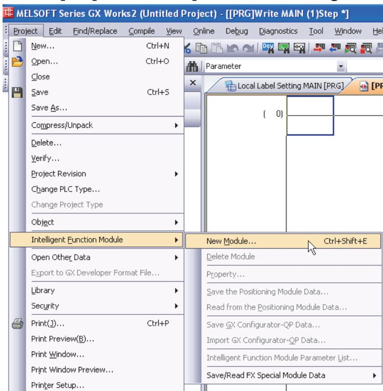
**2** When the "New Module" dialog box appears, set "Module Type", "Module Name" and "Module No.".
