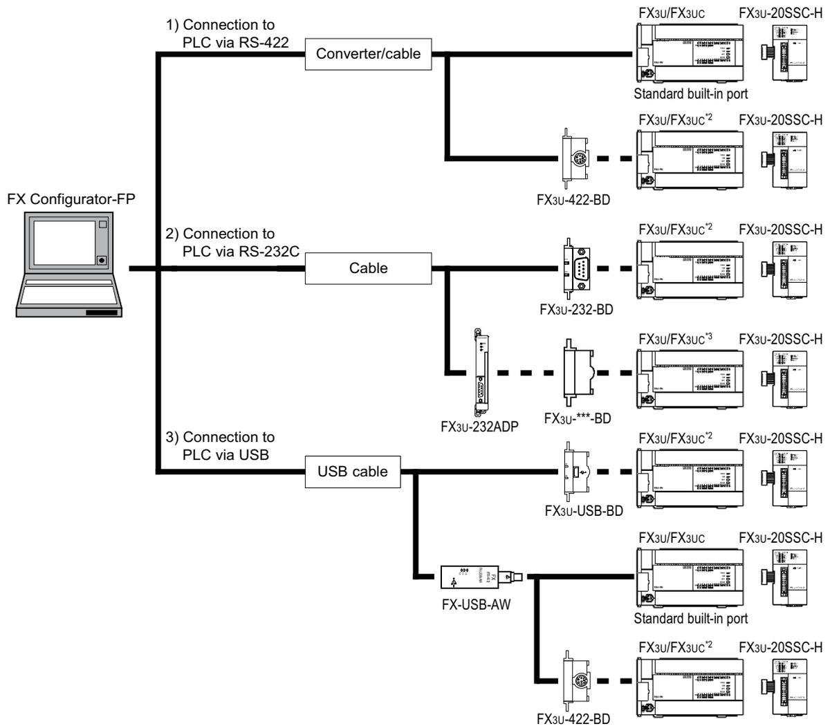
\*2. Expansion boards (FX3U-\*\*\*-BD) can not be attached to the FX3UC-□□MT/D(SS) and FX3UC-16MR/D(S)-T PLC.
