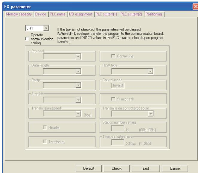
When the PLC type of the project is the FX3U(C), the channel specification (CH1/CH2) combo box appears. When using the FX3U-422-BD, FX3U-232-BD, FX3U-USB-BD or the first FX3U-232ADP connected to the FX3U-CNV-BD, set CH1 and check the settings.
