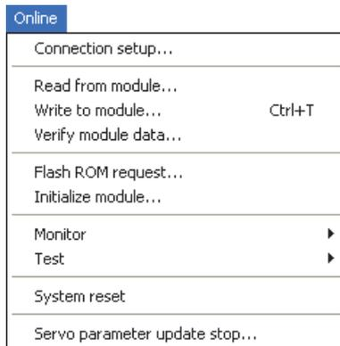
Reads/Writes/Verifies, monitors and tests the module data, etc.
