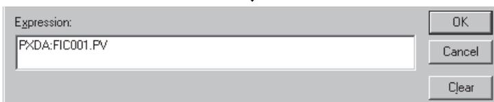
4. A tag name is automatically created at [Expression] of the tag variable setting screen. A format of the created tag name is "Access name:Process control tag name.Tag item".\*1
