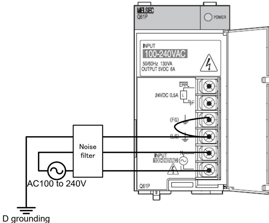
\* An optional noise filter can be installed to the power source line in order to reduce noise more effectively.
