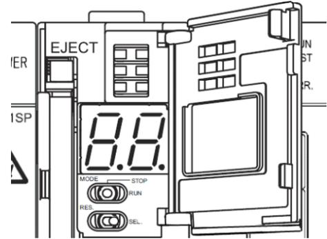
IP address display (Example of 192.168.10.1 set to CH1 and 192.168.3.1 set to CH2.)
