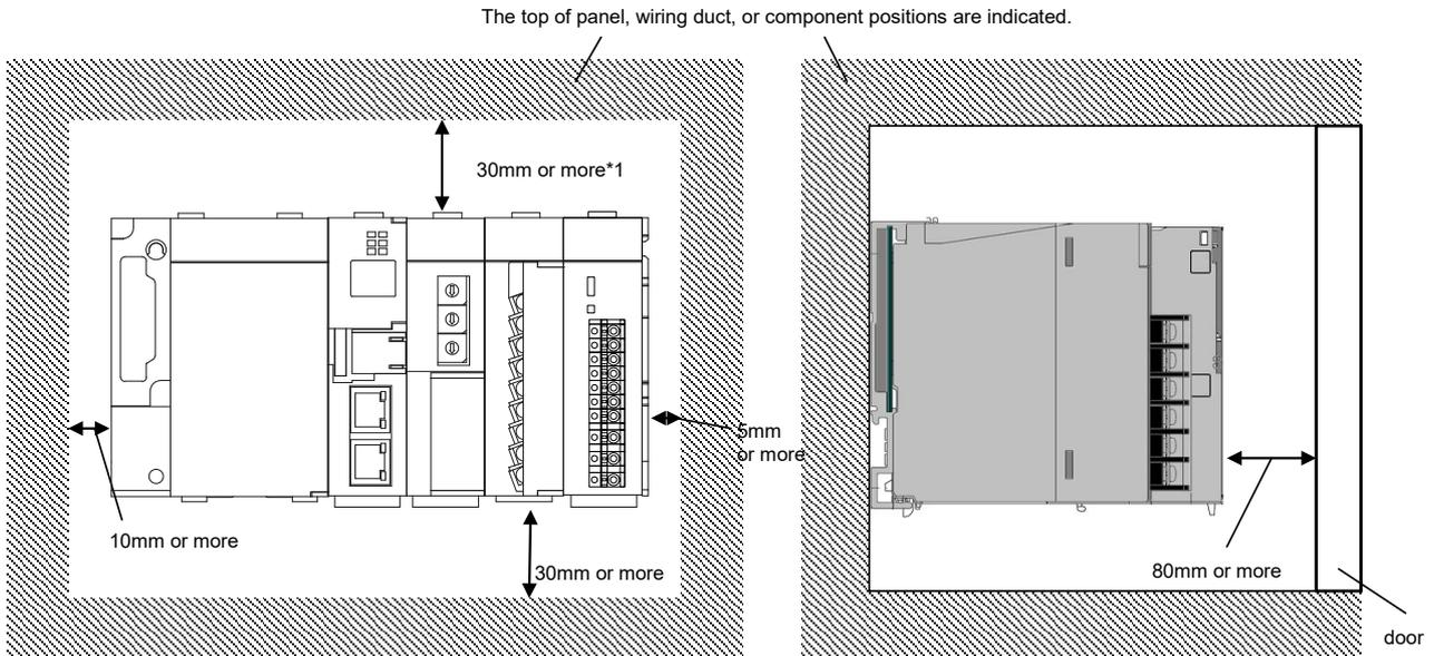
\*1 This length applies when the height of the wiring duct is 50mm or less. If not, the length should be 40mm or more.
