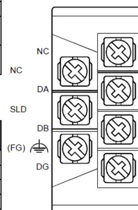
Connect both ends of the shielded wire in a CC-Link dedicated cable to the "SLD" terminal of the unit.
