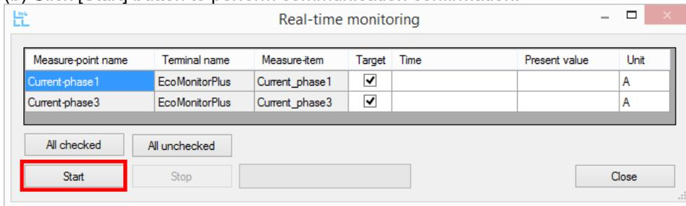
(c) If measured values are displayed in the column of the present values of measuring points for each terminal device, it means that the communication with each connected terminal device has succeeded.
