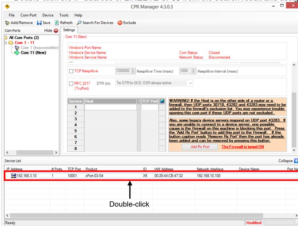
(v) Confirm that the IP address of LINEEYE SI-65 is assigned and click [Save] button.
