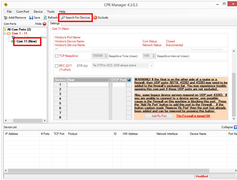
(u) The search result is displayed in Device List. Double-click the IP address of LINEEYE SI-65 from the search result and assign to the COM port.
