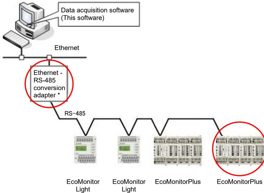
○ : Devices that need the connection of a termination resistor
