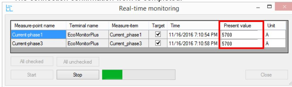
(d) If an error message is displayed or error codes are displayed in the column of the present values of measuring points for each terminal device, it means that the communication with each connected terminal device has failed.
