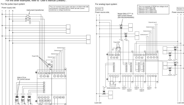
(Note) Connect the k terminal on the secondary side of the dedicated current sensor to the k terminal of the Energy Measuring Unit. Connect the I terminal on the secondary side of the current sensor to the I terminal of the Energy Measuring Unit. Perform the same processing for the 2k, 2l, 3k, and 3l terminals.
