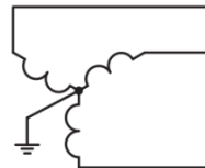
Fig11.4 Three-phase 3-wire (STAR)
