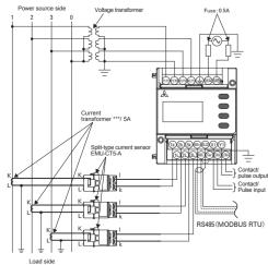
For protection against noise, transmission lines and input/output lines shall not be placed close to or bound together with the power lines and high-voltage lines. Keep distance as below netween them. (except for the terminal block) Condition distance High-voltage line 600V or less 300mm or more Other high-voltage line For the actual usage, connect the FG terminal to ground. (D-type ground: Type 3) Connect it directly to the ground terminal.
