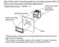
Panel cut dimensions are made larger than the product considering tolerance in panel cut. If you want to prevent dust and other intrusion the gap of panel cut, cut the panel according to the product to be mounted.
