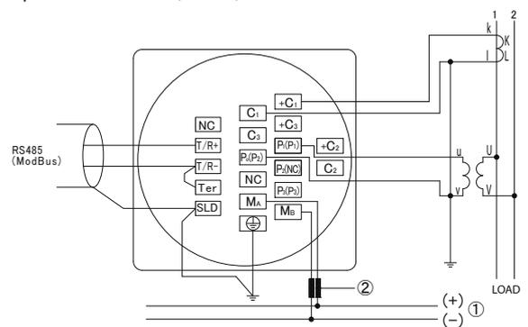
① Auxiliary power supply 100-240 VAC 100 VDC
