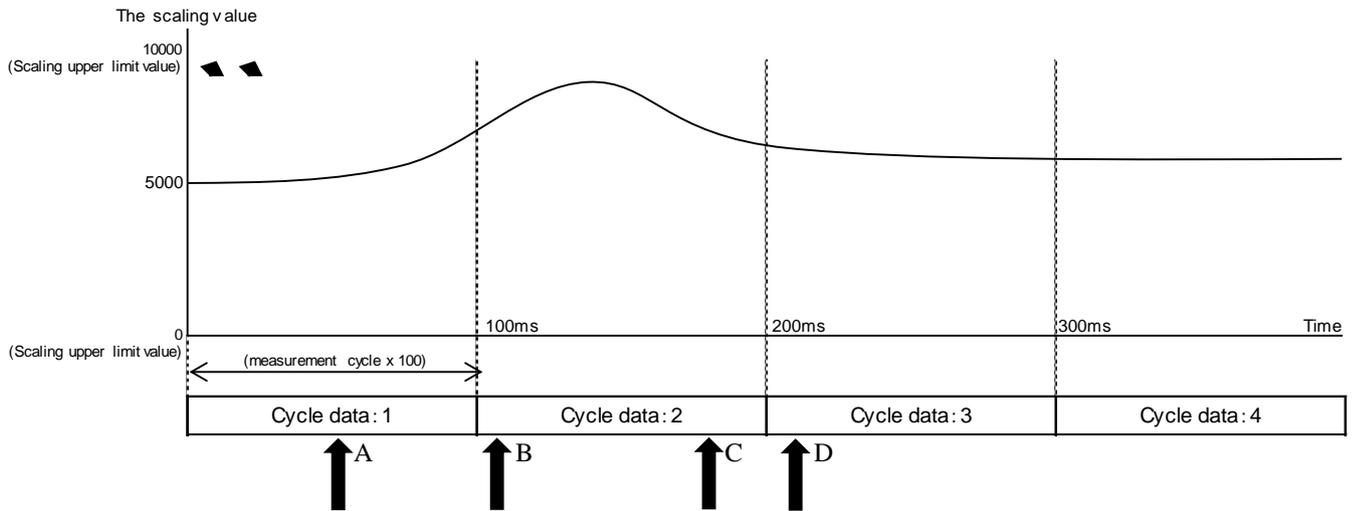
Note1: When monitoring by timing of "A", an A/D conversion is less than 100 times, so 0 replies to cycle data and the scaling value buffer.
