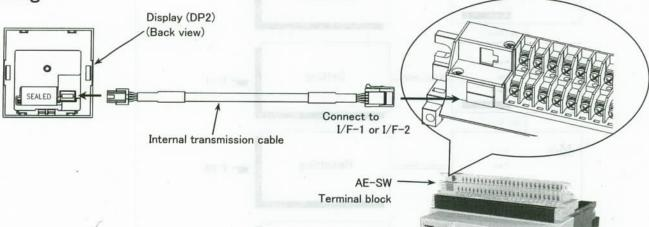
The Display (DP2) is connected to the terminal block of AE-SW with Internal transmission cable as illustrated above.
