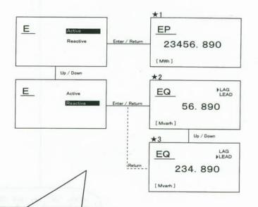
When "Up" key and "Down" key are pressed simultaneously on ★1 marked screen, active energy can be reset. In a similar way, when two keys are pressed on ★2/★3 marked screen, lagging/leading reactive energy can be reset.
