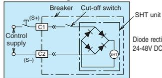
Diode rectifier is not used for control source 24-48V DC.
