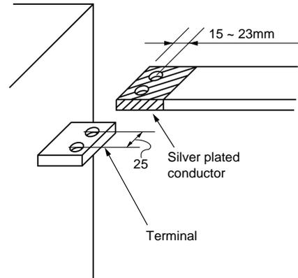
Since fault current flowing through the conductors cause large electromagnetic forces, the conductors should be secured firmly, using the values in Table on the right as a reference. Max busbar supporting distance nearest to ACB is less than 200mm.
