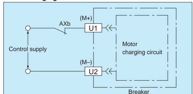
A OFF charging method is also available. The closing spring is charged automatically when the breaker is opened. This is available only by externally connecting in series b contact (AXb) of the auxiliary switch to the motor charging circuit.
