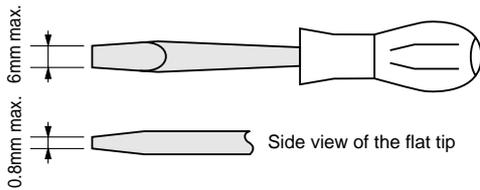
2. Insert the flat-tipped screwdriver into the opening of the electronic trip relay cover. Then, lightly press the screwdriver leftward, and the cover will open.
