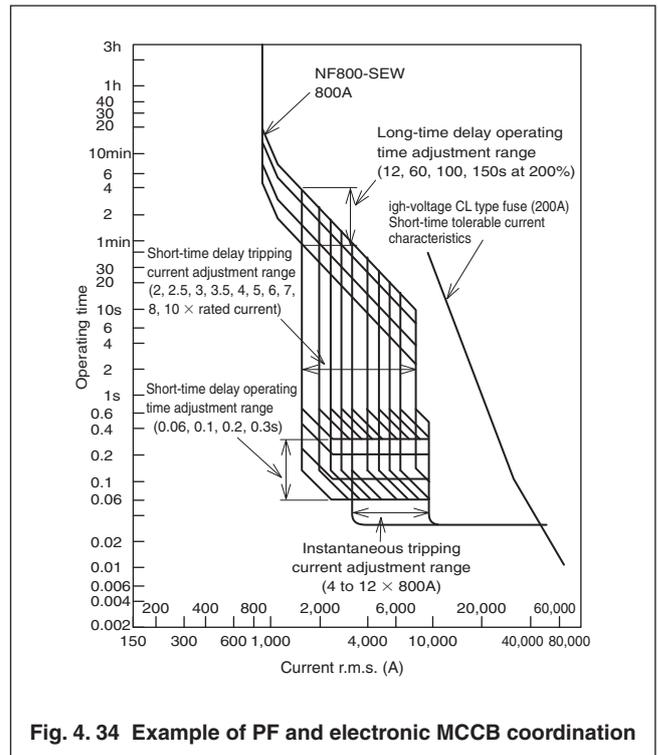
**Fig. 4. 34 Example of PF and electronic MCCB coordination**
