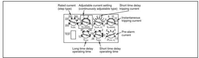
Fig. 2.28 Adjustment module
