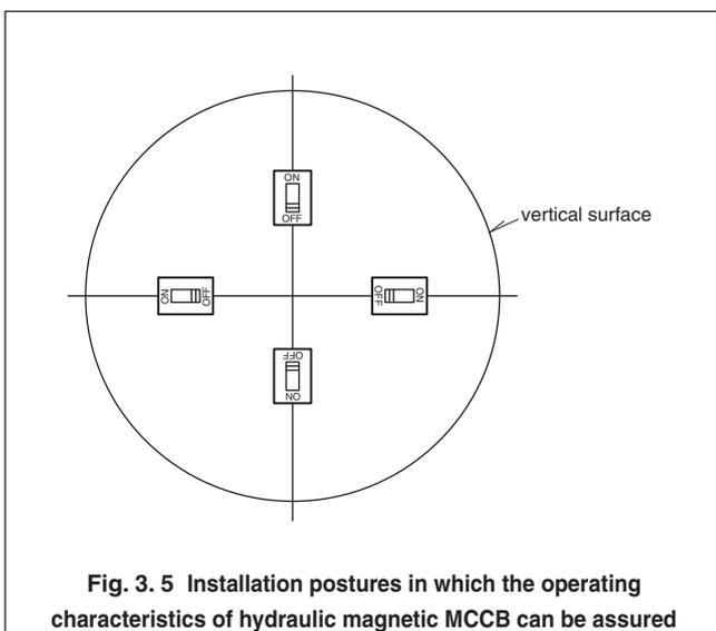
Fig. 3. 5 Installation postures in which the operating characteristics of hydraulic magnetic MCCB can be assured
