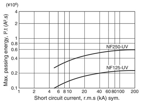
**Fig. 2.24** Passing  $I^2.t$  characteristics of models NF125-UV and NF250-UV
