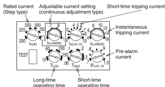
**Fig. 4. 7 Electronic type MCCB characteristics setting section**
