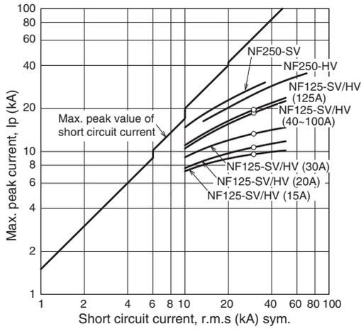
**Fig. 2.19** Passing current peak value characteristics of models NF125-SV/HV and NF250-SV/HV
