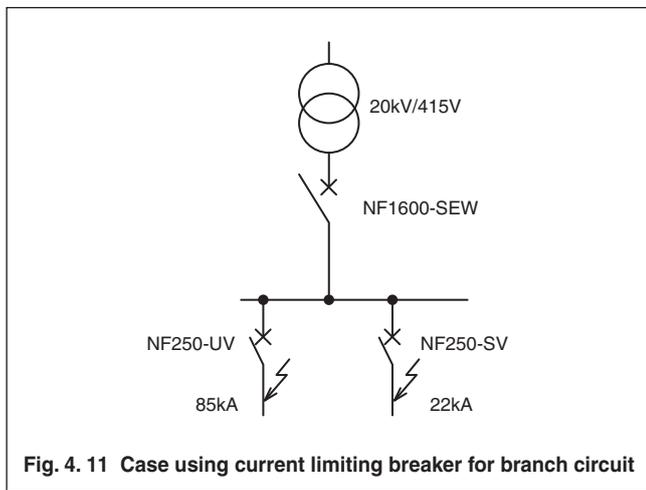
Fig. 4. 11 Case using current limiting breaker for branch circuit
