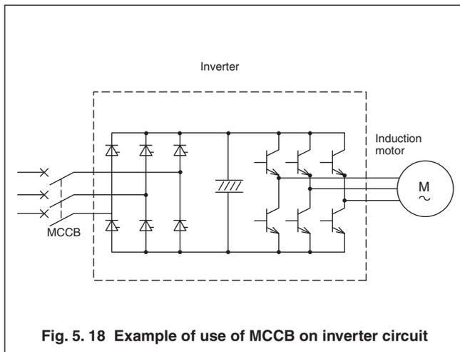
Fig. 5. 18 Example of use of MCCB on inverter circuit
