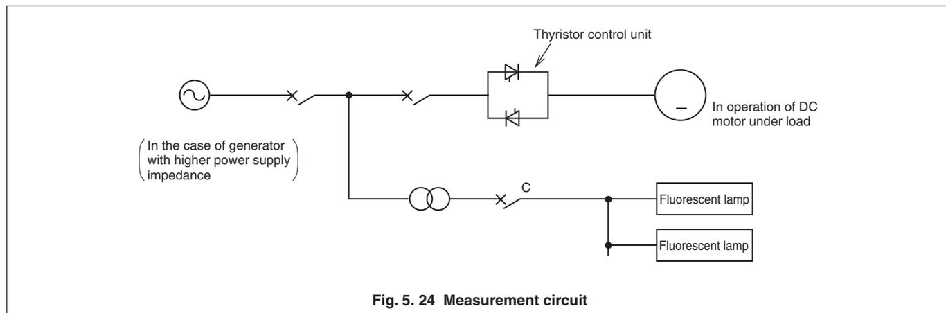
Fig. 5.24 Measurement circuit
