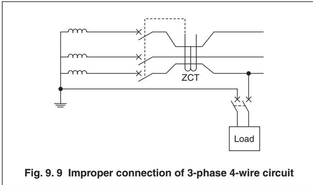
**Fig. 9.9 Improper connection of 3-phase 4-wire circuit**
