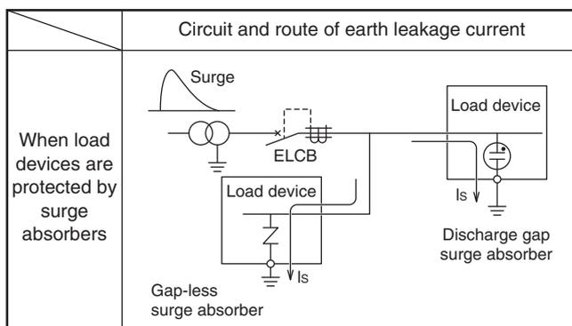
**Fig. 9.21 Transient leakage current caused by surge absorbers**
