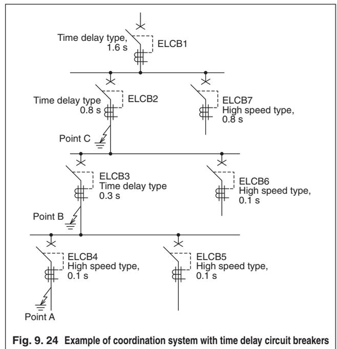
Fig. 9. 24 Example of coordination system with time delay circuit breakers
