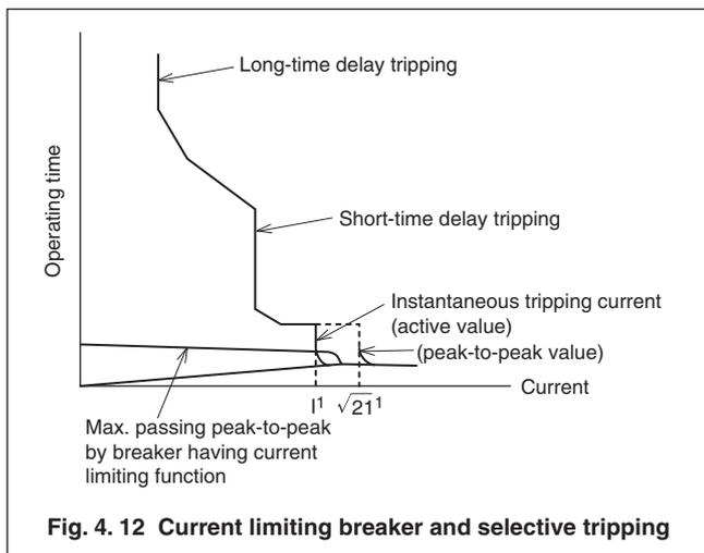
Fig. 4. 12 Current limiting breaker and selective tripping
