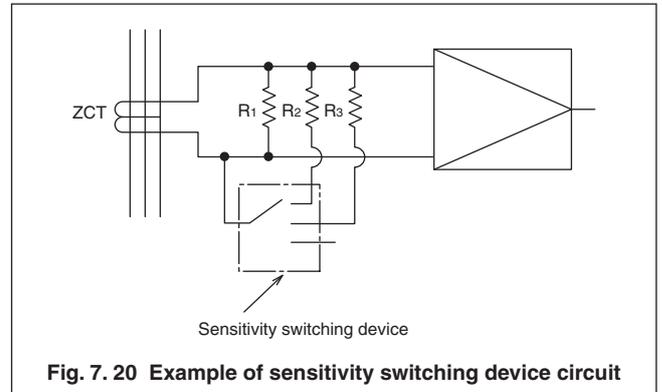
Fig. 7.20 Example of sensitivity switching device circuit
