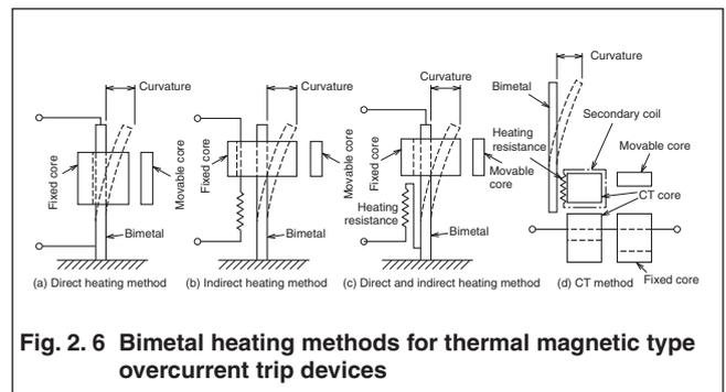
Fig. 2.6 Bimetal heating methods for thermal magnetic type overcurrent trip devices
