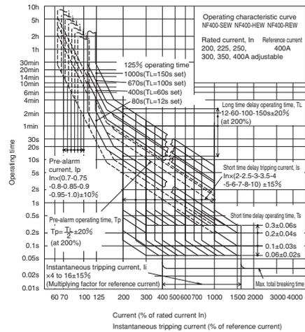
Fig. 2.29 Example of operating characteristic curves
