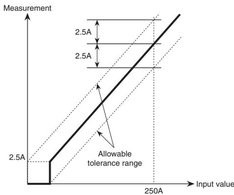
**Fig. 2. 34 Measurement accuracy**
