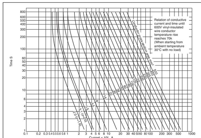
**Fig. 4.16 Current time characteristics for 600V vinyl-insulated wire conductor temperature 100°C to reach rise value 70K**
