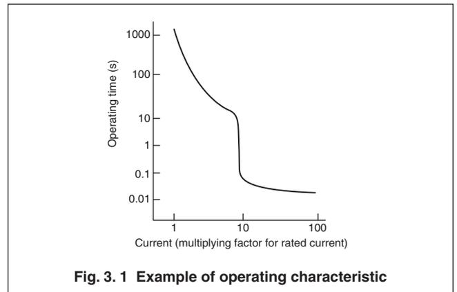
**Fig. 3. 1 Example of operating characteristic**
