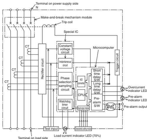
Fig. 2.27 Circuit diagram of electronic overcurrent trip device
