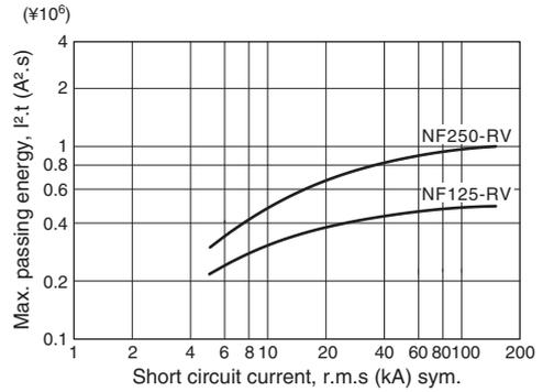
**Fig. 2.22** Passing  $I^2.t$  characteristics of models NF125-RV and NF250-RV
