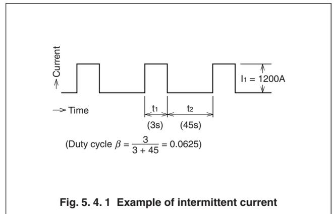
Fig. 5.4.1 Example of intermittent current
