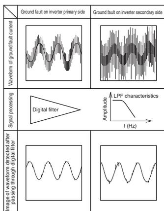
**Fig. 7.12 Effect of digital filter**
