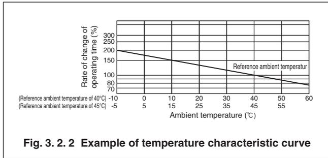
**Fig. 3. 2. 2 Example of temperature characteristic curve**
