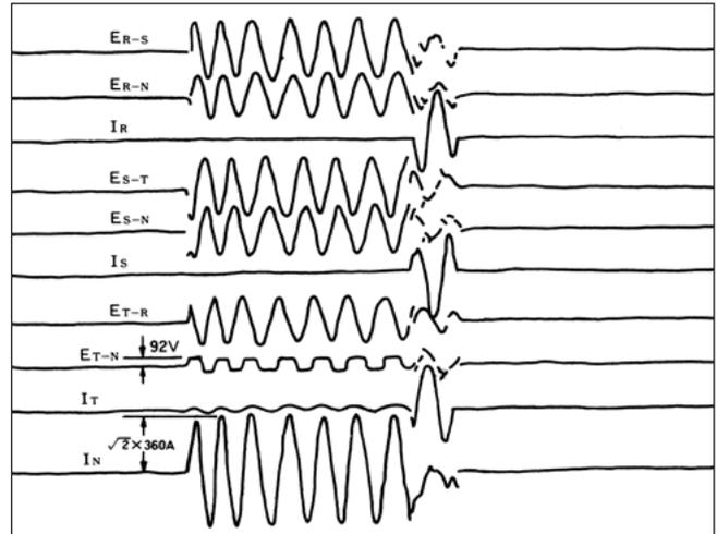
Fig. 9. 22 Example of MCCB breaking for phase to phase arcing short circuit caused by arc ground fault
