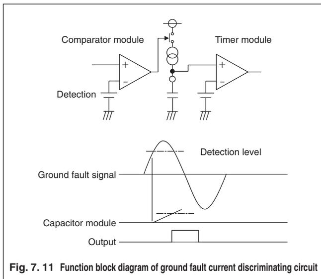
**Fig. 7.11 Function block diagram of ground fault current discriminating circuit**
