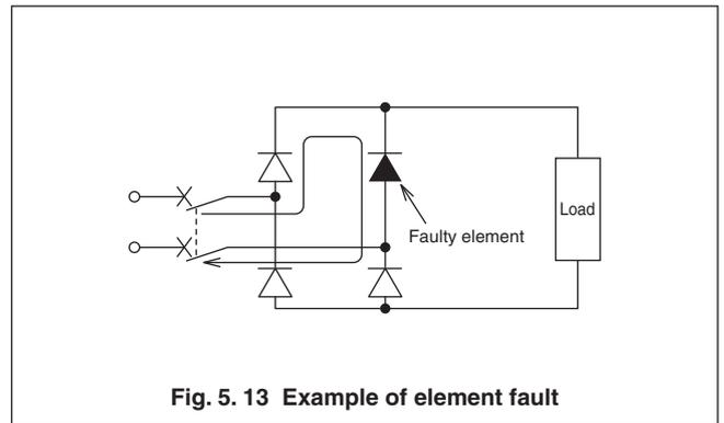
Fig. 5.13 Example of element fault
