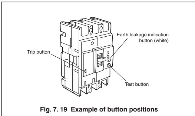
Fig. 7.19 Example of button positions
