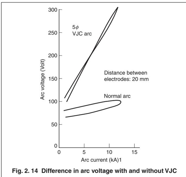
Fig. 2. 14 Difference in arc voltage with and without VJC
