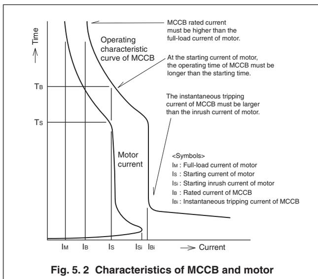
**Fig. 5. 2 Characteristics of MCCB and motor**
