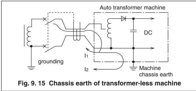
Fig. 9.15 Chassis earth of transformer-less machine
