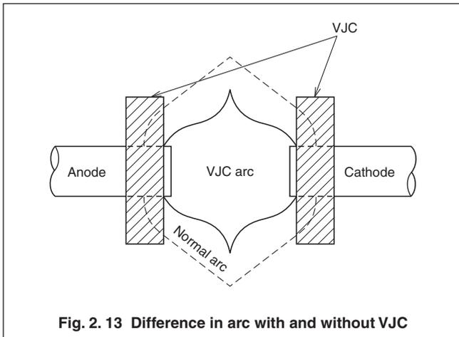
Fig. 2. 13 Difference in arc with and without VJC
