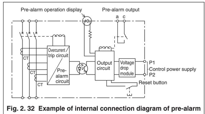
**Fig. 2.32 Example of internal connection diagram of pre-alarm**
