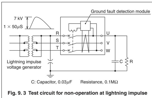
**Fig. 9. 3 Test circuit for non-operation at lightning impulse**
