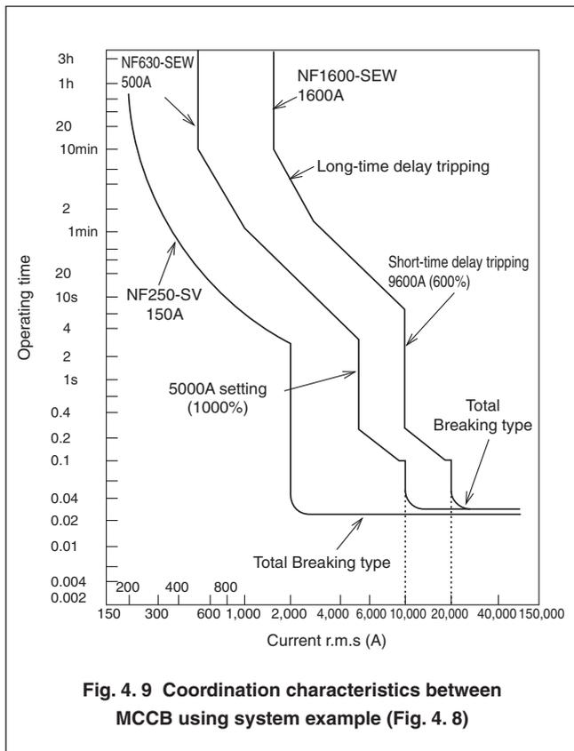
**Fig. 4. 9 Coordination characteristics between MCCB using system example (Fig. 4. 8)**
