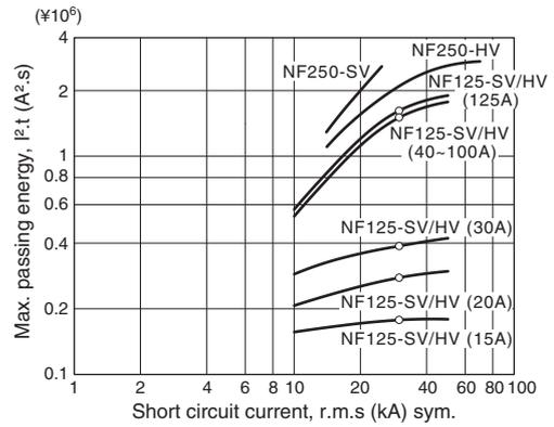
**Fig. 2.20** Passing  $I^2.t$  characteristics of models NF125-SV/HV and NF250-SV/HV
