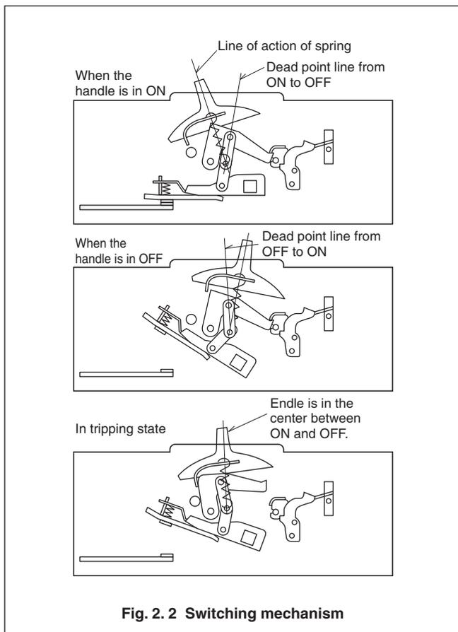
**Fig. 2.2 Switching mechanism**
