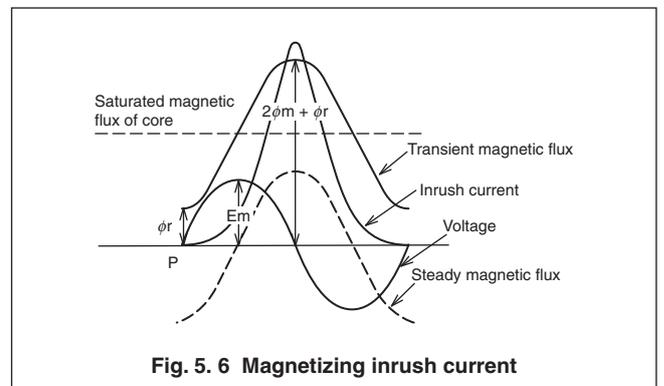
**Fig. 5. 6 Magnetizing inrush current**
