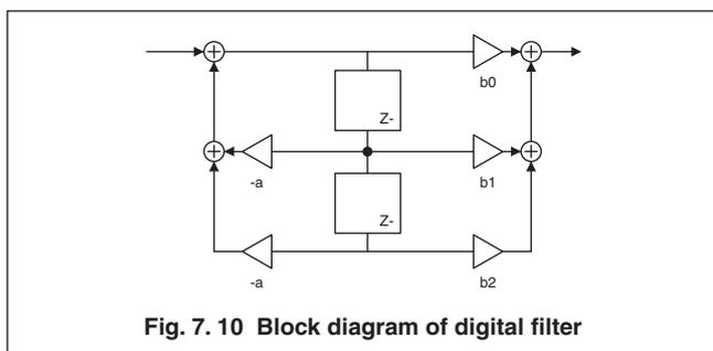
**Fig. 7.10 Block diagram of digital filter**
