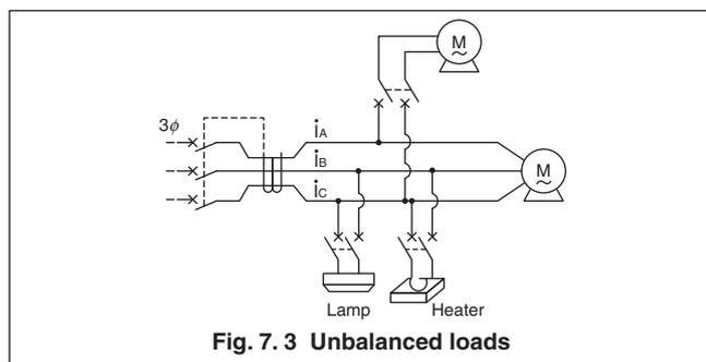
Fig. 7.3 Unbalanced loads
