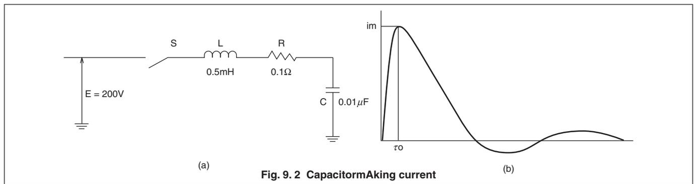
**Fig. 9.2 CapacitormAking current**
