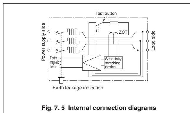
Fig. 7.5 Internal connection diagrams
