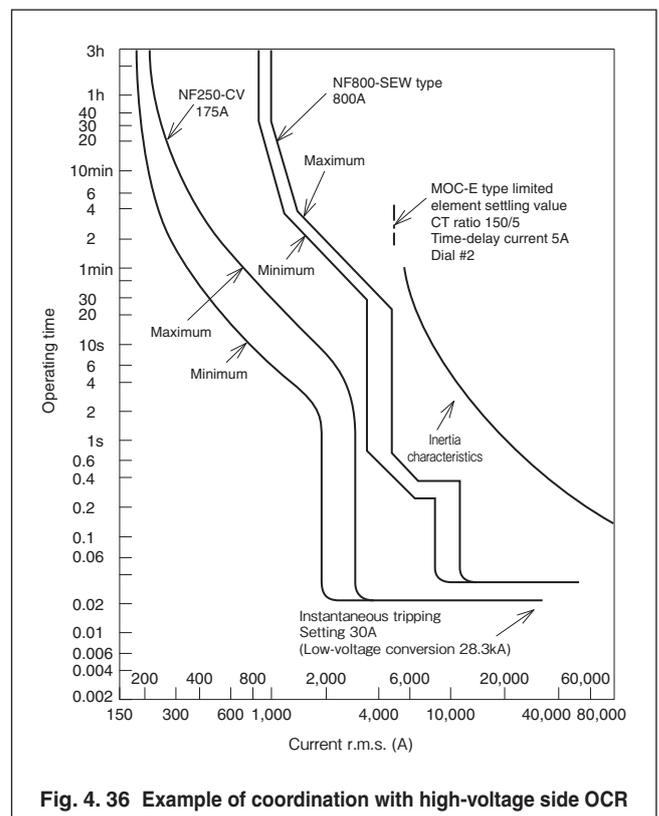
Fig. 4.36 Example of coordination with high-voltage side OCR
