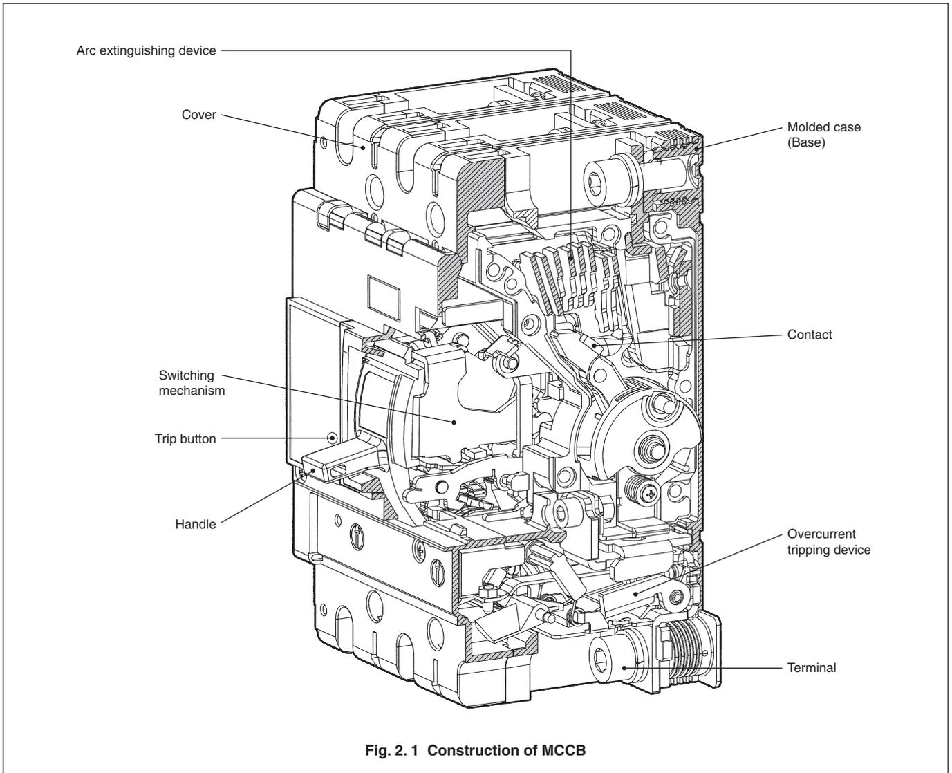
Fig. 2. 1 Construction of MCCB
