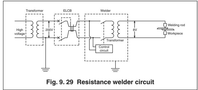
Fig. 9. 29 Resistance welder circuit
