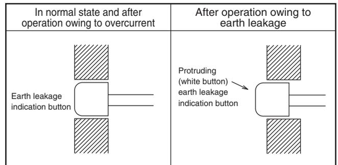
Fig. 7.18 Indication with earth leakage indication button
