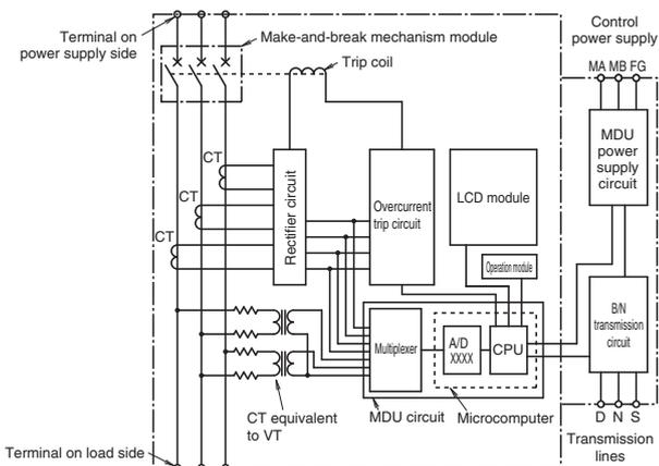
Fig. 2. 33 MDU block diagram
