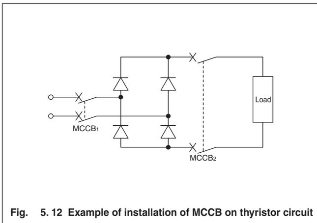
Fig. 5.12 Example of installation of MCCB on thyristor circuit
