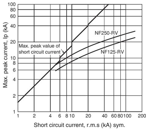
**Fig. 2.21** Passing current peak value characteristics of models NF125-RV and NF250-RV
