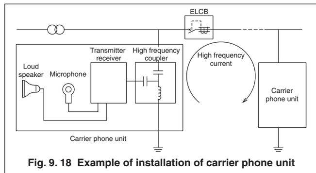
**Fig. 9.18 Example of installation of carrier phone unit**
