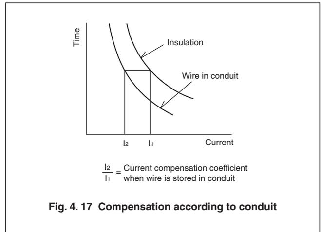
**Fig. 4.17 Compensation according to conduit**
