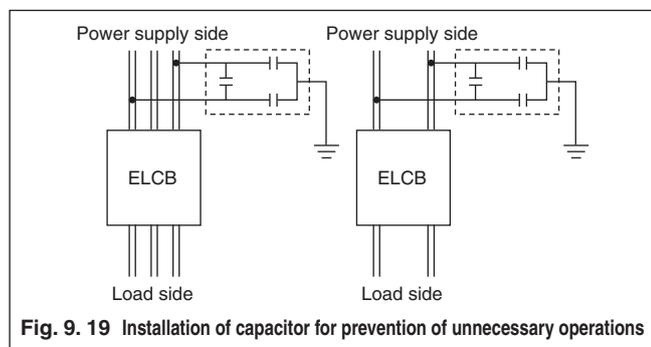
**Fig. 9.19 Installation of capacitor for prevention of unnecessary operations**
