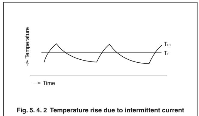
Fig. 5.4.2 Temperature rise due to intermittent current
