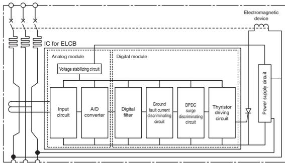
**Fig. 7.9 Structure of electronic circuit**
