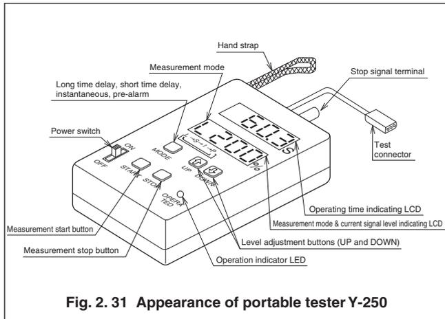
**Fig. 2.31 Appearance of portable tester Y-250**
