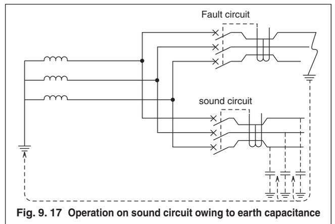
Fig. 9.17 Operation on sound circuit owing to earth capacitance
