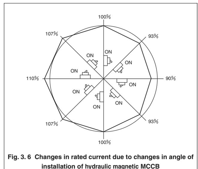
Fig. 3. 6 Changes in rated current due to changes in angle of installation of hydraulic magnetic MCCB
