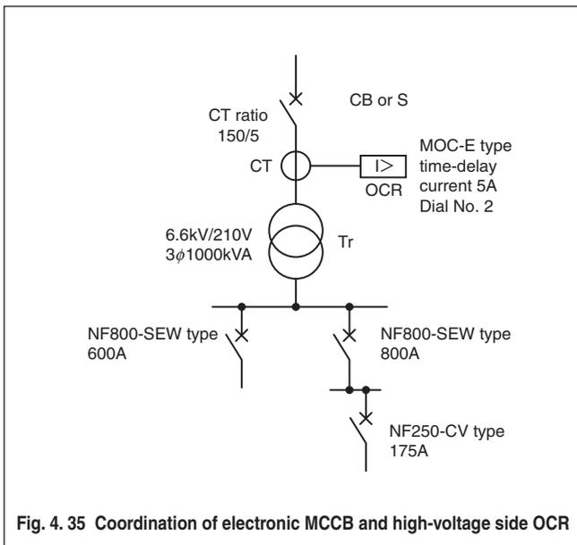
Fig. 4.35 Coordination of electronic MCCB and high-voltage side OCR
