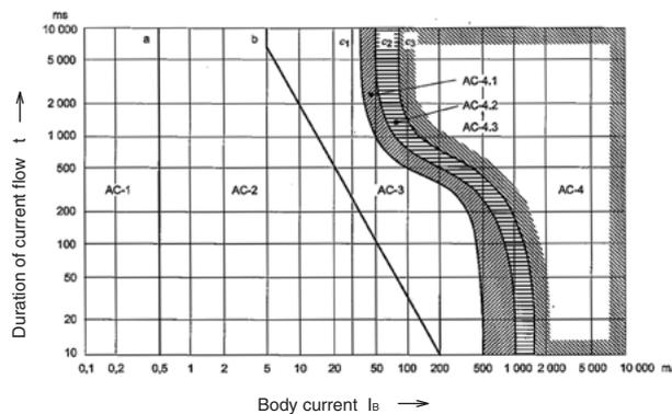
Fig. 6. 5 Effect of AC current (15Hz to 100Hz) on human body (IEC/TS60479-1)
