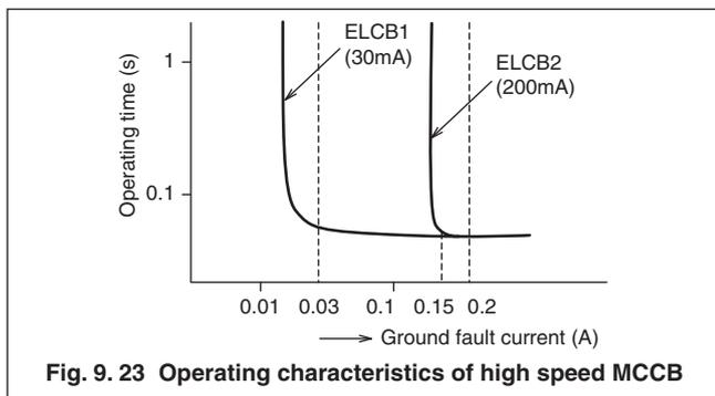
Fig. 9. 23 Operating characteristics of high speed MCCB
