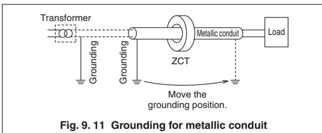
**Fig. 9.11 Grounding for metallic conduit**
