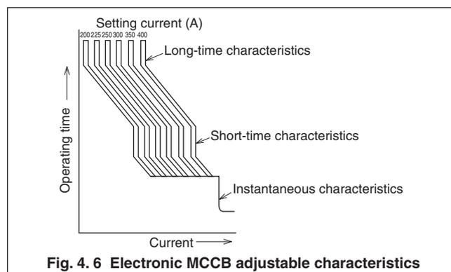
**Fig. 4. 6 Electronic MCCB adjustable characteristics**
