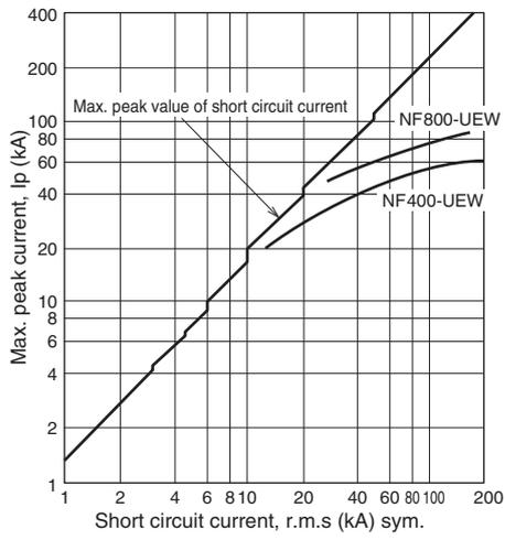
**Fig. 2.25** Passing current peak value characteristics of models NF400-UEW and NF800-UEW
