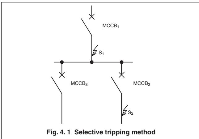
Fig. 4. 1 Selective tripping method
