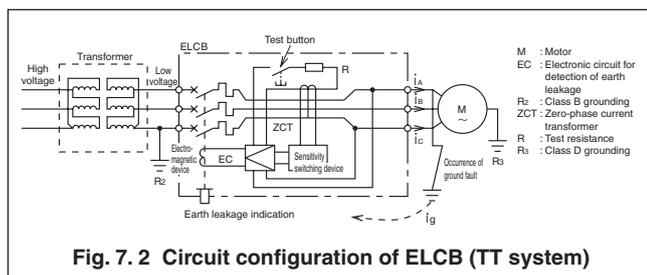
Fig. 7.2 Circuit configuration of ELCB (TT system)
