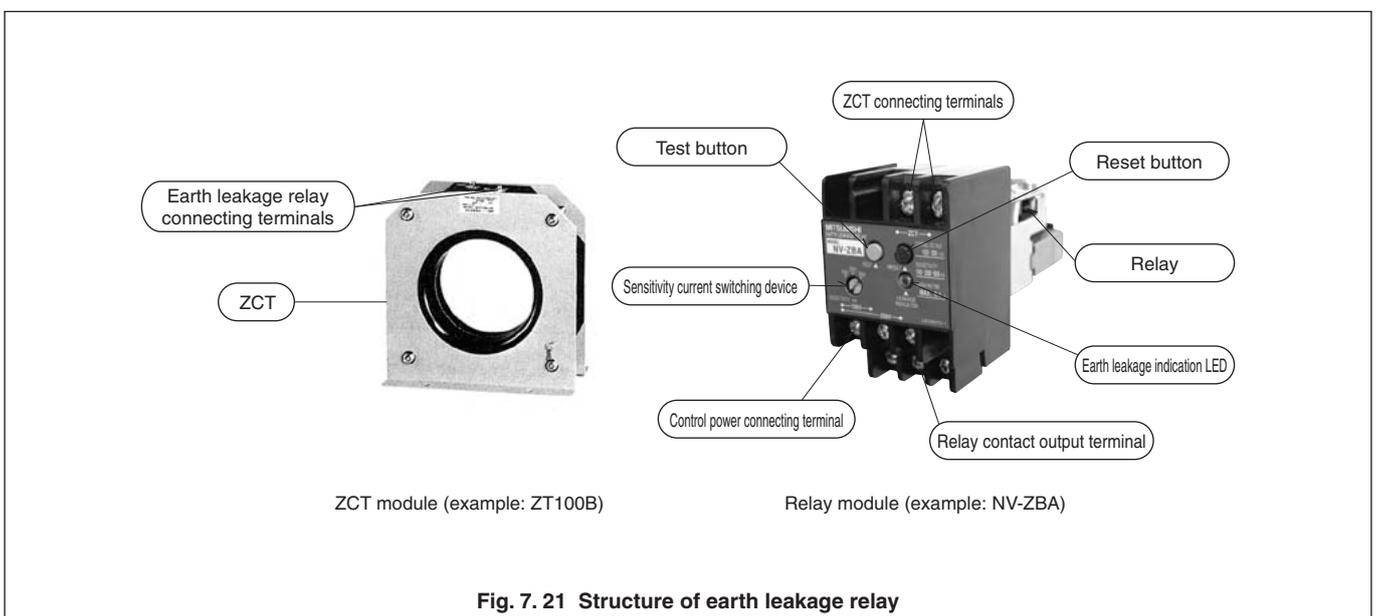
Fig. 7.21 Structure of earth leakage relay
