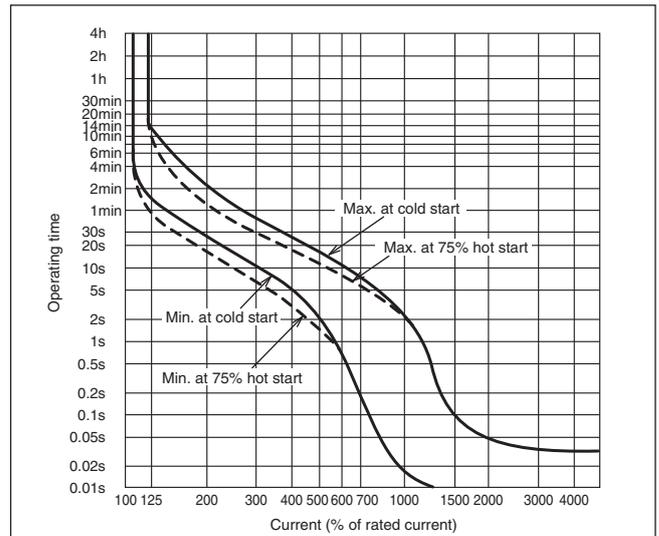
**Fig. 3. 3 Examples of hot start operating characteristic curves**
