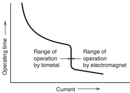
**Fig. 2.7. b Operating time-current characteristics**
