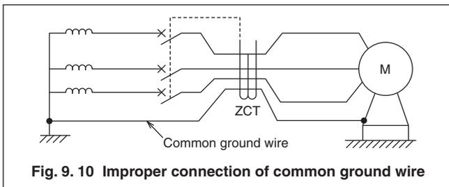
**Fig. 9.10 Improper connection of common ground wire**
