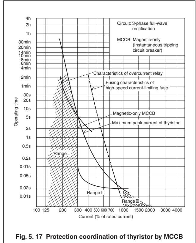
Fig. 5. 17 Protection coordination of thyristor by MCCB
