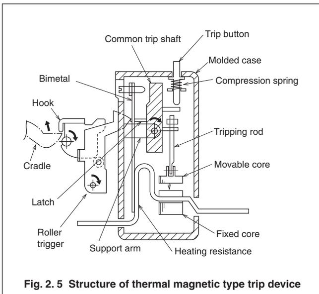
Fig. 2.5 Structure of thermal magnetic type trip device
