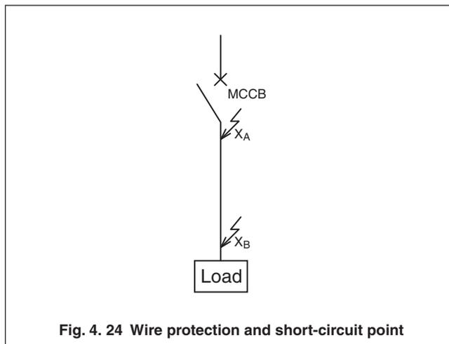
Fig. 4. 24 Wire protection and short-circuit point
