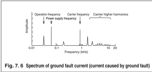
Fig. 7. 6 Spectrum of ground fault current (current caused by ground fault)
