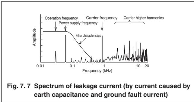
Fig. 7. 7 Spectrum of leakage current (by current caused by earth capacitance and ground fault current)
