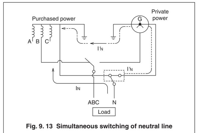
**Fig. 9.13 Simultaneous switching of neutral line**
