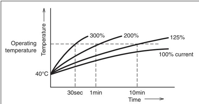
**Fig. 2.7. a Bimetal temperature-time characteristics**
