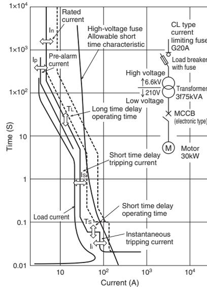
Fig. 2.30 Overload protection coordination diagram
