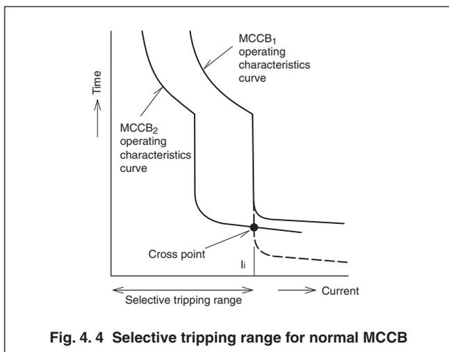
**Fig. 4. 4 Selective tripping range for normal MCCB**
