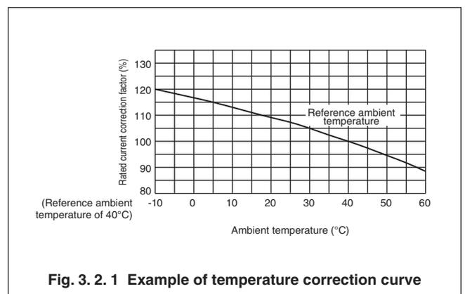
**Fig. 3. 2. 1 Example of temperature correction curve**
