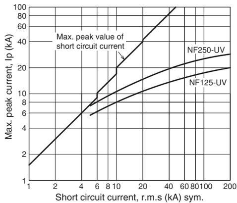
**Fig. 2.23** Passing current peak value characteristics of models NF125-UV and NF250-UV
