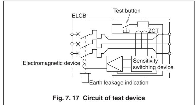
Fig. 7.17 Circuit of test device
