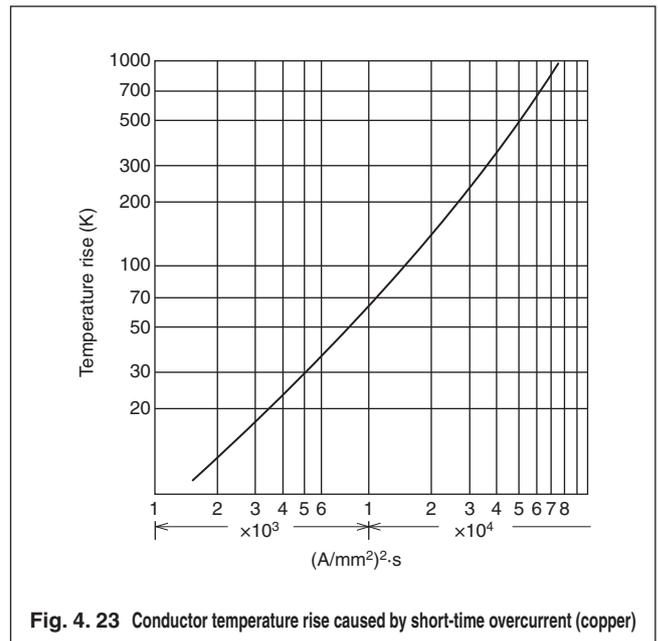
Fig. 4. 23 Conductor temperature rise caused by short-time overcurrent (copper)
