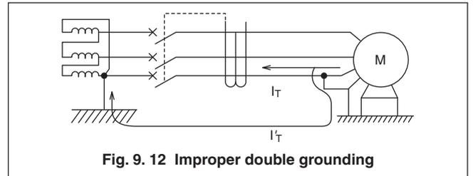
**Fig. 9.12 Improper double grounding**
