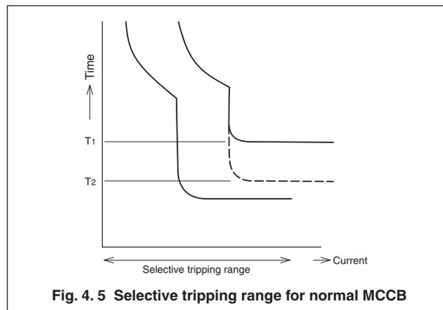
**Fig. 4. 5 Selective tripping range for normal MCCB**
