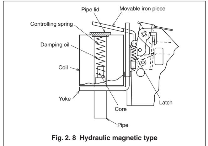
**Fig. 2.8 Hydraulic magnetic type**
