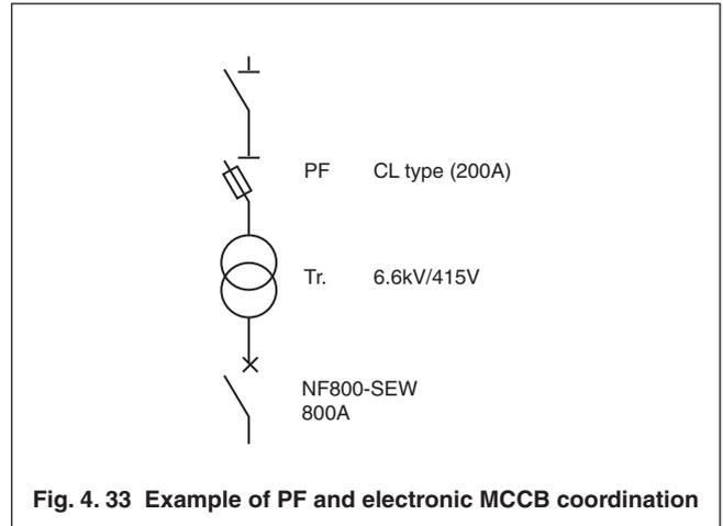
**Fig. 4. 33 Example of PF and electronic MCCB coordination**
