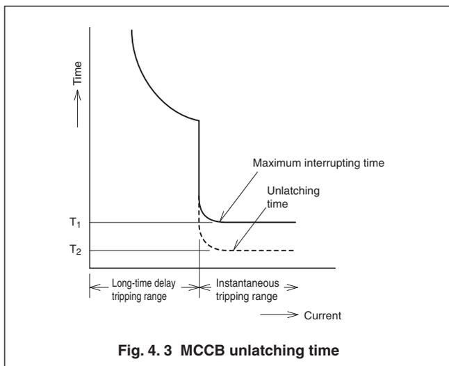
**Fig. 4. 3 MCCB unlatching time**
