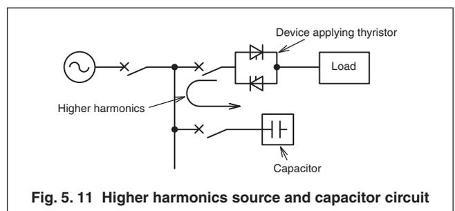
**Fig. 5. 11 Higher harmonics source and capacitor circuit**
