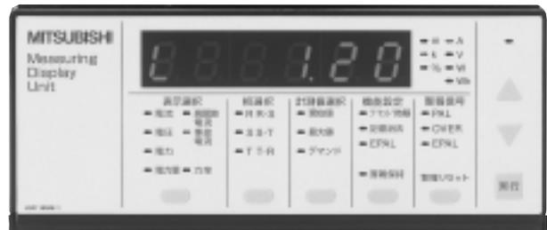
**Example of NV630-SEPM long-delay tripping display**
