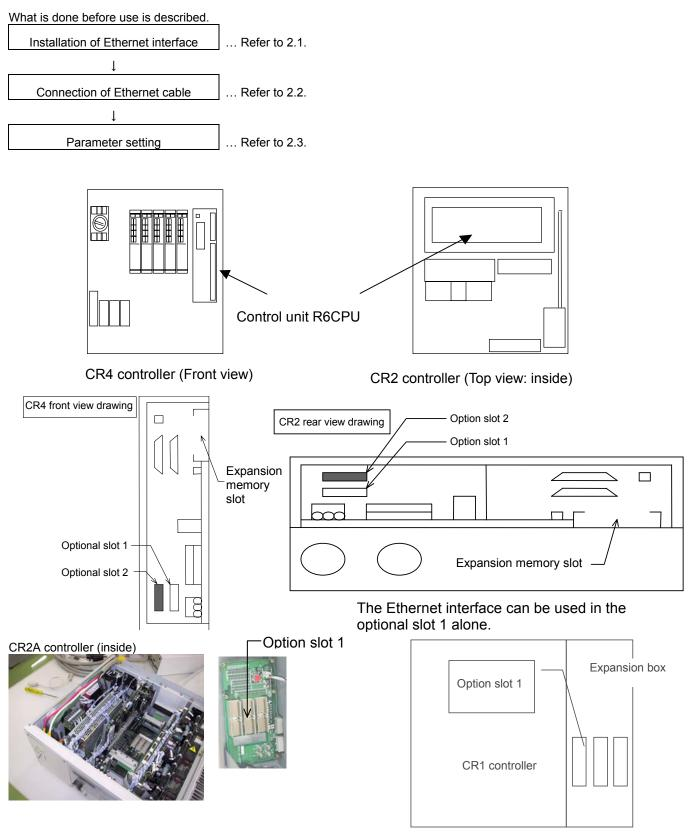
Install the CR1 controller in the expansion option box. Refer to the separate manual "Controller setup, basic operation, and maintenance" for detail.
