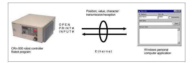
The data link function of the Ethernet interface has the two kinds shown below.
