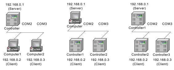
Two or more clients are not connectable with the one line number COMn. Change the line number, when using the robot controller as the server and connecting two or more clients.
