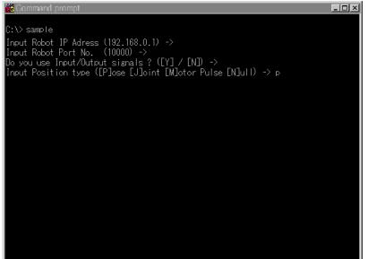
If communication cannot be carried out correctly, refer to section "2.4 Checking the connection", and check the connection cable or restart the controller and sample.exe.
