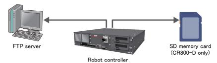
Robot information at error occurrence can be saved in the FTP server or SD memory card (CR800-D only). The following four types of robot information can be saved.
