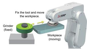
Fig.7-115:Example of polishing
