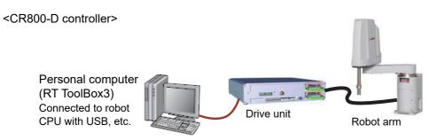
Fig.5-13:Connecting the devices (CR800-D controller)
