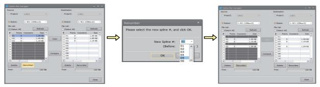
Fig.7-74: Change the spline No.
