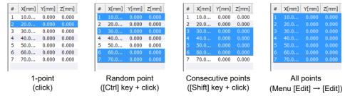
Fig.7-48:Selecting the path point data
