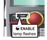
The status display lamp "ENABLE" on the front of the T/B blinks.
