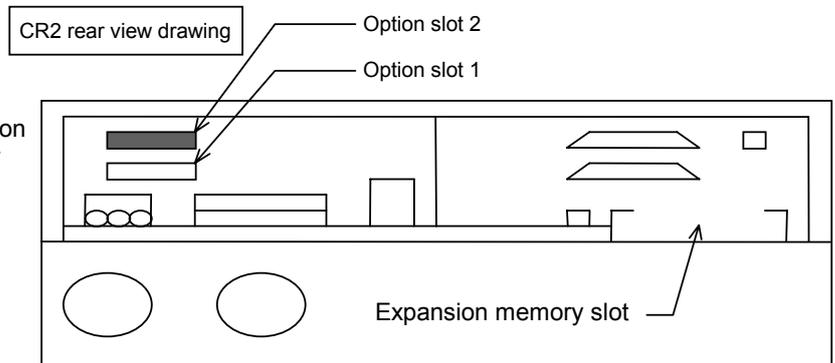
The Ethernet interface can be used in the optional slot 1 alone.
