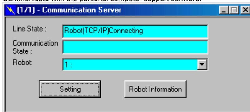
Communication can be carried out with the Ethernet interface TCP/IP in the same manner as RS-232-C communication.
