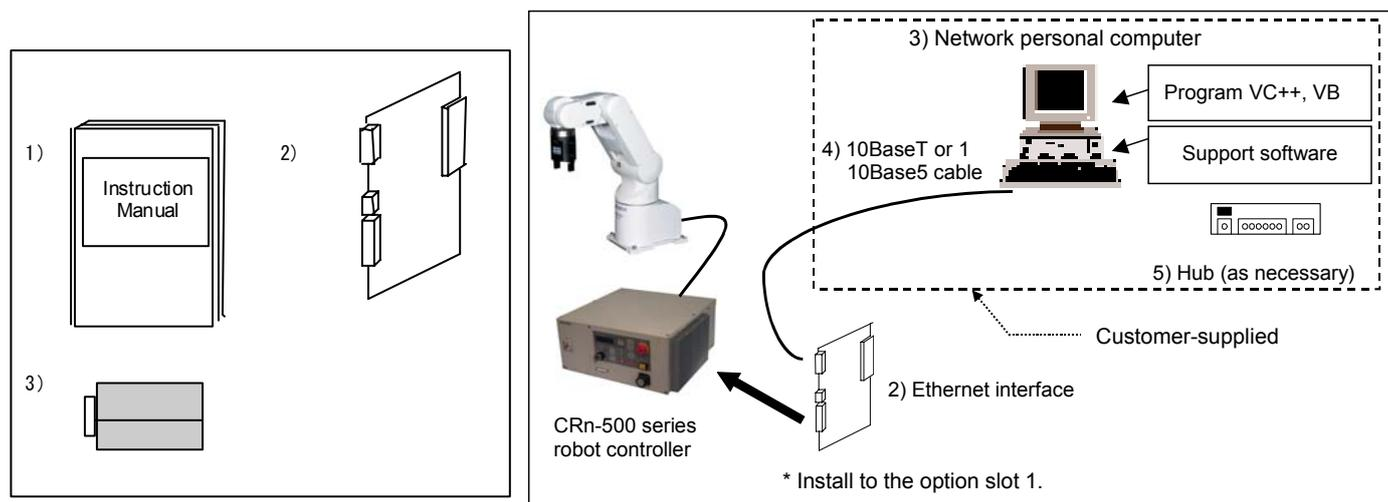
In addition to the standard robot system configuration, the following is necessary. These devices are separately procured by the customer.
