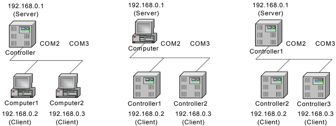
Two or more clients are not connectable with the one line number COMn. Change the line number, when using the robot controller as the server and connecting two or more clients.
