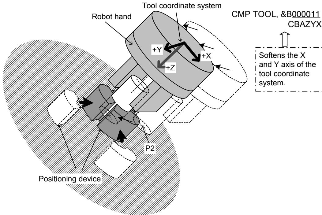
Fig.4-17:The example of using the compliance mode
