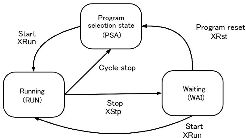
Fig.4-4: Operation state of each slot
