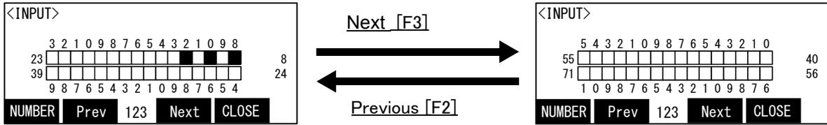
Press the function key corresponding to "Next", then display the next input signal screen. Press the function key corresponding to "Prev", then display the previous input screen
