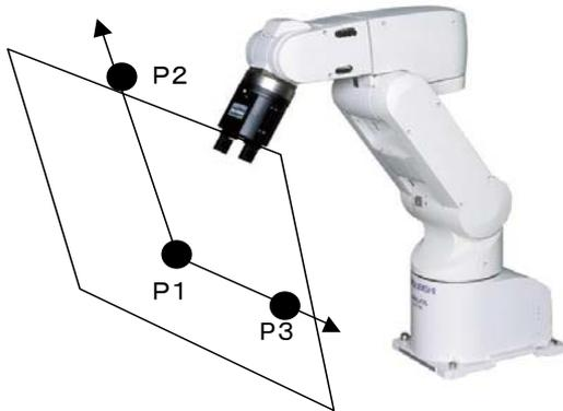
As can be seen in the diagram to the left, any plane can be defined by three points (P1, P2, and P3), after which an evaluation of which side of the plane it is in (the side that includes the robot origin or the other side) can be performed. This function can be used to prevent collision with the floor or interference with peripheral devices. Maximum of eight planes can be monitored. There is no limit to the plane.
