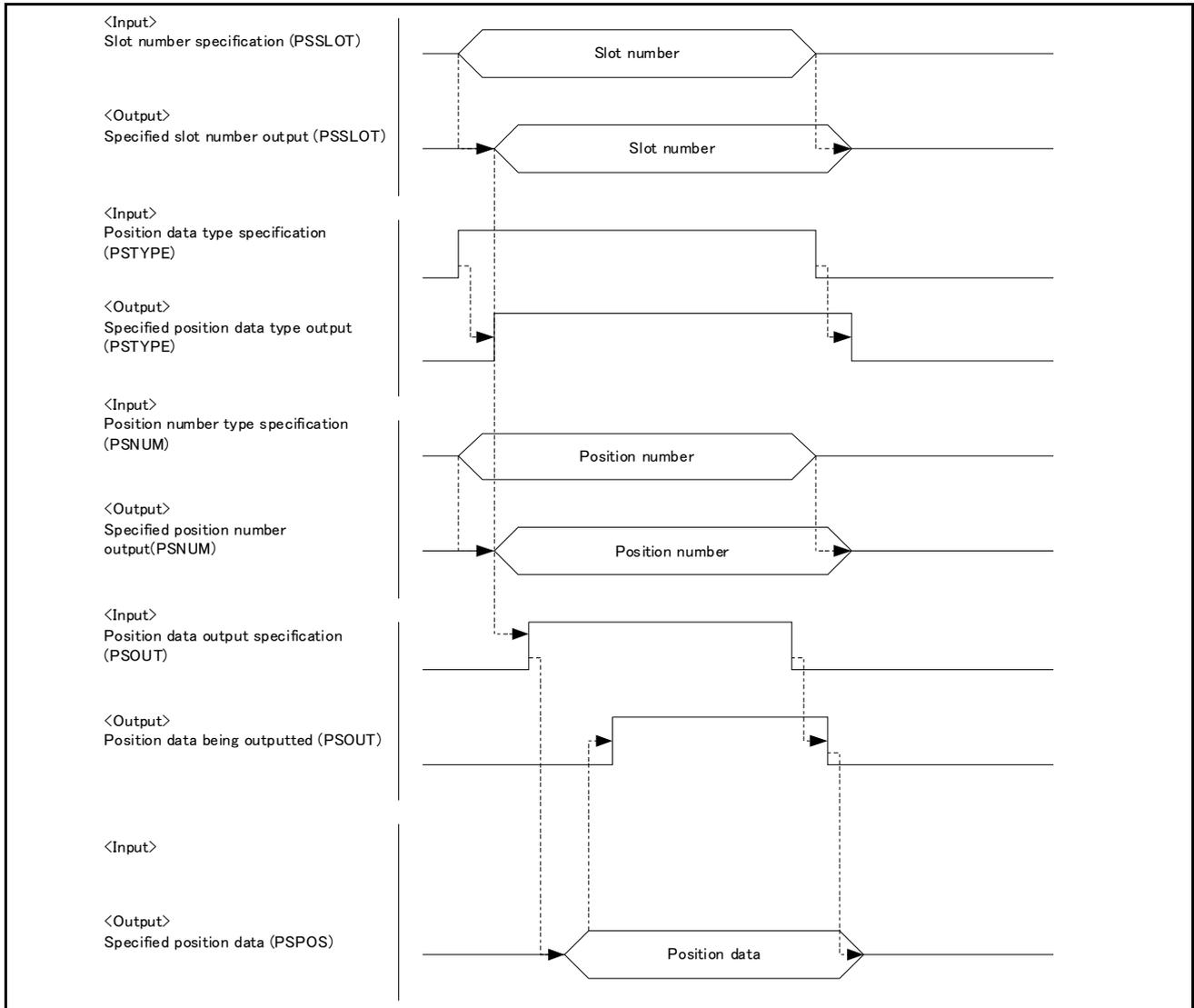
Fig.6-6:Example of external operation timing chart (Part 5)
