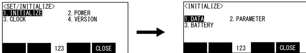
2) Press the [2] key in the initial menu screen, and select the parameter. Display the screen of confirmation.
