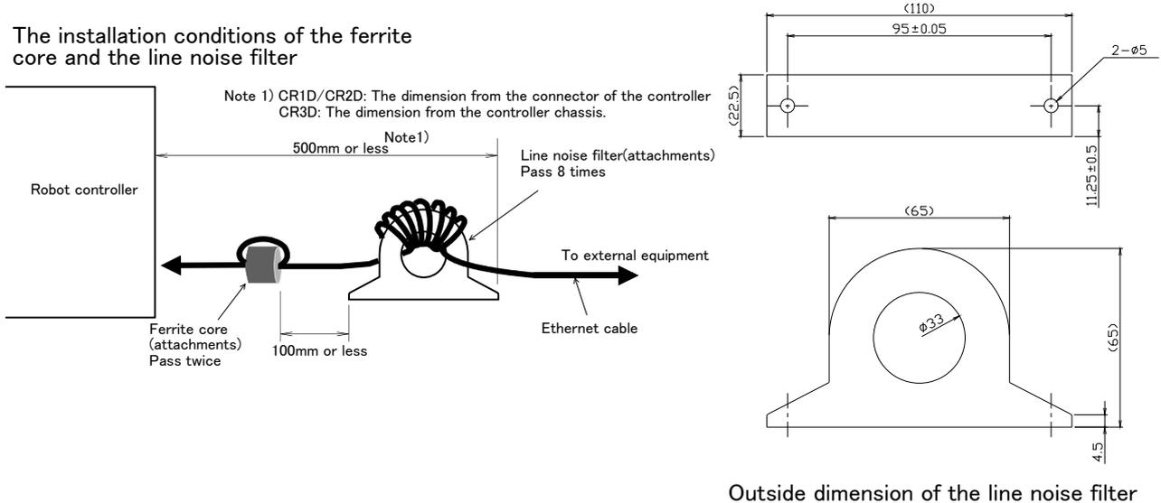
Fig.5-4 : Installation to the Ethernet cable of ferrite core and filter (CE Marking)
