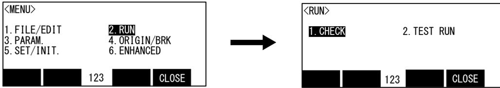
2) Press the [2] key, and display the test operation screen.
