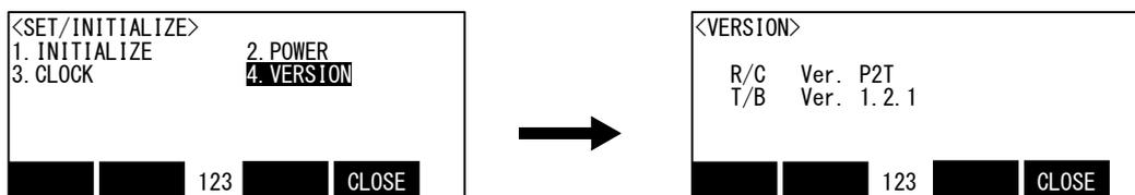
2) Press the function key corresponding to "Close", and return to the set/initial screen.
