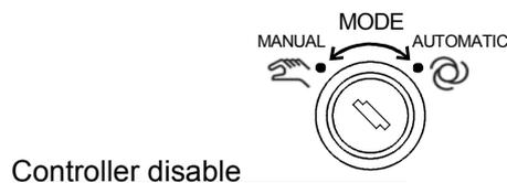
1) Set the [Mode selection switch] on the front of the controller to "MANUAL".
