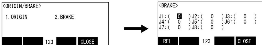
3) Input "1" into the axis which release the brake.
