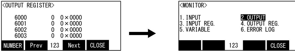
7) Press the function key corresponding to "Close", and return to the monitor menu screen.
