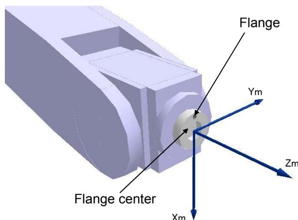
Fig.4-8:Mechanical interface coordinate system
