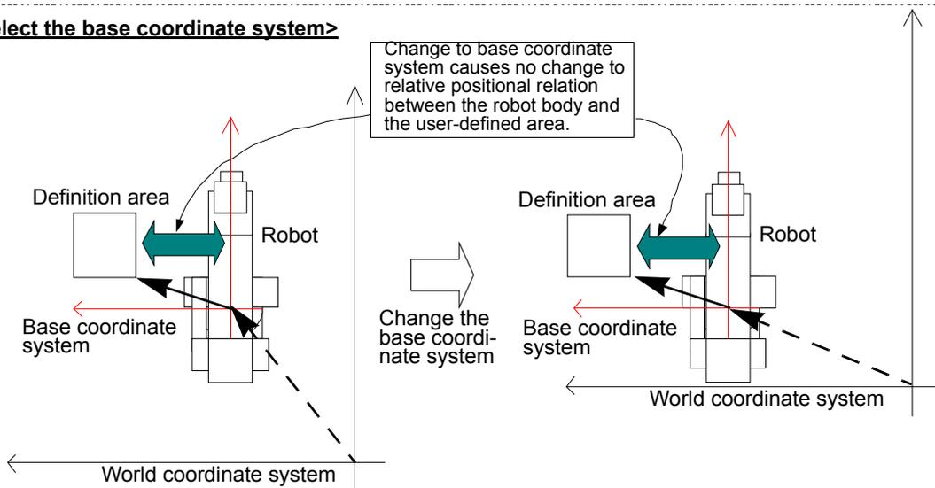
Fig.5-3:Difference between "Worle coordinate system" and "Base coordinate system"
