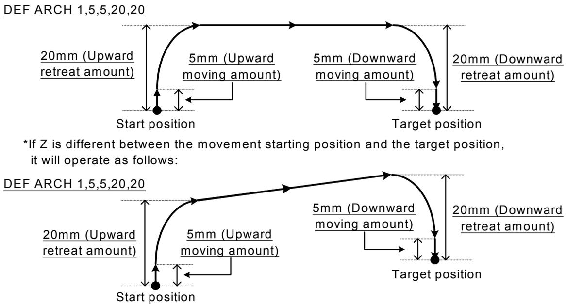
Fig.4-22:Example of arch interpolation motion path (seen from the side)
