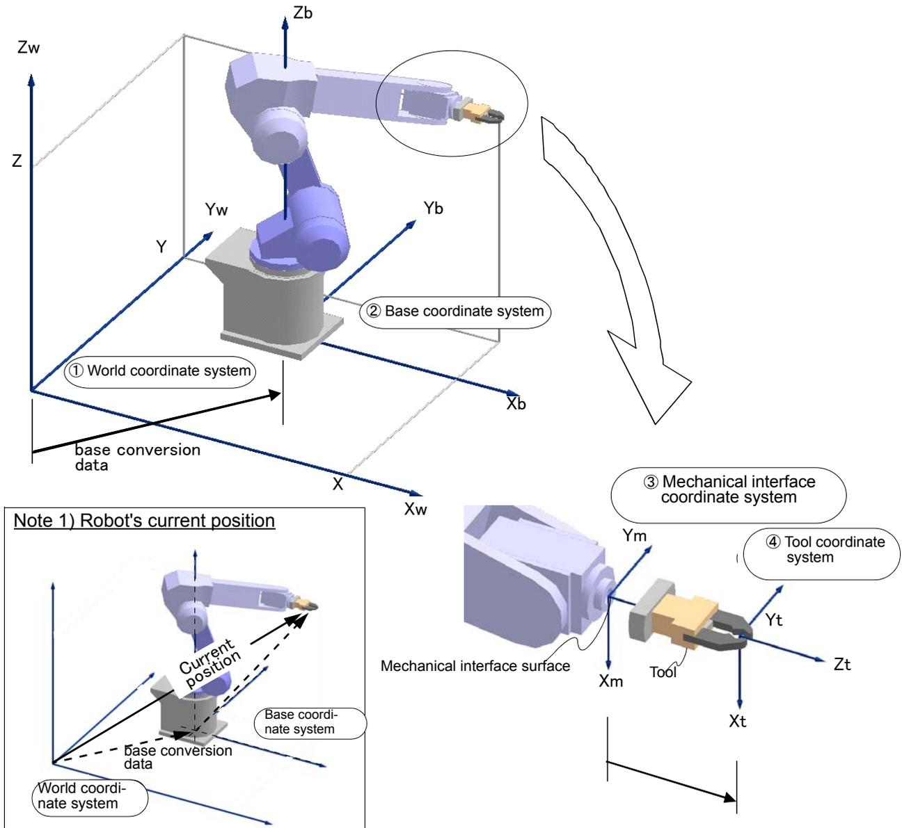
Fig.4-5:Robot's coordinate system
