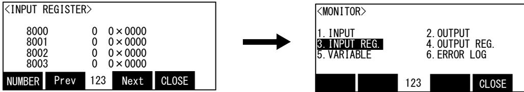
6) Press the function key corresponding to "Close" in monitor menu screen is pressed, finish the monitor, and return to the original screen.
