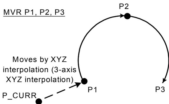
Fig.4-24:Example of circular interpolation motion path 1
