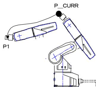
Fig.4-21: Example of joint interpolation motion path
