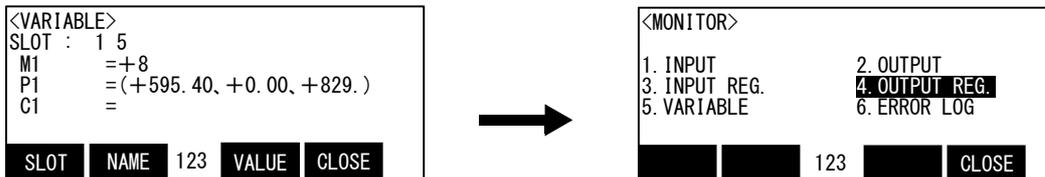
7) Press the function key corresponding to "Close" in monitor menu screen is pressed, finish the monitor, and return to the original screen.
