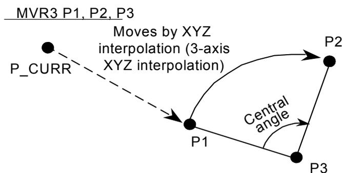
Fig.4-26:Example of circular interpolation motion path 3
