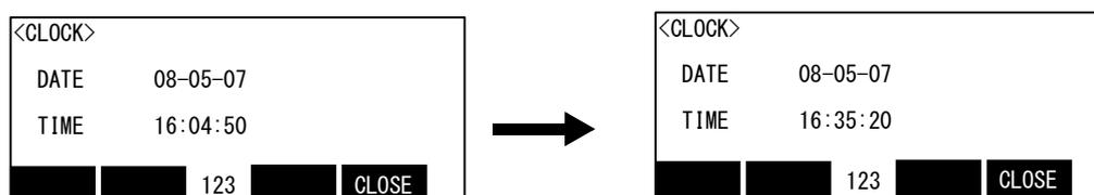
3) Press the function key corresponding to "Close", and return to the set/initial screen.
