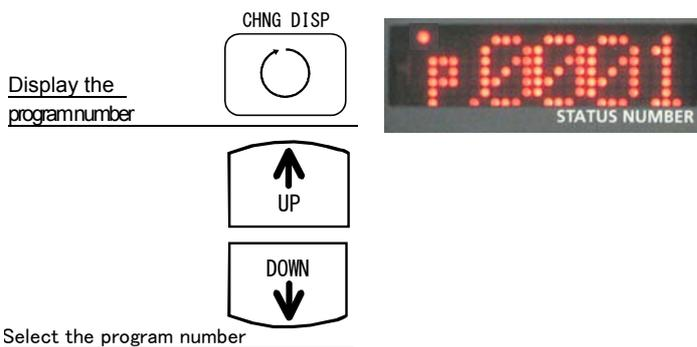
When the [UP] switch is pressed, the registered program Nos. will scroll up, and then the [DOWN] switch is pressed, the program Nos. will scroll down.
