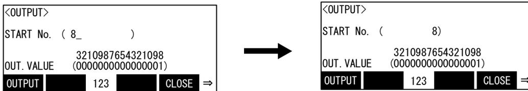
5) Press the function key corresponding to "Close", and return to the output monitor screen.
