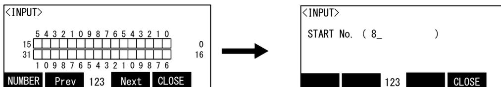
3) Display the ON/OFF state of the 32 points at the head for the input signal No. 8. Black painting indicates ON and white indicates OFF.
