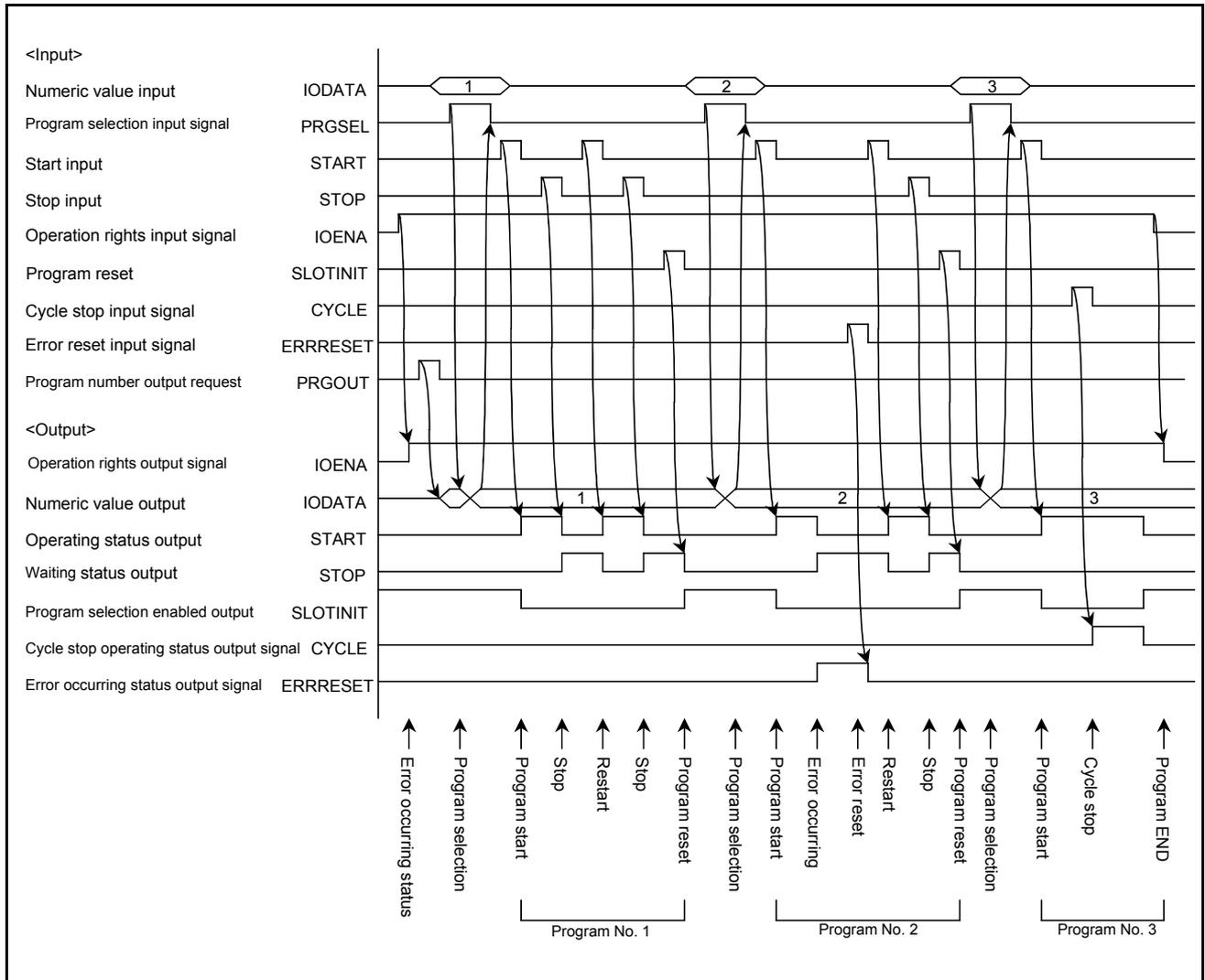
Fig.6-2:Example of external operation timing chart (Part 1)
