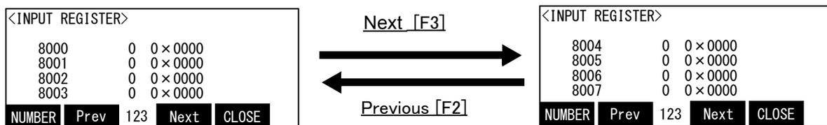
Press the function key corresponding to "Next", then display the next input register screen. Press the function key corresponding to "Prev", then display the previous input register screen.
