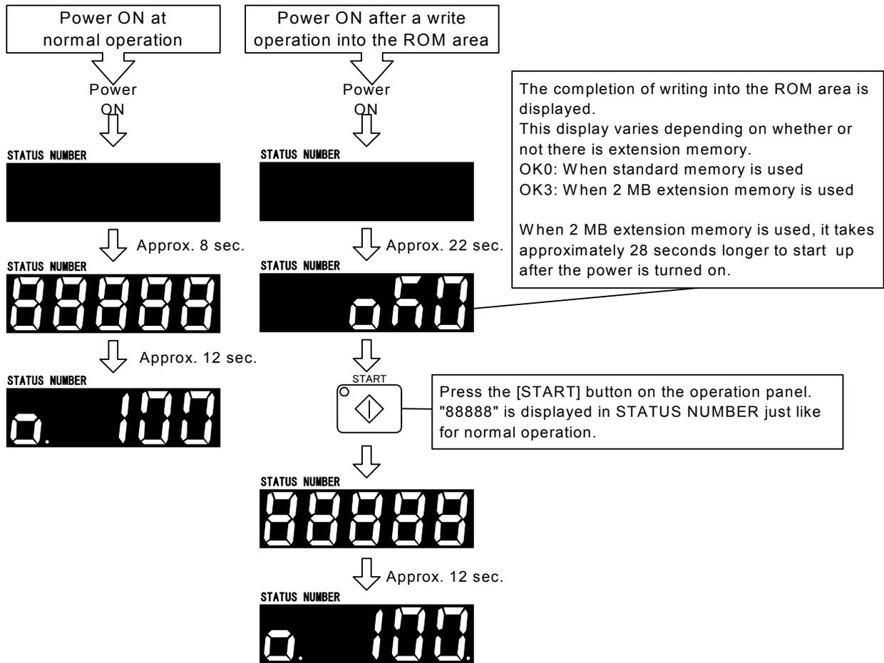
**Caution** If switching from the RAM operation to the ROM operation is performed without copying any program into the ROM area, there would be no program to execute, or a program in which the corrected content has not been reflected would be executed. Therefore, be sure to perform the program copy operation described above.
