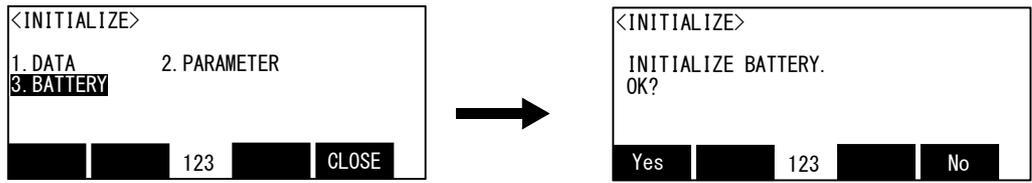
3) If it initializes, press the function key corresponding to "Yes". If it does not initialize, press the function key corresponding to "no".
