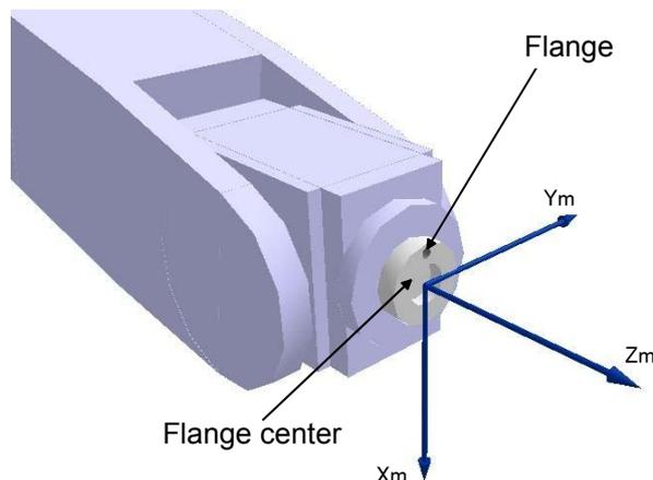
Fig.4-8:Mechanical interface coordinate system
