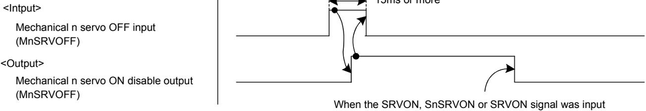
(26) MnSRVON (Mechanical n servo ON input/output during mechanical n servo ON)
