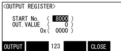
If the function key which corresponds for "Close" is pressed, it can also return to the monitoring screen on the basis of No. 8000 of the output register, but the output value can be changed on the current screen. The case where the value of the output register No. 8000 is set as 12 (decimal number) is shown in the following.
