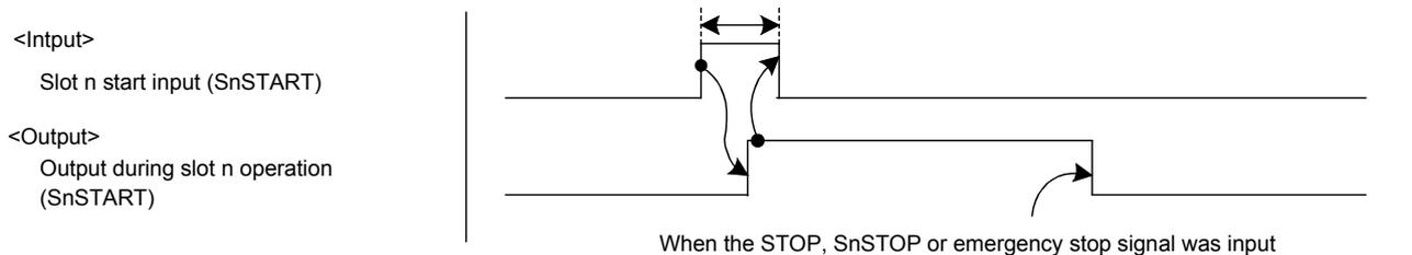
(24) SnSTOP (Slot n stop input/output during slot n aborting)
