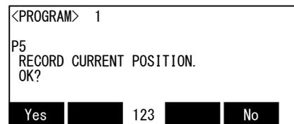
3) Press the function key corresponding to "Yes", then the robot's current position data will be taught to P5, and display will return to the original command edit screen. The teaching can be canceled if the function key corresponding to "No" is pressed.
