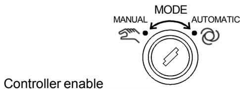
2) Set the controller [MODE] switch to "AUTOMATIC".
