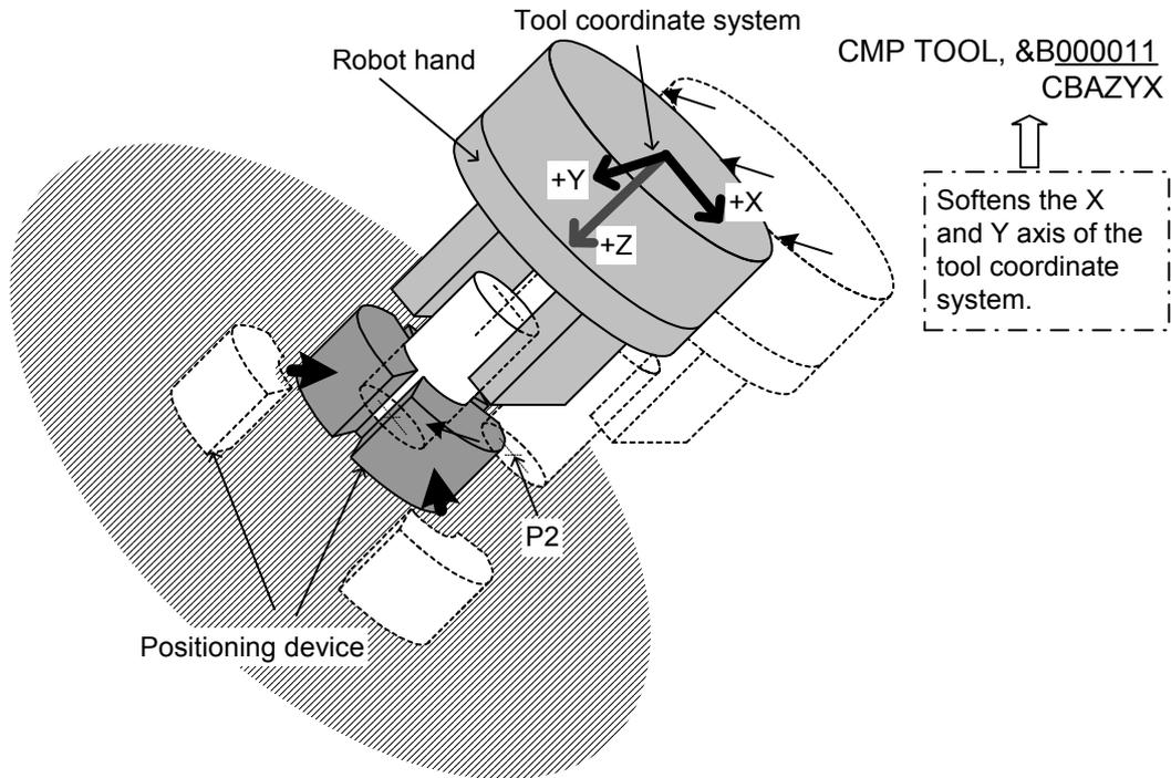
Fig.4-17: The example of using the compliance mode
