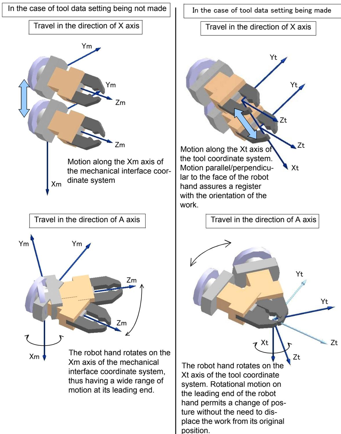
Fig.4-11: Tool jogging operation with/without tool data
