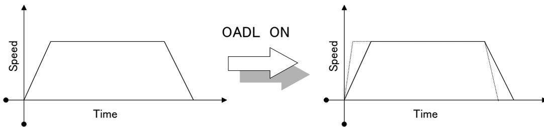
Fig.4-29:Acceleration/deceleration pattern at light load
