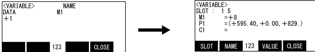
6) Press the function key corresponding to "Close", and return to the monitor menu screen.
