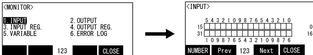
The case where the state of the input signals 8-15 is confirmed is shown in the following.
