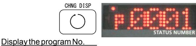
3) Press the controller [CHG DISP] switch, and display the program No.
