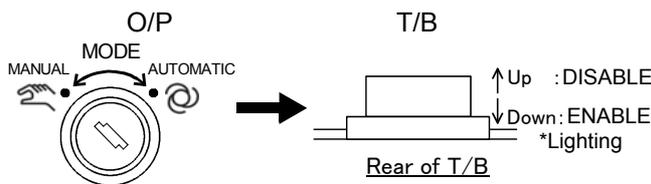
1) Set the controller [MODE] switch to "MANUAL".
