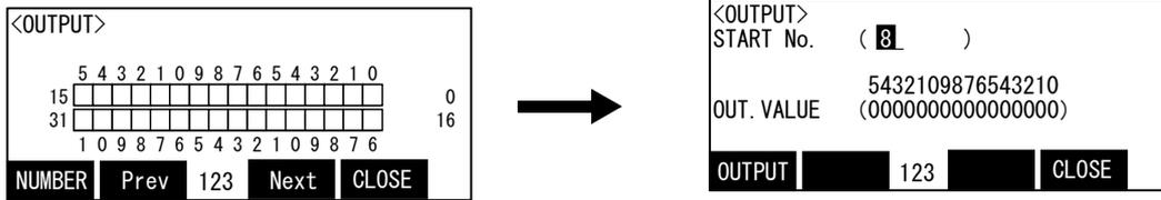
4) Move the cursor to the position of "8" of the output value by the arrow key.
