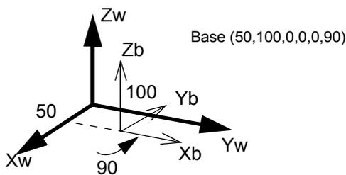
Fig.4-14:Conceptual diagram of the base coordinate system
