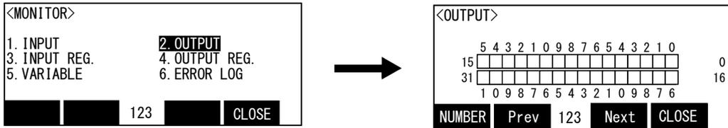
The case where the state of the output signals 8–15 is confirmed is shown in the following.
