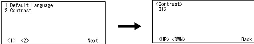
4) If it makes the screen bright, the [F1] key is pressed, if it makes it dark, press the [F2] key, and set it as the good brightness. It becomes so bright that the numerical value is large. .
