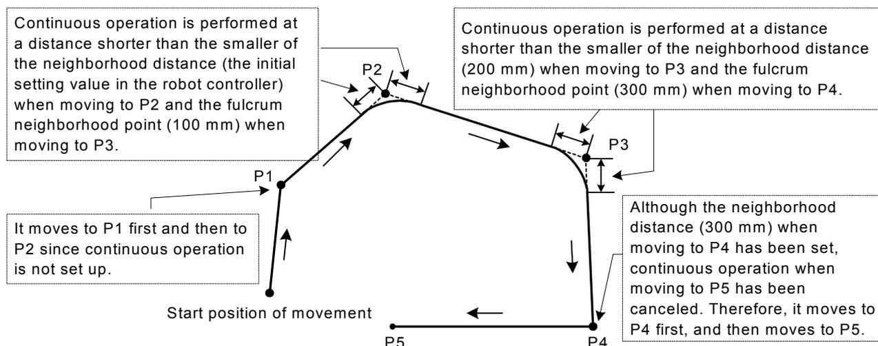
Fig.4-18:Example of continuous path operation
