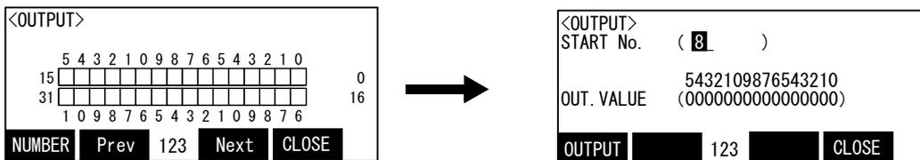
Although the state of the current output signal is displayed on the output value on the display, it is not always the display here in the section which sets up the compulsive output value of the signal. Press the function key corresponding to "Close". Display the ON/OFF state of the 32 points at the head for the output signal No. 8. Black painting indicates ON and white indicates OFF.
