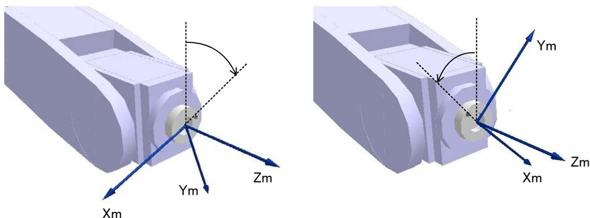
Fig.4-9:Rotation of flange and mechanical interface coordinate system
