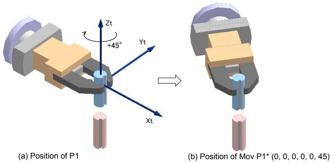
Fig.4-13:Rotational motion in tool coordinate system
