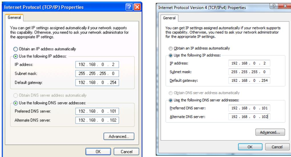
The personal computer IP address is set with the Windows TCP/IP Property Network setting (property in network computer). Because the set-up screen differs with versions of Windows, refer to the manuals enclosed with Windows, etc., for details on setting this address.
