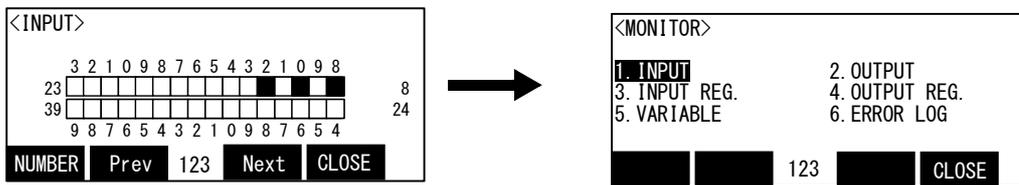
5) Press the function key corresponding to "Close" in monitor menu screen is pressed, finish the monitor, and return to the original screen.
