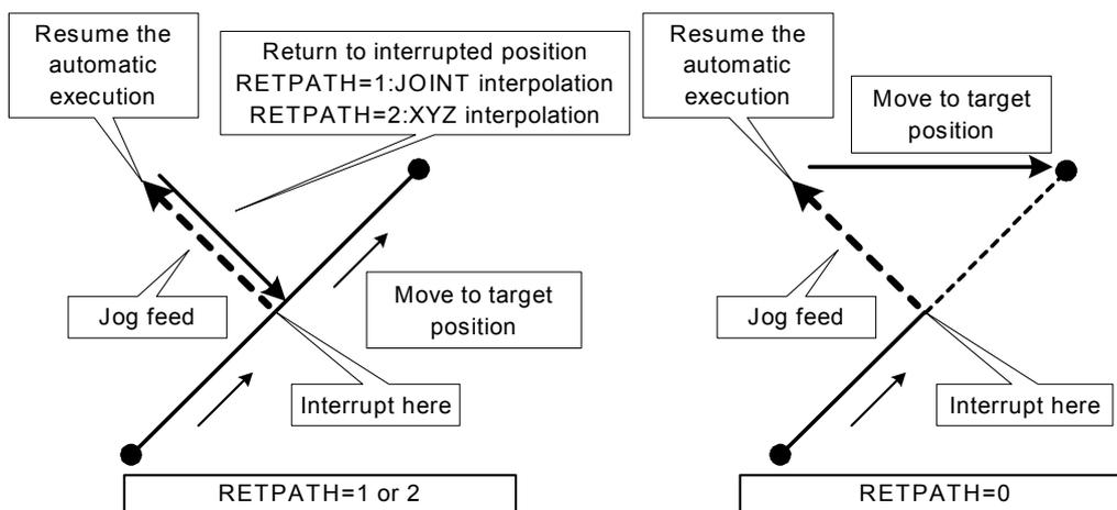
[Caution] If movement other than a joint jog (XYZ, tools, cylindrical, etc.) has been used when the "RETPATH" parameter is set to 1, joint interpolation will be used to return to the original position at the time pause took place. Therefore, be careful not to interfere with peripheral devices.
