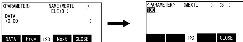
If the [EXE] key is pressed, the buzzer will sound, the value will be fixed and it will return to the screen of the parameter.
