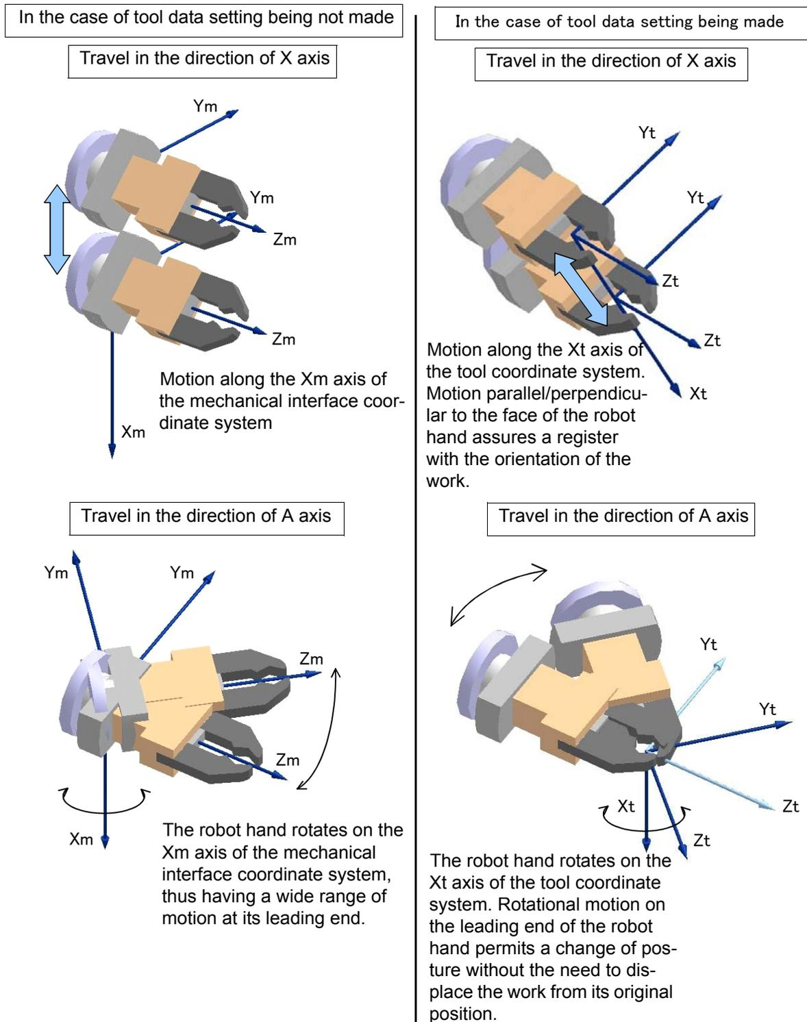
Fig.4-11: Tool jogging operation with/without tool data
