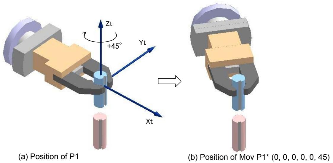
Fig.4-13:Rotational motion in tool coordinate system
