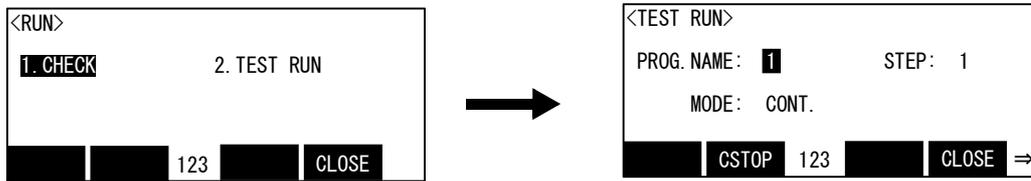
3) When the function key ([F2]) corresponding to "CSTOP" is pressed during program execution, it is change to the cycle mode of operation. The "cycle" is displayed after the mode and the [END] button of the operation panel blinks. Finish operation after executing the last line of the End command or the program.
