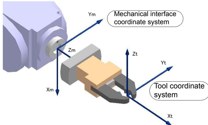
Fig.4-10: Mechanical interface coordinate system and tool coordinate system
