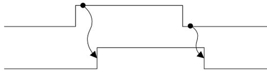
(45) MnWUPMD (Mechanism n warm-up operation status output signal)
