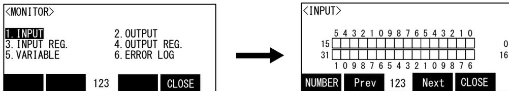
The case where the state of the input signals 8-15 is confirmed is shown in the following.
