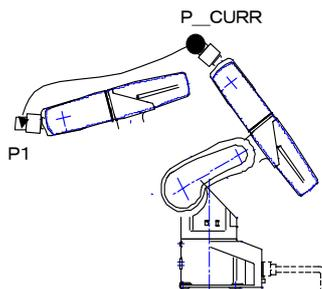
Fig.4-21: Example of joint interpolation motion path
