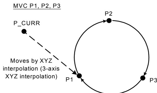
Fig.4-23:Example of circle interpolation motion path
