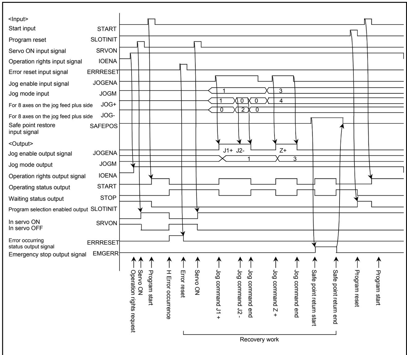
Fig.6-5:Example of external operation timing chart (Part 4)
