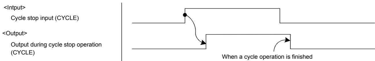
(15) MELOCK (Machine lock input/output during machine lock)
