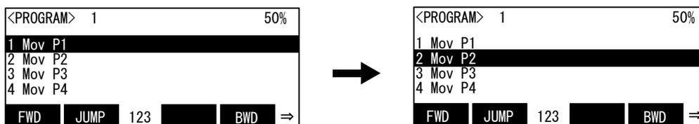
Whenever it presses the function key corresponding to "FWD", step to the following step.
