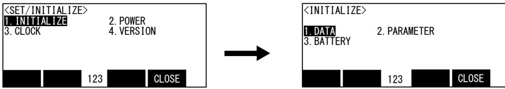
2) Press the [3] key in the initial menu screen, and select the battery. Display the screen of confirmation
