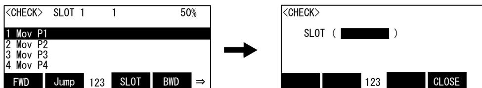
Input the slot number to wish and press the [EXE] key.
