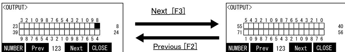
Press the function key corresponding to "Next", then display the next output signal screen. Press the function key corresponding to "Prev", then display the previous output screen
