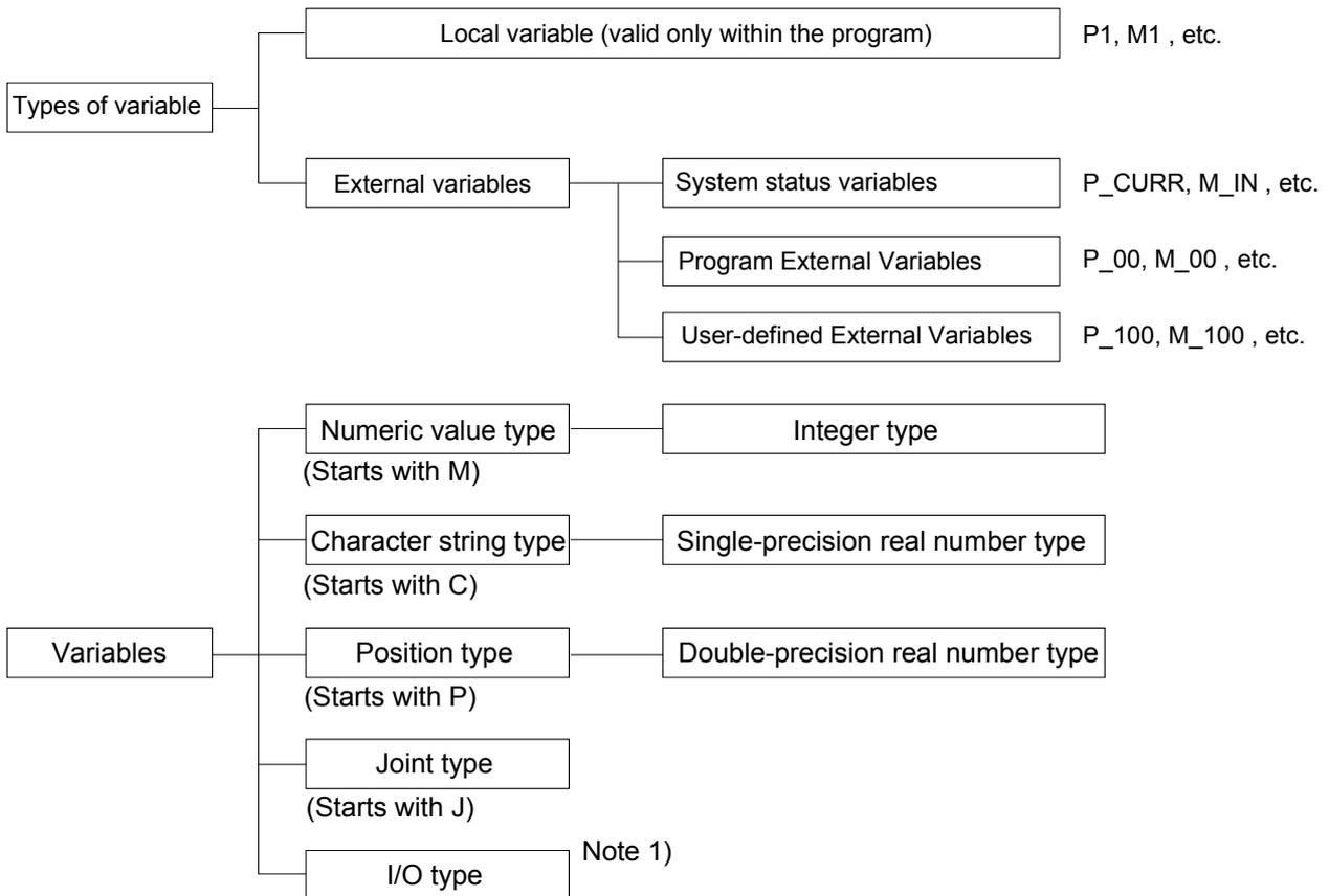
Note 1) The identifiers include those determined by the robot status variable (M\_IN, M\_OUT, etc.), and those declared in the program with the DEFIO command.
