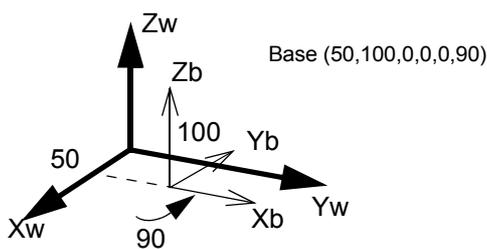
Fig.4-14:Conceptual diagram of the base coordinate system
