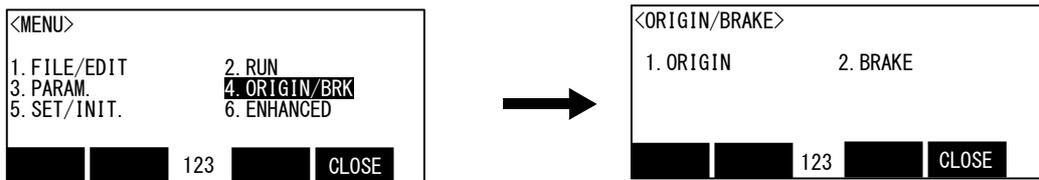
2) Press the [2] key in the origin/break screen, and display the break release screen.
