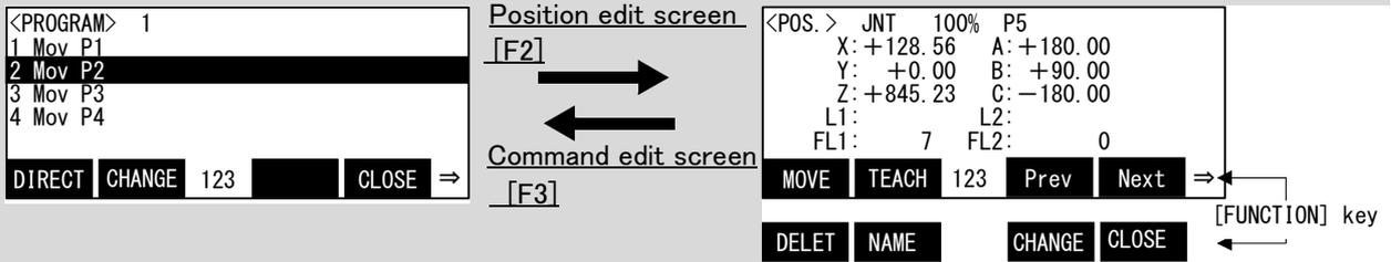
The position variable of order can be called one by one by Prev (F3) and Next (F4). Usually, although it is the call of only the position variable, change the function key and the call can do the joint variable by the name (F2). After calling the joint variable, the joint variable of order can be called one by one by Prev (F3) and If it displays to the head or the last by the joint variable, it will return to the position variable by the next display.
