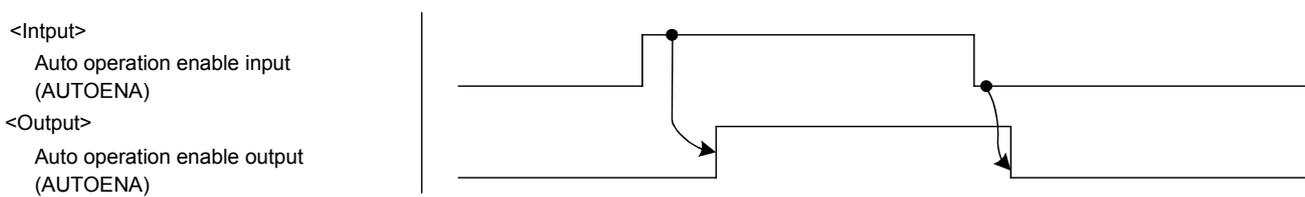
(14) CYCLE (Cycle stop input/output during cycle stop operation)
