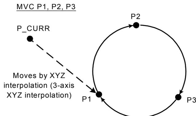
Fig.4-23:Example of circle interpolation motion path
