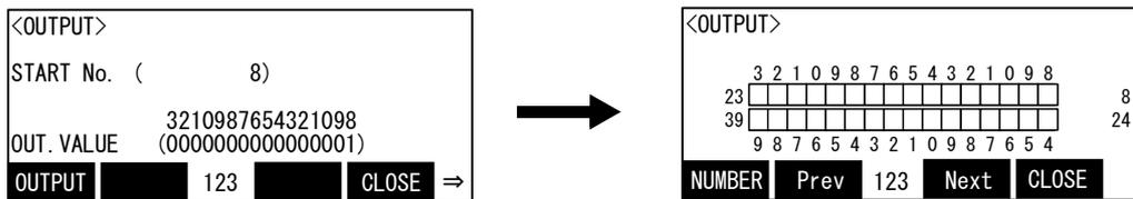
6) Press the function key corresponding to "Close", and return to the monitor menu screen.
