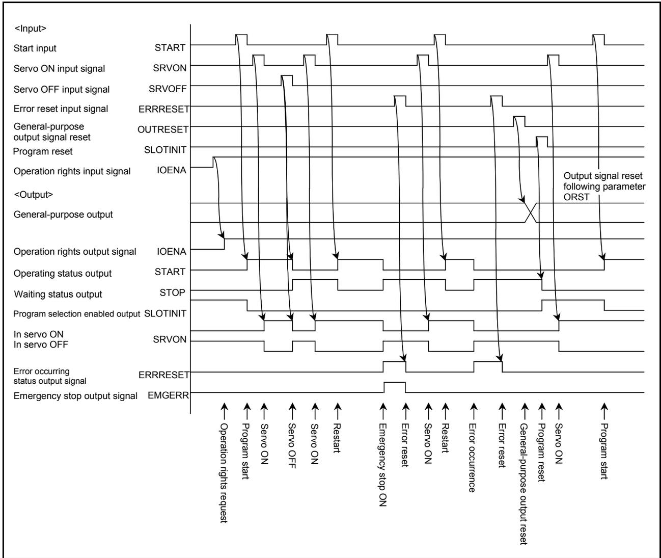
Fig.6-4:Example of external operation timing chart (Part 3)
