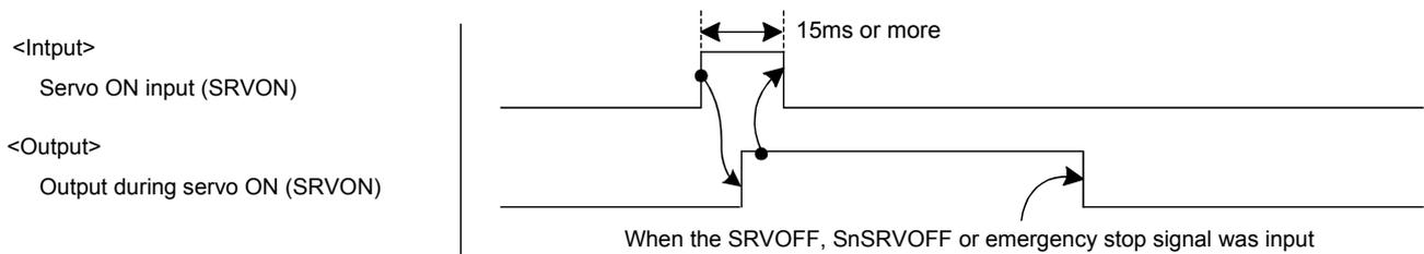
(12) SRVOFF (Servo OFF input/servo ON disable output)
