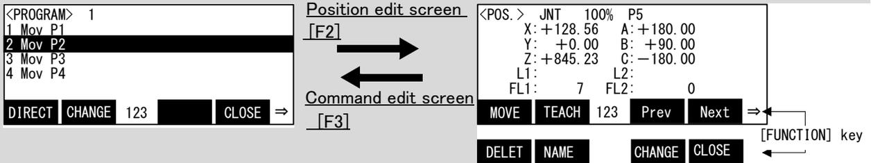
The position variable of order can be called one by one by Prev (F3) and Next (F4). Usually, although it is the call of only the position variable, change the function key and the call can do the joint variable by the name (F2). After calling the joint variable, the joint variable of order can be called one by one by Prev (F3) and If it displays to the head or the last by the joint variable, it will return to the position variable by the next display.
