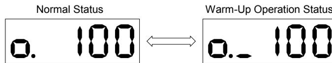
Fig.5-6:Override Display in the Warm-Up Operation Status
