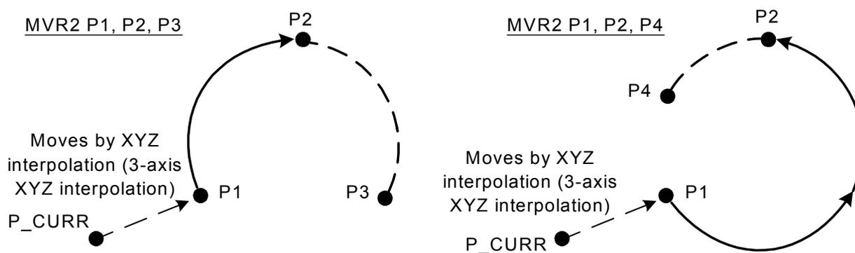
Fig.4-25:Example of circular interpolation motion path 2
