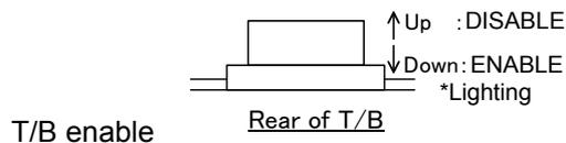
2) Set the T/B [ENABLE] switch to "ENABLE".
