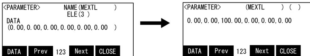
If the [EXE] key is pressed, the buzzer will sound, the value will be fixed and it will return to the screen of the parameter.
