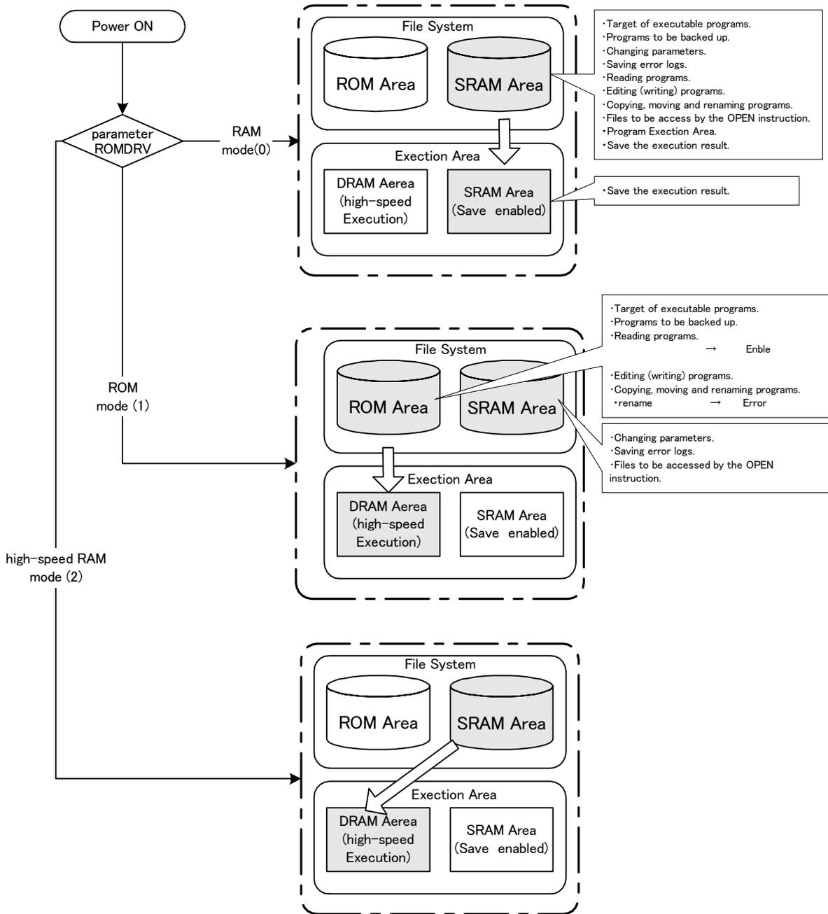
DRAM is used as execution memory during ROM operation/high-speed RAM operation; it can perform language processing at a maximum speed of about 1.2 times faster than that of SRAM memory used for normal RAM operation. (The speed varies depending on the contents of each program.)
