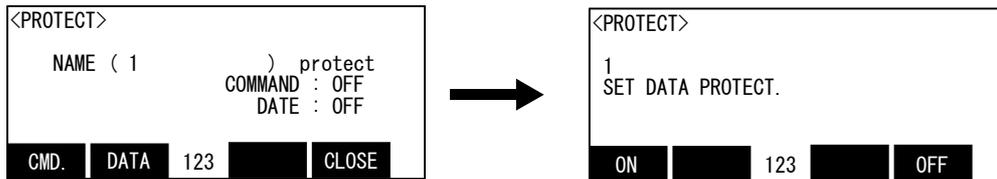
If the function key corresponding to "ON" is pressed, it will be set up for "protecting." If the function key corresponding to "OFF" is pressed, it will be set up for "not protecting."
