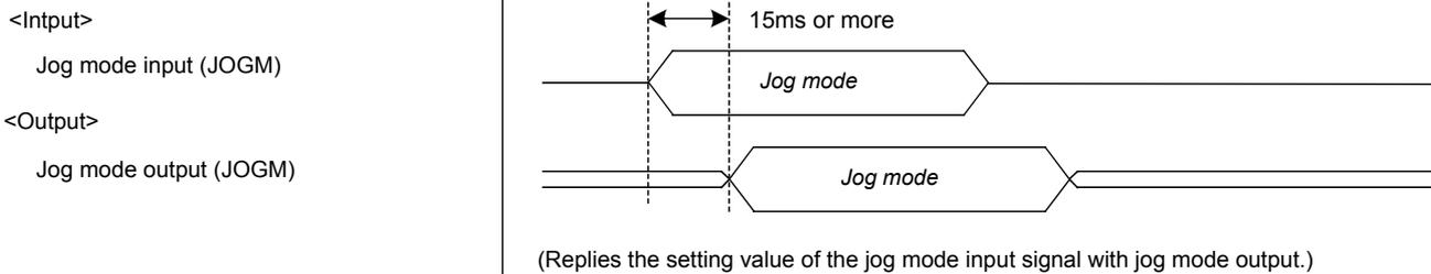
(37) JOG+ (Input for 8 axes on jog feed plus side)
