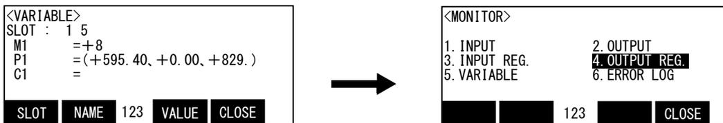
7) Press the function key corresponding to "Close" in monitor menu screen is pressed, finish the monitor, and return to the original screen.
