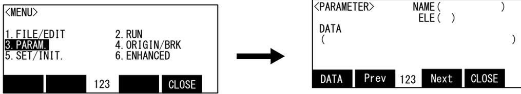
An example of changing the parameter "MEXTL (tool data)" Z axis (3rd element) setting value from 0 to 100mm is shown below.
