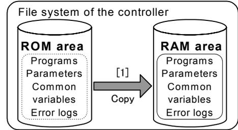
**CAUTION** If the information in the RAM area is restored into the ROM area, all the contents of the parameters changed during the ROM operation, the values of common variables, and logs of errors occurred are discarded. If any parameter was changed during the ROM operation, change the parameter again after switching to the RAM operation is complete.
