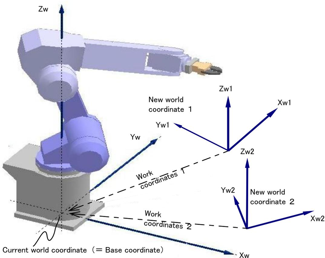
Fig.4-15:Base conversion with a work coordinate system number being specified
