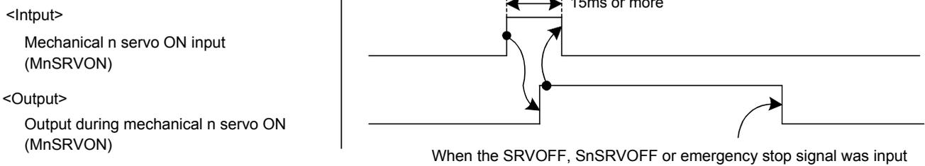
(27) MnMELOCK (Mechanical n machine lock input/output during mechanical n machine lock)
