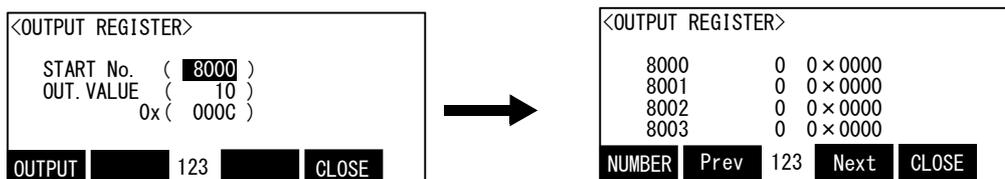
6) Press the function key corresponding to "Close", and return to the output menu screen
