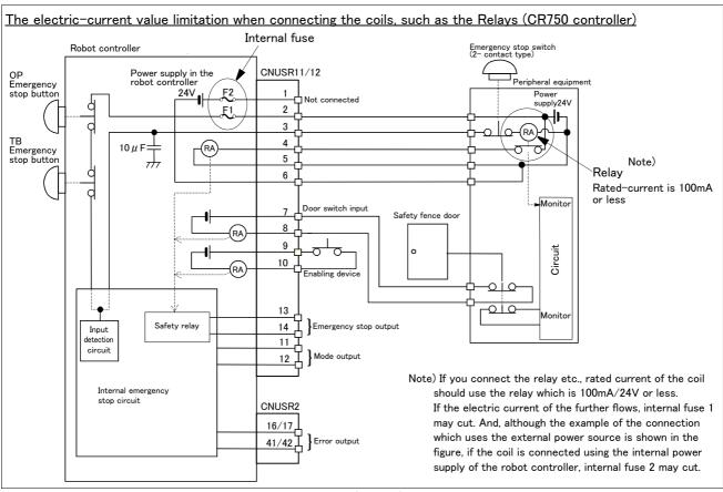
Fig.2-40: Limitations when connecting the relay etc. (CR750)
