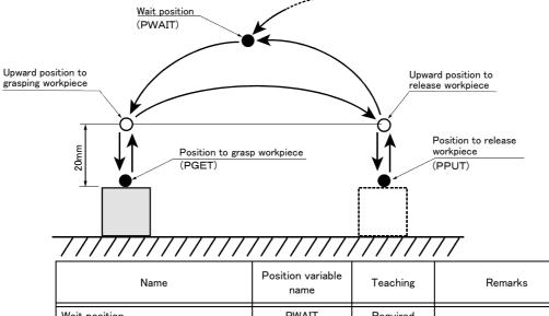
**PWAIT** Wait position Required Upward position to grasping Not required Designate with commands. workpiece PGET Position to grasp workpiece Required Upward position to release workpiece Not required Designate with commands. Position to release workpiece **PPUT** Required
