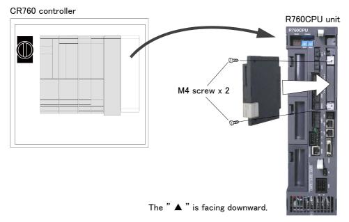
Fig. 3-3: Installing the extension memory cassette
