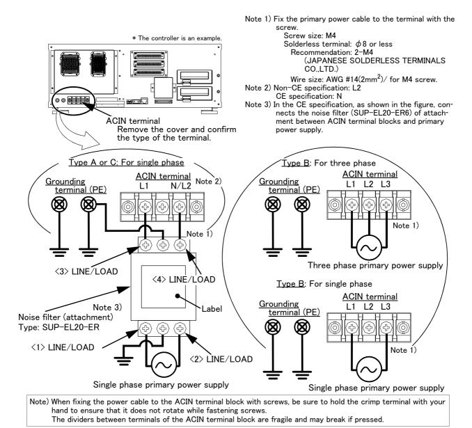
Fig. 2-10: Connecting the power cable and grounding cable (CR750)
