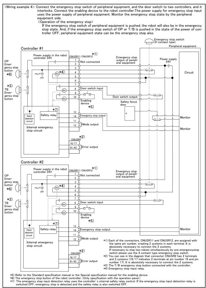
Fig.2-28: Example of safety measures (Wiring example 4)
