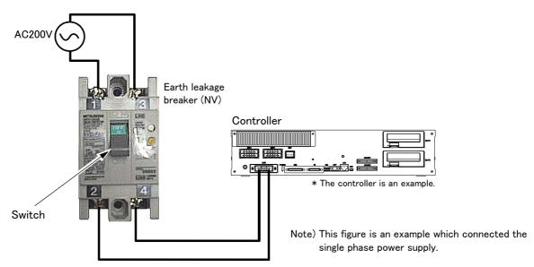
Operate the earth leakage breaker of installation outside to do the controller's power supply ON/OFF. Turns ON the switch of the earth leakage breaker of installation outside. The controller power turn on, and the power lamp lights up.
