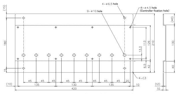
Fig. 2-4: Metal plate for fixation to placing vertically (reference) (CR750 controller)
