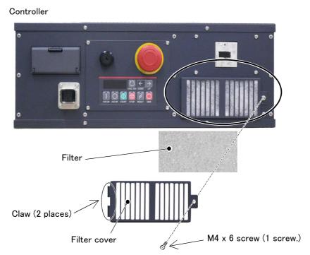
Fig. 5-4: Cleaning, exchanging the filter (CR750 controller)
