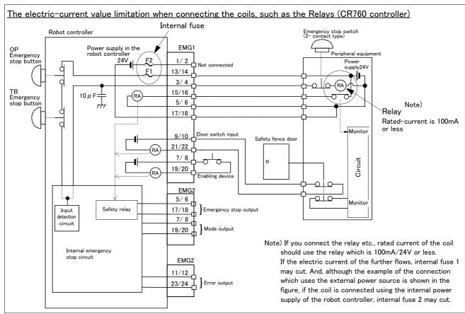
Fig.2-42: Limitations when connecting the relay etc. (CR760)
