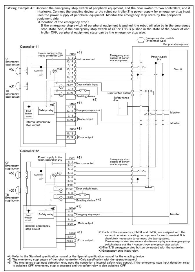
Fig.2-38: Example of safety measures (Wiring example 4)
