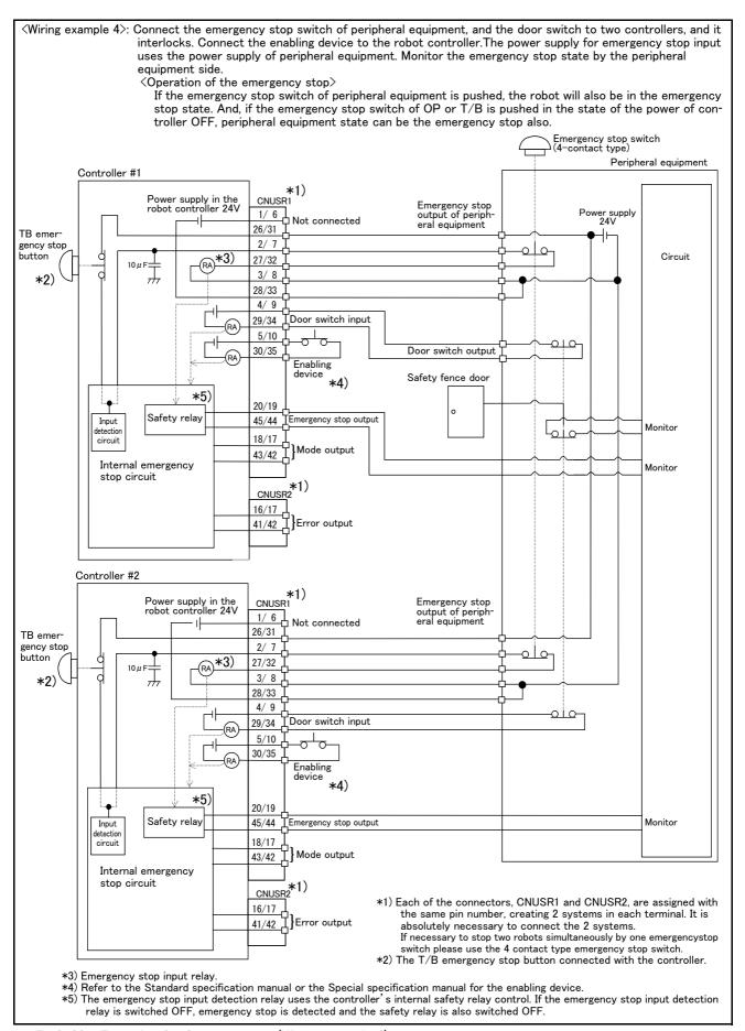
Fig.2-33: Example of safety measures (Wiring example 4)
