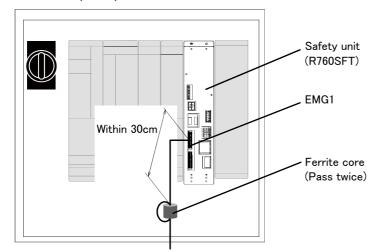
Fig. 2-13: Emergency stop cable connection
