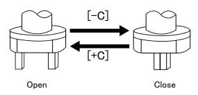
Opening and closing hand 1 Open: Press [+C] key Close: Press [-C] key Opening and closing hand 2 Open: Press [+B] key Close: Press [-B] key Opening and closing hand 3 Open: Press [+A] key Close: Press [-A] key Opening and closing hand 4 Open: Press [+Z] key Close: Press [-Z] key Opening and closing hand 5 Open: Press [+Y] key Close: Press [-Y] key Opening and closing hand 6 Open: Press [+X] key
