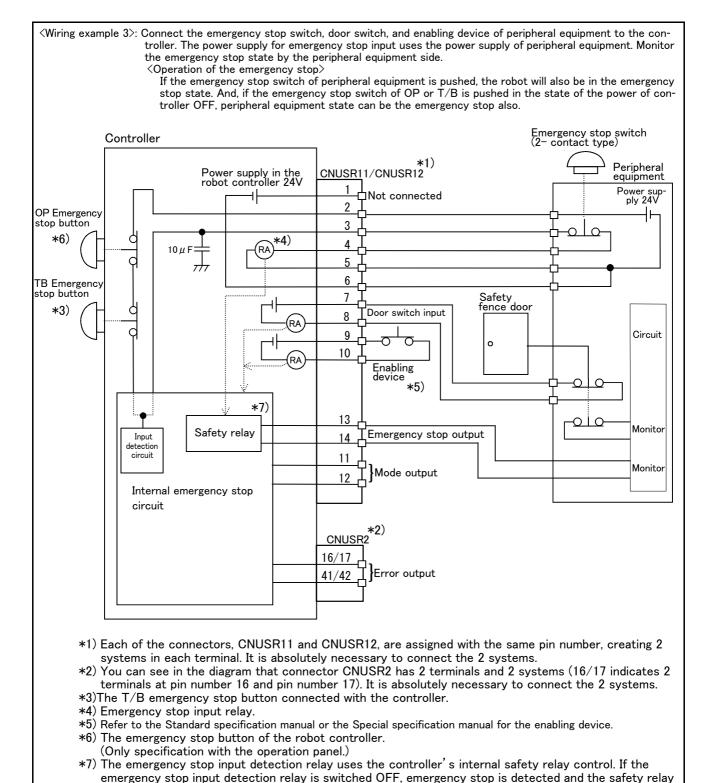
Fig.2-27: Example of safety measures (Wiring example 3)
