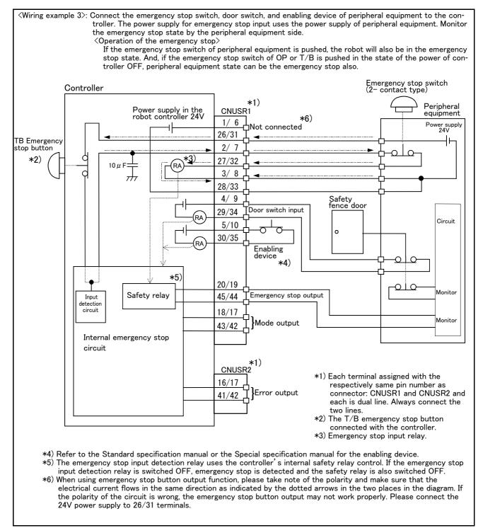
Fig.2-32: Example of safety measures (Wiring example 3)
