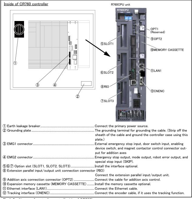
Fig.4-5: Names of controller parts (inside of CR760)
