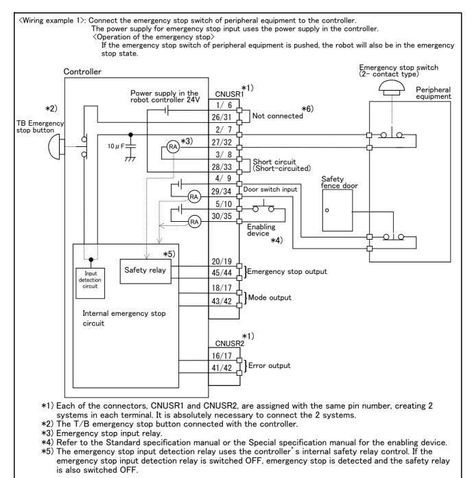
Fig.2-30: Example of safety measures (Wiring example 1)
