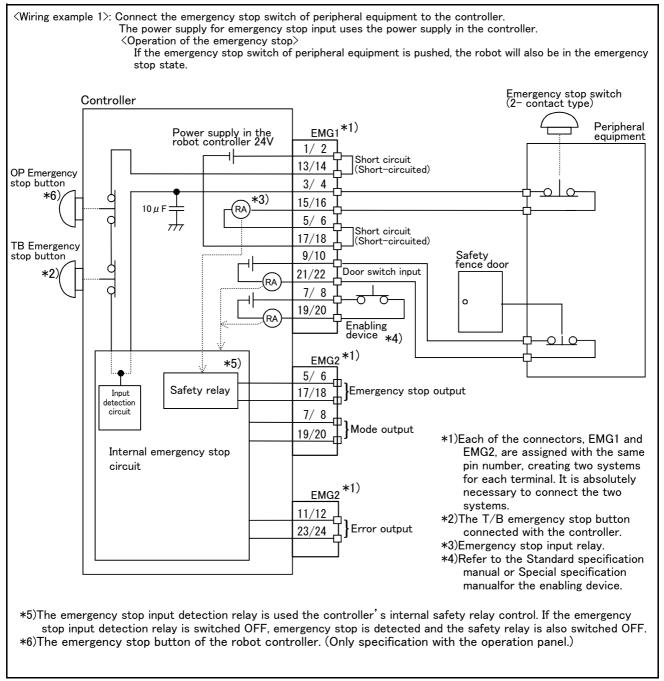
Fig.2-35: Example of safety measures (Wiring example 1)
