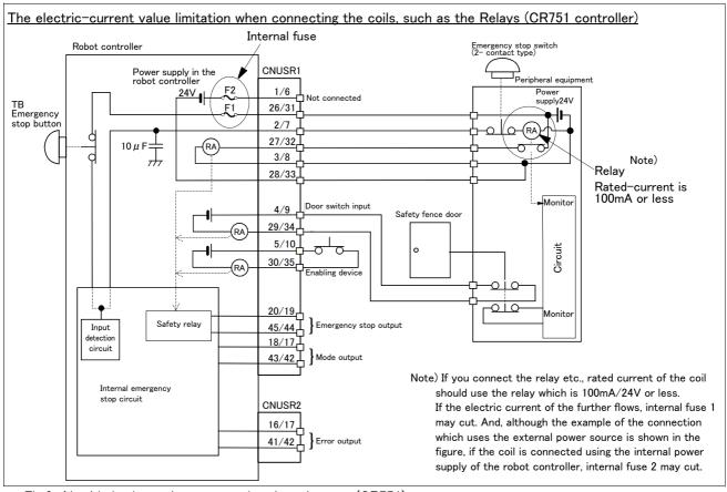
Fig.2-41: Limitations when connecting the relay etc. (CR751)
