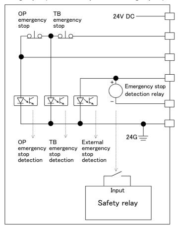
Fig.2-43: Internal circuit of controller
