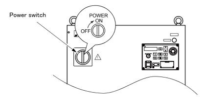
Turn the controller [POWER] switch ON. The controller power turn on, and the STATUS NUMBER display lights up.
