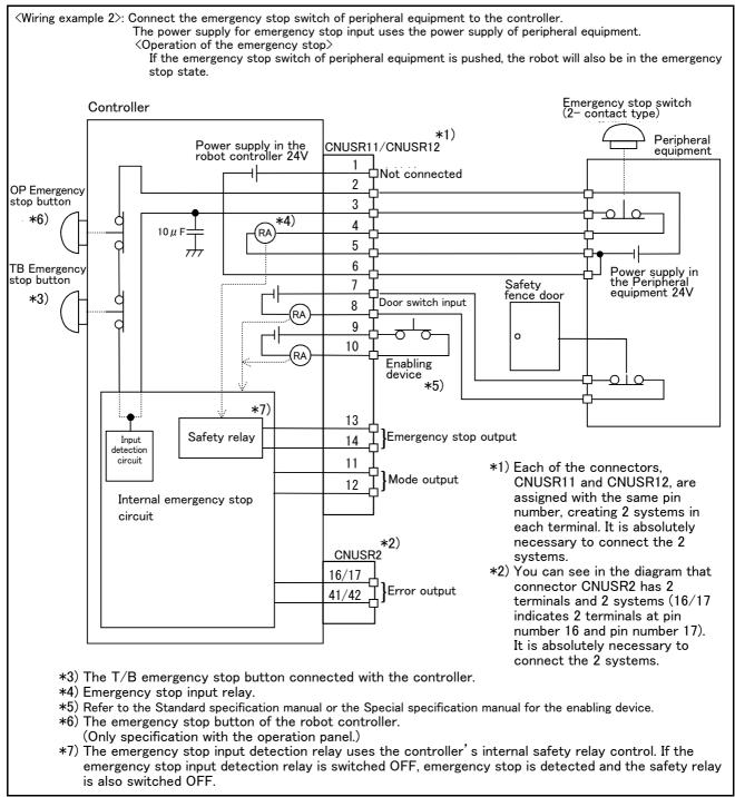
Fig.2-26: Example of safety measures (Wiring example 2)
