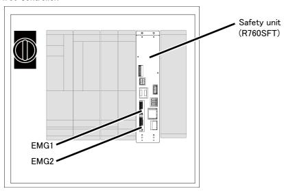
Fig. 2-22: Arrangement of connectors for exclusive input/output signals
