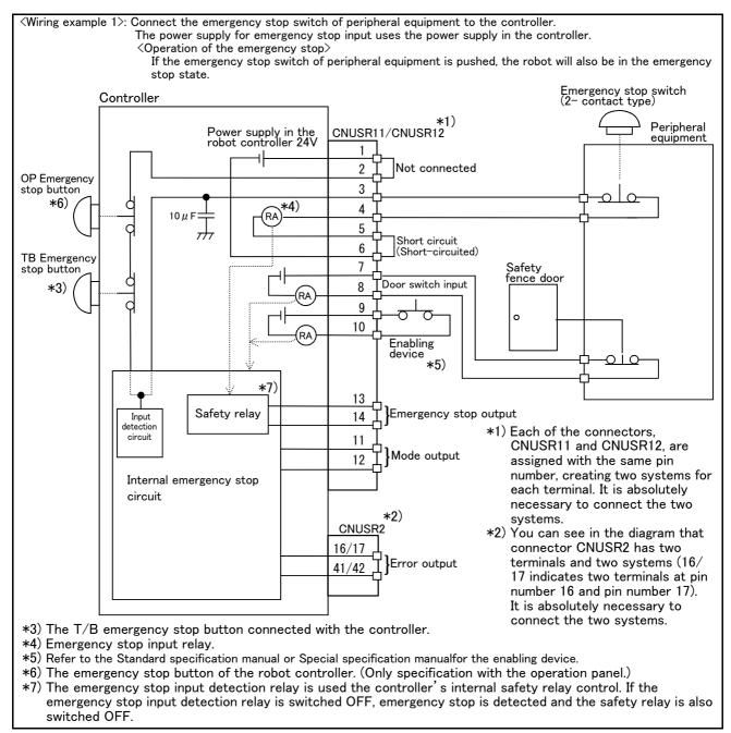
Fig.2-25: Example of safety measures (Wiring example 1)
