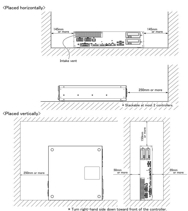
Fig. 2-5: Installation dimensions (CR751 controller: Thin type)
