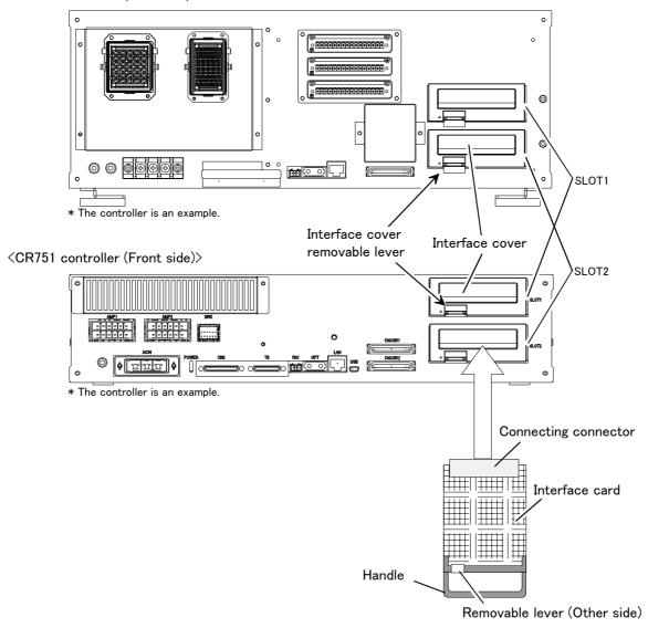
Fig. 3-1: Installation of the interface card (CR750/CR751 controller)
