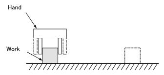
1) Move the robot with jog operation, and set the end of the hand to the position for grasping the workpiece. When the position has been set, open and close the hand to confirm that the workpiece can be grasped.
