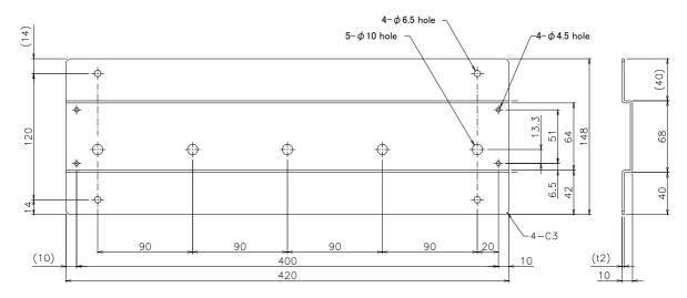
Fig. 2-6: Metal plate for fixation to placing vertically (reference)
