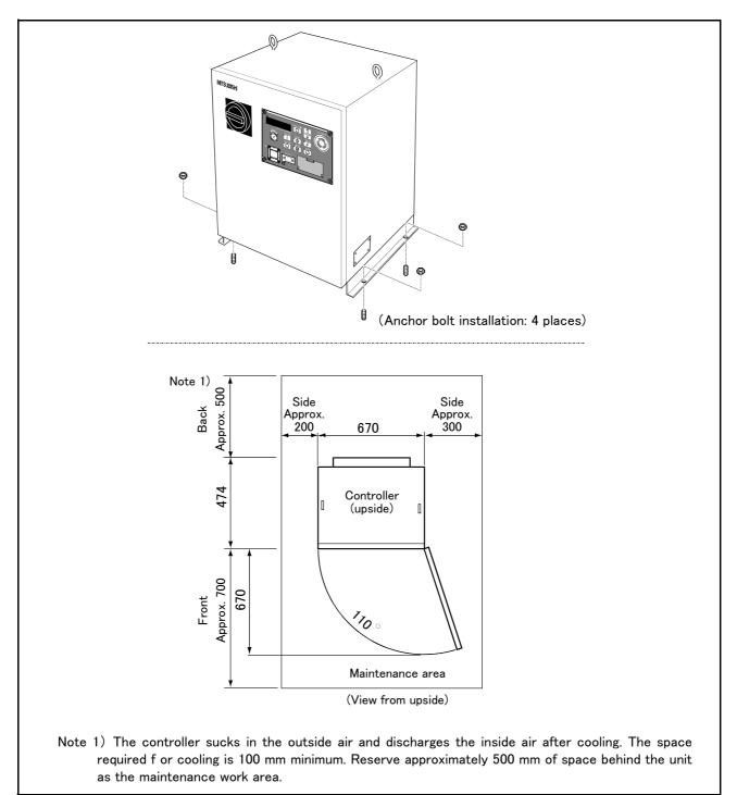
Fig. 2-9: Installation dimensions (CR760 controller)
