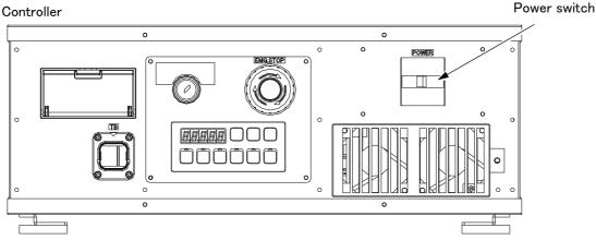
Turn the controller [POWER] switch ON. The controller power turn on, and the STATUS NUMBER display lights up.
