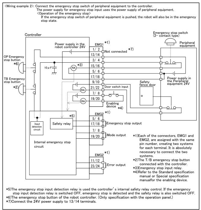
Fig.2-36: Example of safety measures (Wiring example 2)
