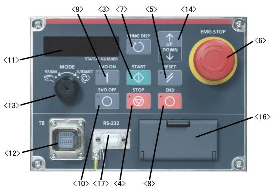
Fig.4-3: Names of controller parts (CR760)
