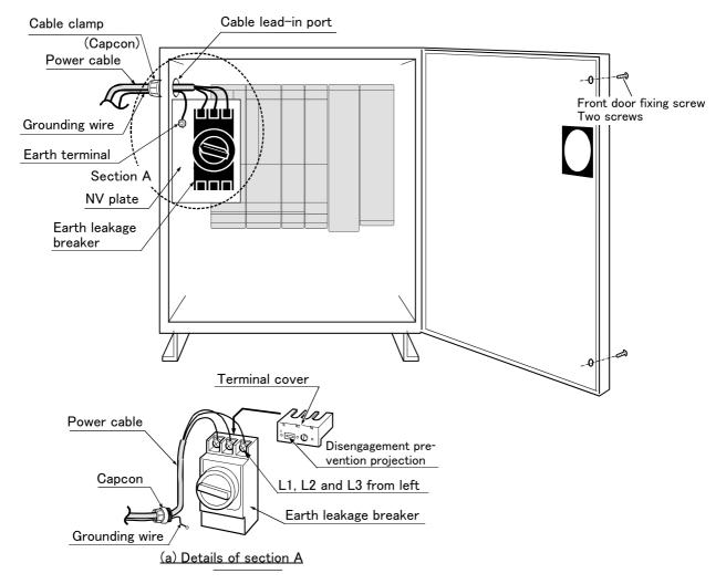
Fig. 2-12: Connecting the power cable and grounding cable (CR760)
