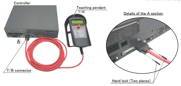
Fig. 4-7: Installing and removing the T/B (CR751 controller)
