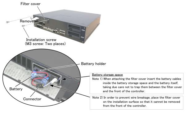
Fig. 5-3: Exchange of the battery (CR751 controller)
