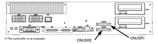
Fig. 2-19: Arrangement of connectors for exclusive input/output signals
