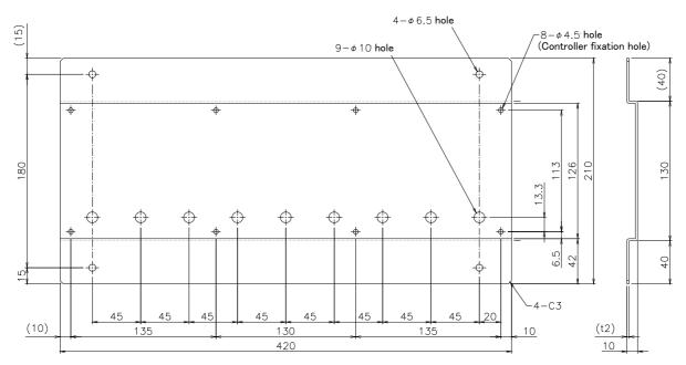
Fig. 2-8: Metal plate for fixation to placing vertically (reference)
