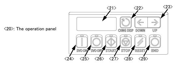
Fig.4-1: Names of controller parts (CR750)
