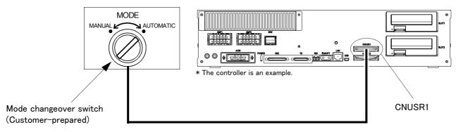
Fig.2-23: Mode changeover switch image figure (CR751)
