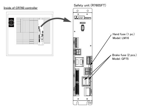
Fig.2-2 : Pneumatic hand's power fuse and brake fuse exchange place (CR760 controller)
