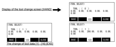
4) Press the function key assigned for "CLOSE" and finish.
