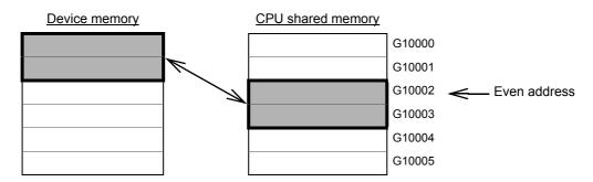
Fig.4-34:Preventing 32-bit data separation
