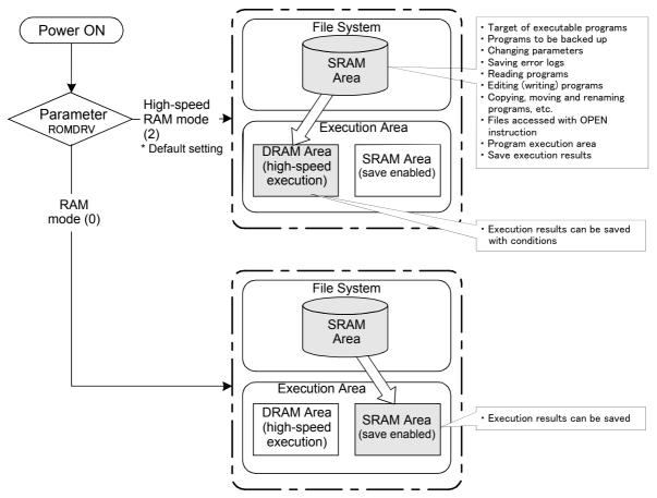
Fig.5-4:High-speed RAM operation image
