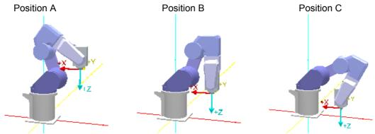
The robot can pass a singular point when the robot's motion path passes through the singular point. If the motion path does not go through the singular point (passes near the singular point), the robot continues operation without switching the value of the structure flag.
