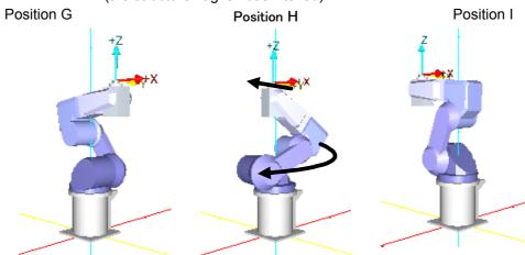
**CAUTION** When passing near a singular point, the robot may rotate in a wide circle as in the case of position H in the figure above. Be sure to keep an eye on the robot and avoid getting in the way when working near the robot, such as when teaching positions.
