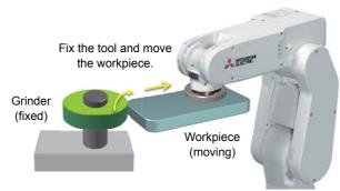
Fig.7-56:Example of polishing
