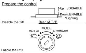
1) Set the T/B [ENABLE] switch to "DIS-ABLE".
