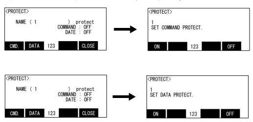
If the function key corresponding to "ON" is pressed, it will be set up for "protecting." If the function key corresponding to "OFF" is pressed, it will be set up for "not protecting."
