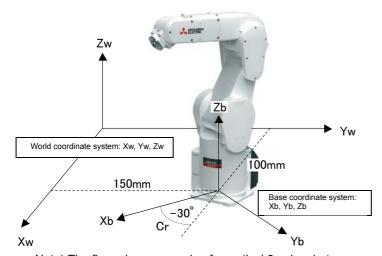
Note) The figure is an example of a vertical 6-axis robot. In horizontal 4-axis robot is the same.
