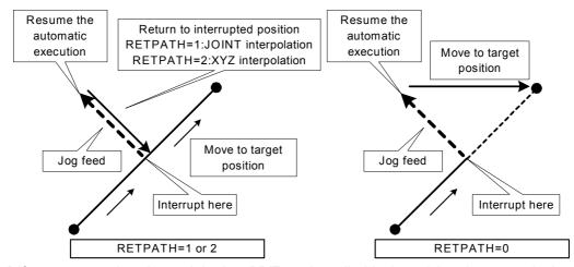
[Caution] If movement other than a joint jog (XYZ, tools, cylindrical, etc.) has been used when the "RET-PATH" parameter is set to 1, joint interpolation will be used to return to the original position at the time pause took place. Therefore, be careful not to interfere with peripheral devices.
