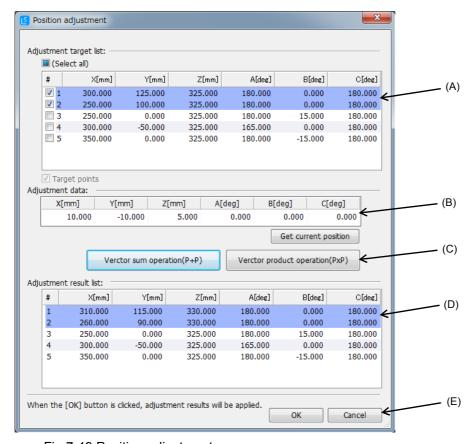
Fig.7-49:Position adjustment screen
