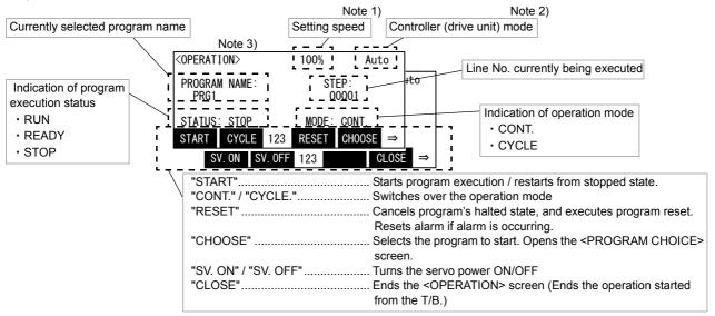
Note 1) If the controller (drive unit) mode is "MANUAL", low speed movement will take place even if the set speed is 100%. (To confirm the movements)
