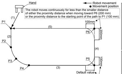
The robot moves continuously for less than the smaller distance of either the proximity distance when moving toward P5 (default value) or the proximity distance to the starting point of the path to P6 (200 mm).
