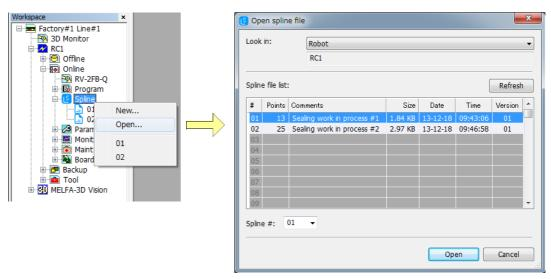
Fig.7-25:Selecting and opening a spline file from the list
