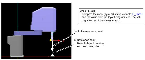
Fig.5-23:Checking the setting for calibration between robots
