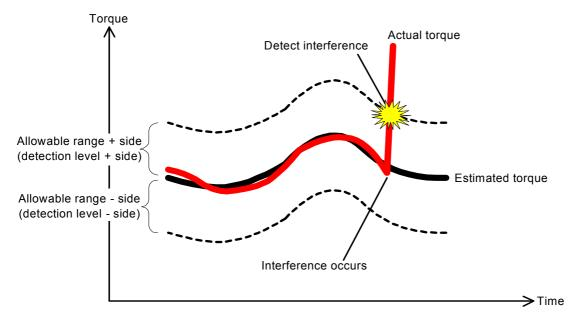
Fig.5-10:Interference detection principle
