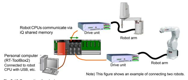
Fig.5-13:Connecting the devices
