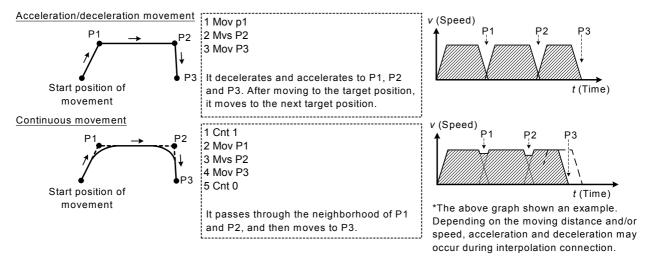
Fig.4-17:Acceleration/deceleration movement and continuous movement
