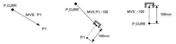
Fig.4-26:Example of movement at linear interpolation
