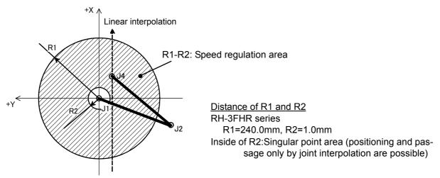
Fig.4-33:Speed regulation area and singular point area
