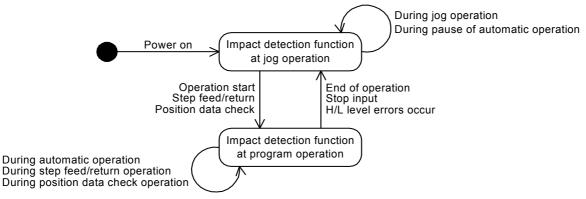
Fig.5-11:State transition diagram illustrating switch between program operation and jog operation
