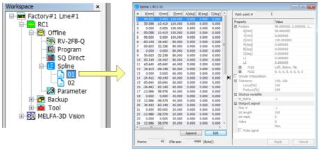
Fig.7-23:Opening a spline file saved in the personal computer
