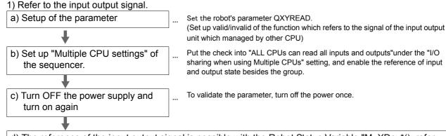
d) The reference of the input output signal is possible with the Robot Status Variable "M XDev\*(): referthe parameter
