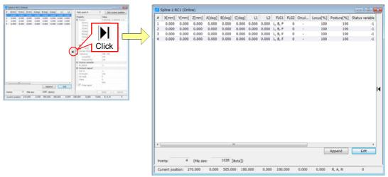
Fig.7-27: State with path point data list area display expanded
