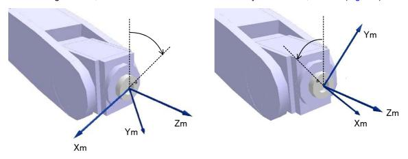
Fig.4-7:Rotation of flange and mechanical interface coordinate system
