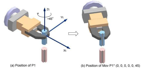
Fig.4-11:Rotational motion in tool coordinate system
