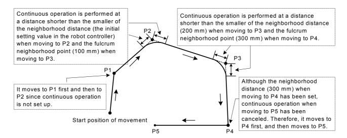
Fig.4-16:Example of continuous path operation
