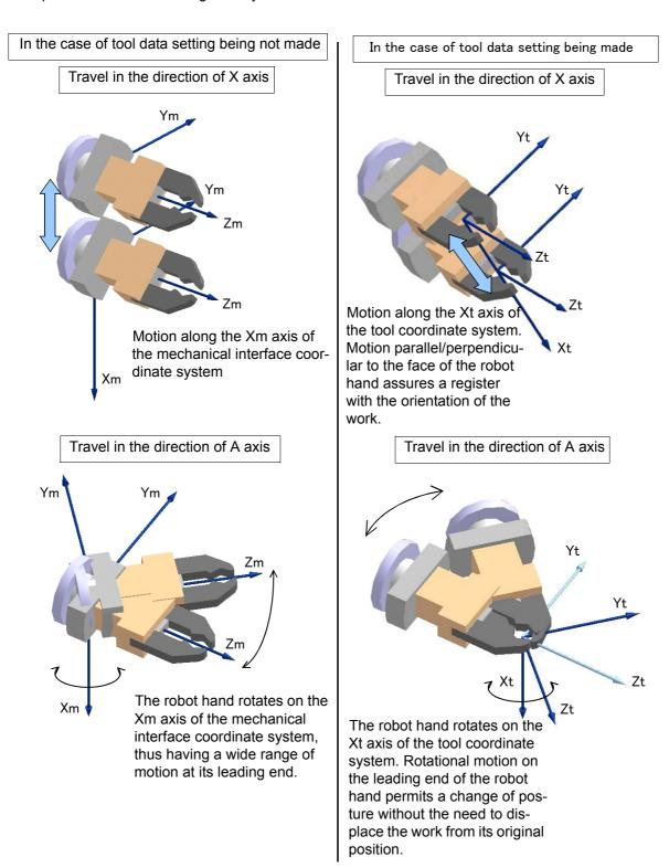
Fig.4-9:Tool jogging operation with/without tool data
