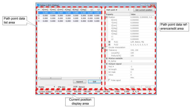
Fig.7-26:Spline File Edit screen
