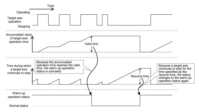
Fig.5-8:Example of Switching Between the Normal Status and the Warm-Up Operation Status
