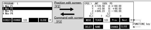
The position variable of order can be called one by one by "Prev" (F3) and "Next" (F4). Usually, although it is the call of only the position variable, change the function key and the call can do the joint variable by the "NAME" (F2). After calling the joint variable, the joint variable of order can be called one by one by "Prev" (F3) and If it displays to the head or the last by the joint variable, it will return to the position variable by the next display.
