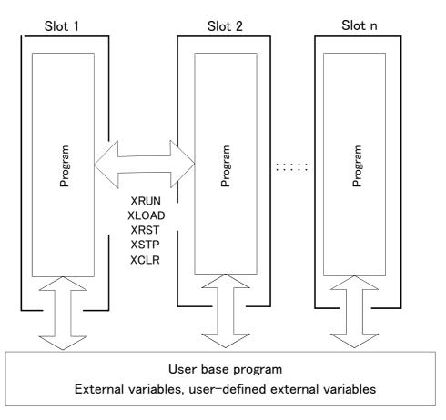
Fig.4-1:Multitask slot environment
