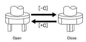
Opening and closing hand 1 Open: Press [+C] key Close: Press [-C] key Opening and closing hand 2 Open: Press [+B] key Close: Press [-B] key Opening and closing hand 3 Open: Press [+A] key Close: Press [-A] key Opening and closing hand 4 Open: Press [+Z] key Close: Press [-Z] key Opening and closing hand 5 Open: Press [+Y] key Close: Press [-Y] key Opening and closing hand 6
