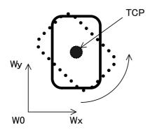
Fig.7-58:Example of C element movement in the WORK jog
