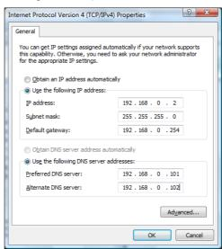
The personal computer IP address is set with the Windows TCP/IP Property Network setting (property in network computer). Because the set-up screen differs with versions of Windows, refer to the manuals enclosed with Windows, etc., for details on setting this address.
