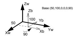
Fig.4-12:Conceptual diagram of the base coordinate system
