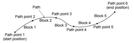
Fig.7-9:Spline interpolation terminology
