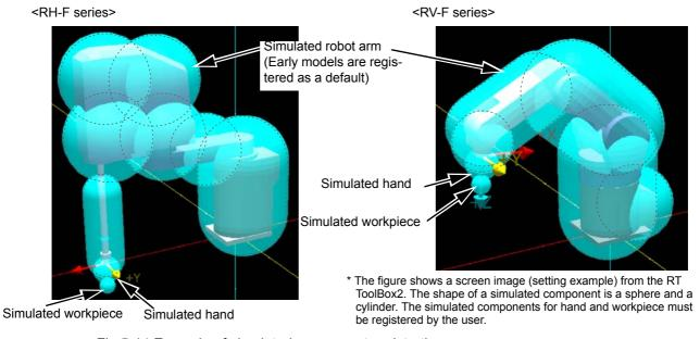
Fig.5-14:Example of simulated component registration
