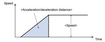
Fig.4-28: Acceleration with <Acceleration/deceleration distance>
