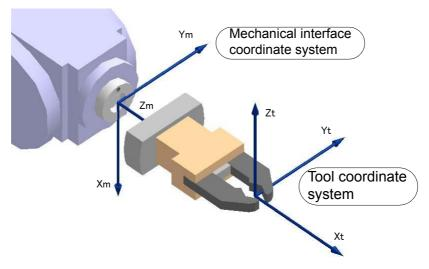
Fig.4-8:Mechanical interface coordinate system and tool coordinate system
