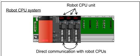
Fig.5-26:Direct communication with robot CPUs
