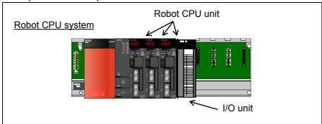
Fig.5-24:Sequencer input/output unit direct control
