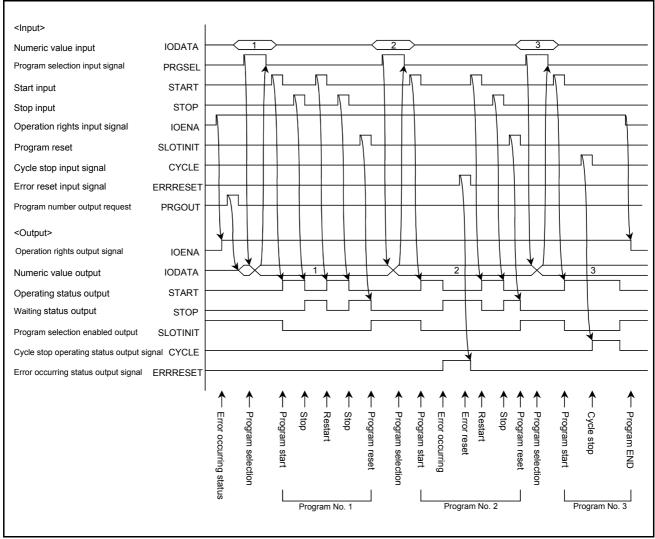
Fig.6-4:Example of external operation timing chart (Part 1)
