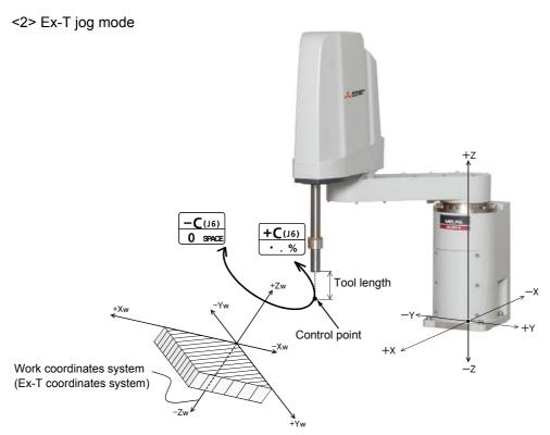
When the [+C (J6)] keys are pressed, the control point will rotate in the plus direction around the Z axis
