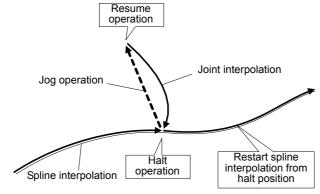
Fig.7-11:Behavior during halt and resume
