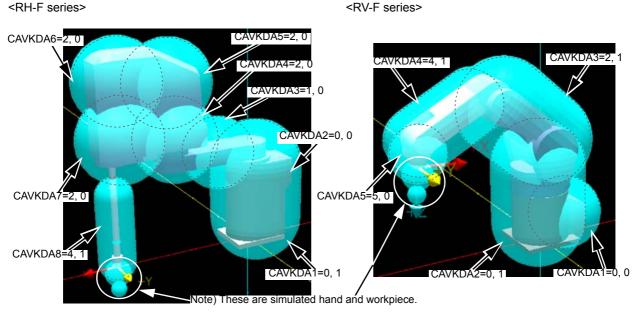
Fig.5-17:Example of registration sections and simulated component type settings
