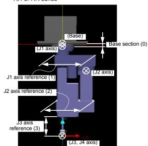
Note) The numbers in parentheses indicate the 1st element (registration section (Jn axis)) setting values of the parameters: CAVKDA1 to 8 (registration section and shape of simulated components).
