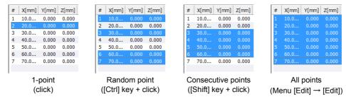
Fig.7-28:Selecting the path point data
