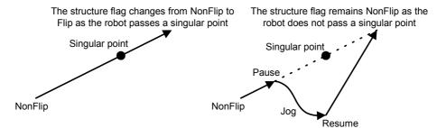
(8) If the singular point passage function is specified, the operation speed may be lowered compared to normal linear interpolation, etc. Moreover, the singular point passage function may affect the execution speed of programs as the function involves complicated processing. Specify the singular point passage function only for interpolation instructions where the function is required.
