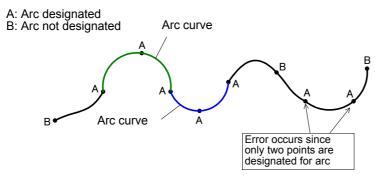
Fig.7-14:Example of error in arc designation
