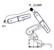
Fig.4-20:Example of joint interpolation motion path
