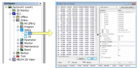
Fig.7-24:Opening a spline file saved in the controller
