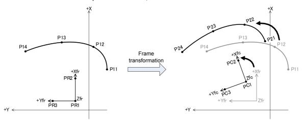
Fig.4-30: Example of frame transformation
