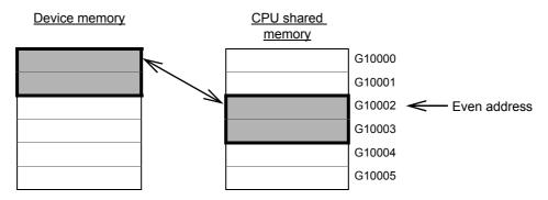
Fig.4-35:Preventing data inconsistency of 32-bit data
