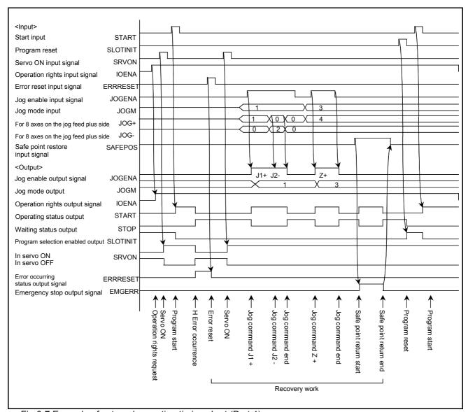
Fig.6-7:Example of external operation timing chart (Part 4)
