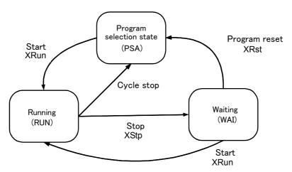
Fig.4-2:Operation state of each slot
