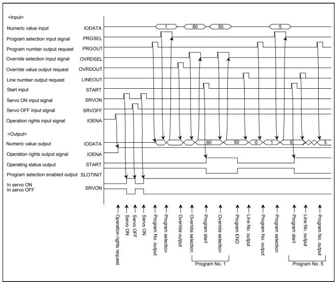
Fig.6-5:Example of external operation timing chart (Part 2)
