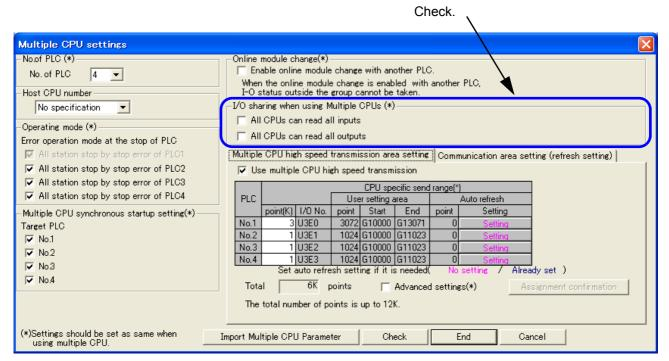
Fig.5-25:The setting screen of multi-CPU in GX Developer
