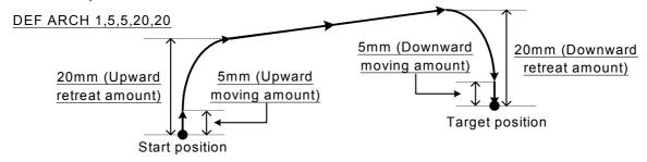
Fig.4-21:Example of arch interpolation motion path (seen from the side)
