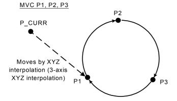
Fig.4-22:Example of circle interpolation motion path
