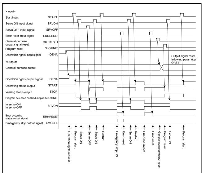
Fig.6-6:Example of external operation timing chart (Part 3)
