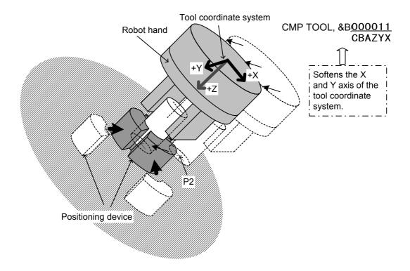
Fig.4-15:The example of using the compliance mode
