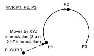
Fig.4-23:Example of circular interpolation motion path 1
