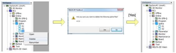
Fig.7-40:Deleting a spline file
