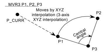
Fig.4-25:Example of circular interpolation motion path 3
