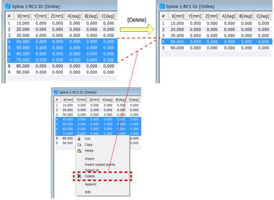
Fig.7-35:Deleting the path point data
