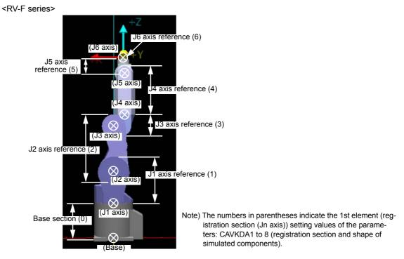
Fig.5-16:Registration sections of simulated components of RV-F series (supplement)
