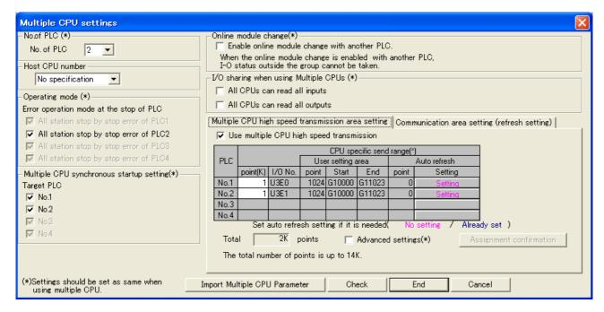
Fig.6-1:Sequencer CPU: Setting screen on GX Developer (example)
