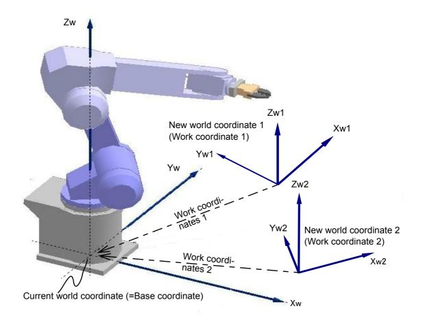
Fig.4-13:Base conversion with a work coordinate system number being specified
