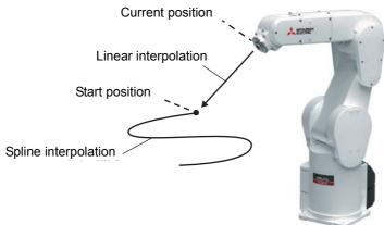
Fig.7-10:When current position and start position differ
