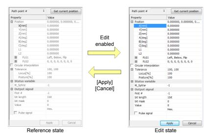
Fig.7-29:Switching between path point data reference/edit area reference state and edit state
