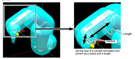
Fig.5-19:Simulated component size (supplement)
