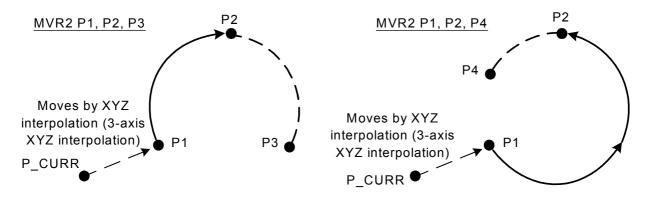
Fig.4-24: Example of circular interpolation motion path 2
