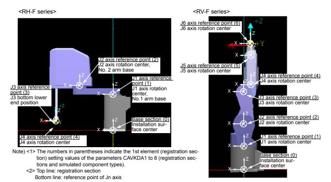
Fig.5-18:XYZ direction of reference point (Jn axis) for each simulated component
