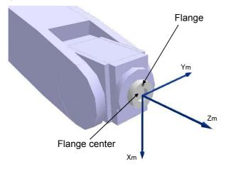
Fig.4-6:Mechanical interface coordinate system
