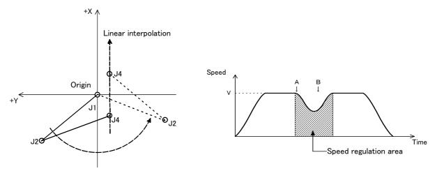
Fig.4-31:Passing through near the origin point
