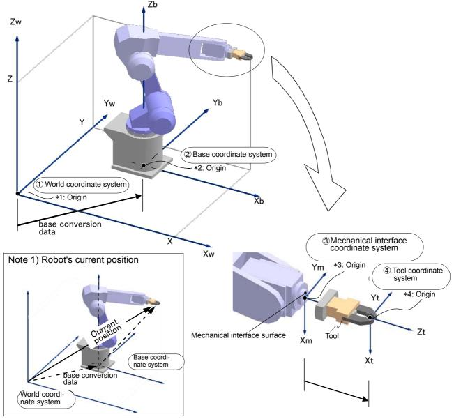
Fig.4-3:Robot's coordinate system
