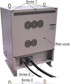
1) Turn off the controller power and primary power supply, and wait for at least three minutes. Remove the rear screw 1 (3 positions), loosen the screw 2 (2 positions), and then remove the rear cover.
