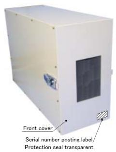
Fig.3-12: Sticking the serial number posting label
