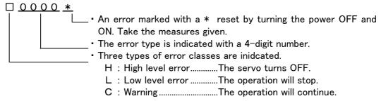
The axis No. may be indicated at the last digit of the error No. Example) H0931 No. 1 axis motor overcurrent.
