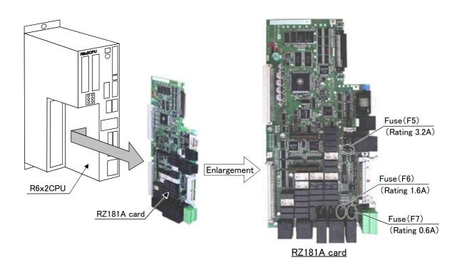
(3) Place where fuse replacement is required in the event of error No. H0084 \* Replace the fuse (F5) of the RZ181A card.
