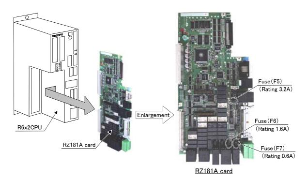
(4) Place where fuse replacement is required in the event of error No. H0085  $\ast$  Replace the fuse (F7) of the RZ181A card.
