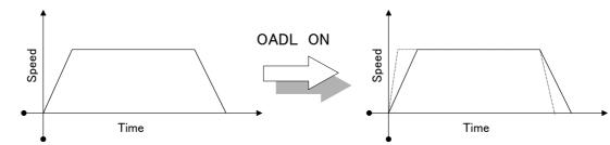
Fig.4-18:Acceleration/deceleration pattern at light load
