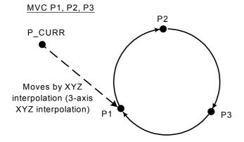
Fig.4-11:Example of circle interpolation motion path
