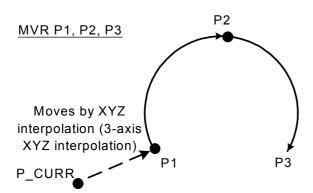
Fig.4-12:Example of circular interpolation motion path 1
