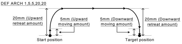
\*If Z is different between the movement starting position and the target position, it will operate as follows:
