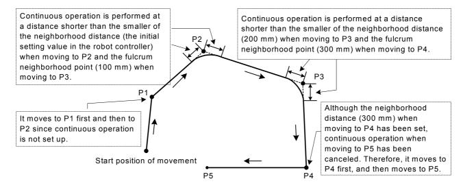
Fig.4-6:Example of continuous path operation
