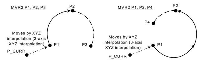
Fig.4-13:Example of circular interpolation motion path 2
