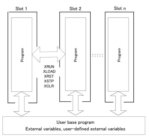
Fig.4-1:Multitask slot environment
