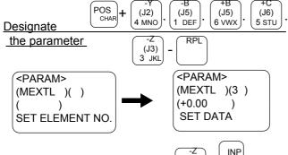
4) Press the [3] key to designate the 3rd element (Z axis), and press the [INP] key. The parameter MEXTL Z axis current value will appear as +0.00.
