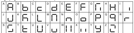
The character "P" is fixed at the beginning of the program name display, which means that the number of characters that can be displayed are four or less. Make sure to use no more than four characters when entering the program name.
