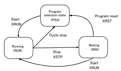
Fig.4-2:Operation state of each slot
