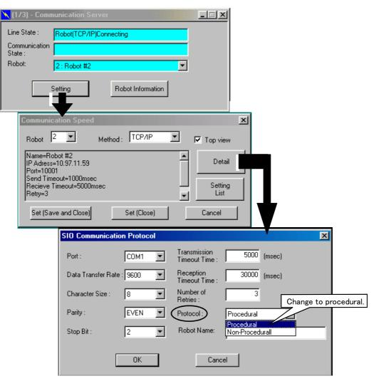
When communicating with the R/C using your custom software, reset the R/C protocol setting to "Non-Procedural" in advance.
