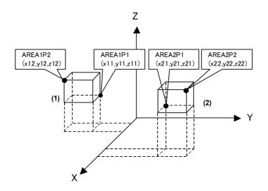
When operation is performed together with peripheral devices, work area may have to be shared. Under such circumstances, one device must let the other know when it is within the shared area. For this purpose, a robot can be configured to output a signal while it is in a certain area by setting parameters.
