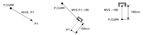
Fig.4-15:Example of movement at linear interpolation
