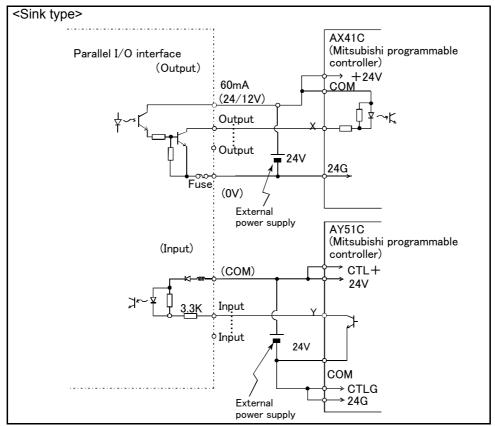
Fig.9-1:Connection with a Mitsubishi PLC (Example of sink type)
