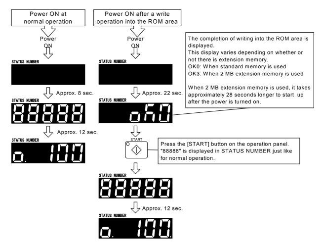
The time required to start up after the power is turned on is based on controller software version H7. It varies depending on the version in use and how memory is used.
