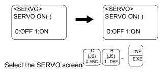
5) To turn ON/OFF the servo, press the [0] key when the servo is OFF or the [1] key when the servo is ON while lightly holding the deadman switch, and then press the [INP] key. (It is also possible to turn the servo on by pressing the [STEP/MOVE] key.)
