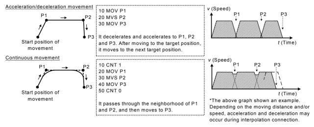
Fig.4-7:Acceleration/deceleration movement and continuous movement
