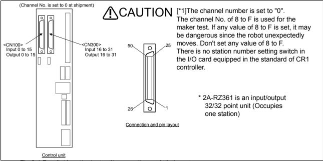
Fig.6-1:Parallel input/output unit connection and pin layout
