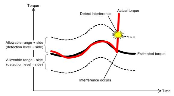
Fig.5-7:Interference detection principle
