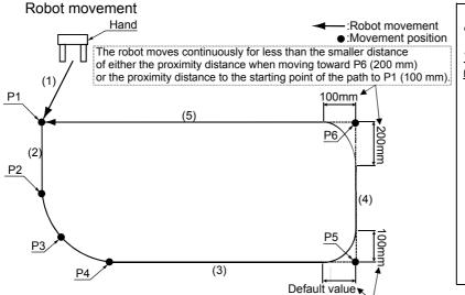
The robot moves continuously for less than the smaller distance of either the proximity distance when moving toward P5 (default value) or the proximity distance to the starting point of the path to P6 (200 mm).
