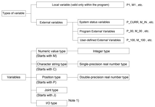
Note 1) The identifiers include those determined by the robot status variable (M\_IN,M\_OUT, etc.), and those declared in the program with the DEFIO command.
