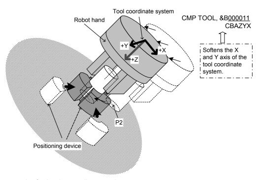
Fig.4-5: The example of using the compliance mode
