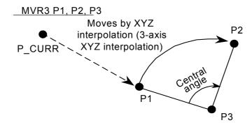
Fig.4-14:Example of circular interpolation motion path 3
