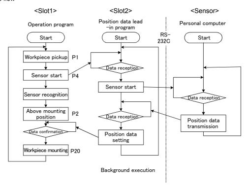
P1: Workpiece pickup position (Vacuum timer DLY 0.05)
