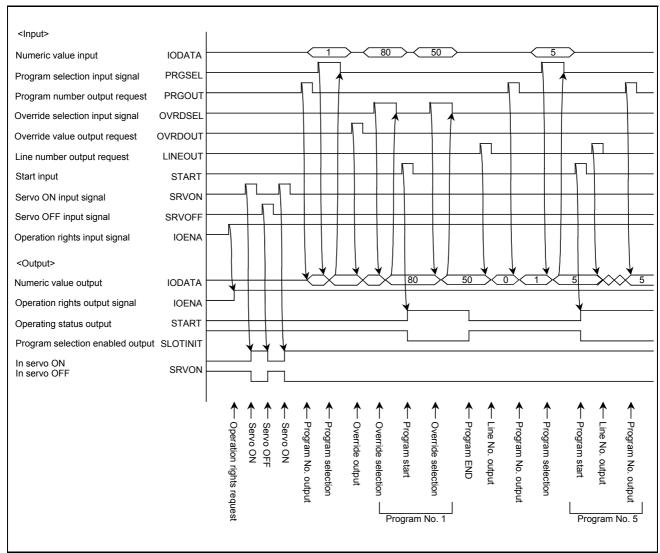
Fig.6-3:Example of external operation timing chart (Part 2)
