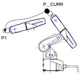
Fig.4-9:Example of joint interpolation motion path
