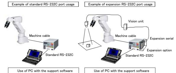
Caution)The example above is for robot controller CR1. Controllers other than the CR1 do not require expansion option box.
