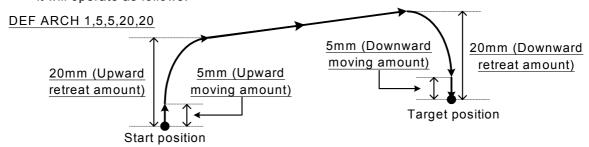
Fig.4-10:Example of arch interpolation motion path (seen from the side)
