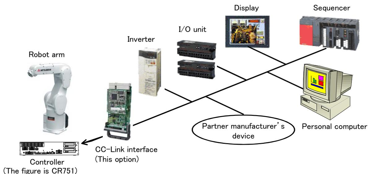
Fig.3-31 : Example of CC-Link Product Configuration
