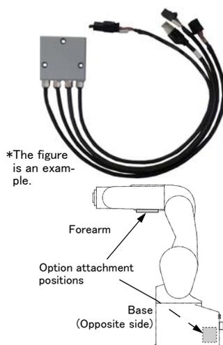
The Forearm external wiring set and the Base external wiring set are used to pull out the hand input signal cables and communication cables etc. from the underneath of the forearm and the side of the base.
