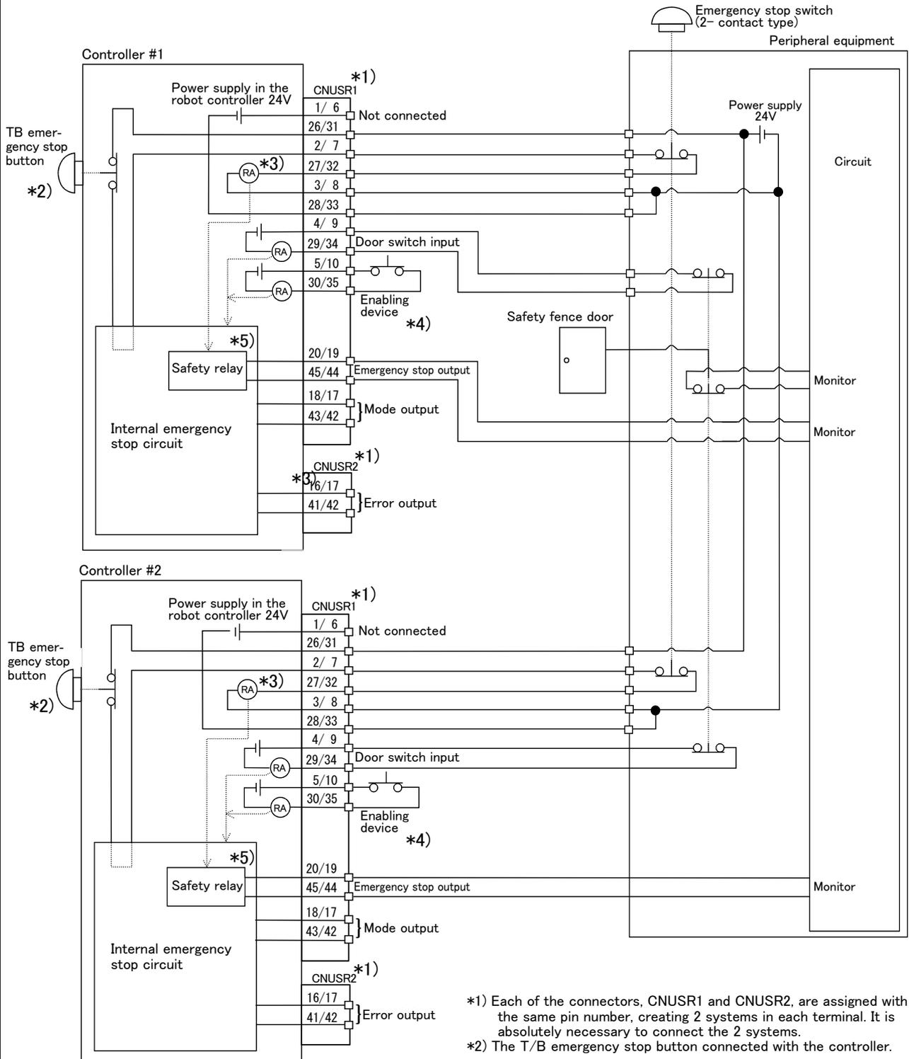
Fig.6-4 : Example of safety measures (CR751 wiring example 4)
