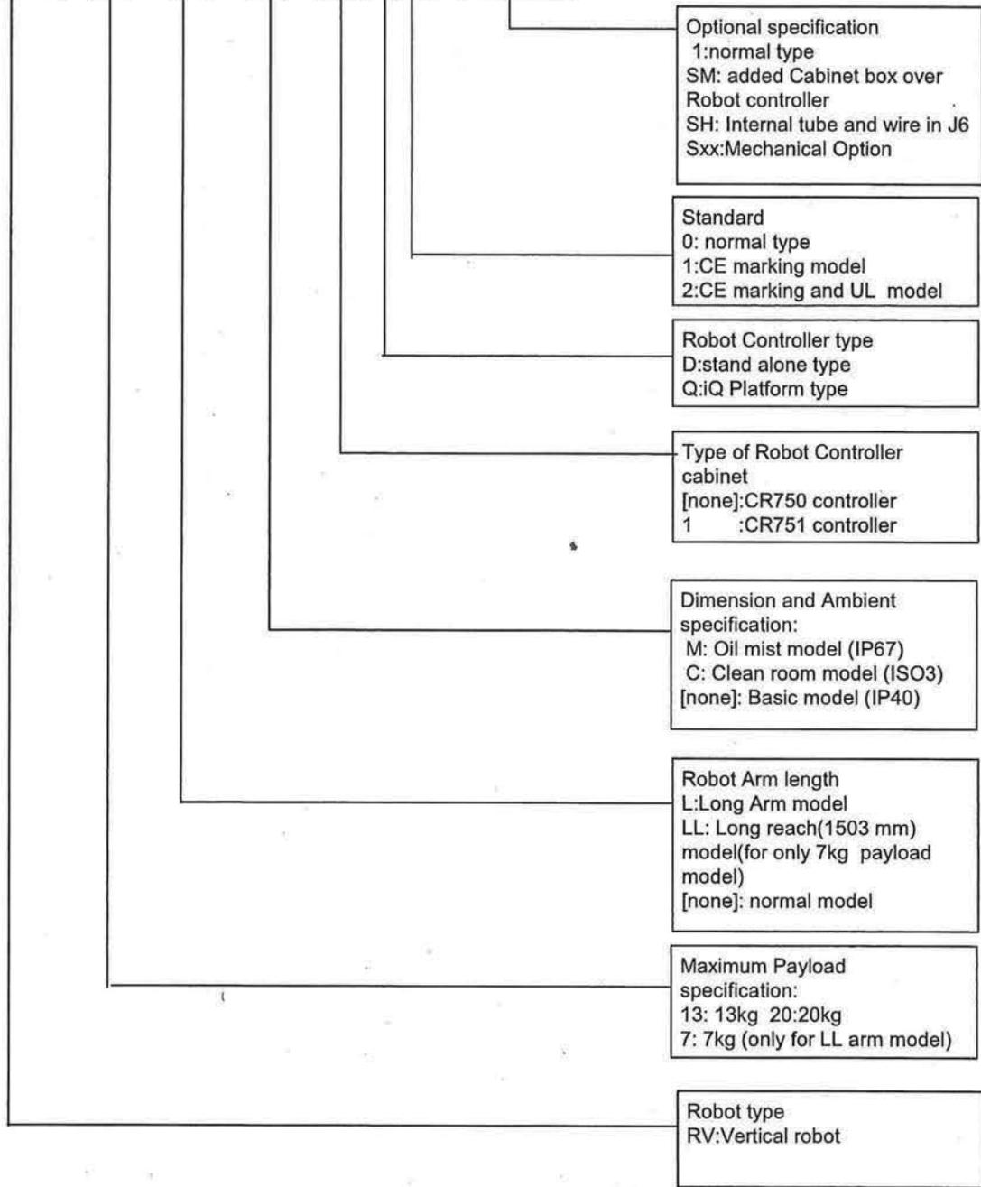
Fig.1-5 Nomenclature of F series robot of RV-13F,20F,7FLL series
