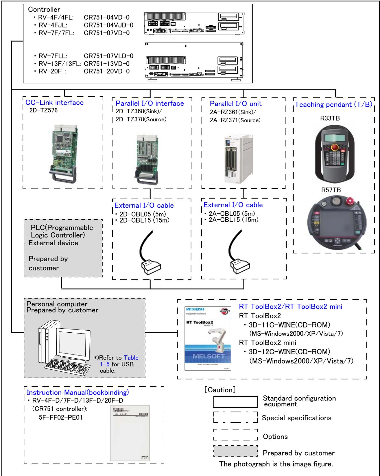
Fig.1-2 : Structural equipment
