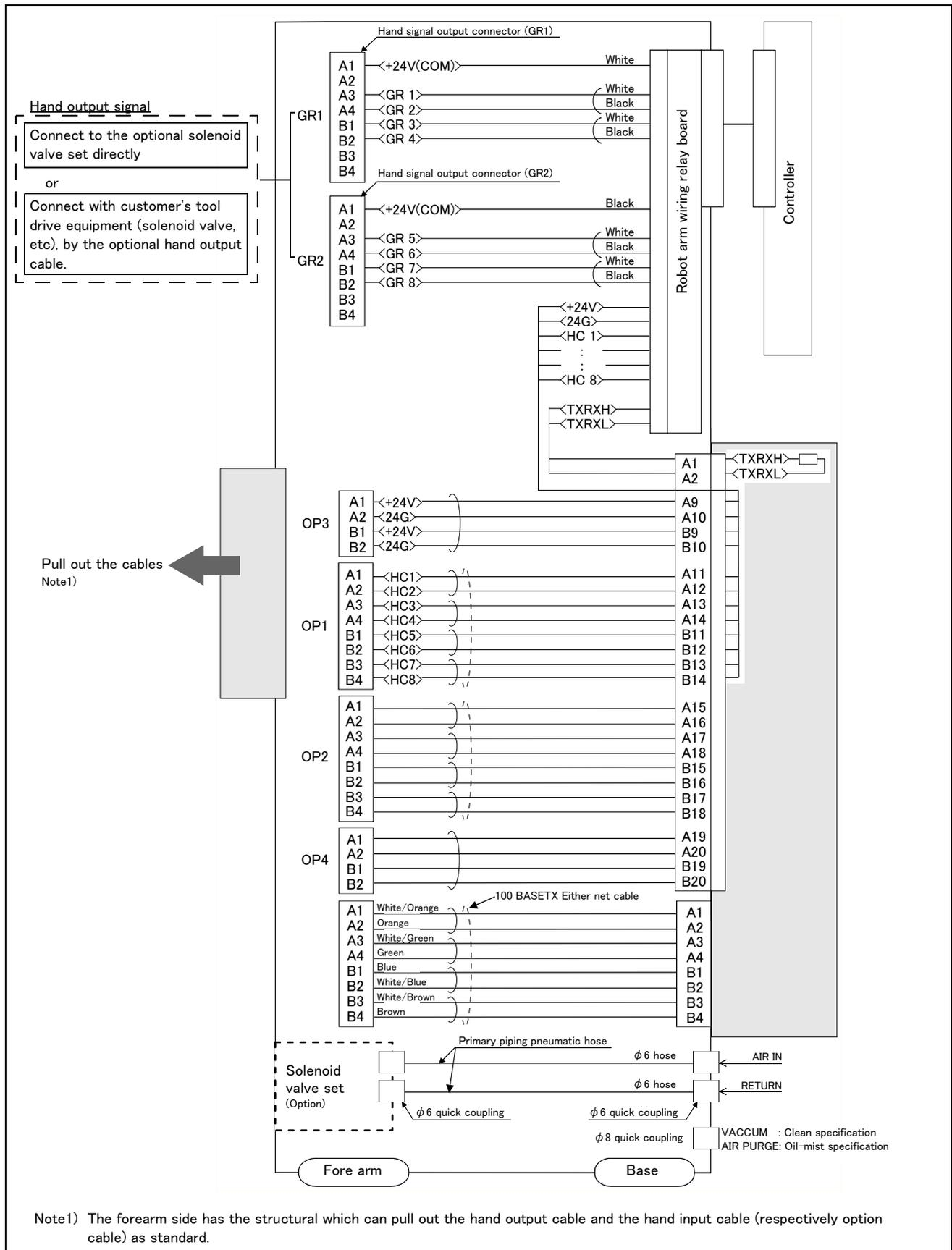
Fig.2-26 : Wiring and piping system diagram for hand and example the solenoid valve installation
