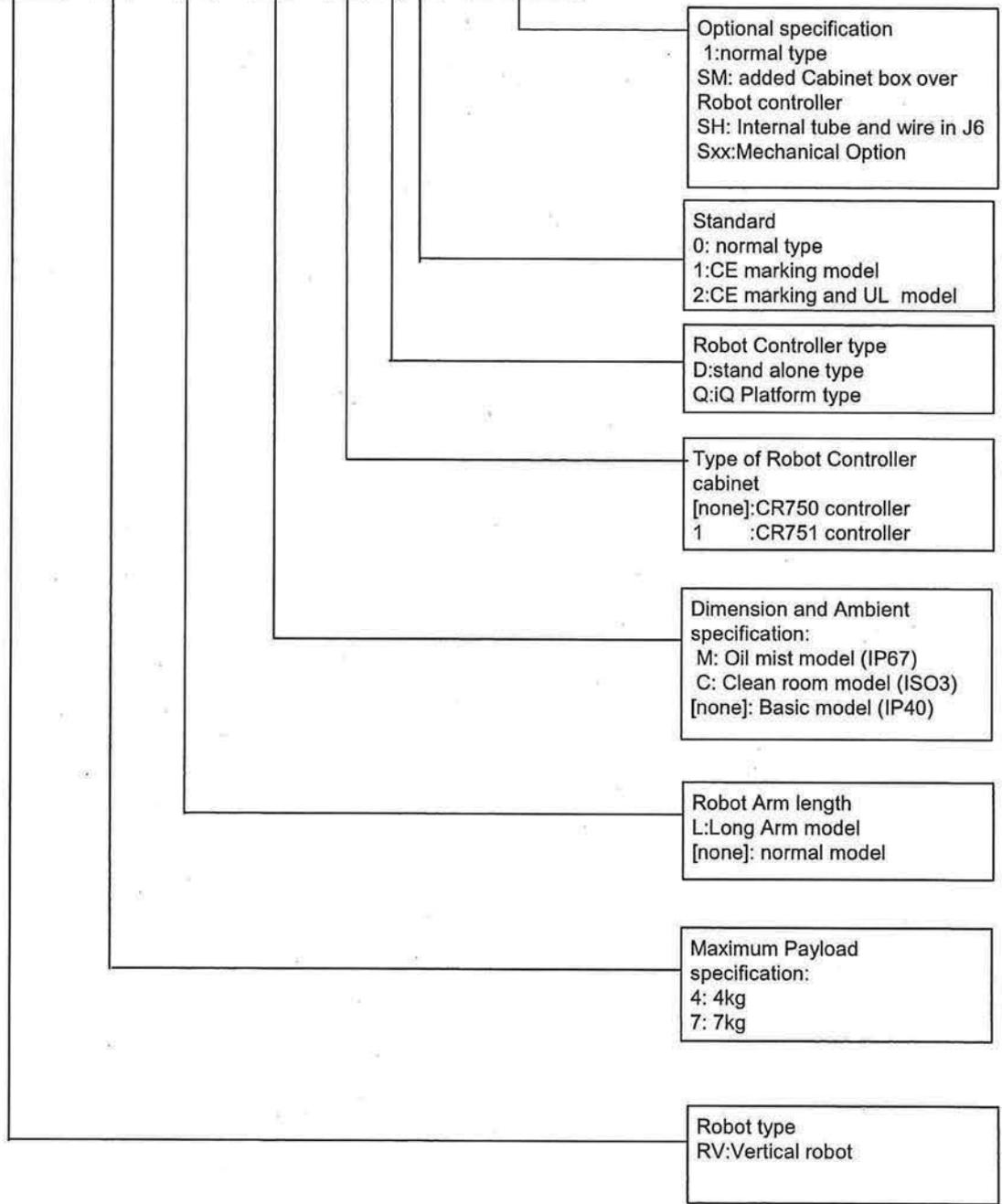
Fig.1-4 Nomenclature of F series robot of RV-4F,7F series
