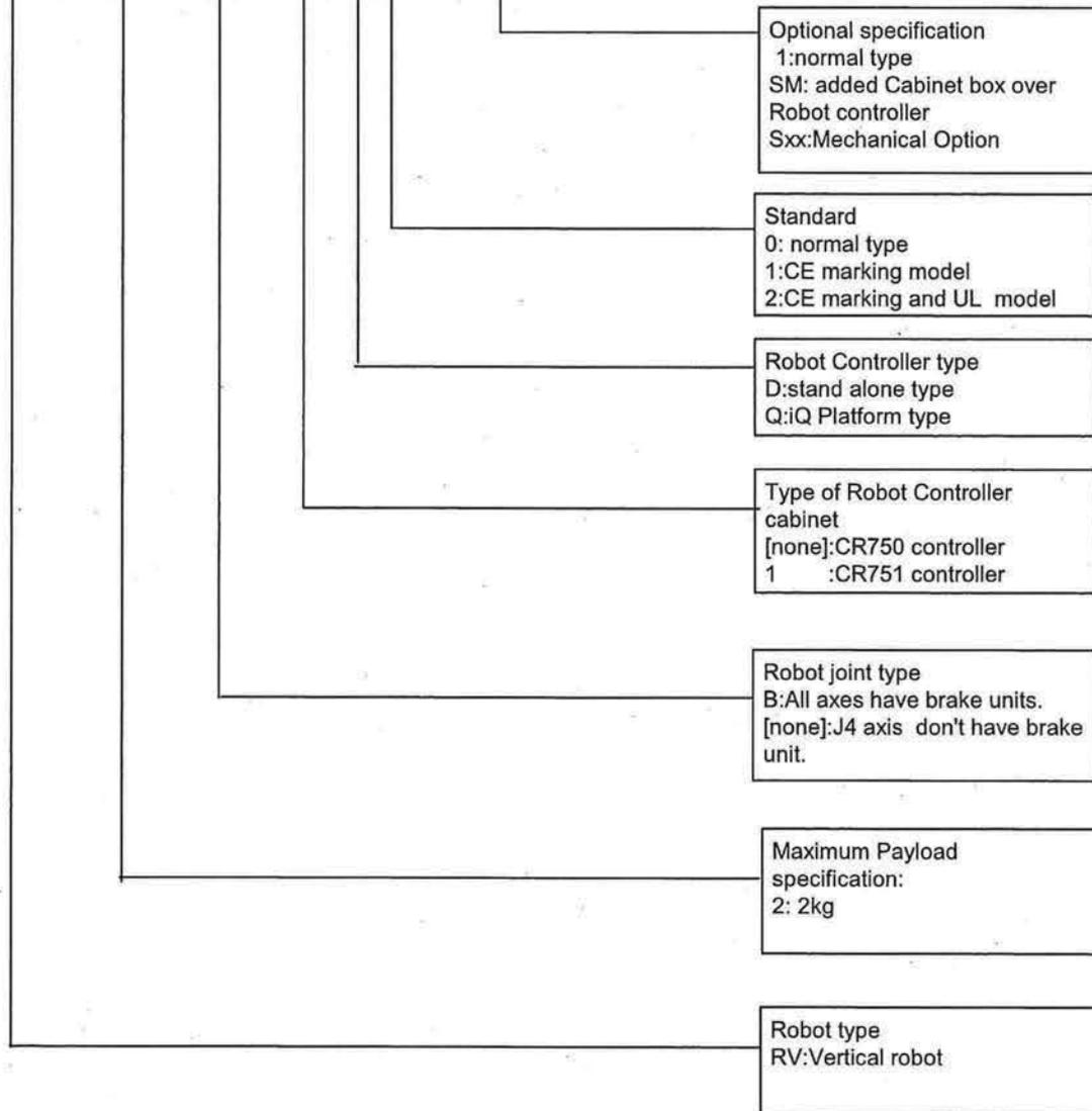
Fig.1-3 Nomenclature of F series robot of RV-2F series
