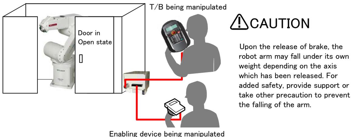
Fig.3-13 : Brake release operation
