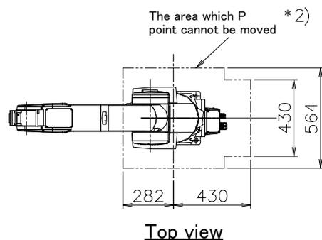
Fig.2-19 : Operating range diagram: RV-13FL
