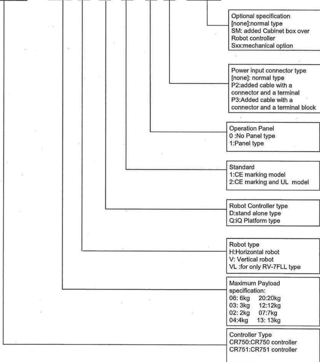
Fig.2-1 Nomenclature of F series robot controller
