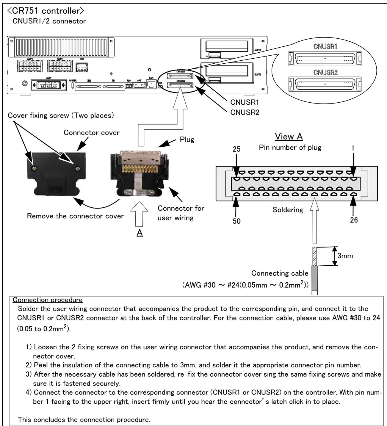
Fig.3-10 : Method of wiring for external emergency stop connection (CR751 (CNUSR1/2))
