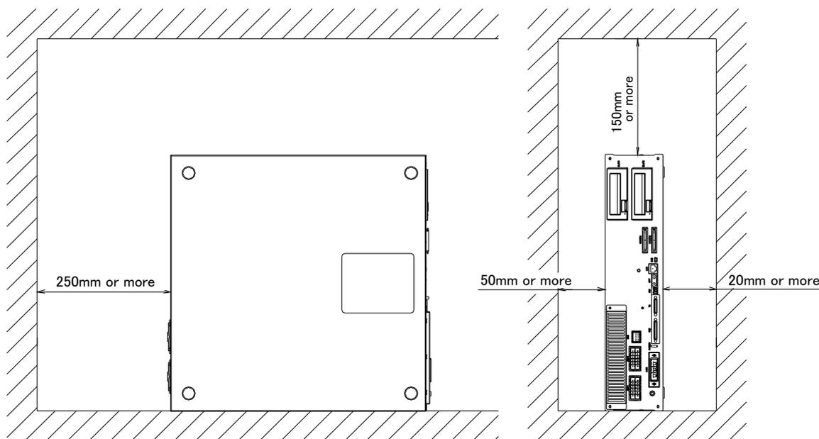
Fig.3-4 : Installation of controller (RV-4F/7F series)
