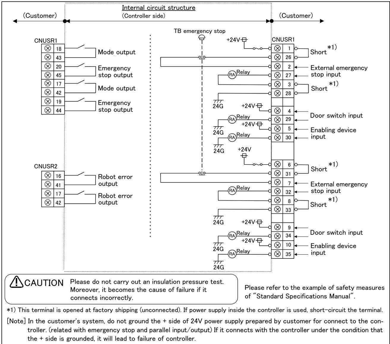
Fig.3-9 : External emergency stop connection (CR751)
