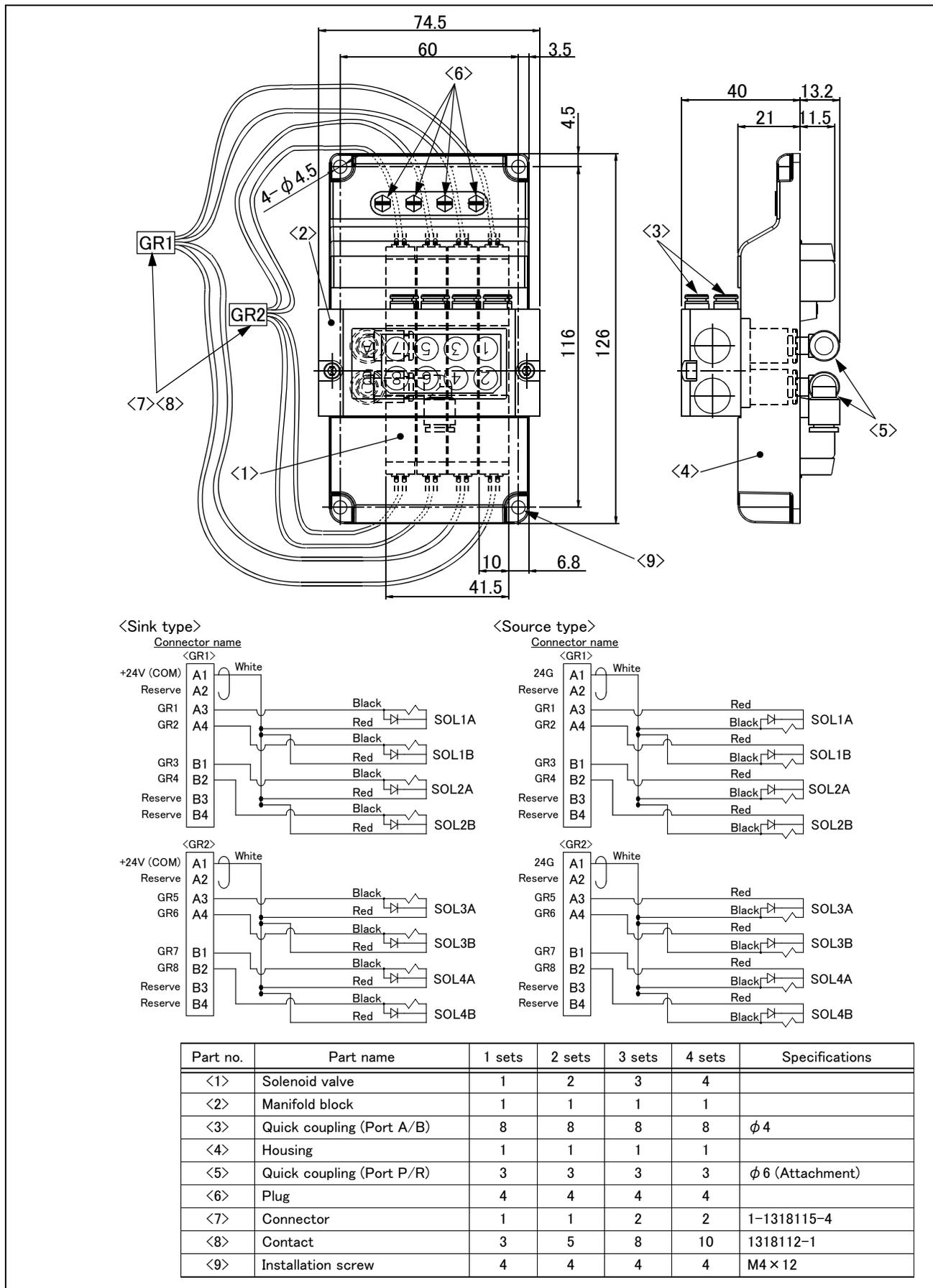
Fig.2-36 : Outline dimensional drawing (1F-VD0\*-02/1F-VD0\*E-02)
