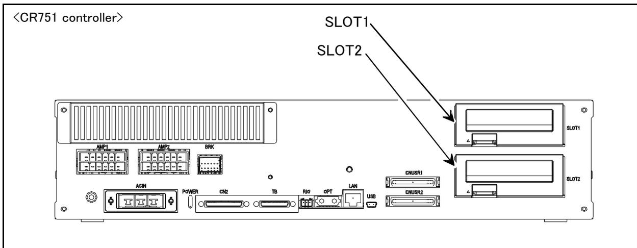
Fig.3-23 : Parallel I/O interface installation position (CR751)
