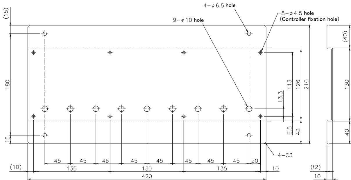
Fig.3-7 : Metal plate for fixation to placing vertically (Reference for RV-13F series)
