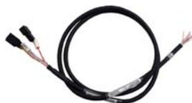
The hand input cable is used for customer-designed pneumatic hands. It is necessary to use this to receive the hand's open/close confirmation signals and grasping confirmation signals, at the controller. One end of the cable connects to the connector for hand input signals, which is in the wrist section of the hand. The other end of the cable connected to the sensor inside the hand customer designed.
