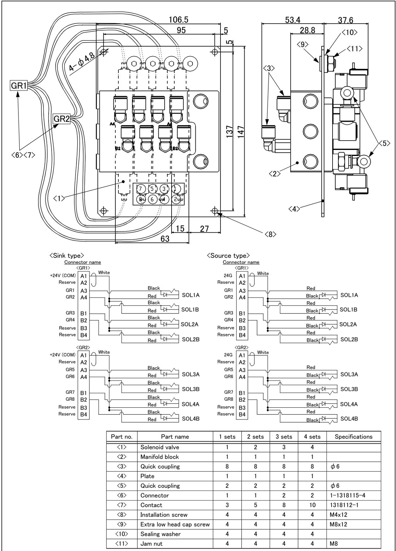
Fig.2-37 : Outline dimensional drawing (1F-VD0\*-03/1F-VD0\*E-03)
