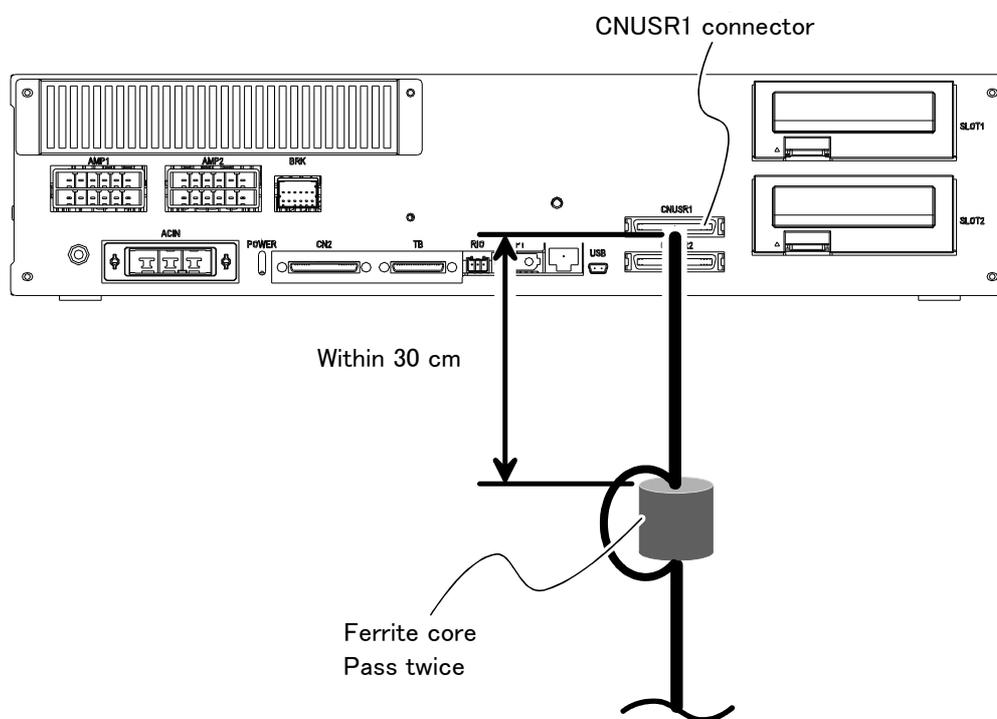
Fig.3-8 : Emergency stop cable connection (CR751)
