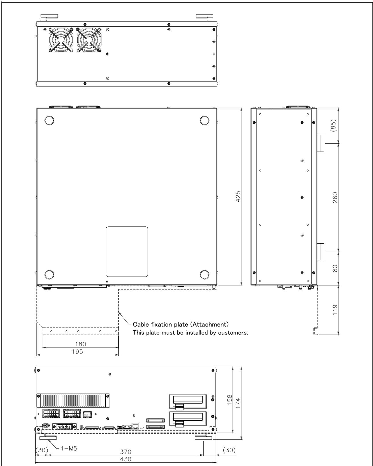
Fig.3-3 : Outside dimensions of controller (CR751: RV-13F series)
