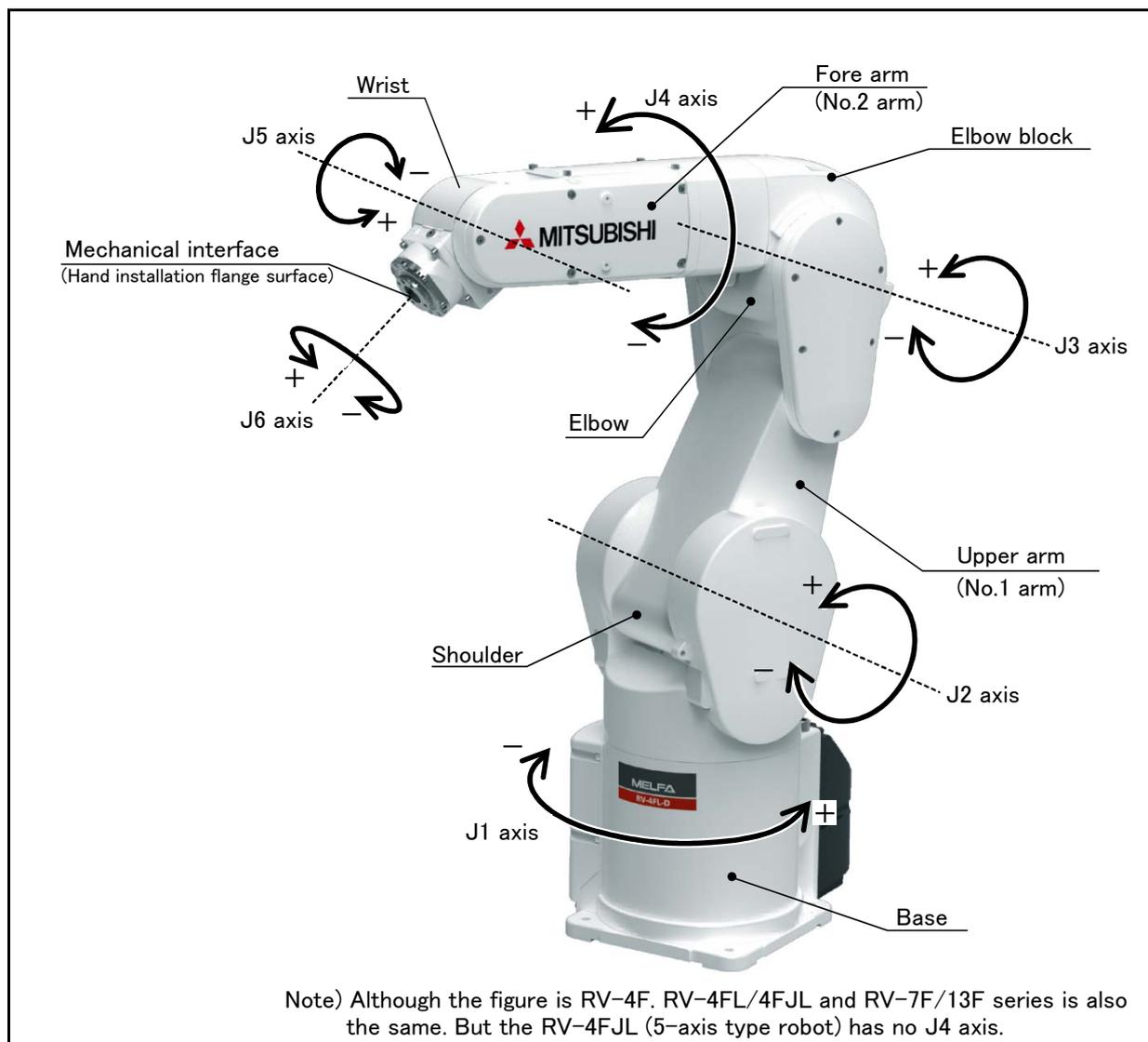
Fig.2-5 : Names of each part of the robot
