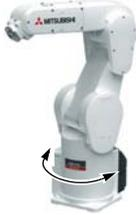
The operating range of J1 axis is limited by the robot arm's mechanical stopper and the controller parameters.
