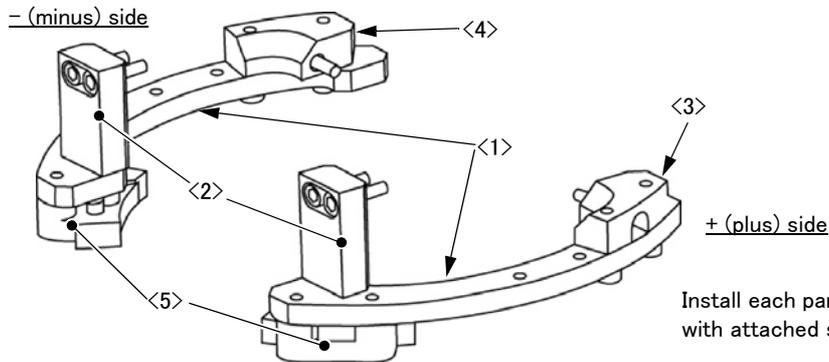
Install each parts to the upper arm lower part with attached screw.
