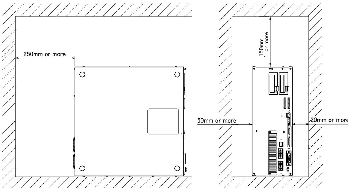
Fig.3-6 : Installation of controller (RV-13F series)
