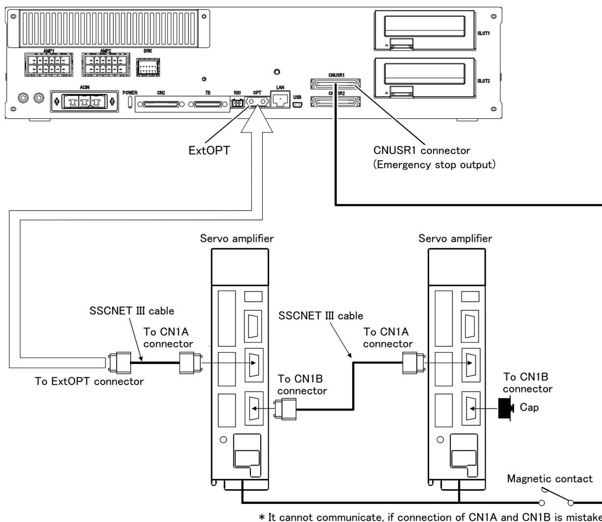
Fig.3-16 : Example of addition axis connection (CR751)
