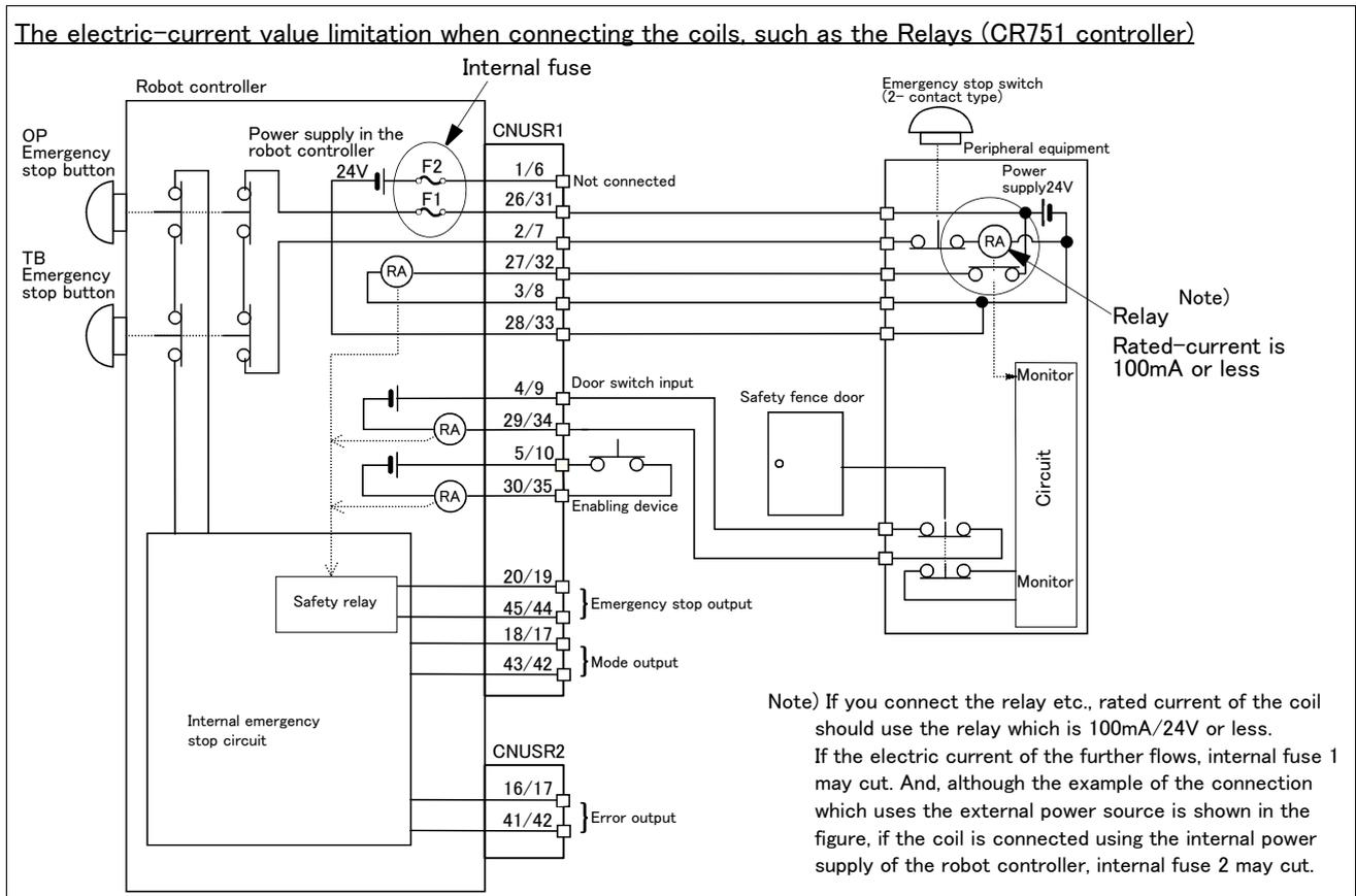
Fig.6-6 : Limitations when connecting the relay etc. (CR751)
