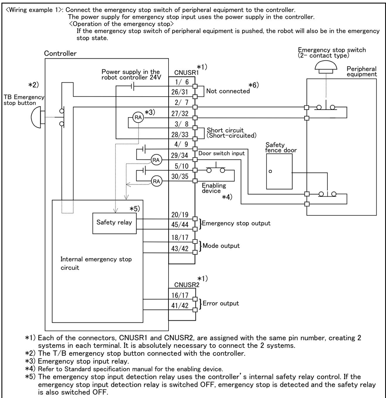
Fig.6-1 : Example of safety measures (CR751 wiring example 1)
