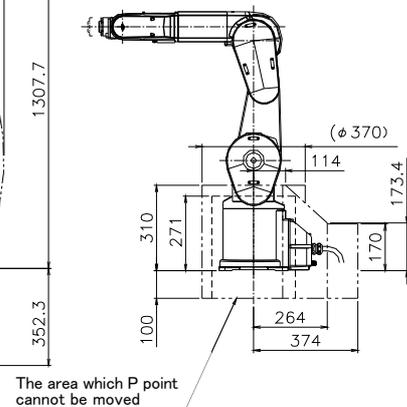
Fig.2-13 : Operating range diagram: RV-7FL
