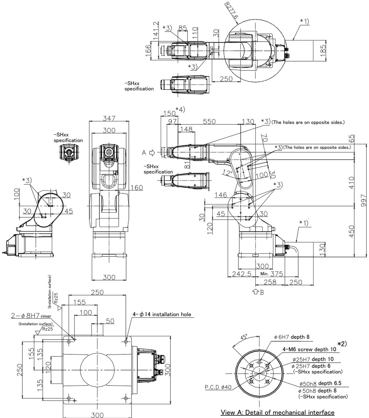
View B bottom view drawing: Detail of installation dimension
