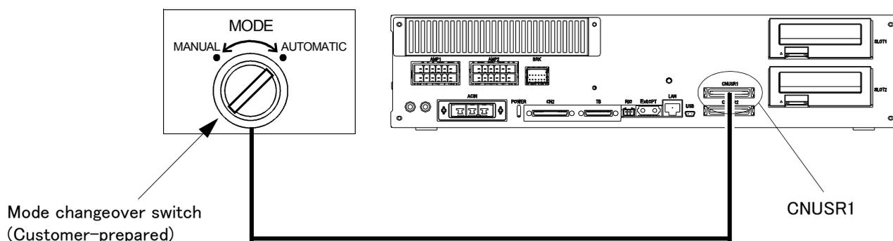
Fig.3-14 : Mode changeover switch image figure (CR751)
