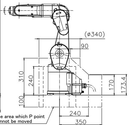
Fig.2-9 : Operating range diagram: RV-4FL/4FJL
