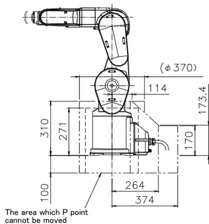
Fig.2-11 : Operating range diagram: RV-7F
