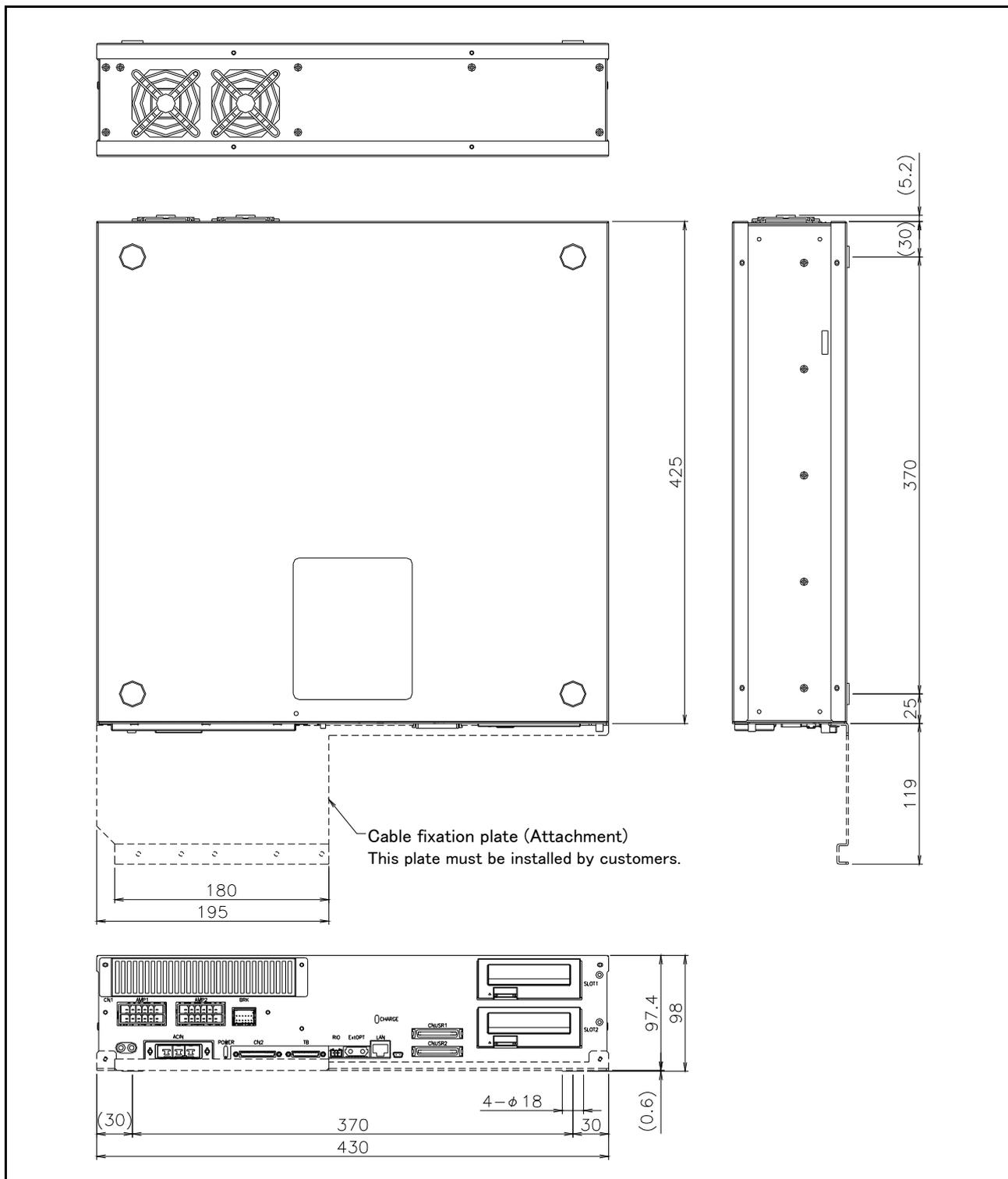
Fig.3-2 : Outside dimensions of controller (CR751: RV-4F/7F series)
