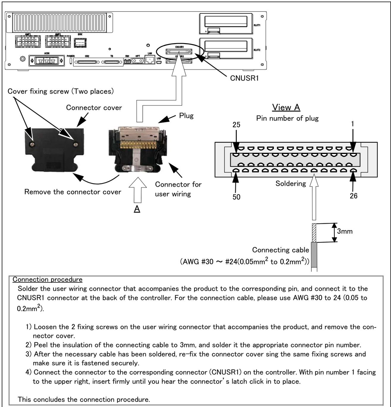
Fig.3-15 : Connection of the mode changeover switch input (CR751)
