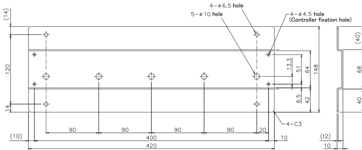
Fig.3-5 : Metal plate for fixation to placing vertically (Reference for RV-4F/7F series)
