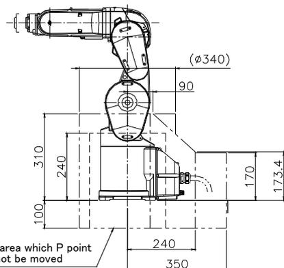
Fig.2-7 : Operating range diagram: RV-4F
