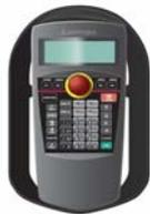
This is used to create, edit and control the program, teach the operation position and for jog feed, etc.
