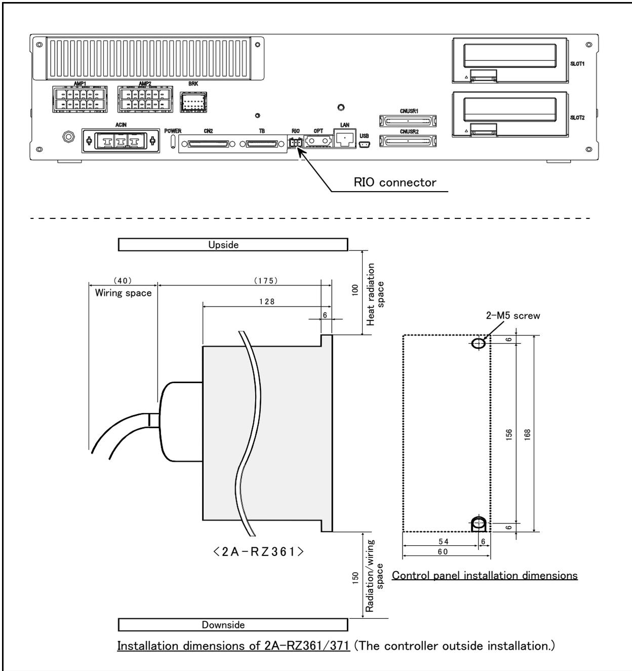
Fig.3-27 : Installing the parallel I/O unit (CR751)
