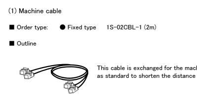
This cable is exchanged for the machine cable (5 m for fixed type) that was supplied as standard to shorten the distance between the controller and the robot arm.
