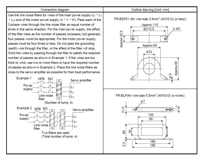
Fig.3-29 : Example of noise filter installation
