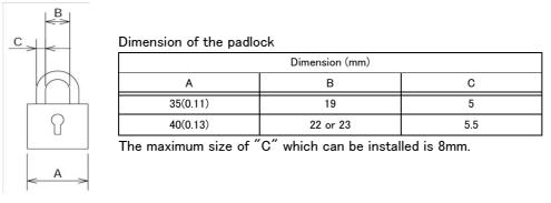
Fig.3-3 : Operation lock of the power switch(DU3-700)
