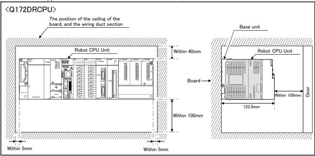
Fig.3-17 : Installation of robot CPU Unit
