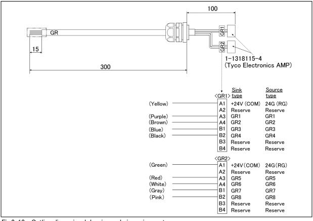
Fig.2-13 : Outline dimensional drawing and pin assignment
