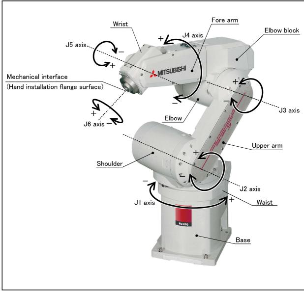
Fig.2-2 : Names of each part of the robot
