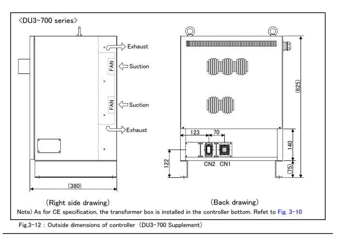
(2) Outside dimensions of robot CPU unit
