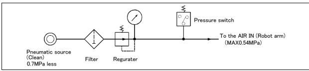
Fig.2-9 : Air supply circuit example for the hand
