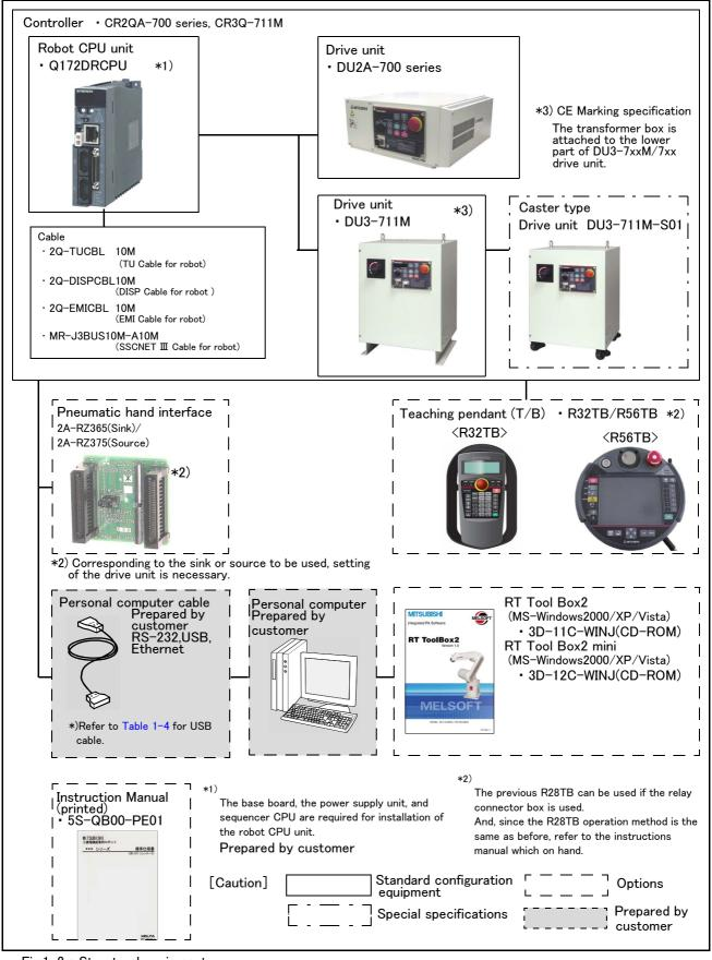
Fig.1-2 : Structural equipment
