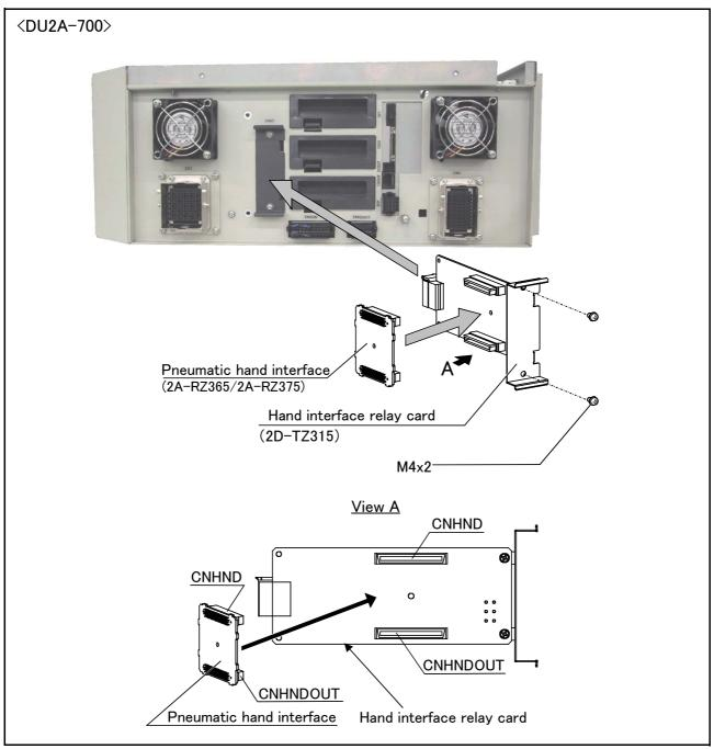
Fig.3-35 : Installation of the pneumatic hand interface (DU2A-700)
