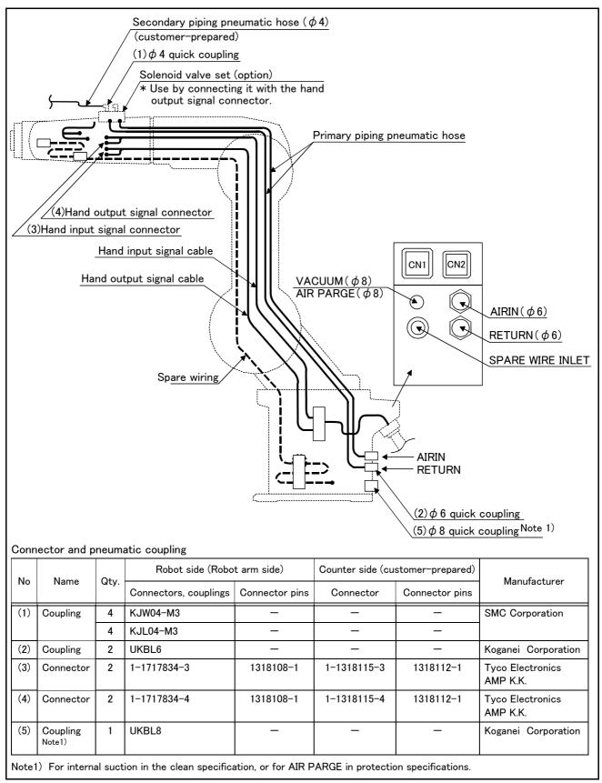
Fig.2-6 : Wiring and piping for hand
