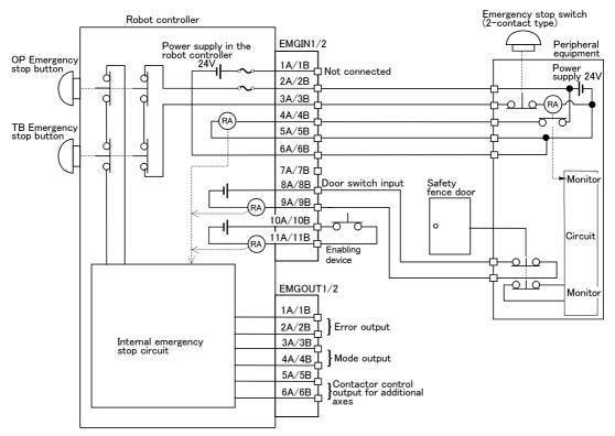
Fig.6-5 : Limitations when connecting the relay etc.
