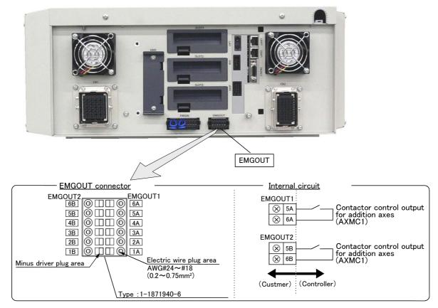
Fig.3-31 : EMGOUT connector (DU2A-700)
