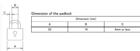
Fig.3-2 : operation lock of the power switch(DU2A-700)
