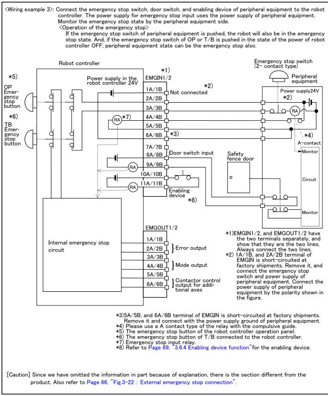
Fig.6-3 : Example of safety measures (Wiring example 3)
