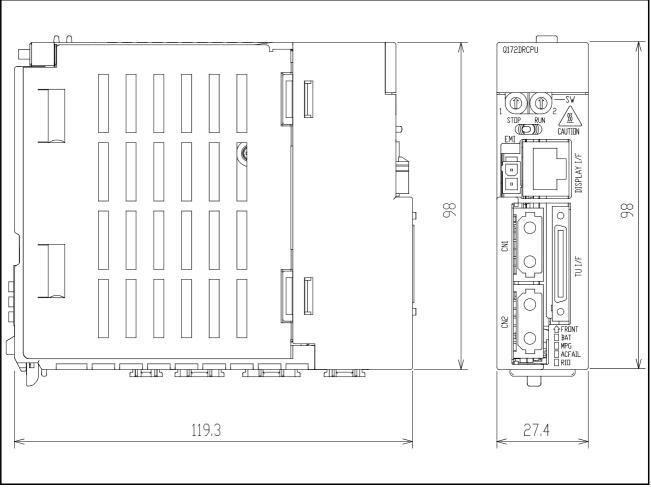
Fig.3-13 : Outside dimensions of robot CPU
