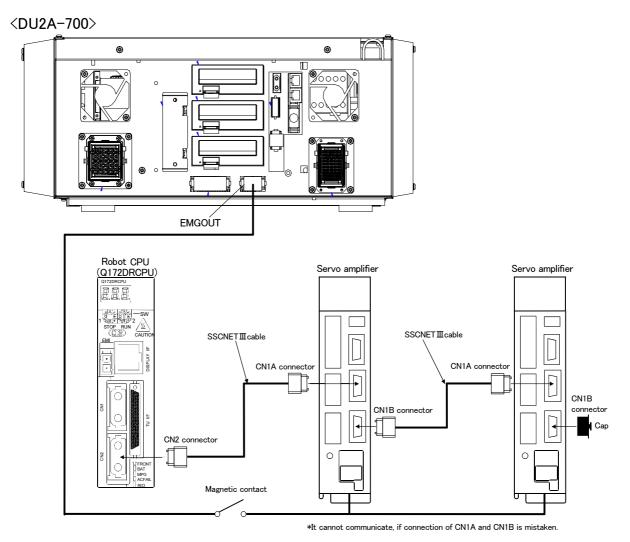
Fig.3-26 : Example of addition axis connection (DUA2-700)
