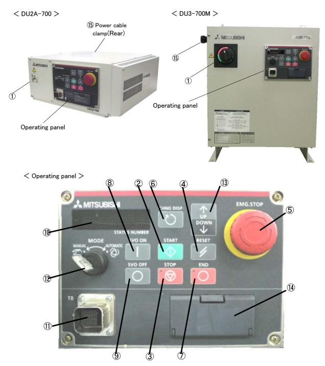
Fig.3-1 : Names of drive unit parts
