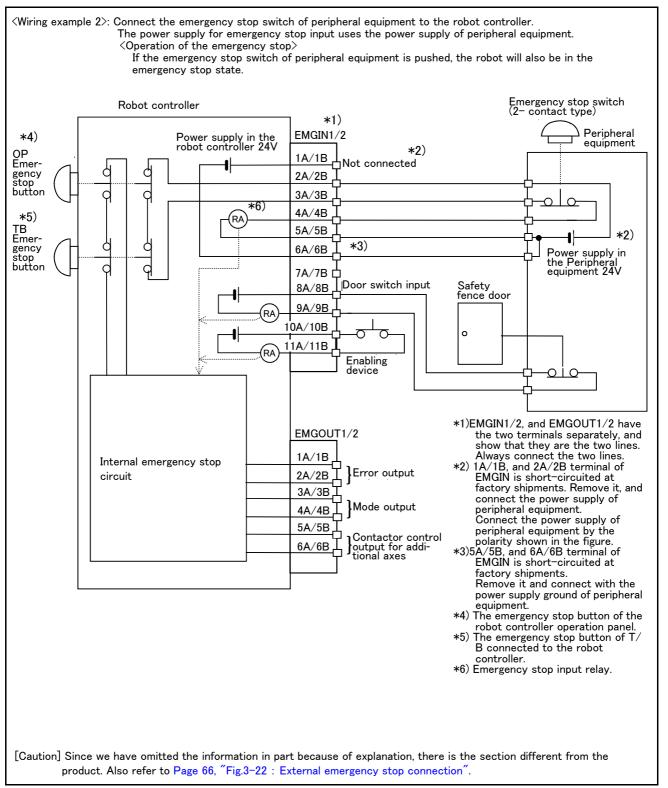
Fig.6-2 : Example of safety measures (Wiring example 2)
