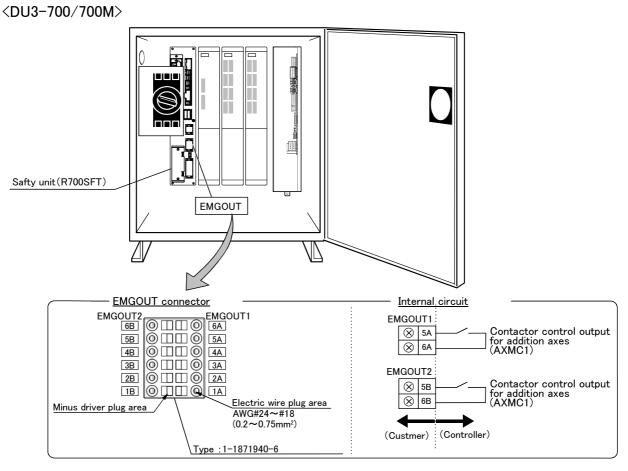
Fig.3-32 : EMGOUT connector (DU3-700/700M)
