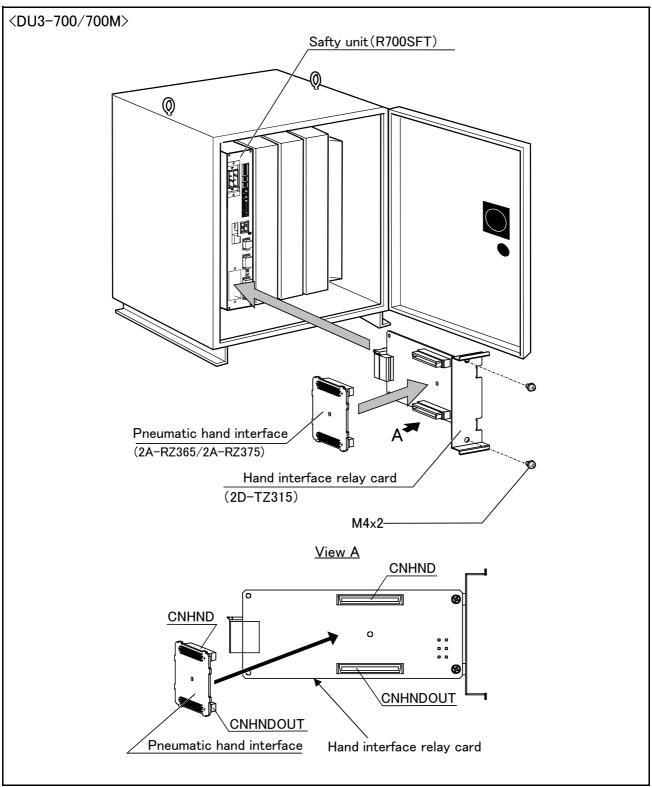
Fig.3-36 : Installation of the pneumatic hand interface (DU3-700/700M)
