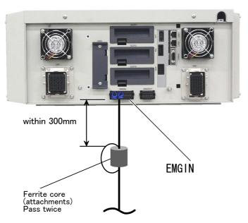
Pin allotment of EMGIN and the EMGOUT connector is shown in Fig. 3-22.
