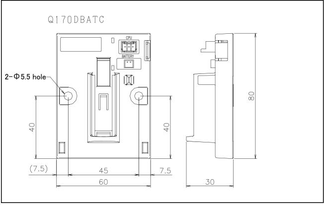
Fig.3-14 : Outside dimensions of battery unit
