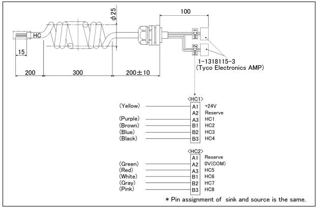
Fig.2-12 : Outside dimensional drawing and pin assignment
