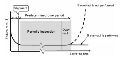
Fig.2-15 : Periodic inspection/overhaul periods
