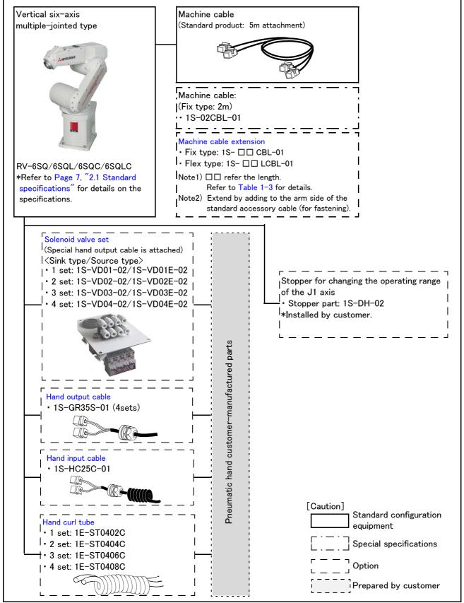
Fig.1-1 : Structural equipment (Robot arm)
