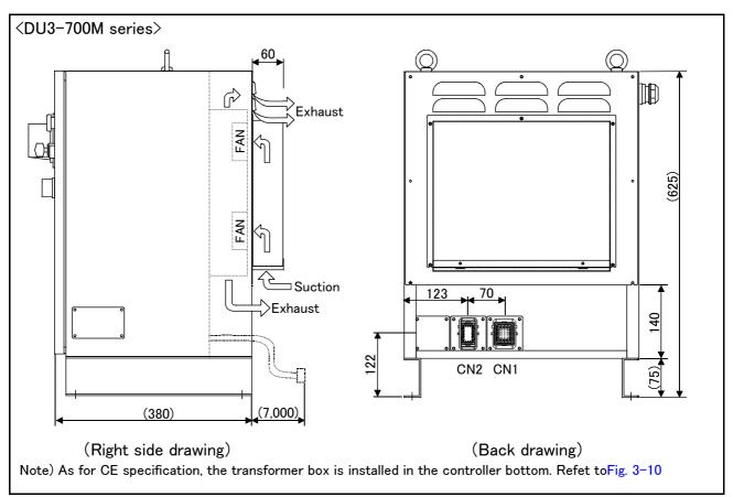
Fig.3-11 : Outside dimensions of controller (DU3-700M Supplement)
