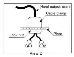
Fig.3-5: Installing the hand output cable
