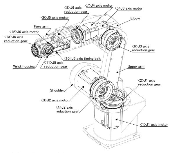
Fig 5-2: Outline structure of robot arm
