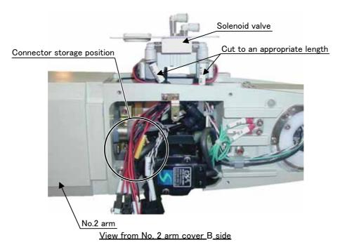
Fig.3-2: Solenoid valve installation diagram details 1
