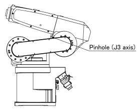
7) Move the J3 axis slowly toward the front using both hands. Align the pinhole of the No.1 arm and the pinhole at the base section, feed through the origin jig ( $\phi$ 8) into the pinholes and fasten.
