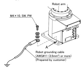
Fig.2-5: Connecting the grounding cable
