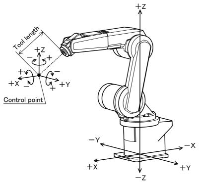
st While maintaining the flange surface posture, the axis moves straight along the base coordinate system.
