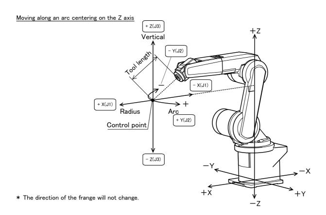
Assuming that the current position is on an arc centering on the Z axis, the robot moves along that arc.
