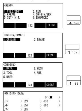
1) Press the [4] key on the menu screen, and display the ORIGIN/BRAKE screen.
