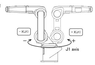
• When the [+X (J1)] keys are pressed, the J1 axis will rotate in the plus direction. When the [-X (J1)] keys are pressed, Rotate in the minus direction.
