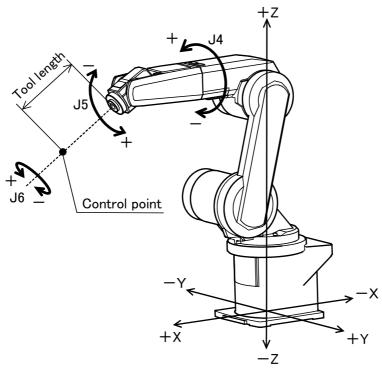
\* The axis moves straight along the base coordinate system. At this time, the flange surface posture is not maintained.
