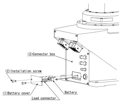
Fig.5-13: Replacing the battery
