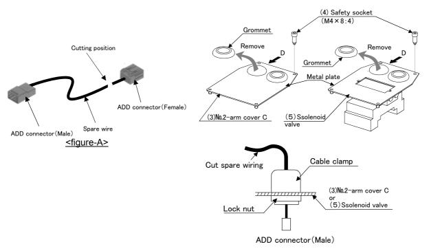
Fig.2-8: Installation and connection of spare wiring
