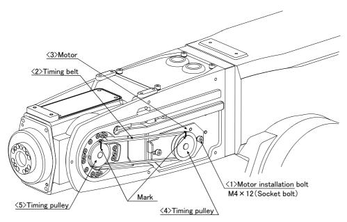
Fig.5-9: Inspection, maintenance and replacement of J5-axis timing belt
