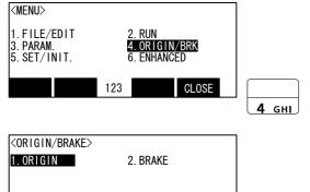
1) Press the [4] key on the menu screen, and display the Origin/Break selection screen.
