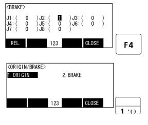
8) Detach the [F1] key and work the brake. Press the [F4] key and return to the origin / brake screen.
