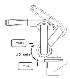
• When the [+Y (J2)] keys are pressed, the J2 axis will rotate in the plus direction. When the [-Y (J2)] keys are pressed, Rotate in the minus direction.
