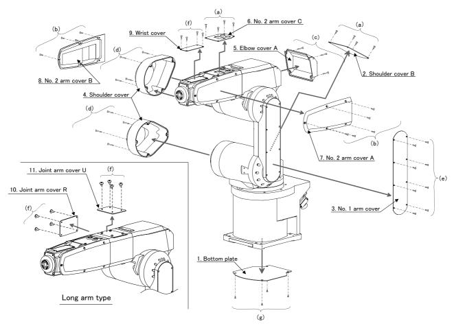
Fig.5-3 : Installing/removing the cover
