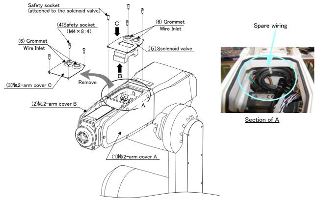
Fig.2-7: Drawer of spare wiring (Fore arm side)
