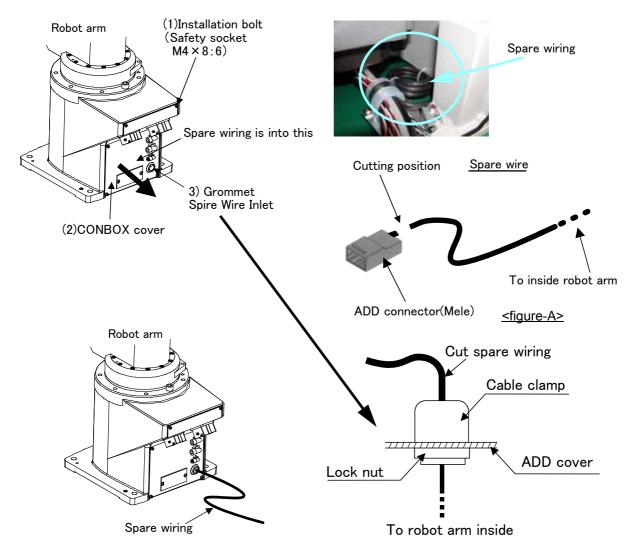
Fig.2-9: Pull out spare wiring(Base area)
