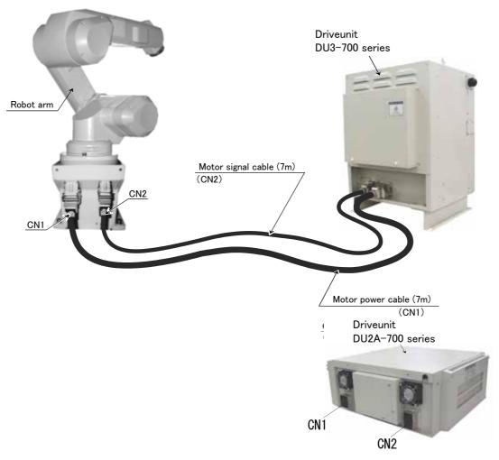
Fig.2-6: Connecting the machine cables
