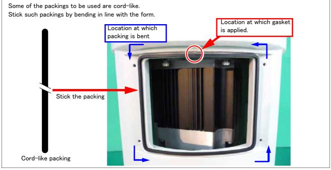
Fig.5-6: Sticking the cord-like packing
