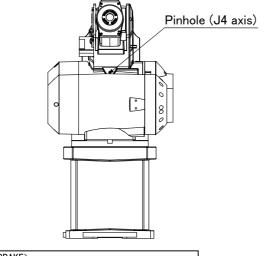
7) Slowly rotate the J4 axis in the direction of minus with both hands. Align the pinholes of the No. 1 arm and shoulder, feed through the origin jig ( $\phi$ 6) into the pinholes and fasten.
