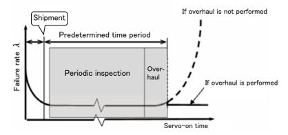
Fig.5-14: Periodic inspection/overhaul periods
