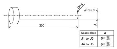
Fig.5-15: Reference dimension of origin setting tool
