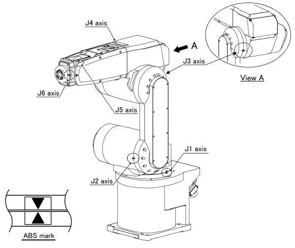
Fig.5-16: ABS mark attachment positions
