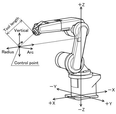
\* The current position is set as the arc centering on the Z axis, and the axis moves along that arc, expands and contracts in the radius direction, and moves vertically. At this time, the flange surface posture is maintained. Also, while maintaining the flange surface position, the flange surface posture changes.
