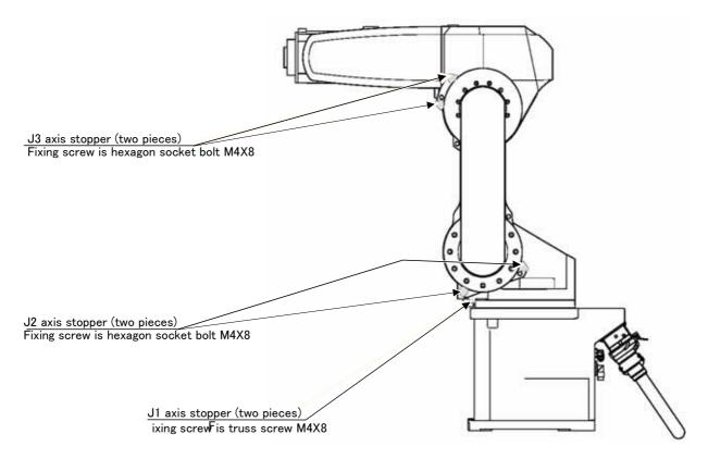
Fig.5-12: Stopper installation position
