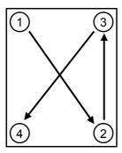
$\ensuremath{\mathsf{Fig.5-8}}$  : Example of order which tighten bolts
