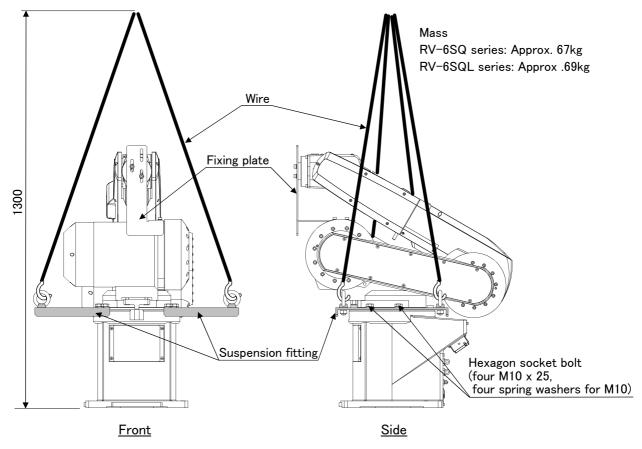
Fig.2-2: Transportation procedures (transporting with a crane)
