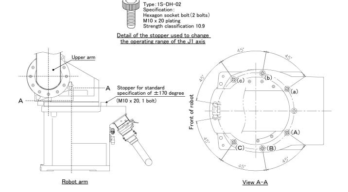
Fig.3-6: Installation of operating range change option
