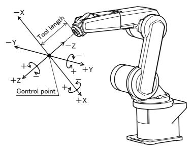
\* While maintaining the flange surface posture, the axis moves straight along the tool coordinate system.
