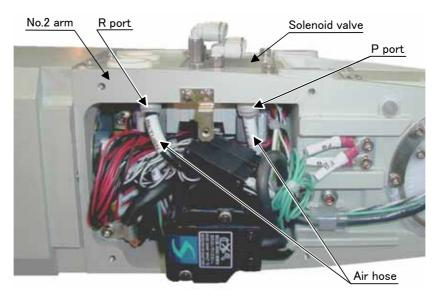
Fig.3-3: Solenoid valve installation diagram details 2
