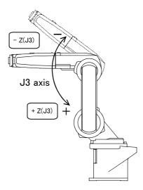
• When the [+Z (J3)] keys are pressed, the J3 axis will rotate in the plus direction. When the [-Z (J3)] keys are pressed, Rotate in the minus direction.
